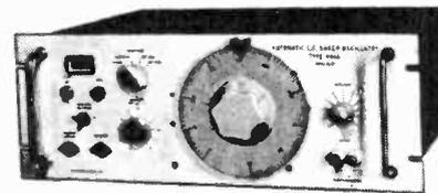
5 Hz-5 KHz 21 sweep speeds from 0.1-10 octaves/minute. Variable O/P up to 10 v. r.m.s. Mains I/P. Excellent condition. **£95.** Carriage extra.
