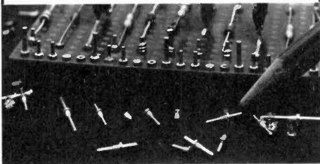
The extensive range of Oxley Snales now include an Eyelet version (which is ideally suited for mounting I.C. Packs and other components for experimental work). They augment the well known standard range of Oxley "Snales" suitable for mounting in 0.040 inches, 0.050 inches diameter holes.
