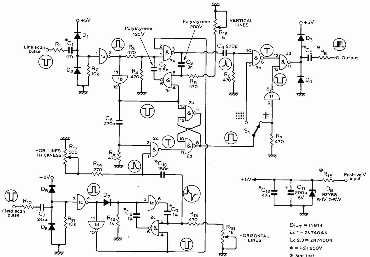
Fig. 1. Block diagram of the crosshatch generator.
