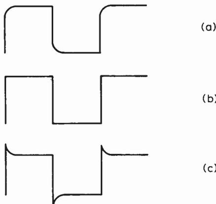
Fig. 2. With the capacitors  $C_1$  and  $C_2$  properly adjusted a square wave is correctly reproduced (b). Too small capacitance gives rounded corners (a) while too much capacitance gives overshoot (c).
