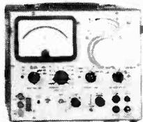
Two light weight units provide level measurements at any audio frequency in 140 and 600 systems, even in the presence of other signals.
