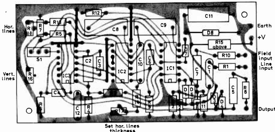
Fig. 2 (Upper) Photograph of the printed circuit board shown actual size (101 mm in length). (Below) Drawing of the component side of the board.
