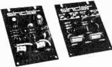
The Z.30 and Z.50 are of advanced design using silicon epitaxial planar transistors to achieve unsurpassed standards of performance. Total harmonic distortion is an incredibly low 0.02% at full output and all lower outputs. Whether you use Z.30 or Z.50 amplifiers in your Project 60 system will depend on personal preference, but they are the same size and may be used with other units in the Project 60 range equally well.
