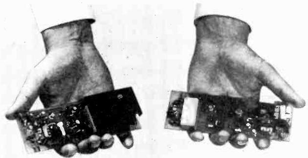
*Transmitter and receiver use plug-in modules for ease of servicing. Low-noise high-gain receiver employs dual gate MOSFET RF devices in conjunction with fast attack, slow release AGC, to give exceptional immunity to blocking and cross modulation and performance approaching base station standards.*
