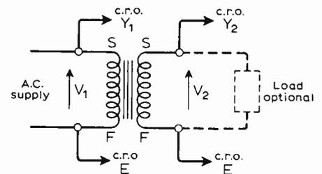
*If the starts and finishes of the windings are not marked they can be quickly established by measuring the inductance of the two windings in series. The connection giving the larger inductance is that in which the finish of one winding is connected to the start of the other winding.*
