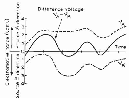
Fig. 3. Graphical illustration of what happens in Fig. 2 over a period of time. At any instant the voltage in the solid-line graph is the result of subtracting  $v_B$  from  $v_A$ .
