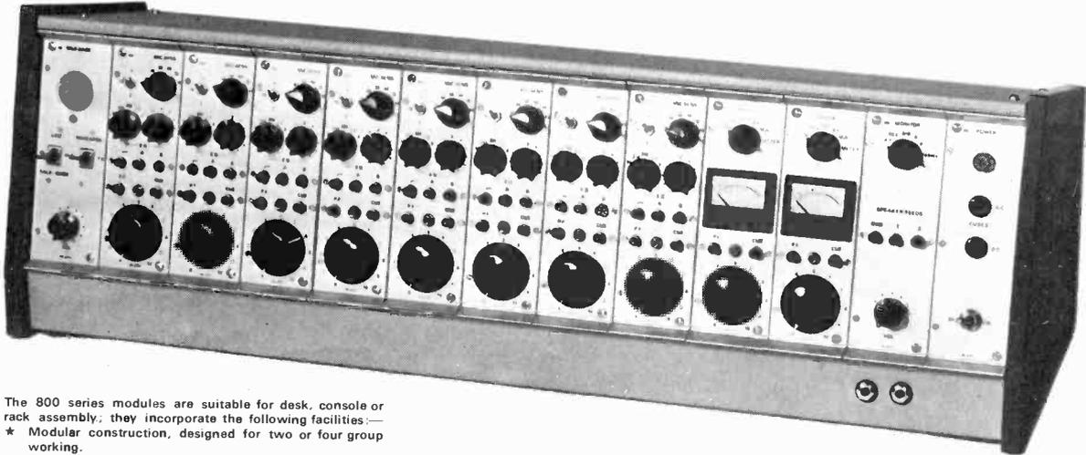
The 800 series modules are suitable for desk, console or rack assembly; they incorporate the following facilities:—
