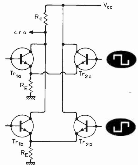
Fig. 5. This diagram shows the two output stages  $Tr_1$  of the two signal channels. These are turned on and off alternately by transistors  $Tr_2$  which are in turn driven on and off by push-pull square waves on their bases.
