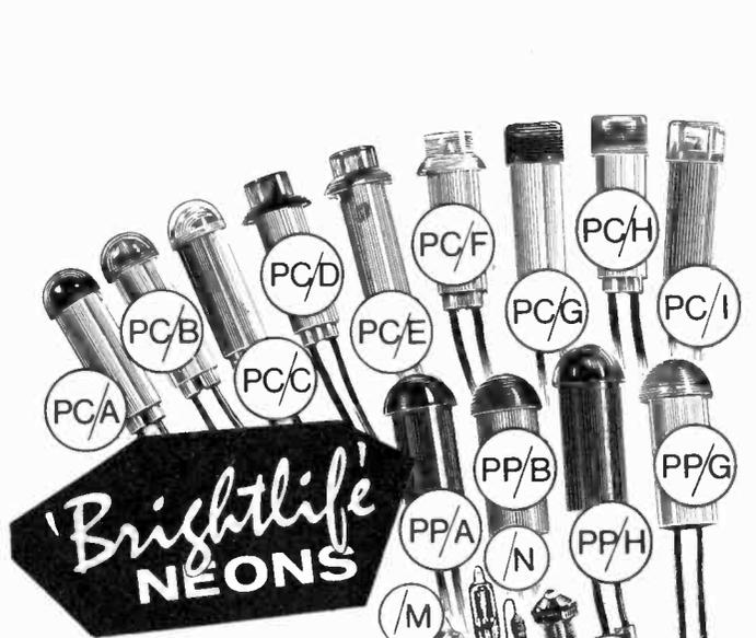
'Brightlife' neons give greater brightness and 25,000 hours average life. The 1/2" diameter neons are moulded in polypropylene which diffuses the light and the 3/4" diameter neons are moulded in polycarbonate which gives higher light transmission. Both types give a glow behind the panel to warn maintenance staff. Units are one hole fixing 1/2" and 3/4" diameter clearance.
