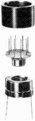
The ovens have no moving parts or electronic circuitry but incorporate a semiconductor heater to provide a self-regulating proportional temperature control. Power requirements are 24V ( $\pm 4V$ ) a.c./d.c. 0.6W (at 25°C ambient). Maximum warm-up time from -55°C is 3 minutes. Jermyn Industries, Manufacturing Division, Vestry Estate, Sevenoaks, Kent.
