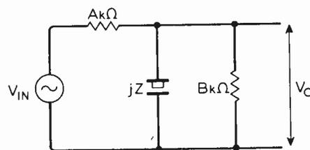
Fig. 1 The familiar circuit used to study the charging of a capacitor.
