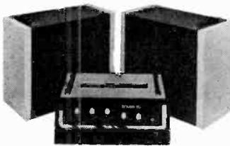
*Output Power* 45 watts R.M.S. (Sine wave drive). *Frequency response:* -3 db points 30 Hz at 18 KHz. *Total distortion:* less than 2% at rated output. *Signal to noise ratio:* better than 60 db. *Speaker Impedance:* 3, 8 or 15 ohms. *Bass Control Range:* ±13 db at 60 Hz. *Treble Control Range:* ±12 db at 10 KHz. *Inputs:* 4 inputs at 5 mV into 470 K. Each pair of
