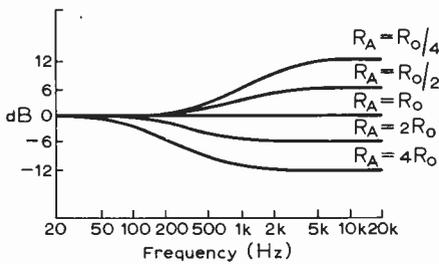
Fig. 4. Operation of tone-balance control,  $R_A$  in Fig. 3.
