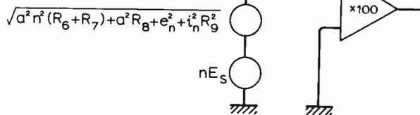
generated by the amplifier current noise flowing through the total resistance in the transformer secondary. This voltage source is in series with an equivalent resistance *R<sub>9</sub>*. The amplifier is approximated by a noiseless, infinite input impedance amplifier with a gain of 100.
