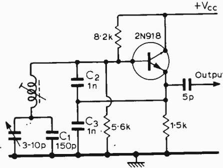
In this Gouriet-Clapp oscillator overall temperature coefficient was reduced to +3 p.p.m./deg C by using the simple equations in this article and making  $C_1$  a parallel combination of a silvered mica capacitor and a polystyrene capacitor.
