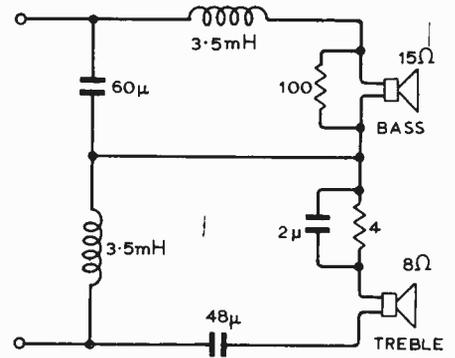
Fig. 3. Crossover circuit using a  $\frac{1}{2}$ -section series network. Resistors can be  $\frac{1}{2}W$ .
