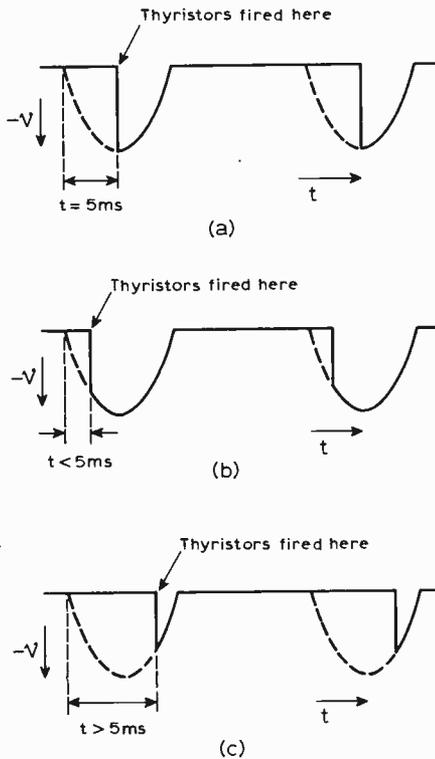
Fig. 4. Optimum firing conditions for good current stabilization.
