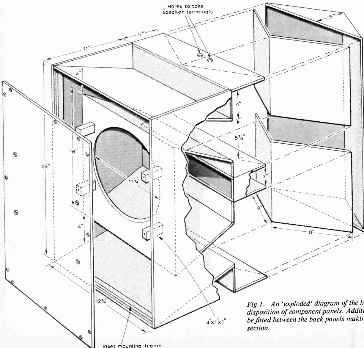
Fig. 1. An 'exploded' diagram of the bass horn showing disposition of component panels. Additional bracing should be fitted between the back panels making up the corner section.
