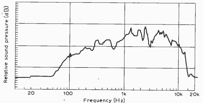
*Decca DPT receiver. (left) Frequency response of audio amplifier; signal fed across volume control; output loaded with 15Ω. (right) Frequency response from loudspeaker with input signal as before; 1V r.m.s. across l.s. at 1kHz. Mic. as above.*
