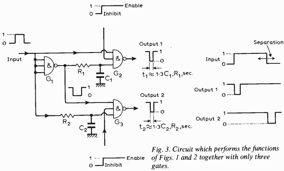
Fig. 3. Circuit which performs the functions of Figs. 1 and 2 together with only three gates.
