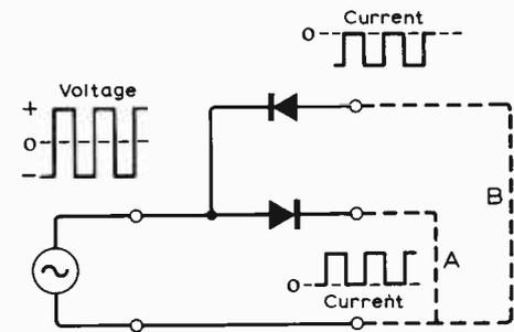
Fig. 3. Use of rectifiers for "steering" parts of input waveforms into different circuits, A and B.
