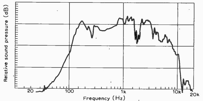
*Philips G23T212-02 receiver. (left) Frequency response of audio amplifier; signal fed to top of volume control and earth; output loaded with 35Ω. (right) Frequency response from loudspeaker with input signal as before; 1V r.m.s. across l.s. at 1kHz. Mic. as above.*
