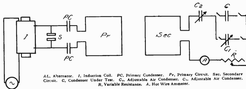
A.L., Alternator. I, Induction Coil. PC, Primary Condenser. Pr, Primary Circuit. Sec, Secondary Circuit. C, Condenser Under Test. C<sub>2</sub>, Adjustable Air Condenser. C<sub>1</sub>, Adjustable Air Condenser. R, Variable Resistance. A, Hot Wire Ammeter.
