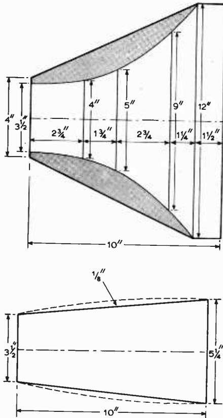
Fig. 2. Details of wood sections used in constructing the treble horn. The side sections should be cut along the curve shown dotted (see text).
