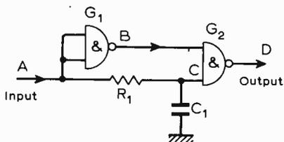
Fig. 2. As Fig. 1 except that the output pulse occurs on the trailing edge of a logical-1 input pulse.
