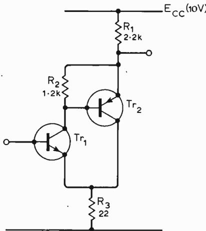
of the order 200kΩ, assuming transistors with current gains of the order 150 to 300 are used in the circuit. The voltage gain of the circuit is then given approximately by the formula
