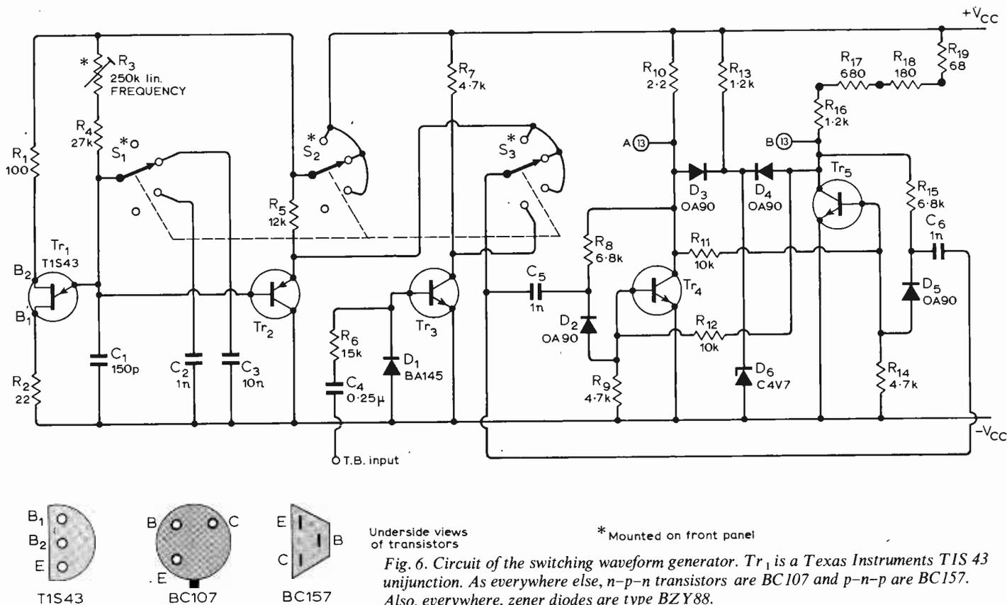
Fig. 6. Circuit of the switching waveform generator.  $Tr_1$  is a Texas Instruments TIS 43 unijunction. As everywhere else, n-p-n transistors are BC107 and p-n-p are BC157. Also, everywhere, zener diodes are type BZY88.
