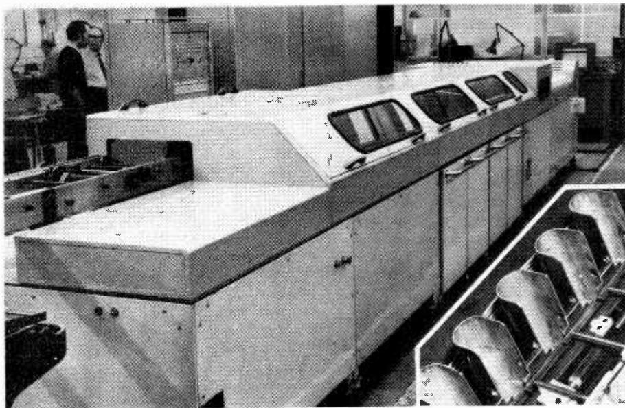
Mullard's semiconductor testing machine Apollo. Jigs containing batches of the devices to be tested are loaded into the rack on the left. The computer installation can be seen in the background. The insert shows five of the 36 shutes which lead to the output bins. Three of the solenoid actuated plungers which knock the devices out of the jigs into the shutes under the control of the computer can also be seen.
