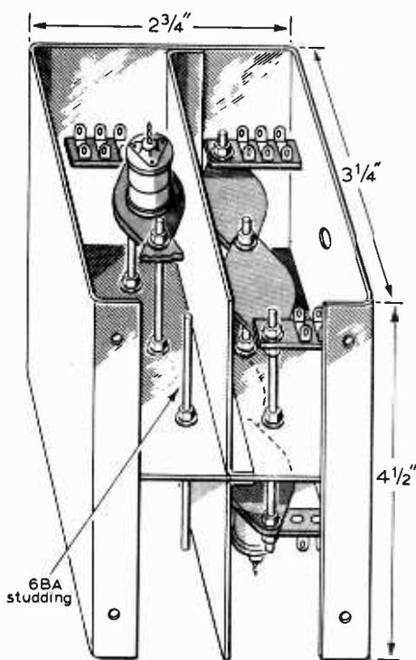
Fig. 4. Details of the attenuator sub-unit.
