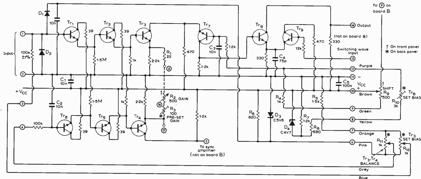
Fig. 5. Circuit of Channel A amplifier showing the external connections to the bias controls. Channel B is identical except that there is no 330Ω collector resistor for  $Tr_{8B}$  nor an output to the sync amplifier. The outputs of the two boards are joined directly together and the one resistor shown here is common to both  $Tr_{8A}$  and  $Tr_{8B}$ . All n-p-n transistors are BC107 and p-n-p are BC157.
