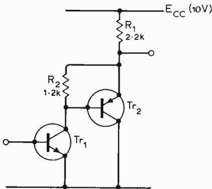
Typical voltage gains measured for the circuit were of the order of 1500, in good agreement with theoretical values. If a high-gain transistor (or Darlington pair) is used for  $Tr_2$ , the voltage gain of the circuit is limited by the parameter  $h_{oe}$  of transistor  $Tr_1$ .
