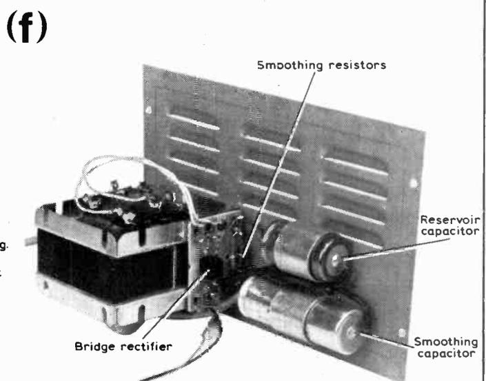
(a) End view showing how the amplifier boards are mounted. (b) General view of the top showing the channel A attenuators and amplifier board. (c) Rear view showing the sawtooth generator and bistable board, also the pre-set controls and decoupling components. (d) Underside view showing the channel B attenuators and amplifier board. (e) The complete instrument. (f) The power supply components are mounted on the back of the case. The transformer used is actually unnecessarily large.
