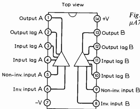
Fig. 3. Connections of the μA739 integrated circuit.
