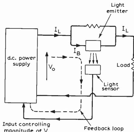
Fig. 1. Basic circuit of opto-electronic current controller.
