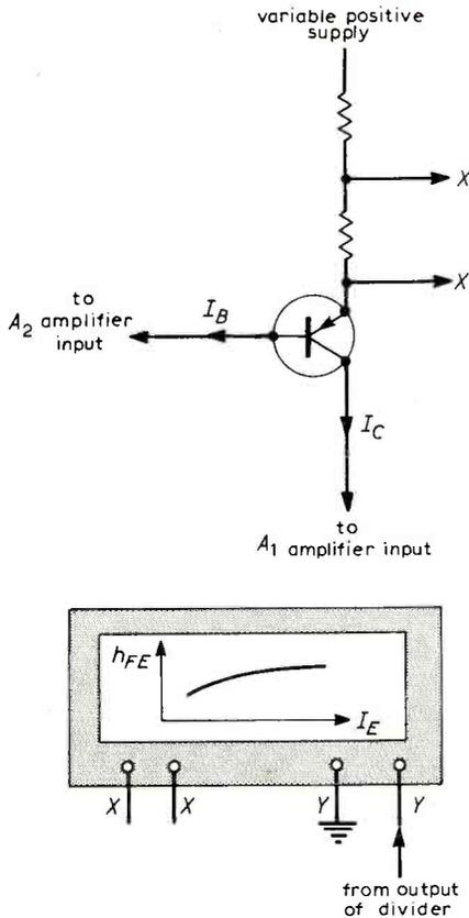
Fig. 7.11. Measurement of transistor  $h_{FE}$  variations using divider circuit.
