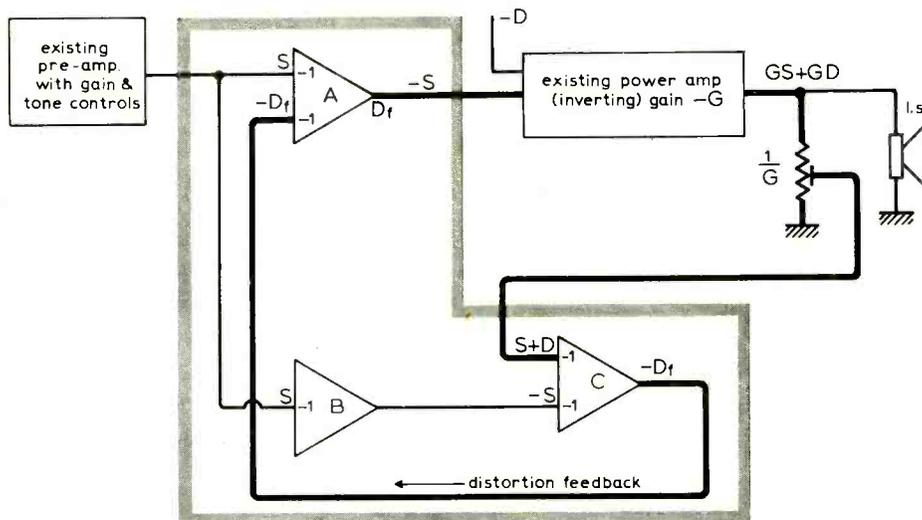
Fig. 1. Distortion reducer with inverting power amplifier. D, equivalent amplifier input distortion; GD, distortion at amplifier output; D<sub>f</sub>, distortion feedback signal.
