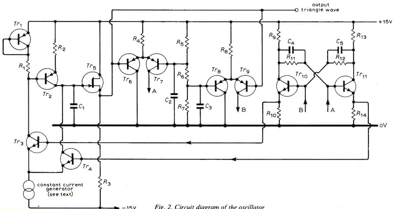
Fig. 2. Circuit diagram of the oscillator.
