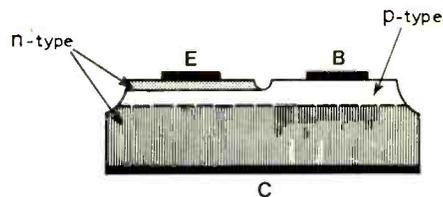
Fig. 4. Mesa transistor, produced by selective masking, diffusion and etching, carried out entirely on one side of the semiconductor slab.
