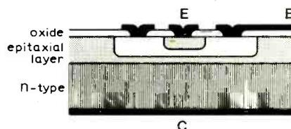
Fig. 5. Planar transistor, like the mesa, produced in one side of a slab of silicon, but with greater control of parameters. The process of epitaxy although first applied to mesa transistors was more fully developed with planar devices.
