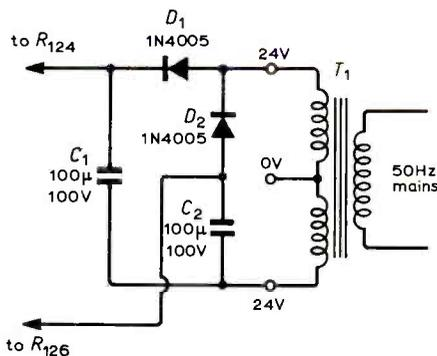
Fig. 7. Alternative high voltage supply circuit.
