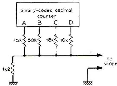
about 0.5V pk-pk. The *n*th step of the function then represents the counter output *n*. It has proved easy to read off counter outputs and as the step from 5 to 6 is set to about half the height of the other steps and easily recognized, poor sync on simple oscilloscopes can be coped with.
