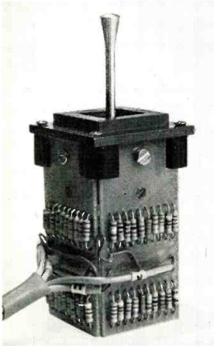
customer specification to meet a particular requirement. Specifications for standard versions are as follows:  $Z_i$  = output impedance of preceding stages is not to exceed 100 $\Omega$ .  $Z_o$  = load impedance of following stages is not to be less than 15,000 $\Omega$ . Insertion loss with joystick in centre (input to any output) =  $2 \times$  element value. Audiotek, Farringdon House, St. Albans Road East, Hatfield, Herts.
