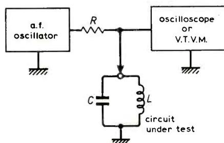
Fig. 6. Resonance testing circuit.
