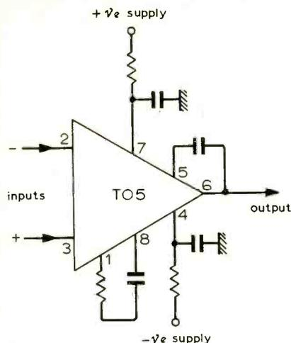
Fig. 2. Alternative circuit connections for TO5 package.
