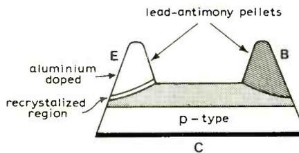
Fig. 2. Cross-section of a p-n-p alloy diffused transistor. Two 100 $\mu\text{m}$  wires are soldered to two lead-antimony pellets. The left-hand pellet also contains a small quantity of aluminium, applied as a paint after an initial alloying cycle. After subsequent heating to complete the alloy the left-hand pellet forms the emitter. The other lead is for the base. (Photo: Mullard Ltd)
