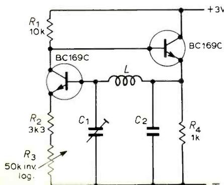
important *R*<sub>2</sub> and the regeneration control *R*<sub>3</sub> may be replaced by one 10kΩ fixed resistance.
