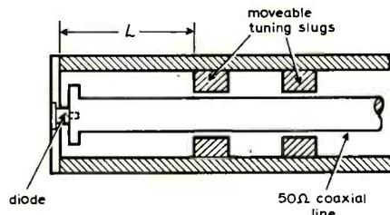
Fig. 4. Trapatt diode coaxial oscillator circuit. Tuning slugs form a variable low-pass filter which appears as a short circuit to Impatt-mode frequencies.
