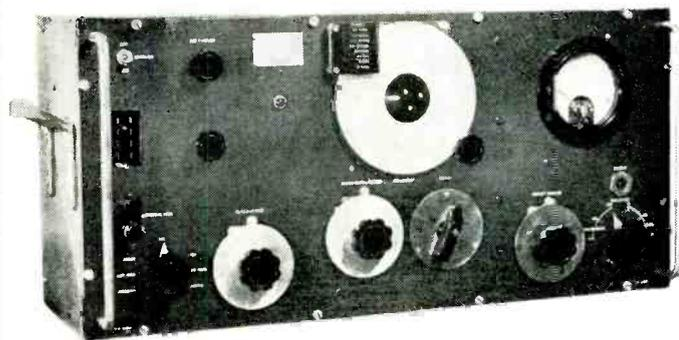
**MARCONI SIGNAL GENERATOR TYPE TF-144G:** Freq. 85 Kc/s-25 Mc/s in 8 ranges. Incremental:  $\pm 1\%$  at 1 Mc/s. Output: continuously variable 1 microvolt to 1 volt. Output Impedance: 1 microvolt to 100 millivolts, 10 ohms 100mV - 1 volt - 52.5 ohms. Internal Modulation: 400 c/s sinewave 75% depth. External Modulation: Direct or via internal amplifier. A.C. mains 200/250V, 40-100 c/s. Consumption approx. 40 watts. Measurements 29 x 12 1/2 x 10 in. Secondhand condition. £27.50 each, Carr. £1.50.
