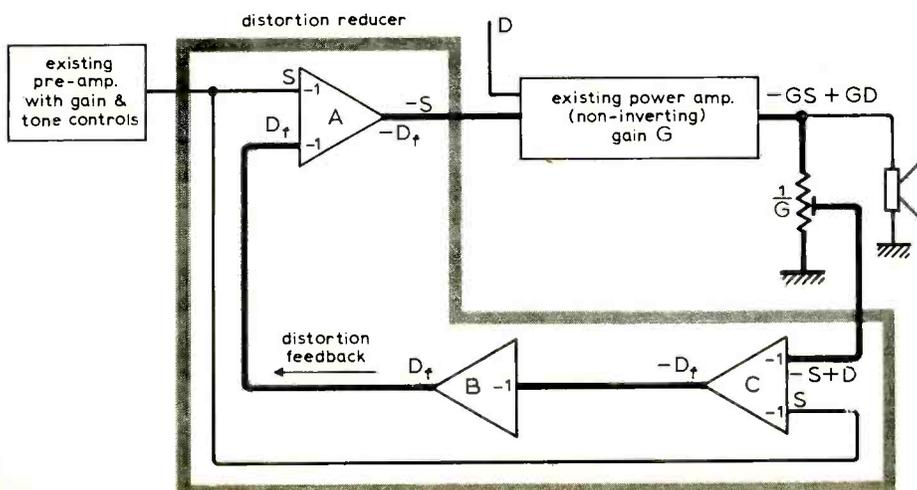
Fig. 2. Distortion reducer with non-inverting power amplifier.
