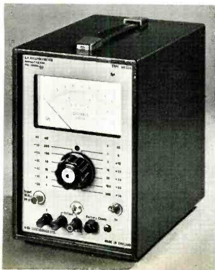
the connection of recorders and oscilloscopes or even a noise dosimeter. The meter can make measurements from 24dB to 140dB s.p.l. using the same microphone type as is fitted to most British units and thus microphone accessories are interchangeable. The CS17A is priced at £68 complete. Custom Electronic Associates Ltd, Castle Associates Division, Redbourne House, North Street, Scarborough, Yorks. YO11 1DE.
