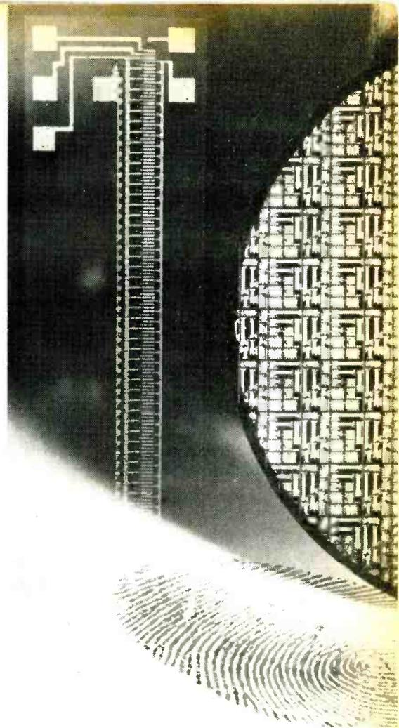
*Small linear structures (the thumbprint gives an impression of the size) are l.s.i. charge-coupled devices for which Siemens have introduced an ion implantation technique, making possible the transfer of charge from one device to the next in a shift register (right in photograph), almost without loss.*
