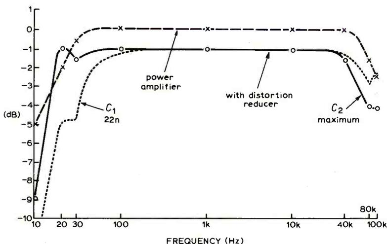
Fig. 8. Frequency response of test amplifier.
