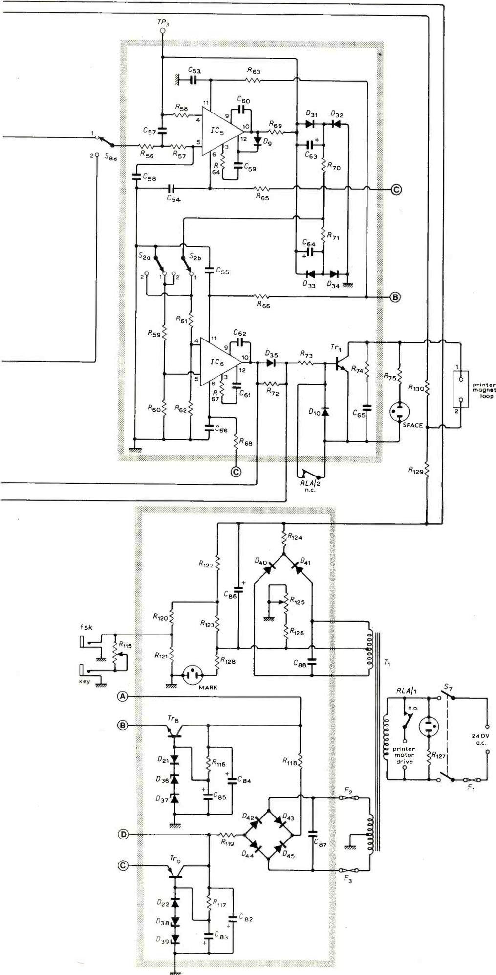
Fig. 1. Circuit diagram. (Partition lines show the limits of printed circuit boards, when used.)
