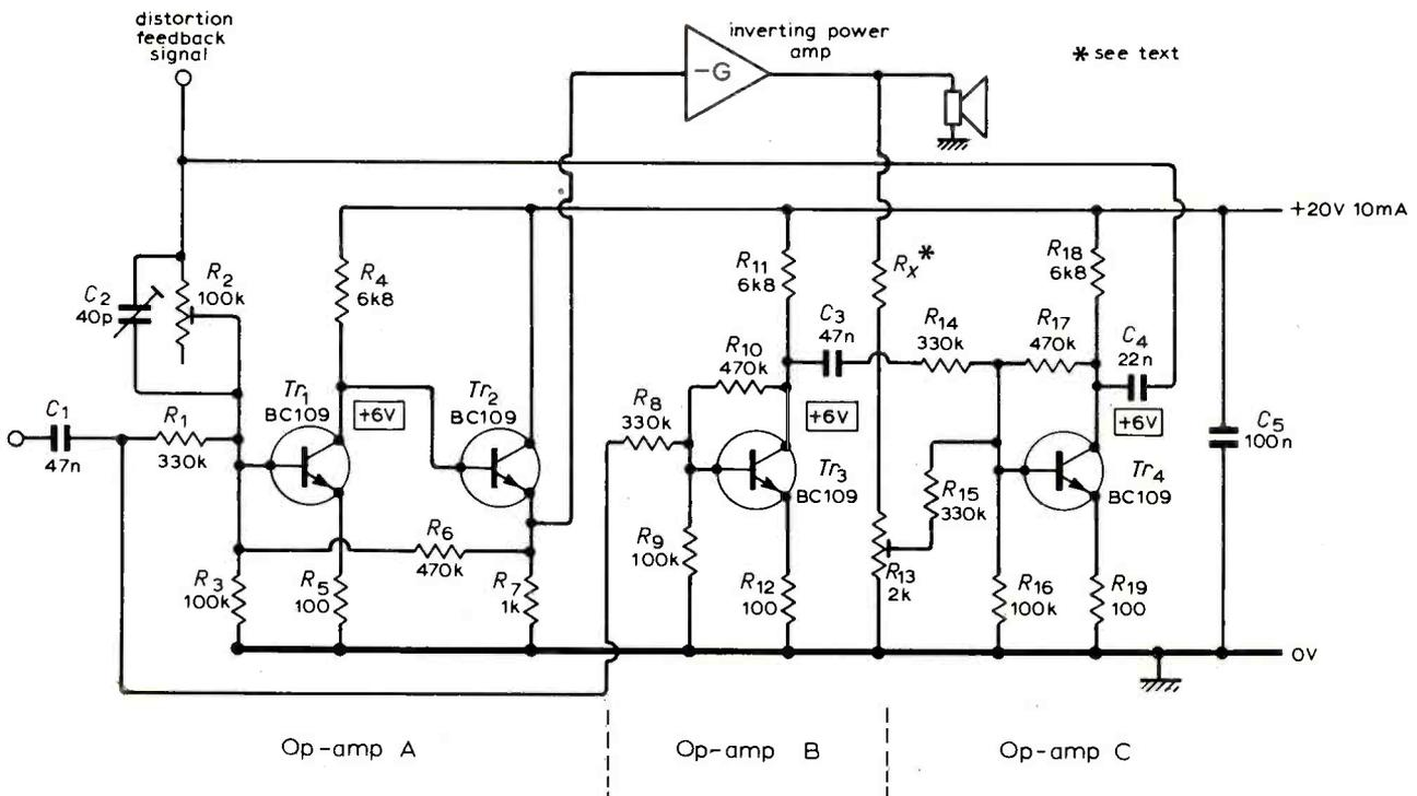
Fig. 4. Circuit of distortion reducer, for use with inverting power amplifiers.
