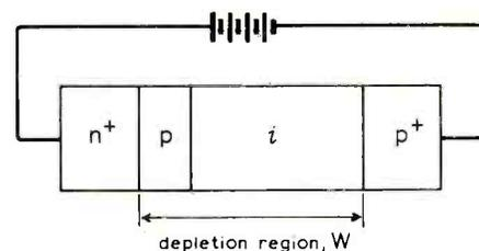
Fig. 1. Classical impatt diode Read structure. Device is reverse biased, with + indicating heavy doping.
