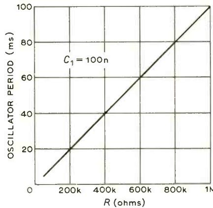
Fig. 5. Oscillator performance with current generator 4(b) demonstrating linear period calibration.
