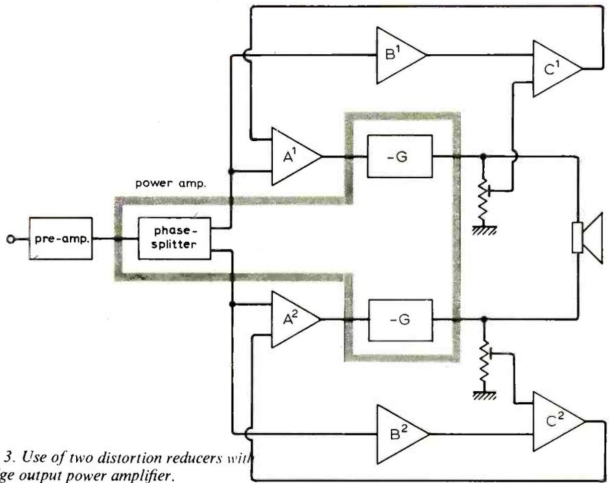
Fig. 3. Use of two distortion reducers with bridge output power amplifier.
