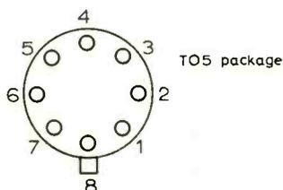
Fig. 3. Pin connections (top view).
