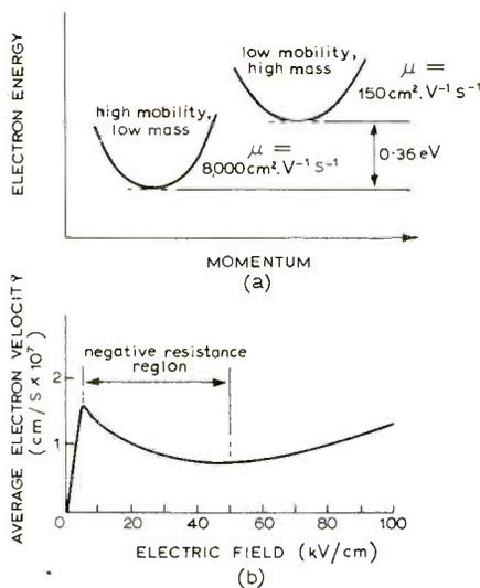
Fig. 5. (a) Energy band diagram for GaAs. The 0.36-eV level represents the quantum energy step between the two levels. (b) Velocity versus electric field for GaAs. Peak indicates the stage at which electrons jump from one level to the other and start to slow down.
