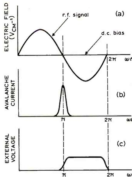
Fig. 2. Field profiles for the Read diode. Note the narrow avalanche region with peak current delayed  $90^\circ$  on peak voltage.
