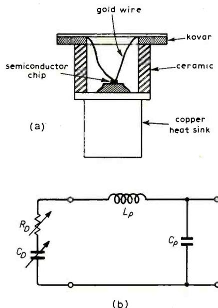
Fig. 3. (a) Typical package used up to 20GHz,  $10 \times$  full size. (b) Simplified equivalent circuit: overall effect of  $L_p$  and  $C_p$  degrades performance of the chip semiconductor
