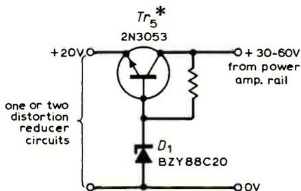
\*fitted with push fit 50°C/W heat sink
