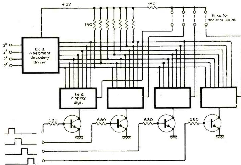
Fig. 6. Multiplexing of the displays, achieved by a switching transistor in the common cathode of an l.e.d.
