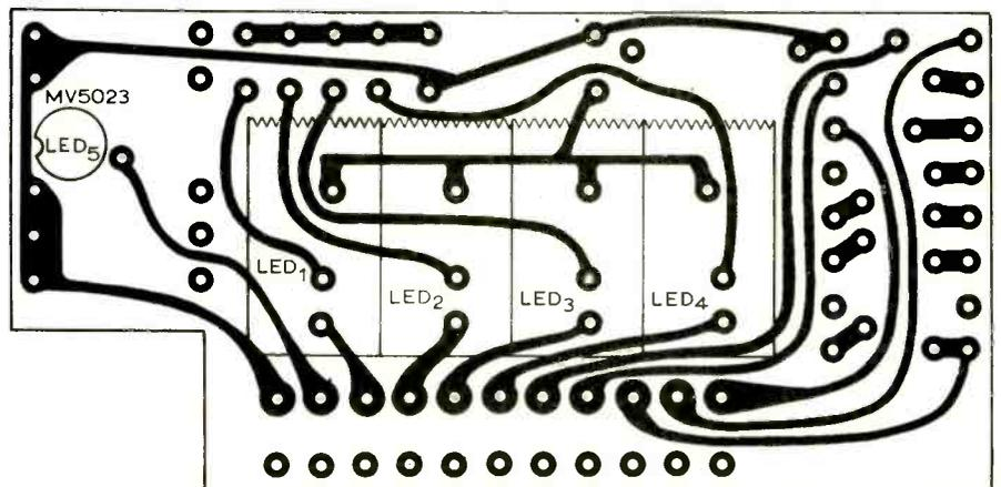
Fig. 12. Component layout and connecting tracks on the front of the display p.c. board.
