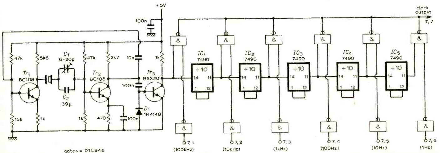
Fig. 7. Master clock and divider chain.
