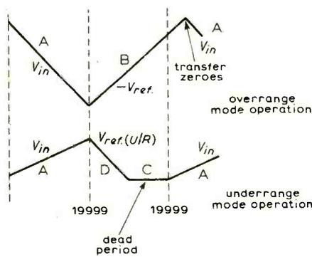
Fig. 7. Waveforms for over-range and under-range operation.
