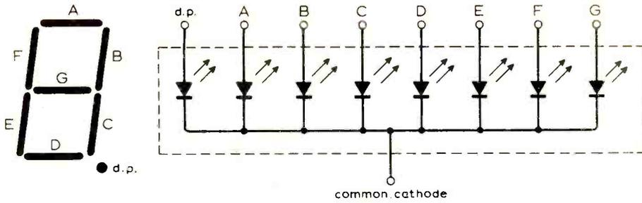
Fig. 5. Configuration and connections of the l.e.d.s in one digit.
