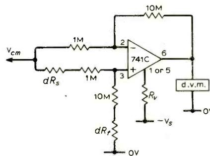
Fig. 5. Optimization of common mode rejection.
