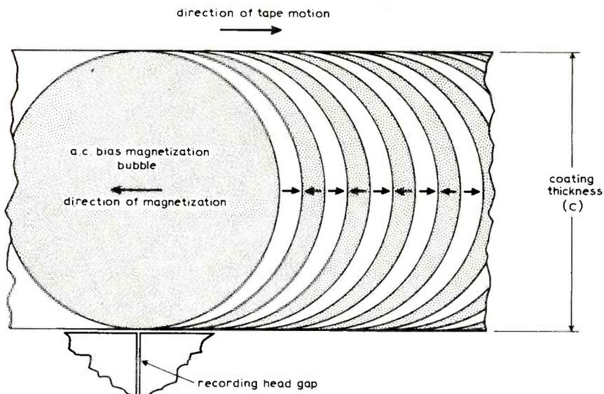
Fig. 3 (a). Recorded magnetization of bias field without signal.
