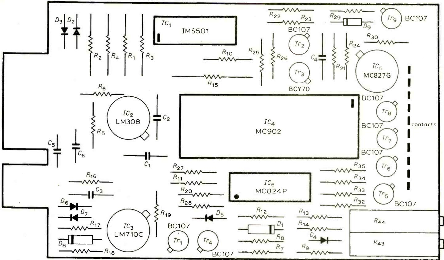
Fig. 10. Component layout on the main p.c. board.
