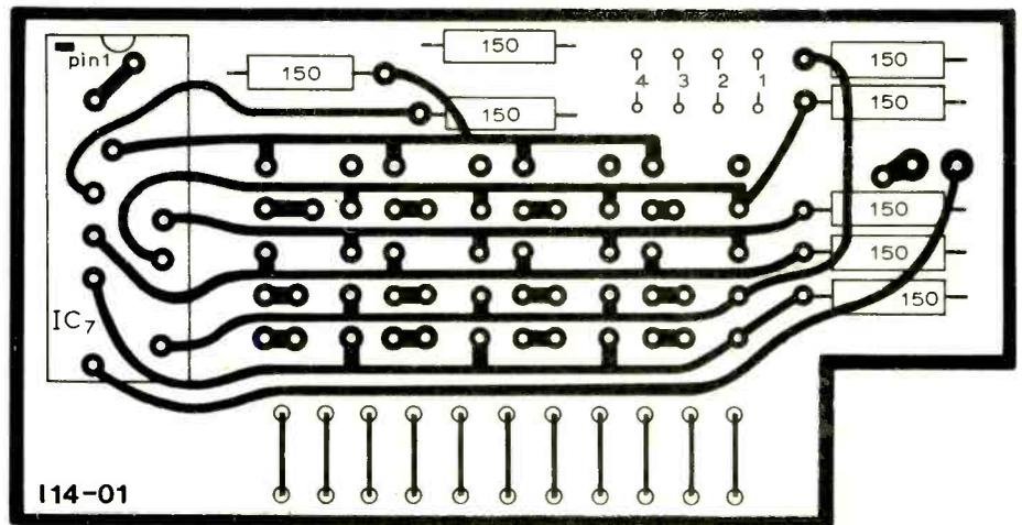
Fig. 11. Component layout and connecting tracks on the rear of the display p.c. board.
