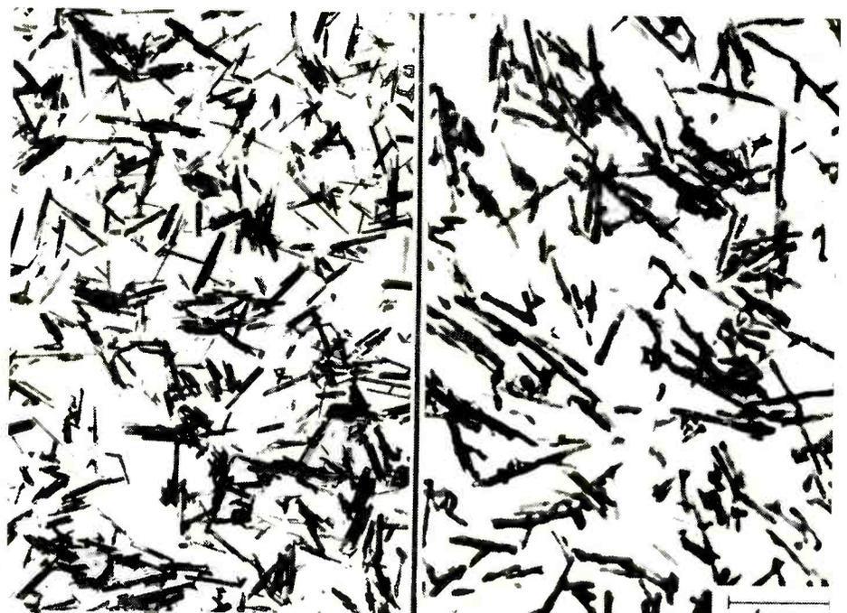
Fig. 4. As yet chromium dioxide has not been produced in a reel-to-reel form; however its magnetic characteristics are different to ferric oxide and represent a considerable step away from compatibility. Many of the changes in the properties are attributable to the differences in physical structure shown here on the left in comparison with ferric oxide (right). Note the cleaner, more needle-like appearance of CrO<sub>2</sub> and the more regular distribution of particle size.
