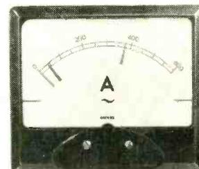
Soliconroller Moving Coil Relay. DC moving coil and AC moving coil rectified. 1 or 2 adjustable alarm controls.
