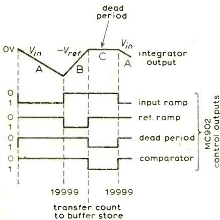
Fig. 3. Waveforms for normal mode operation, in this instance described for input voltages in the range 0 to +1.999V.
