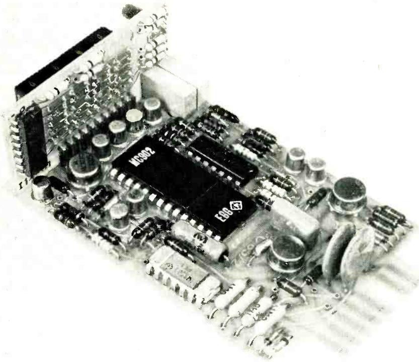
Component layout on the main printed circuit and the rear of the display panel p.c. board. The two boards are constructed separately and then slotted together by means of metal tabs.
