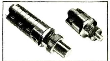
mounted from the rear directly on front panels or on rear sub-assemblies. They are claimed by the makers to be capable of 200,000 load switching operations. Up to 3-pole changeovers are available per switch, with gold-plated terminals and a maximum switching capability of 5A, 240V a.c. non-inductive loads.
