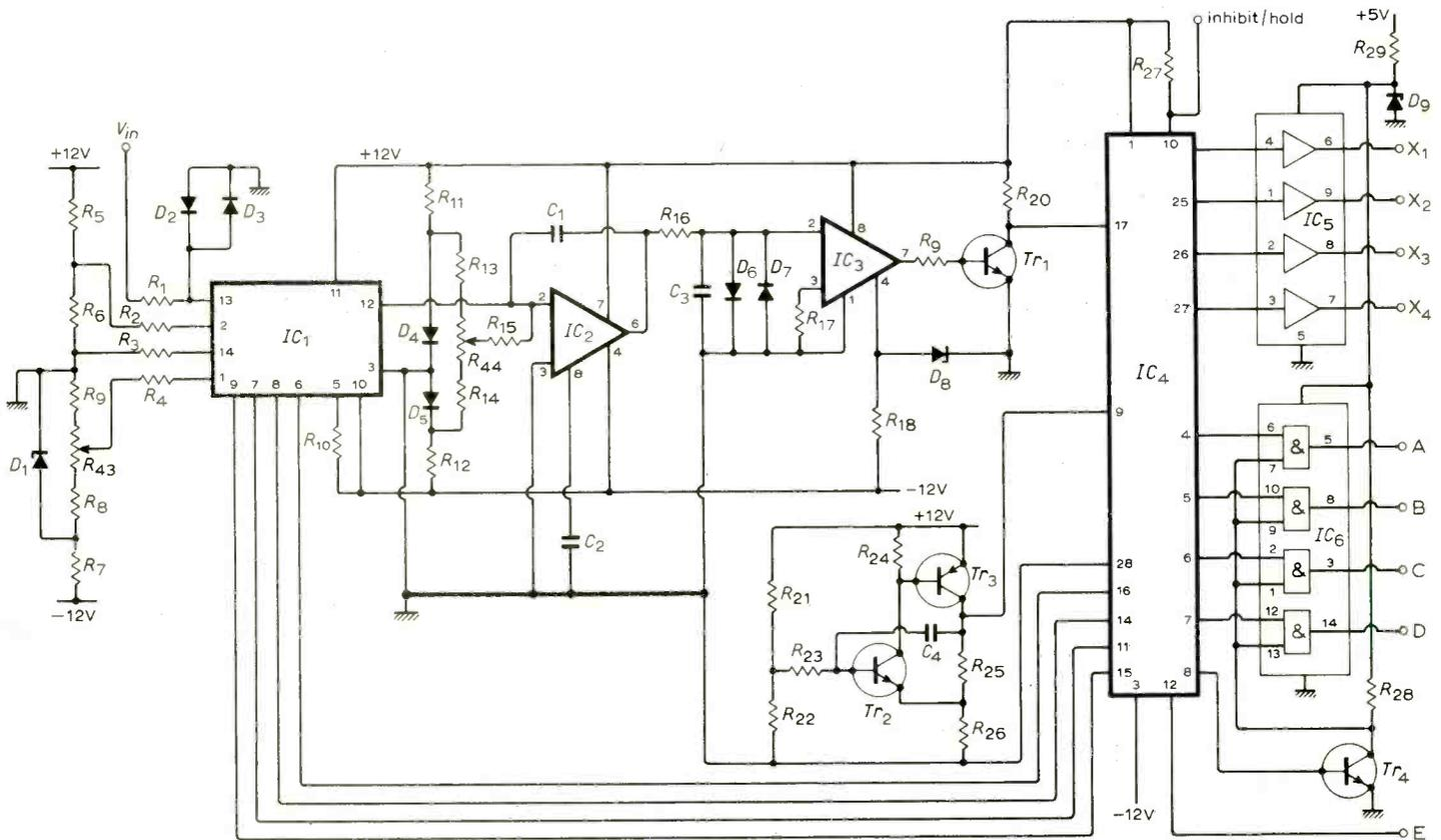
Fig. 8. Circuit diagram of the "processing" section of the d.p.m. This provides the b.c.d. and multiplexing signals for the display circuitry.
