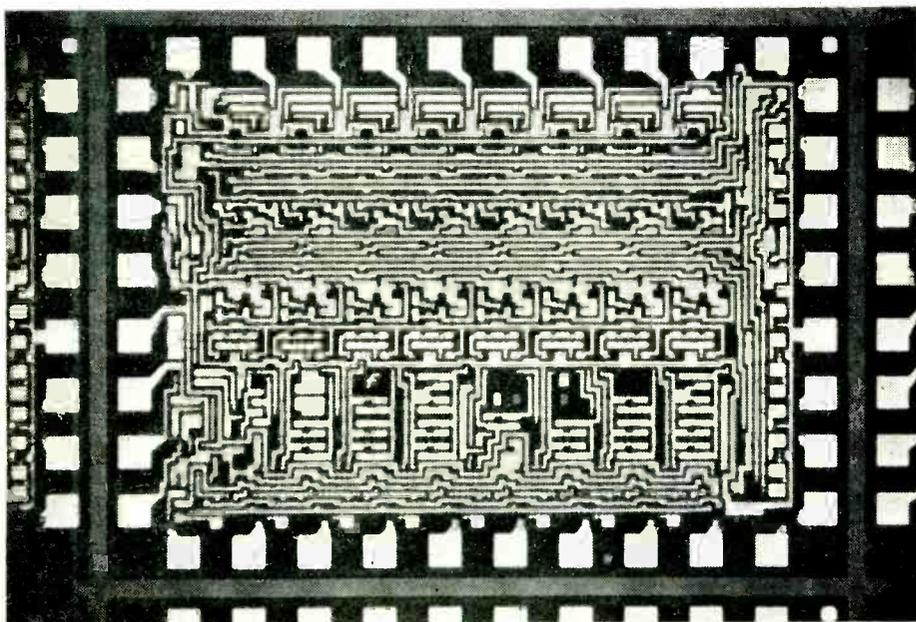
Complete serial arithmetic unit on one chip, for use with eight-bit numbers. The chip consists of 200 m.o.s. gates and was designed in the U.S.A. by Fairchild and marketed in the U.K. in 1968. (photo: S.G.S. (United Kingdom))
