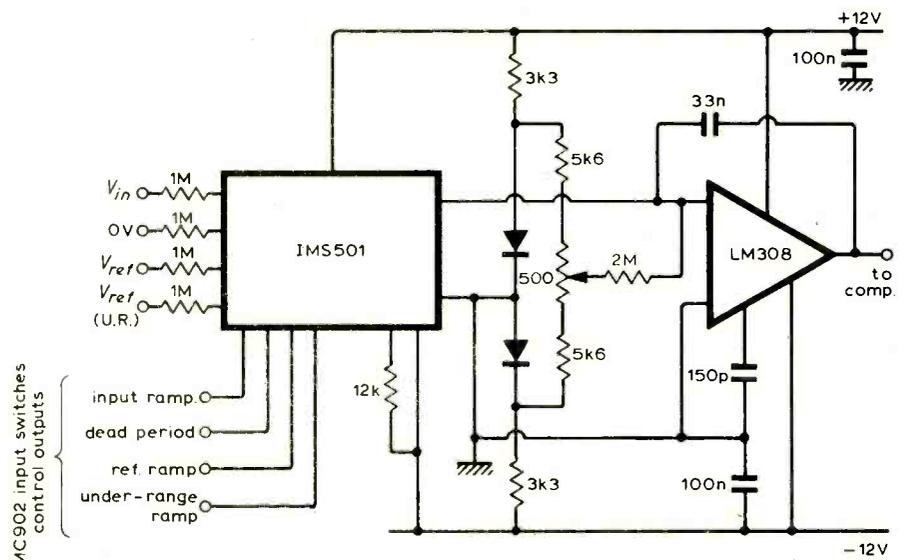
Fig. 4. Circuit of the input switches and integrator.
