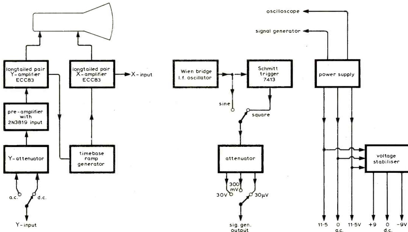
Fig.3. Block diagram of the Generatorscope, showing facilities available.
