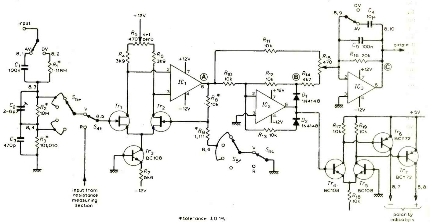
Fig. 8(b). Input amplifier, rectifier and polarity indicator circuit.
