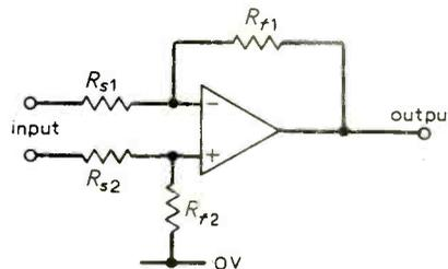
Fig. 1. Op-amp inverting configuration.
