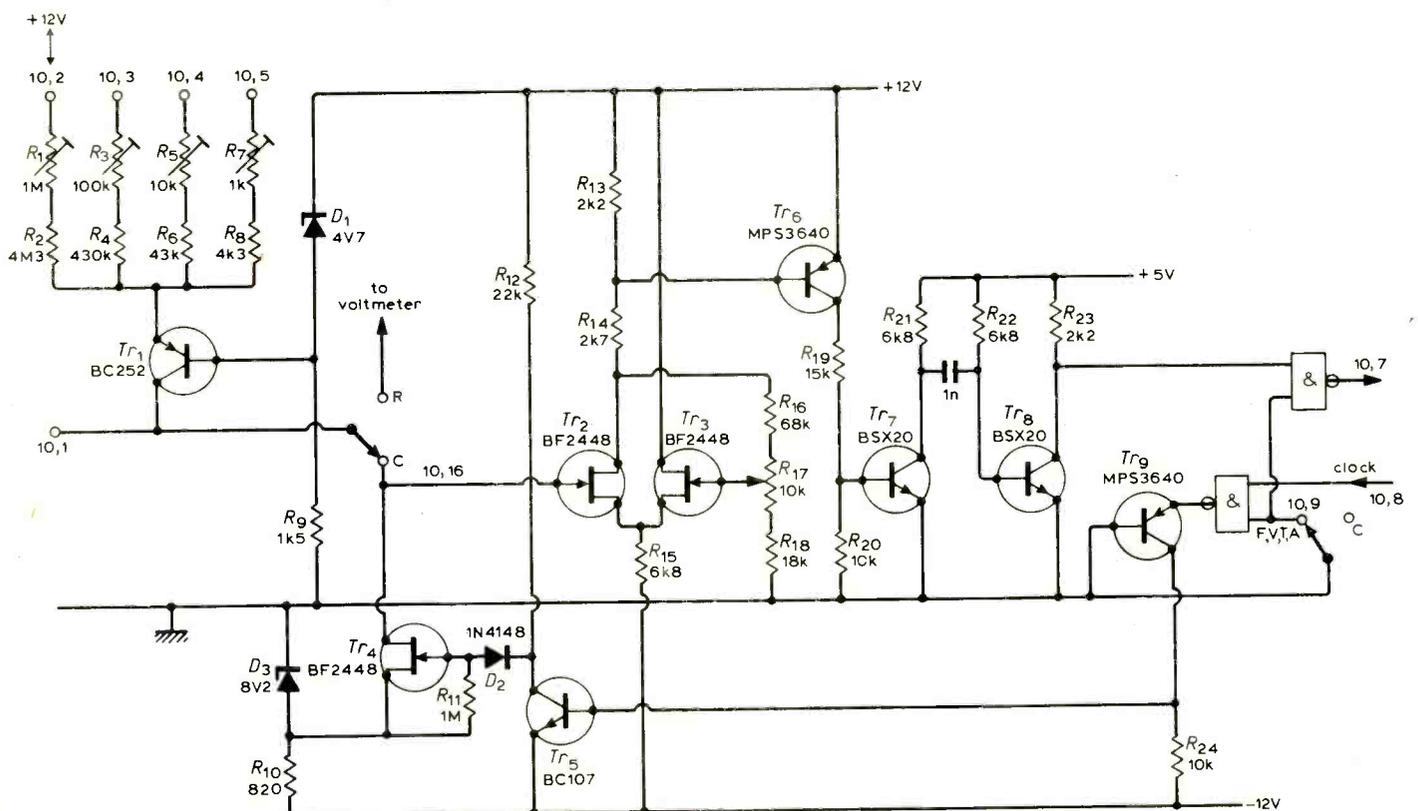
Fig. 10. Capacitance/resistance measuring circuit.
