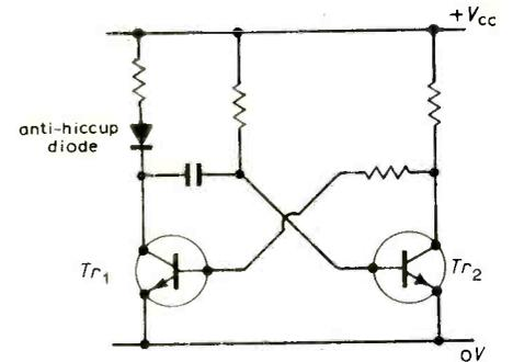
One caution; any connection directly to  $Tr_1$  collector will bypass the protection; connections should be made upstream of the diode.
