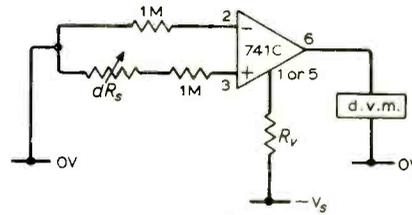
Fig. 4. Nulling additional input offset voltage due to input offset current.
