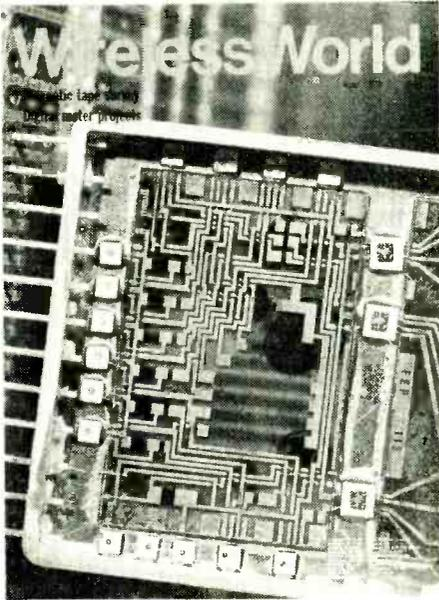
This month's cover illustration is of a Ferranti thin-film hybrid microcircuit (Type FER 118) which contains six amplifiers to interface between t.t.l. and f.e.t.s with fast switching times.
