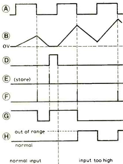
Fig. 9(b). Operation of the "out of range" indicator.
