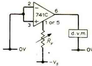
Fig. 3. Connections for nulling input offset voltage.
