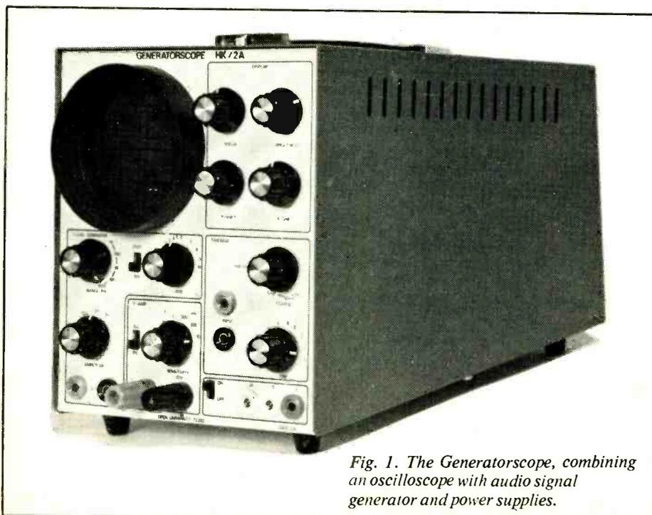
Fig. 1. The Generatorscope, combining an oscilloscope with audio signal generator and power supplies.
