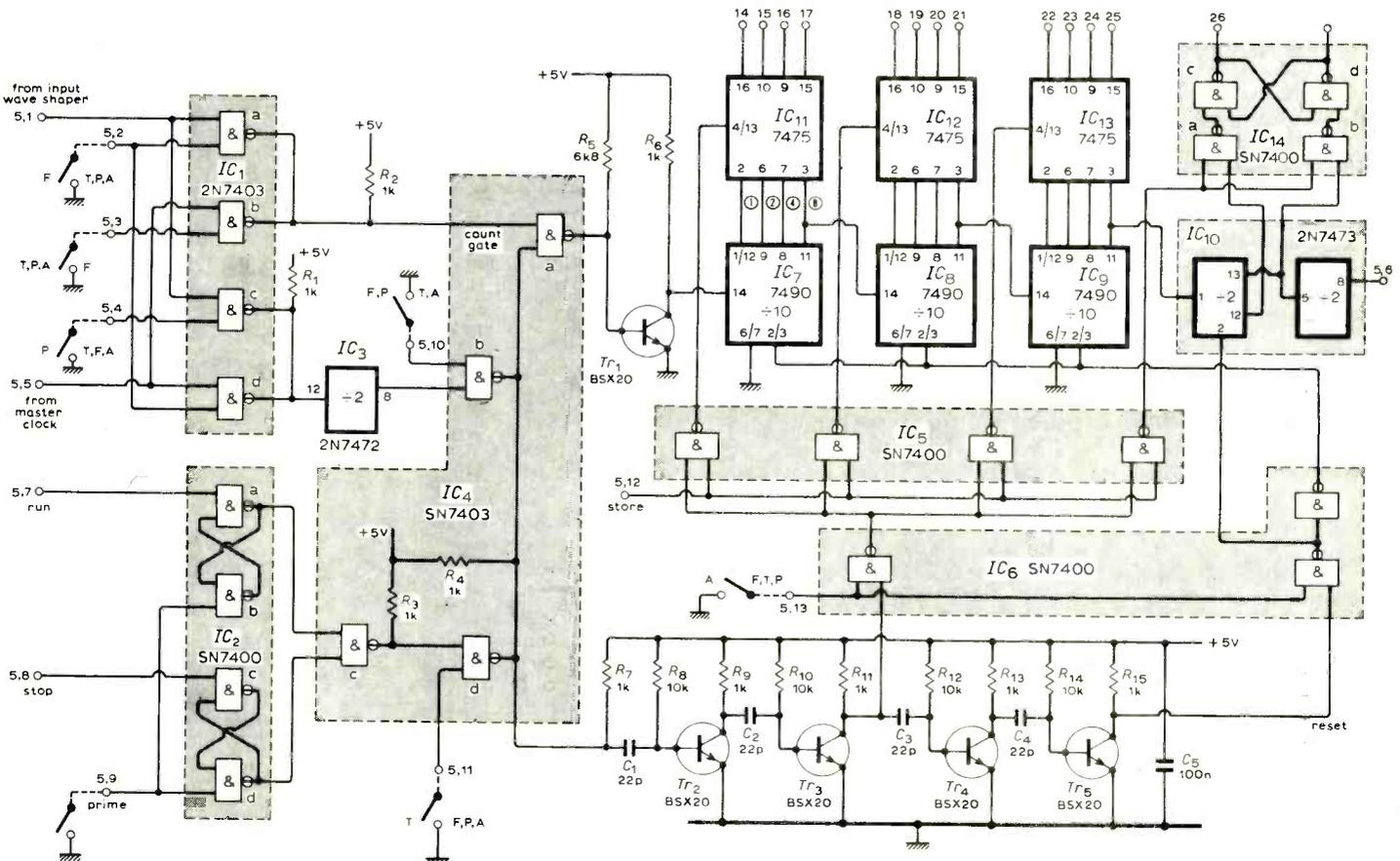
Fig. 5(b). Counter/store and control logic. This shows the general arrangement for these sections. The switch,  $S_1$ , shown dotted, indicates the switching necessary to achieve the various functions: F—Frequency counter; T—Timer; P—Period meter; A—Voltage, resistance and capacitance meter.
