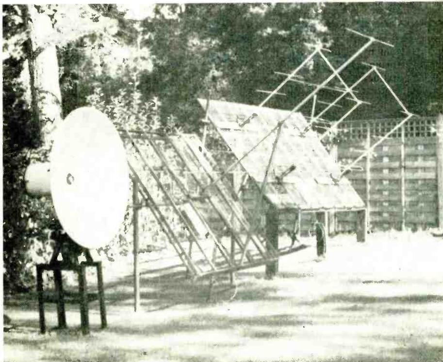
Fig. 1. The radio telescope aerials, which operate at 95 and 136MHz. The four-foot parabola is for future solar observation at microwaves.
