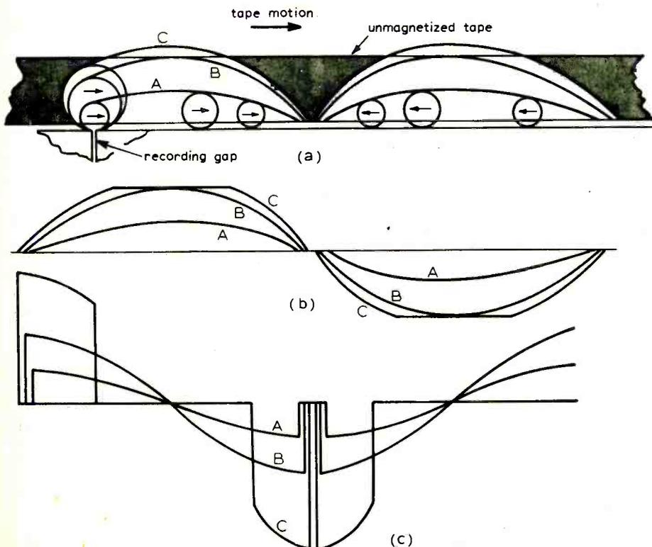
Fig. 2. Depth variable magnetization at long wavelengths and without bias.
