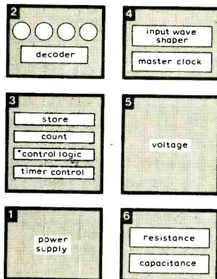
Fig. 2. Block diagram rearranged to show the parts of the circuit which are grouped together for construction.
