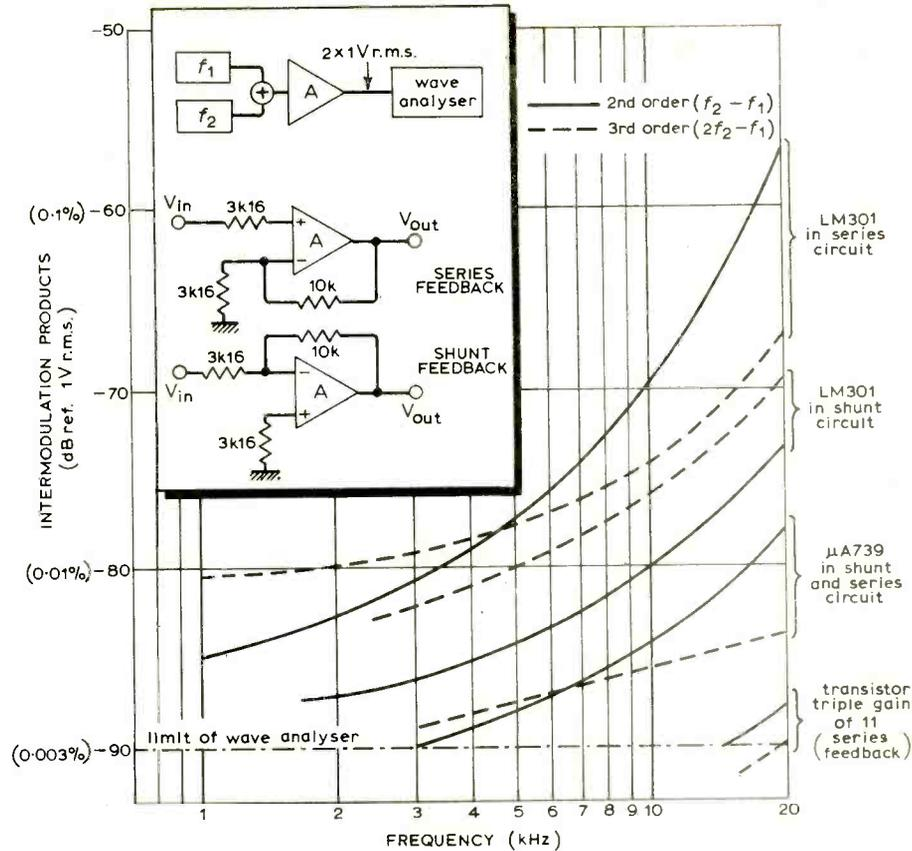
Fig.1. Intermodulation in various amplifiers.
