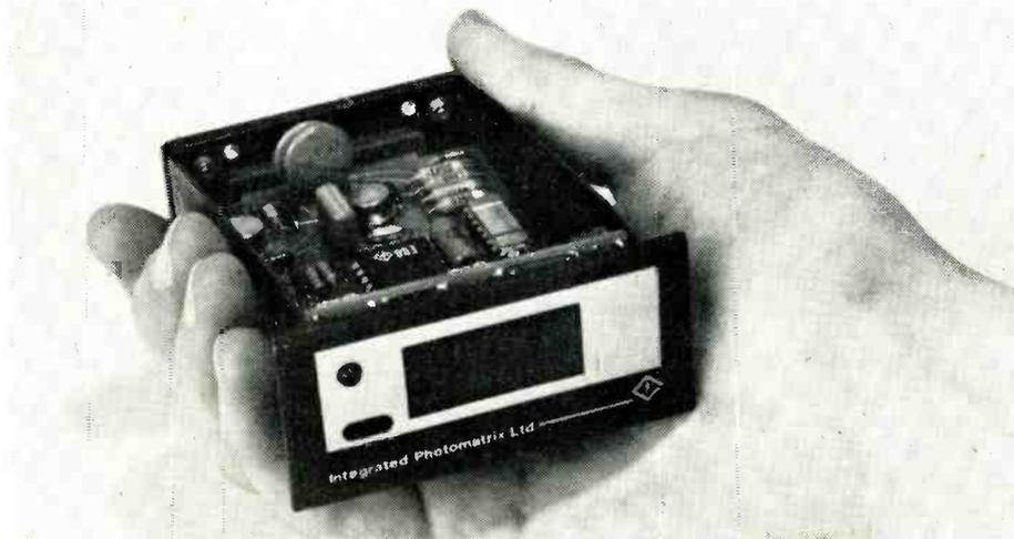
Complete instrument mounted in its chassis. Four l.e.ds provide the numerical display, with a further l.e.d. (on the left) used as an over-range indicator.
