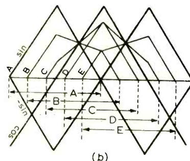
Fig. 5. (a) Resistor network to give family of phase-shifted waveforms. (b) Waveforms at tapping points of (a). Negative halves of curves are ignored. Arrows indicate zero crossings.
