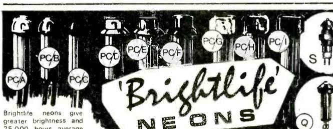
Brightlife neons give greater brightness and 25,000 hours average life. The 0.50 inch diameter dome type neons come in red or white and the 0.375 inch diameter types in red, amber or white. The latter are available in three cap shapes and all may be supplied for 115 V., 240 V. and 440 V. operation with 6" or 30" leads. The miniature Q type neon has Nato numbers and is available for 230 V. as standard as is the sub-miniature S type which we believe to be the smallest available.
