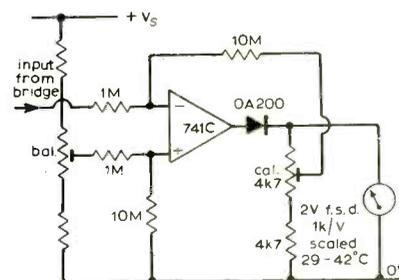
Fig. 2. Temperature scaling circuit using an op-amp.
