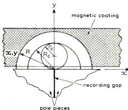
Fig. 1. Radial magnetizing field produced from the pole pieces of a record head.
