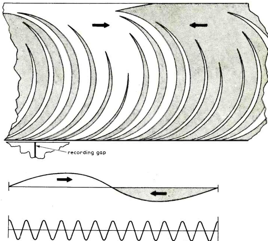
Fig. 3 (b). Magnetization of tape with bias and long wavelength signal combined.
