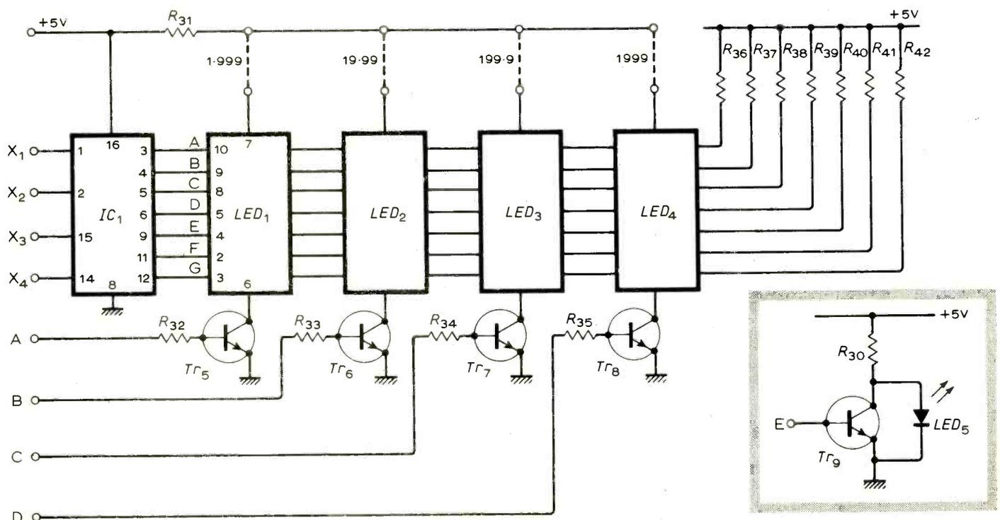
Fig. 9. Circuit of the display l.e.ds and their drivers. Also shown is the circuit for the over-range indicator (inset).
