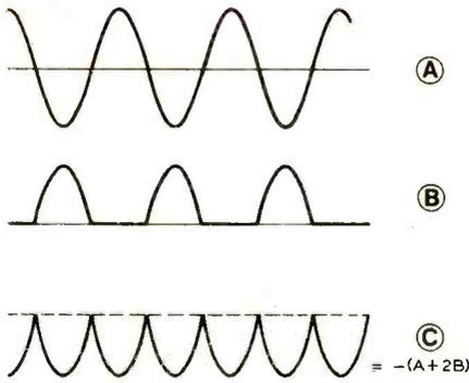
Fig. 8(a). Rectifier waveforms.
