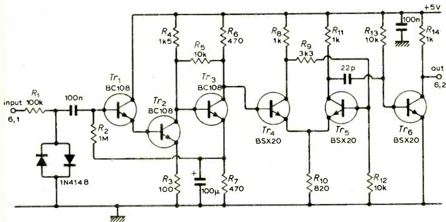
Fig. 6. Input wave shaper.
