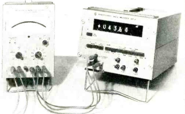
In presenting an input resistance of 50 M $\Omega$  in the range of 1 mV to 320V, the UIG is particularly suitable for measuring DC voltage in electronic circuits. Its high sensitivity, off-earth operation and current ranges are also of advantage in special measurements such as:—
