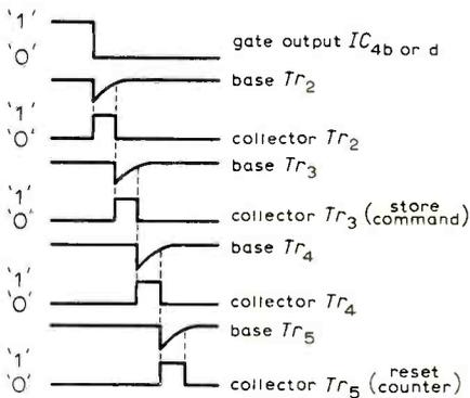
Fig. 5(a). Timing waveforms generated by the control circuit.
