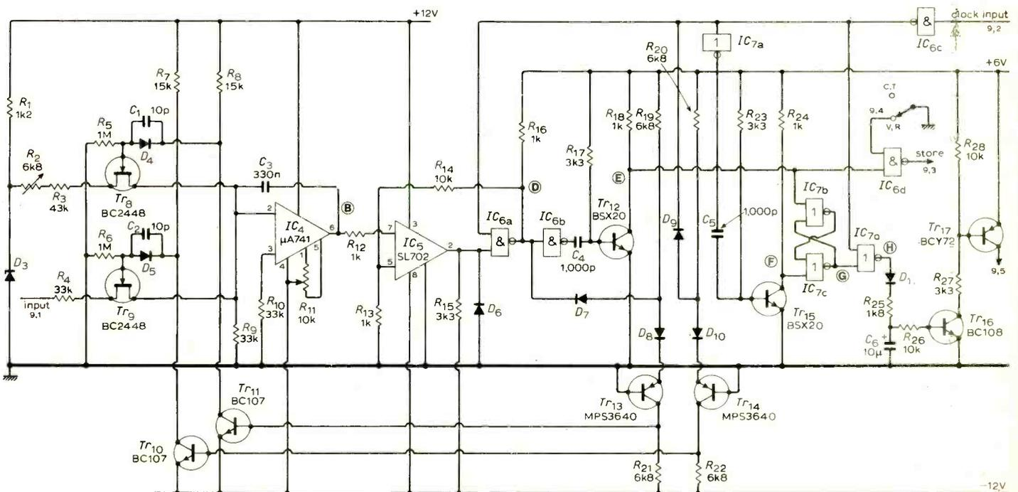
Fig. 9(a). Analogue-to-digital converter.
