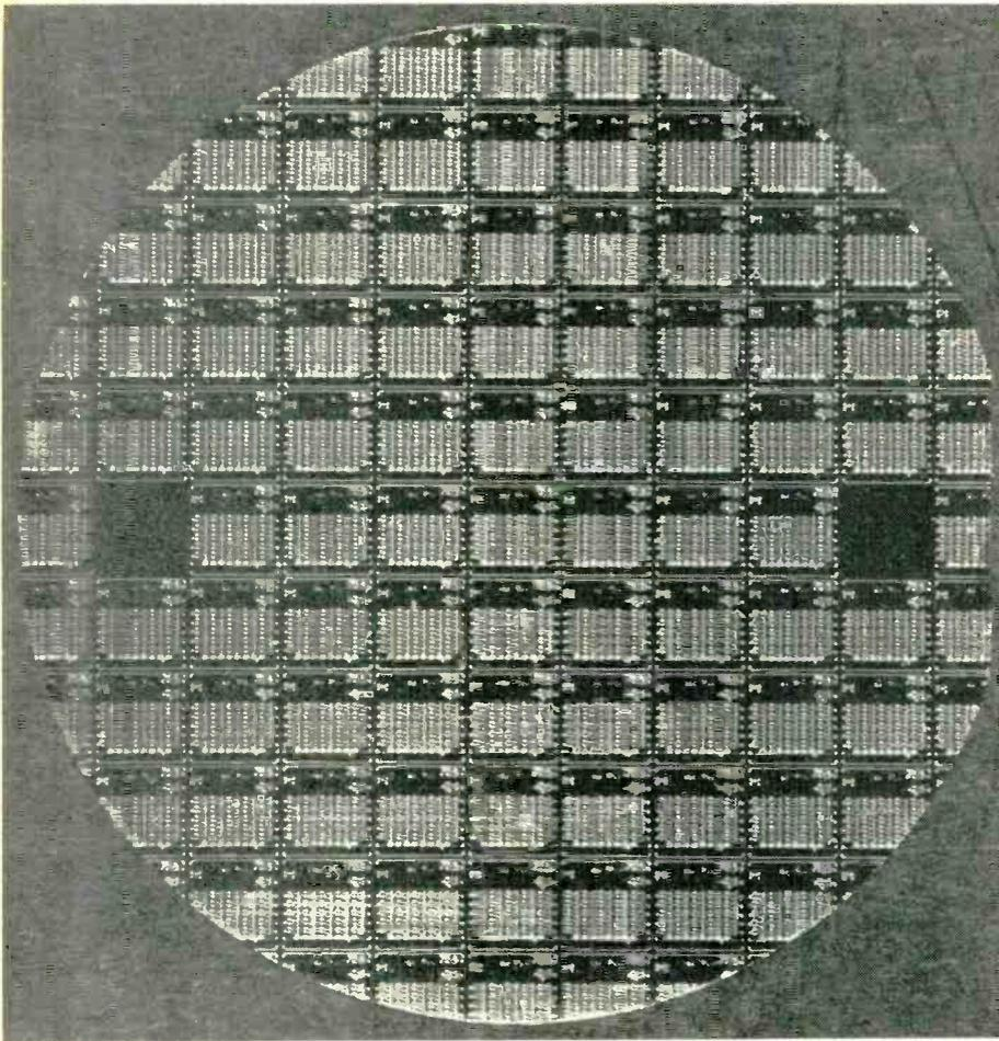
*Silicon slice with over 60 chips each about 5mm square. The circuit was commercially available from Ferranti in late 1972 and contains the components of a 200-gate uncommitted logic array and is an example of the use of c.d.i.*
