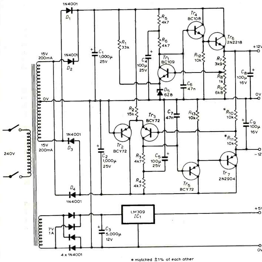
Fig. 3. Power supply and stabilizer circuit.
