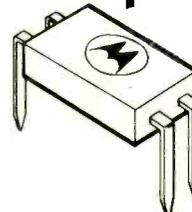
The Motorola 1/4-Watt Audio Amplifier is designed for the output stage of battery powered portable radios.
