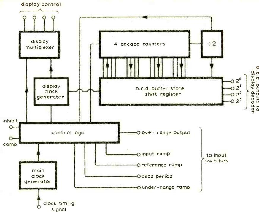
Fig. 1. Basic logic diagram of the MC902 m.o.s. l.s.i. integrated circuit which forms the heart of the design.
