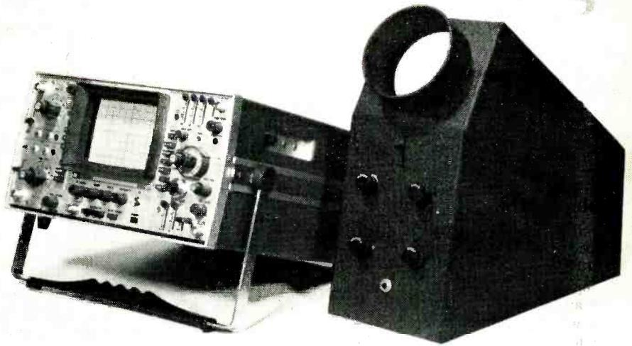
*Pictured on the right is an early Cossor oscilloscope, believed to be only the second portable model made, which has been donated to the Science Museum by O. S. Puckle. Designated the Cossor Portable Mains Oscillograph Type No. 3247, it was manufactured in 1933, selling price was £20. Alongside is one of the latest Cossor 'scopes.*
