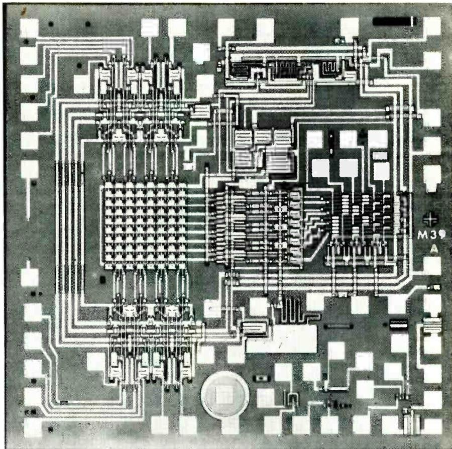
*This chip carries a non-volatile m.n.o.s. 64-bit memory (left-centre) with p-channel m.o.s. decoding circuits which require a 40V signal to drive the memory cells. The storage time for which the memory can be retained in the event of power supply failure and which can be measured in days, months or even years, is a function of the thickness of the oxide and nitride layers. (photo: The Plessey Company)*
