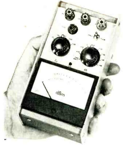
1200 $\Omega$  bridging and terminated, balanced and unbalanced) over a frequency range of 20Hz to 150kHz. Power comes from two internal layer type batteries providing a life in excess of 50 hours if used intermittently. Hatfield Instruments Ltd, Burrington Way, Plymouth PL5 3LZ.
