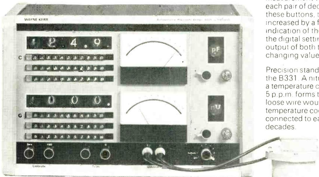
This bridge was designed for use in Standards Laboratories, but ease of operation combined with an in-line readout giving up to 6 figure discrimination has enabled many other applications to be covered.
