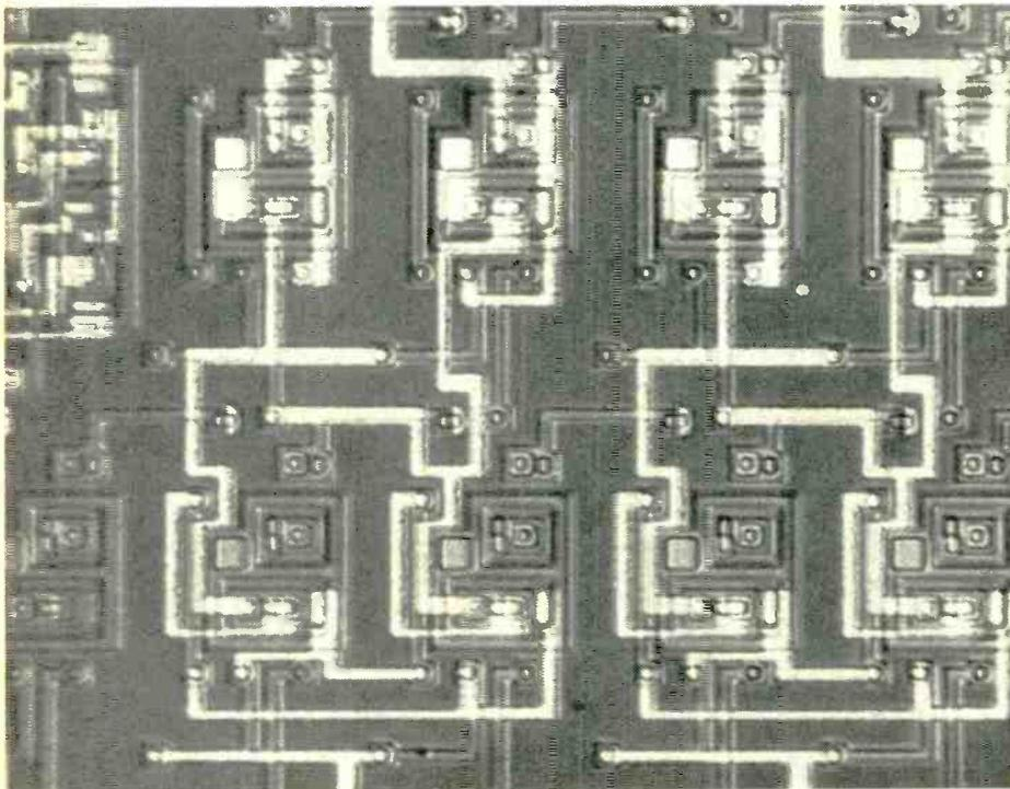
*Left shows one chip of the 60-chip 200-gate uncommitted logic array produced by the c.d.i. process. Right shows a detail of this chip. The function which the chip performs, analogue or digital or both, is selected by the metalization pattern employed, so that only one mask is involved in changes of function. Supply-line connections within the chip are made, not by the aluminium pattern, but through the silicon.*
