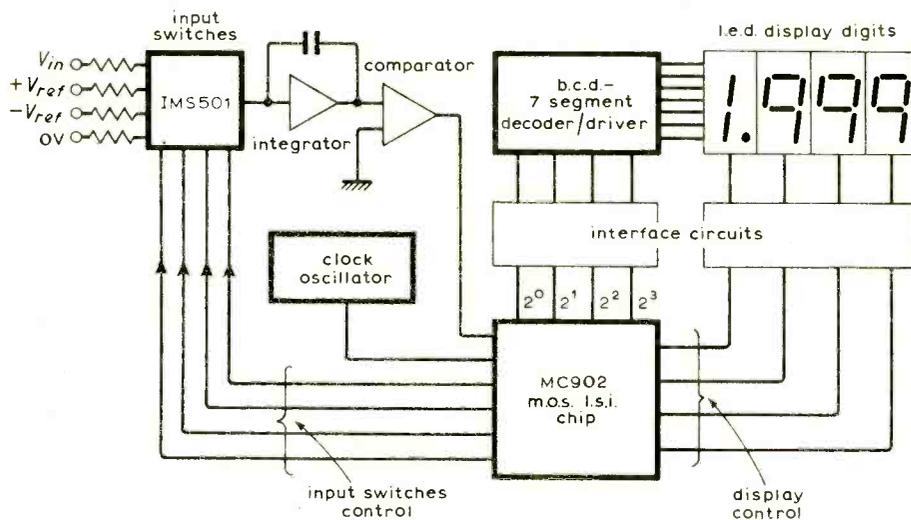
Fig. 2. Block diagram of the digital panel meter.
