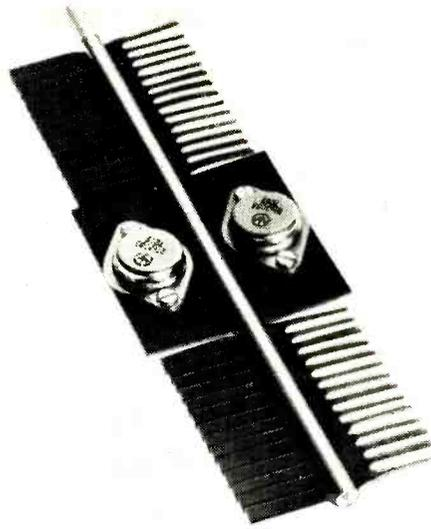
are available for a range of devices including d.i.l. i.c.s. The example shown in the photograph designated the L2220 is  $200 \times 60\text{mm}$ , weighs 60g., accepts two TO-3 devices and has a thermal performance equal to that of a conventional heatsink three times its weight (e.g. the Redpoint 4M). Forced convection performance is  $0.3^\circ\text{C}/\text{W}$ . Price £12.00. Redpoint Associates Ltd, Cheney Manor, Swindon, Wilts.
