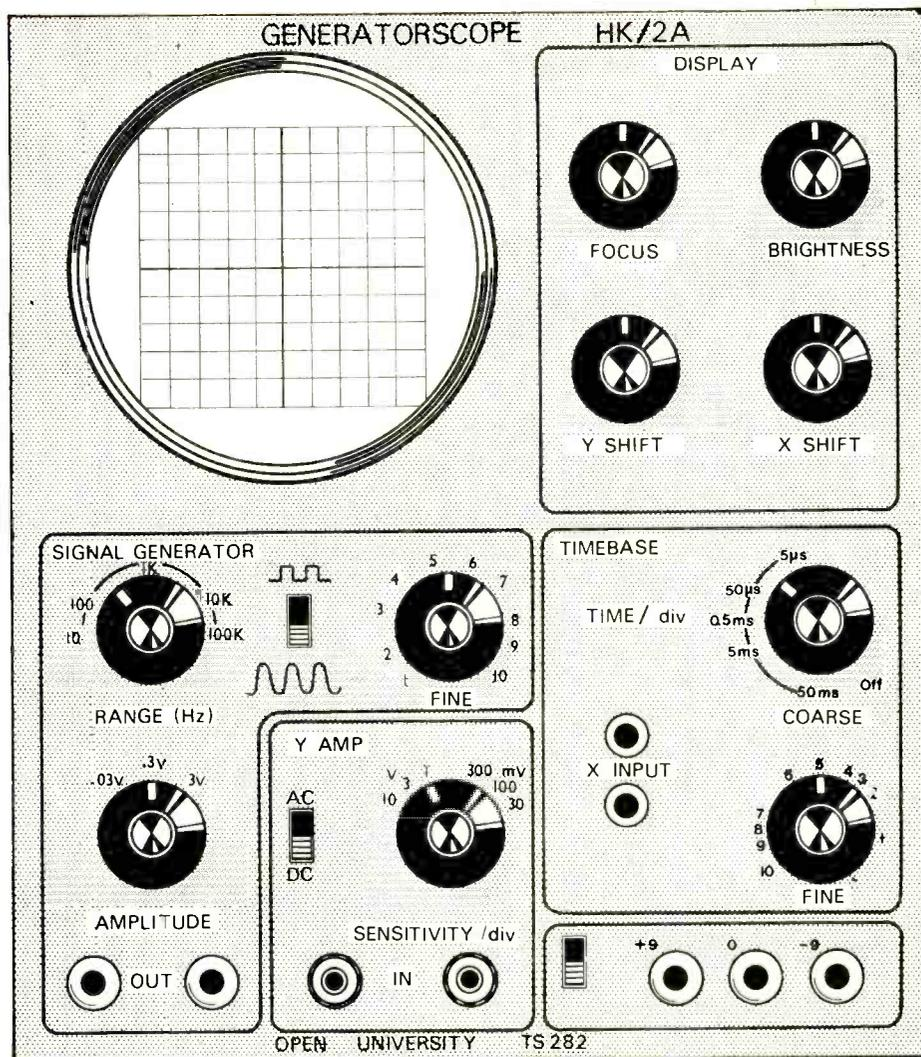
Fig. 2. Layout of the front panel of the Generatorscope.
