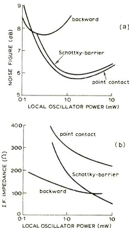
Fig. 3. Increasing oscillator power increases conversion efficiency but also the noise temperature ratio. There is an optimum power level for minimum noise figure.
