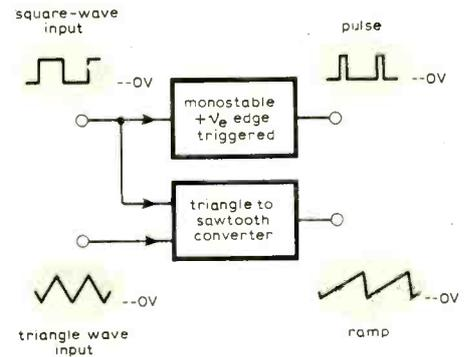
Fig. 11. Function generators of  $VCO_2$  providing a pulse or ramp output.
