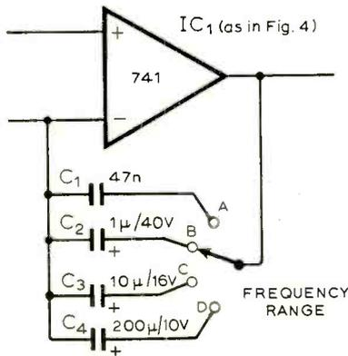
Fig. 10. Different frequency ranges of  $VCO_2$ . The rest of the circuit is the same as in Fig. 4.
