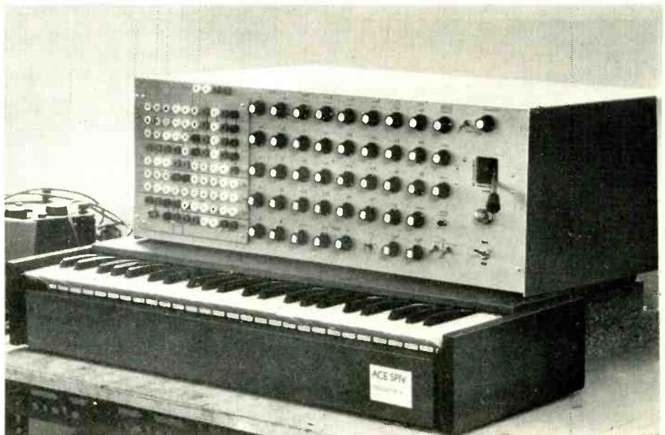
*Manual control of the synthesizer's functions is provided by a control panel, joy-stick and keyboards. The patch panel provides a means, together with voltage summing networks, of linking the internal functions.*
