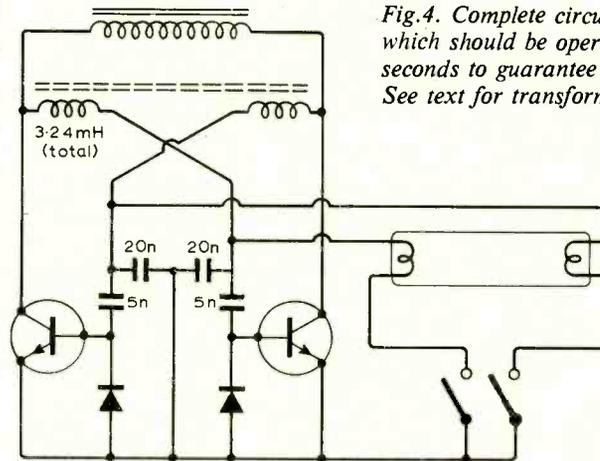
Fig.4. Complete circuit includes starting switch which should be operated for at least ten seconds to guarantee that both filaments heat. See text for transformer winding details.
