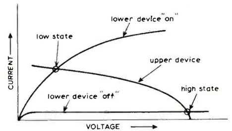
Fig. 1. Load lines of a p-m.o.s. inverter (Fig. C) intersect at a high-current point leading to significant power dissipation, around  $10\text{mW}$ , with the lower device on. Complementary m.o.s. devices avoid this.
