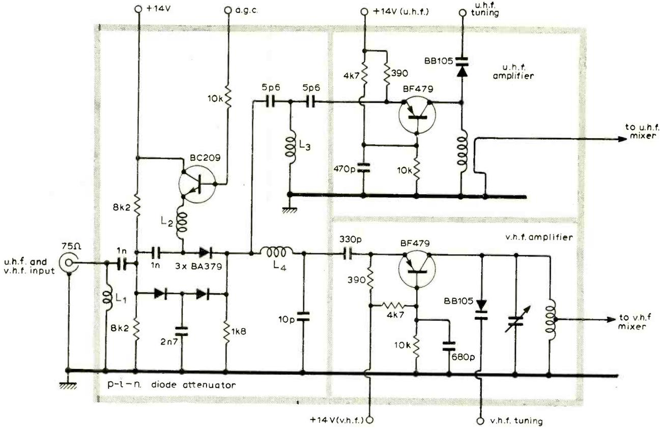
Fig. 5. Combined u.h.f. and v.h.f. television tuner using BF479 for improved cross-modulation and p-i-n diodes for a.g.c.
