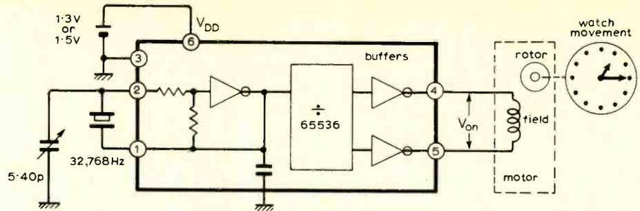
Fig. 9. Electronic watch system features both linear and switching operation of c.m.o.s. This circuit will operate from a 1.3V cell at 6μW.
