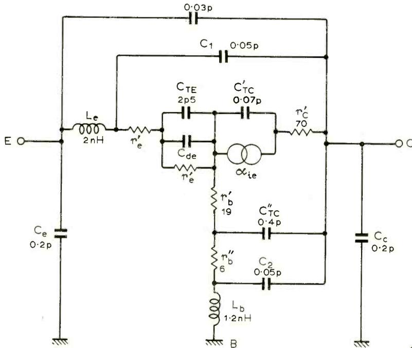
Fig. 4. New base-grid geometry and emitter metallization of BF479, which helps to reduce aluminium migration, and its equivalent circuit.
