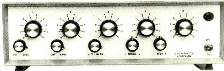
This is a high fidelity amplifier with bass cut controls on each of the three low impedance balanced line microphone stages and a high impedance (1.5 meg.) gram stage with bass and treble controls, plus the usual line or tape input. All the input stages are protected against overload by back to back low self capacity diodes and all use F.E.T.s for low noise, low intermodulation distortion and freedom from radio breakthrough.
