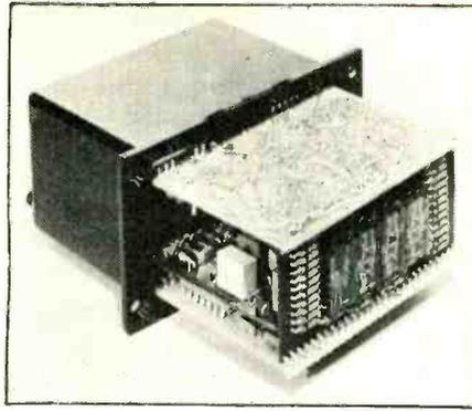
i.e.d.  $3\frac{1}{2}$  digit solid state display is provided, together with additional 100% overrange, overflow, decimal point and polarity displays. The DM-2000 is housed in a case measuring  $3 \times 1.75 \times 2.25$ in and weighs less than 6 oz. All control inputs and digital outputs are t.t.l./d.t.l. compatible. Tranchant Electronics (U.K.) Ltd, Tranchant House, 100a High Street, Hampton, Middlesex.
