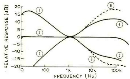
Fig.2. Amplitude/frequency response curves of tone control circuit. 1. Bass boost max. 2. Flat response 3. Bass cut max. 4. Treble boost max. 5. Treble cut max. 6, 7. Treble boost and cut with  $R_7, R_8 = 1$ k $\Omega$ .
