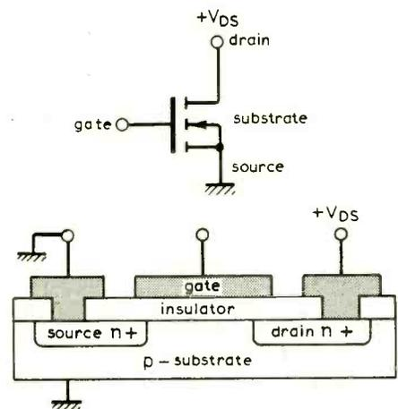
Fig. A. Insulated-gate (m.o.s.) f.e.t.s that work by modulation of a conducting channel can be either a depletion type—conducting with zero bias—or an enhancement type—cut off with zero bias. Illustration shows an n-channel enhancement device.
