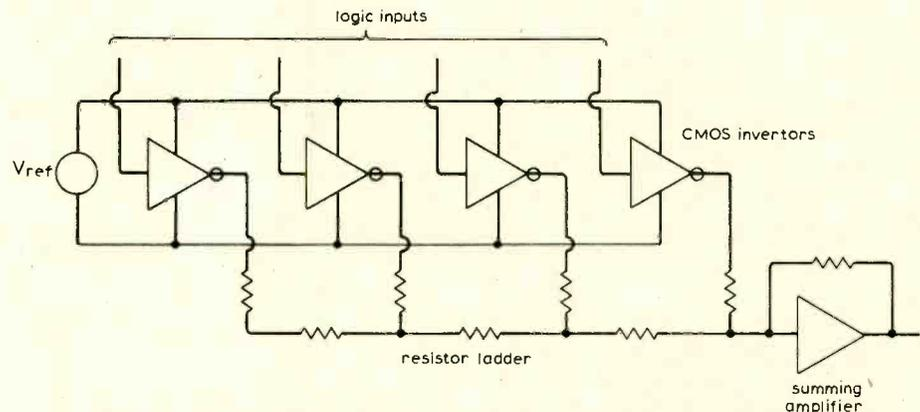
Fig. 10. Technique of digital-to-analogue conversion in which a resistive ladder is switched to generate a linear signal from a digital code.
