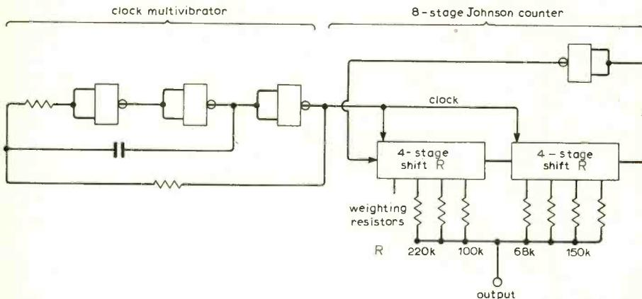
Fig. 14. Function generator using switching approach can provide harmonic content of sine wave of <0.01%.
