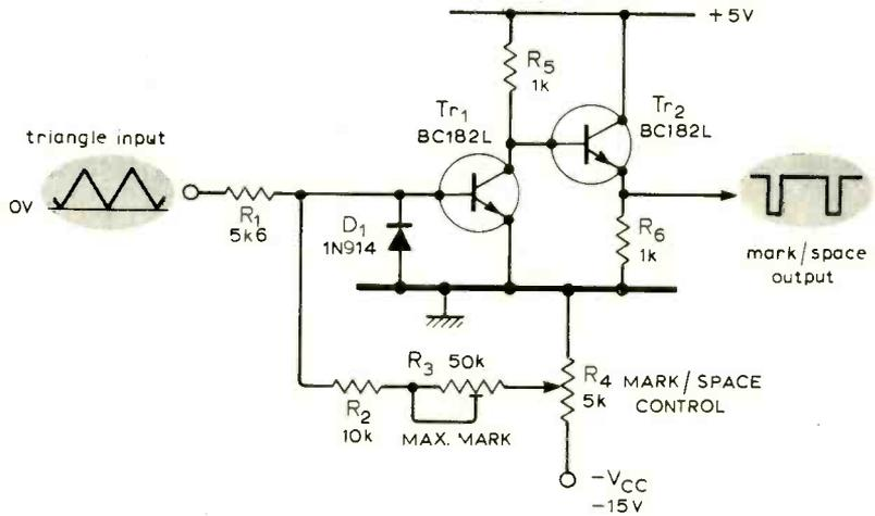
Fig. 6. Mark/space generator whose output mark/space ratio is variable from 15-85%.
