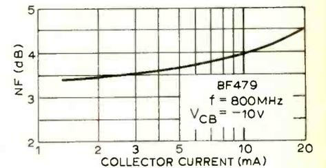
Fig. 3. Lower and more constant noise figure versus temperature and current are features of the BF479 transistor.
