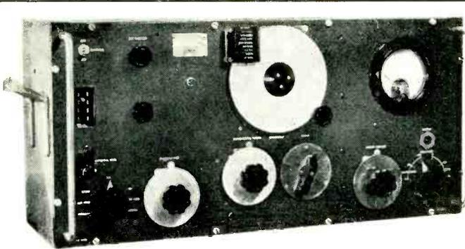
**MARCONI SIGNAL GENERATOR TYPE TF-144G:** Freq. 85 Kc/s-25 Mc/s in 8 ranges. Incremental:  $\pm 1\%$  at 1 Mc/s. Output: continuously variable 1 microvolt to 1 volt. Output Impedance: 1 microvolt to 100 millivolts, 10 ohms 100mV - 1 volt - 52.5 ohms. Internal Modulation: 400 c/s sinewave 75% depth. External Modulation: Direct or via internal amplifier. A.C. mains 200/250V, 40-100 c/s. Consumption approx. 40 watts. Measurements 29 x 12½ x 10 in. Secondhand condition. £27.50 each, Carr. £1.50.
