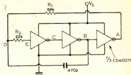
Fig. 13. Voltage-controlled adaptation of Fig. 12. Parts cost £1.00.
