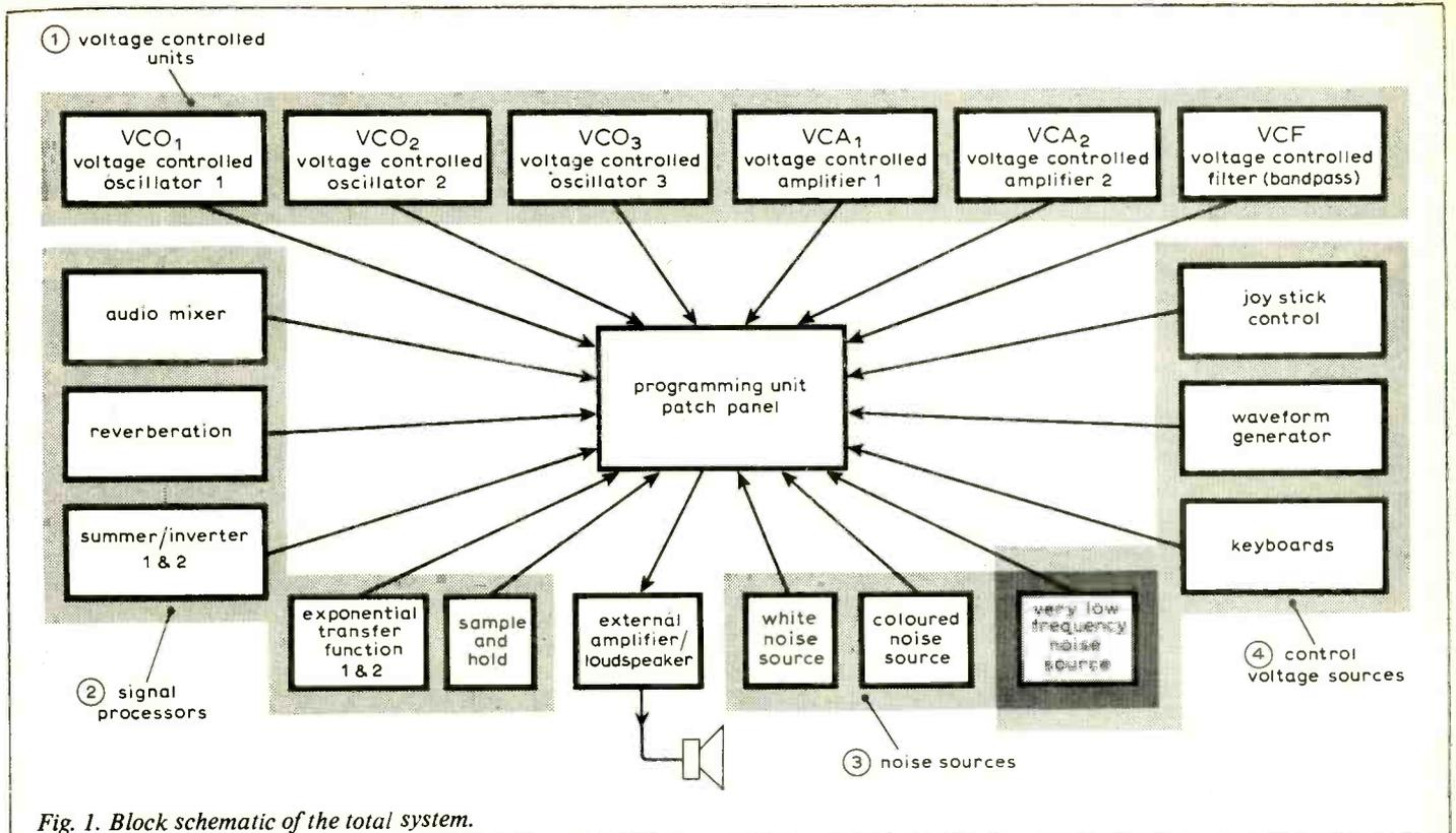
Fig. 1. Block schematic of the total system.
