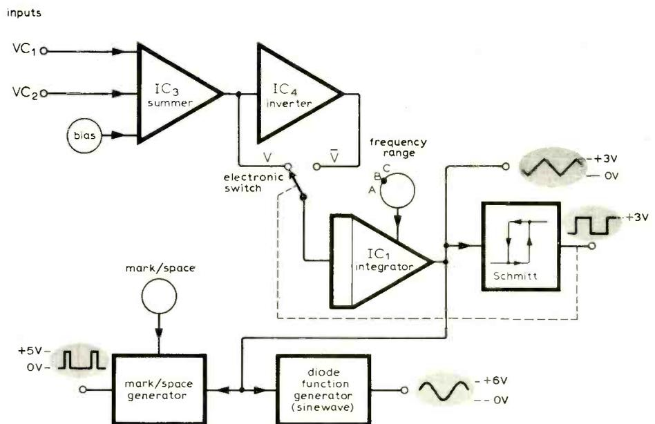
Fig. 3. Oscillator VCO<sub>1</sub> in block diagram form.
