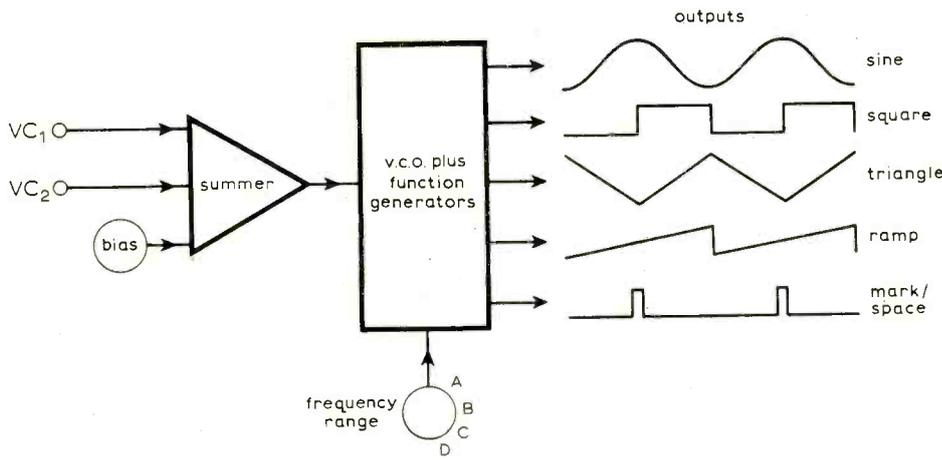
Fig. 9. Functions of voltage controlled oscillator  $VCO_2$
