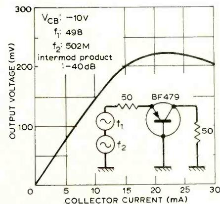
Fig. 2. Linearity of gain up to 15mA or so of BF479 improves cross-modulation performance, the gain control function being taken over by p-i-n diodes.
