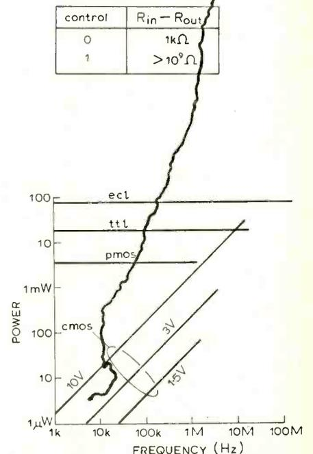
Fig. 8. For c.m.o.s. high speed means high power and low power means low speed.
