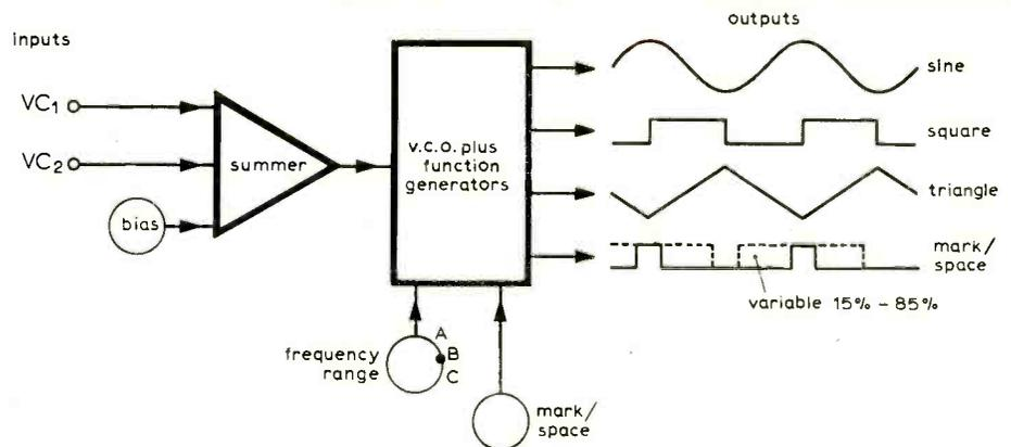
Fig. 2. Functions of voltage controlled oscillator, VCO<sub>1</sub>.
