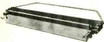
Forms channels and angles down to 45 degrees which can be flattened to give safe edge. Depth of fold according to height of bench.
