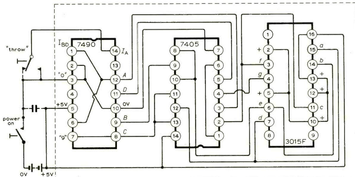
Fig.2. The layout of the circuit, seen from the component side.
