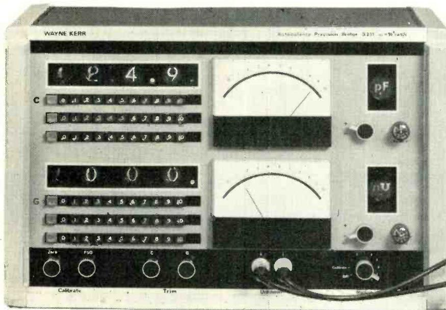
This bridge was designed for use in Standards Laboratories, but ease of operation combined with an in-line readout giving up to 6 figure discrimination has enabled many other applications to be covered.
