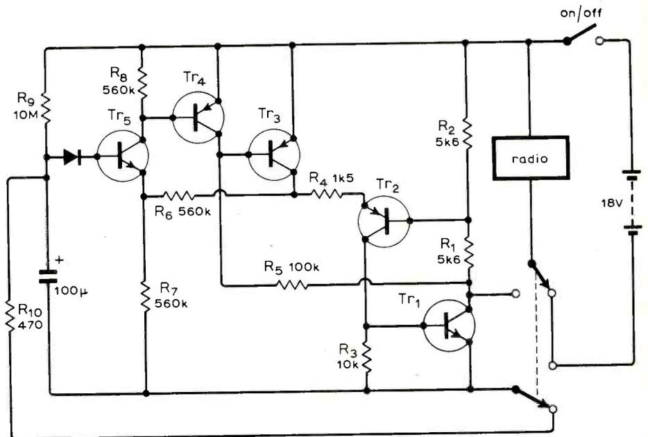
2N3706 for  $Tr_1, Tr_3$  and 2N3702 for  $Tr_2, Tr_3, Tr_4$ .) The capacitor must also have low leakage and some experimentation may be necessary. Resistor  $R_{10}$  discharges the capacitor rapidly to permit another operation immediately. The switch requires a good insulation resistance.
