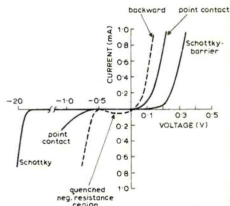
Fig. 1. Large differences in curvature at the origin of the  $I-V$  characteristics govern the behaviour of the diodes as detectors.
