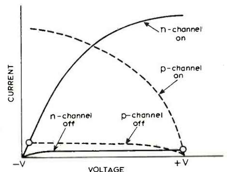
Fig. 3. Load lines of c.m.o.s. device show power dissipation to be low—says  $10\text{nW}$  per gate—in both on and off states.
