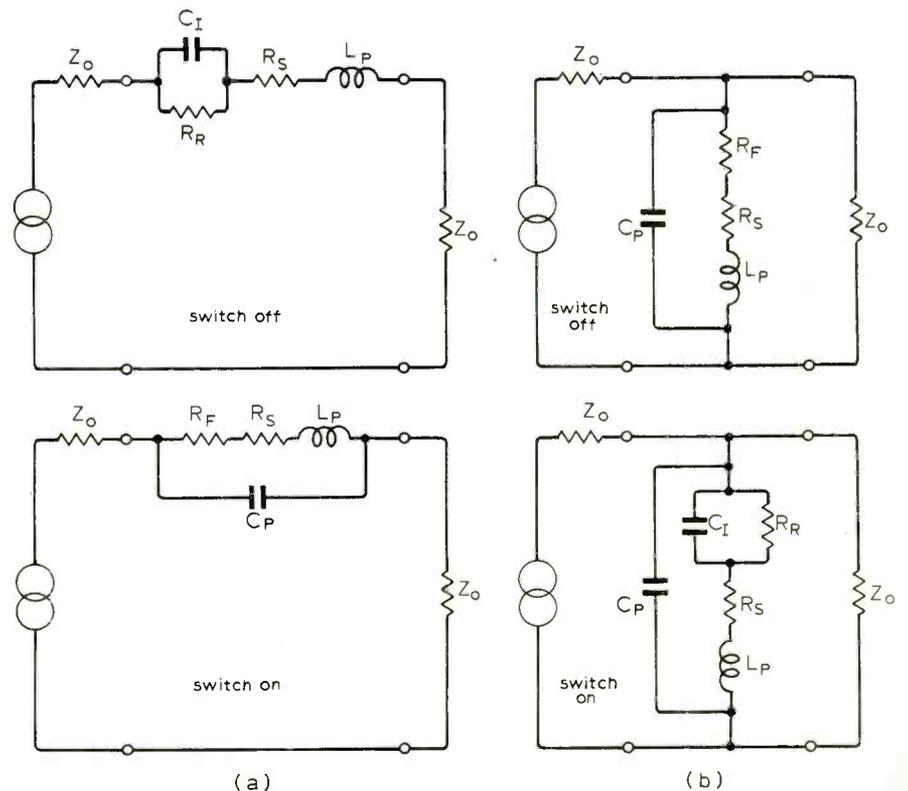
insertion loss is  $10 \log_{10} [2^2 + 2.5^2/4.5^2 + (2150) + 1] = 0.2\text{dB}$ . With the switch off under zero bias and again neglecting  $C_p$ ,  $R_F = 10\text{k}\Omega$  and some algebra indicates that the isolation provided is about 24dB.
