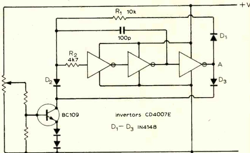
approach an equilibrium under the influence of the d.c. feedback the system switches to hard off when the loop gain round the first two inverters reaches unity. The feedback resistor then causes a current from point A to point D into the capacitor to move back toward the equilibrium. This results in a further regenerative switching edge in the reverse direction.
