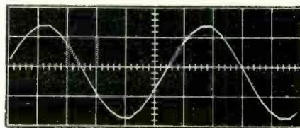
Oscillogram showing a 7-V pk-pk approximation to a 40-Hz sine wave. An harmonic distortion of 0.01% is readily achieved.
