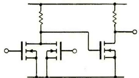
Fig. B. Linear or logical functions can be performed by this simple p-channel i.g.f.e.t. circuit, which can be directly-coupled provided the supply is greater than the threshold voltage.
