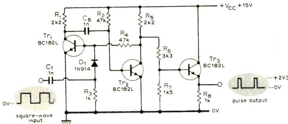
Fig. 12. Circuit of the pulse function generator.
