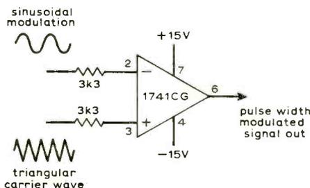
Fig. 12.1 Op-amp used for pulse width modulation.
