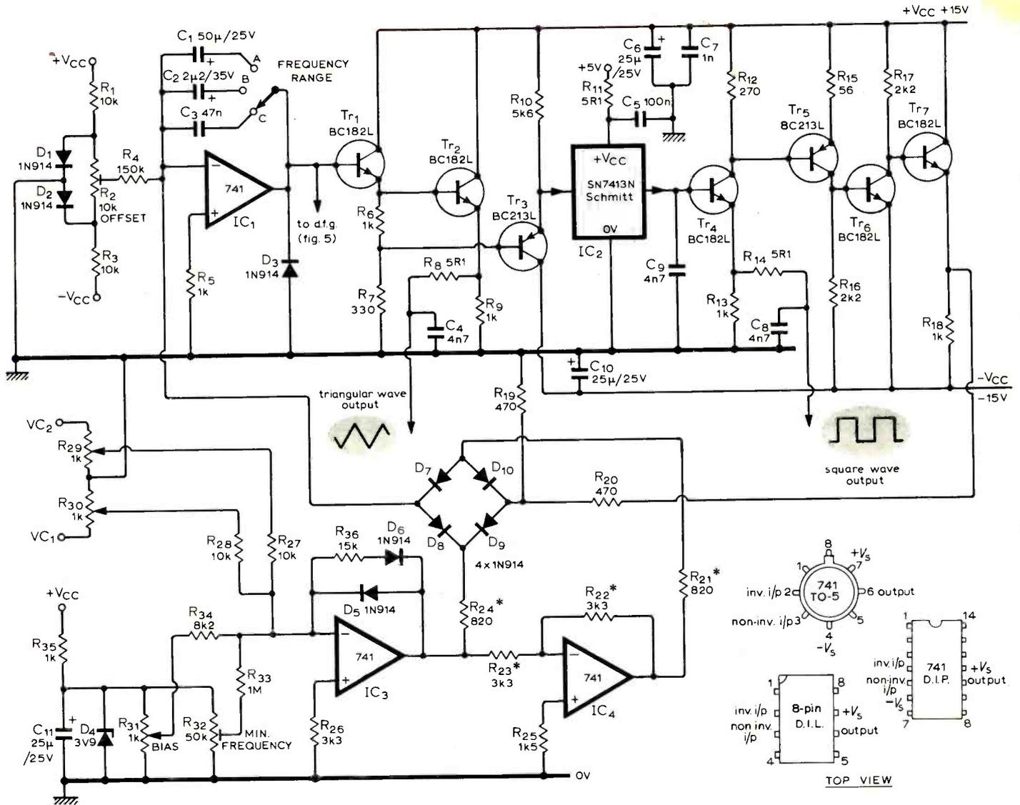
Fig. 4. Circuit of VCO<sub>1</sub>. All resistors are 5%, 1/4W unless asterisked — these are 2%.
