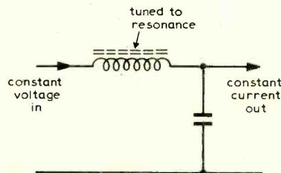
Fig. 2. Gyrator network to convert constant-voltage square wave to constant-current tube drive.
