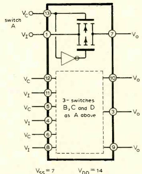
Fig. 11. This quad bilateral switch enables switches to be fully floating.
