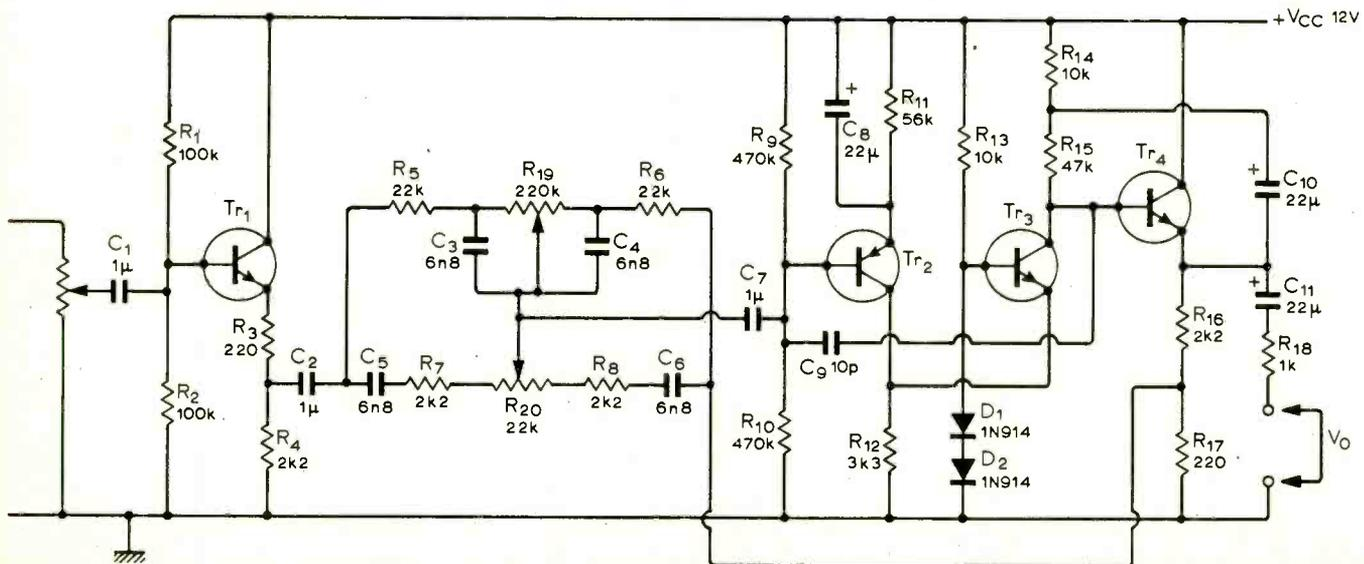
Fig. 1. Circuit diagram of tone control. Transistors  $Tr_1, Tr_3, Tr_4 = BC109, BC114, BC184$ .  $Tr_2 = BC15, BC214, BC309$  etc.
