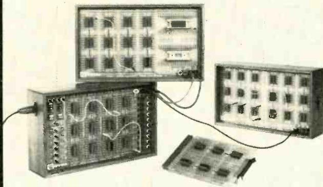
Limrose's new family of low-cost universal mounting boards, plug-in cards and breadboarding systems is useful for development work, device testing and circuit evaluation. Delivery is usually ex-stock. For prices and other information please contact
