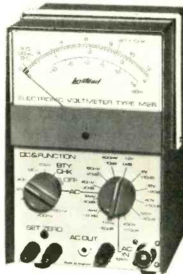
The M2B based on our well tried M2A has been completely redesigned mechanically with a vertical construction that takes only 5" x 5" of bench space. The carrying handle sits neatly on top of the instrument or may be used as a rest when operated in a sloping position. The A.C. frequency range is now 10 Hz to 1 MHz with amplifier output having a maximum gain of 600 times. A feedback circuit linearises the scales and readings start at 60 microvolts. Input impedance on A.C. and D.C. is 10 Megohms.
