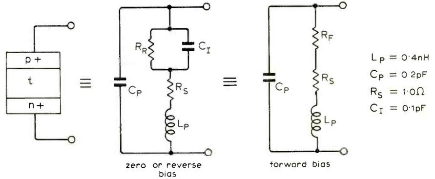
Fig. 4. Equivalent circuits for reverse and forward bias conditions of a silicon p-i-n diode.  $R_S$  is the series resistance associated with the contacts to the i-region of the diode and  $C_I$  is the intrinsic-region capacitance. Values of  $L$  and  $C_p$  are typical of devices used up to the end of X-band (8200 to 12,400MHz).
