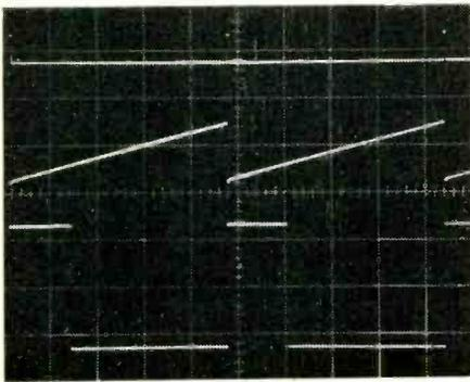
Fig. 15.2 Action of Fig. 15.1 circuit. Top trace shows positive reset pulses; middle trace, integrator output; bottom trace, comparator output. Vertical scale, 10V/div.; horizontal scale, 2ms/div.
