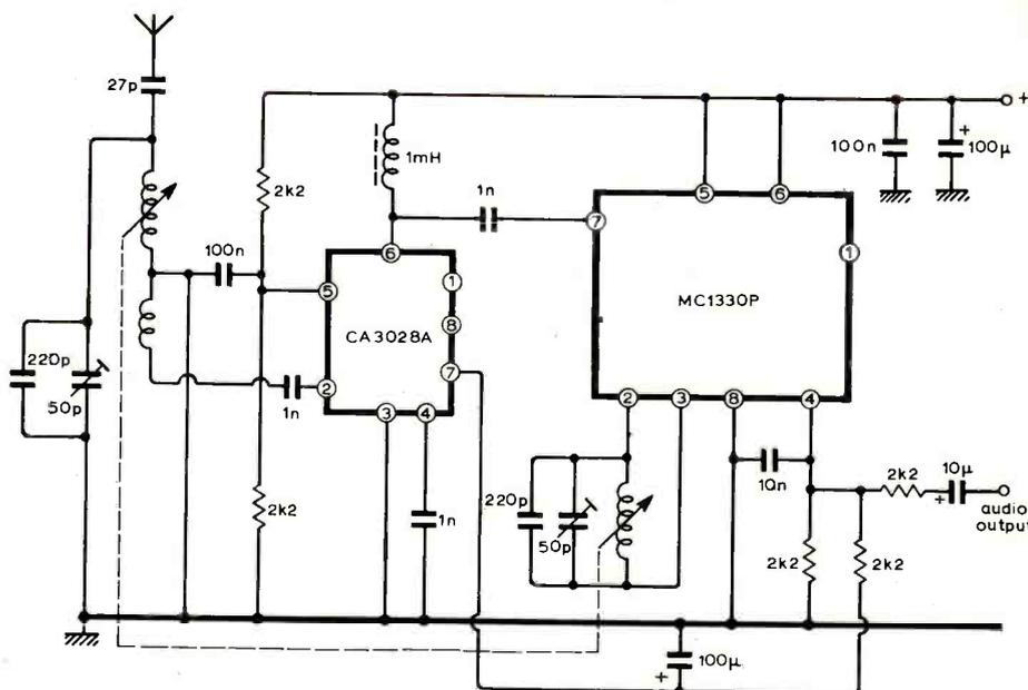
Fig. 5. Circuit of the complete homodyne broadcast tuner.
