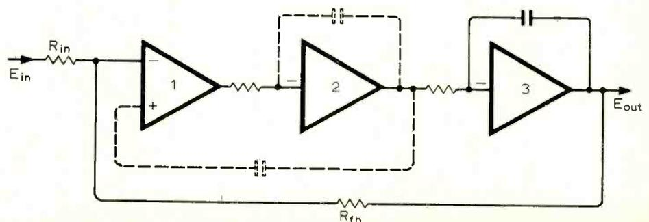
this bandwidth, the known gain of the circuit, and the thermal noise of the input elements. If now one connects across the feedback circuit the components necessary to provide the falling h.f. gain characteristic of the R.I.A.A. curve, the output noise will drop, simply because one has restricted the effective noise bandwidth. If this were not the case, the series feedback connection using an inductive input would be worse than it is.
