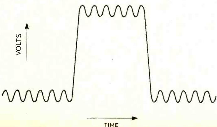
Fig. 25. Test signal used to probe incremental gain.
