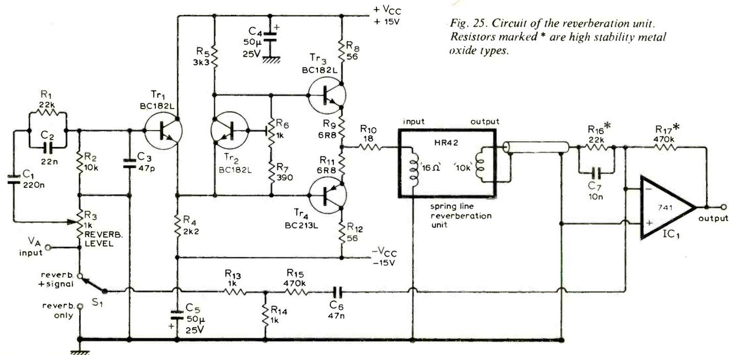
Fig. 25. Circuit of the reverberation unit. Resistors marked \* are high stability metal oxide types.
