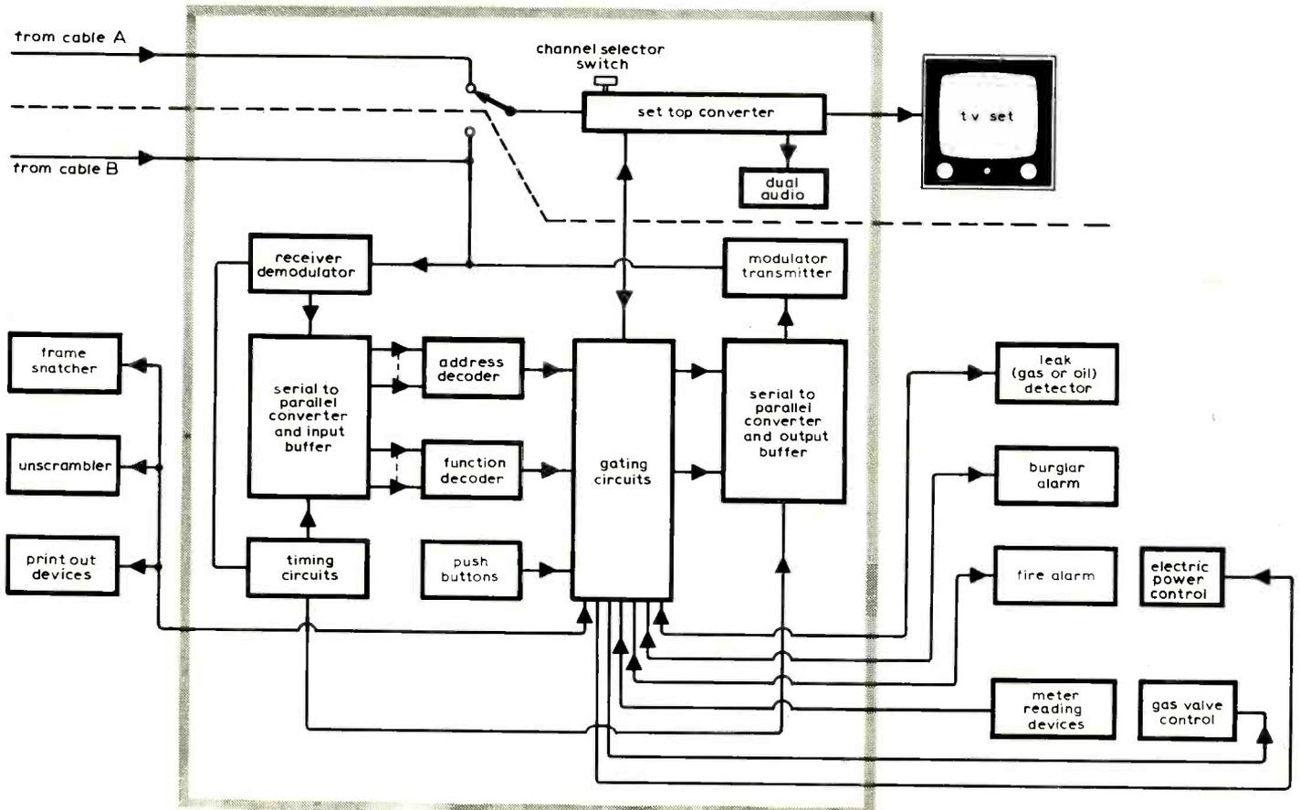
Fig. 2 Subscriber's equipment for TICCIT system (see Fig. 1).
