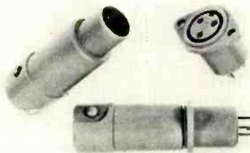
The chassis socket is flange mounted and the free plug has an unusual cable grip providing a firm anchorage. Cables from 5.8-6.5mm diameter may be used. The mated length is 63mm and diameter 18mm. Sealectro Ltd, Walton Road, Farlington, Portsmouth, Hants PO6 1TB.
