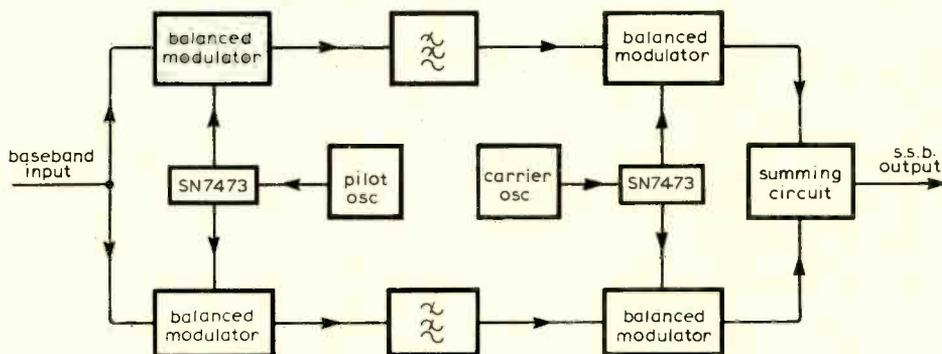
Fig. 6. Block diagram of the modified third method of s.s.b. signal generation.
