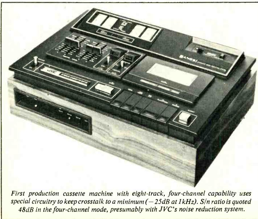
First production cassette machine with eight-track, four-channel capability uses special circuitry to keep crosstalk to a minimum (–25dB at 1kHz). S/n ratio is quoted 48dB in the four-channel mode, presumably with JVC's noise reduction system.
