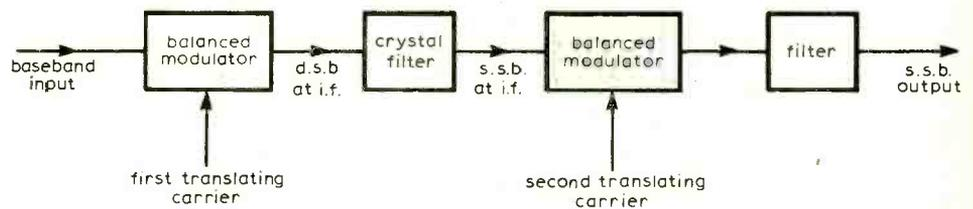
Fig. 1. Filter method for the generation of an s.s.b. signal.
