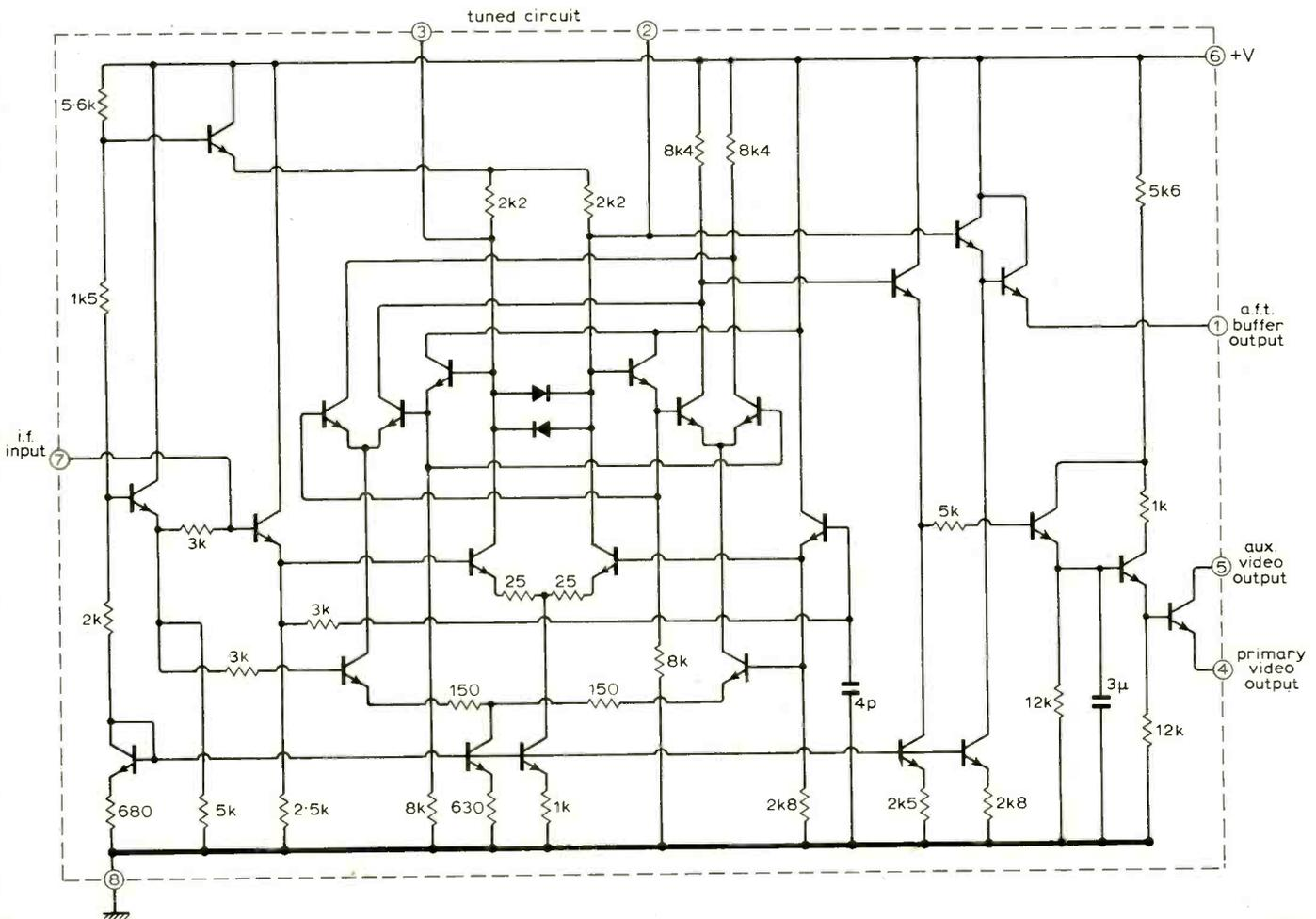
Fig. 4. Circuit diagram of MC1330P.
