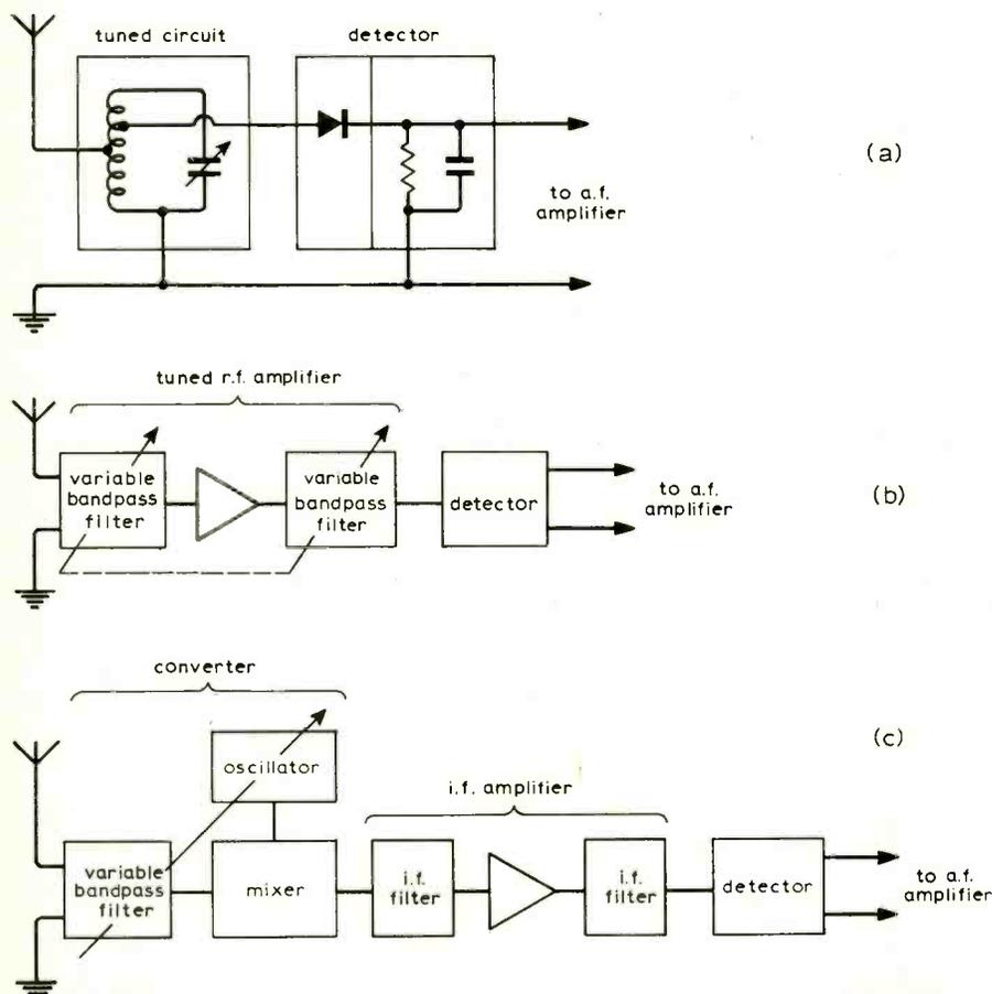
Fig. 1. Broadcast receiver detector and demodulator systems.
