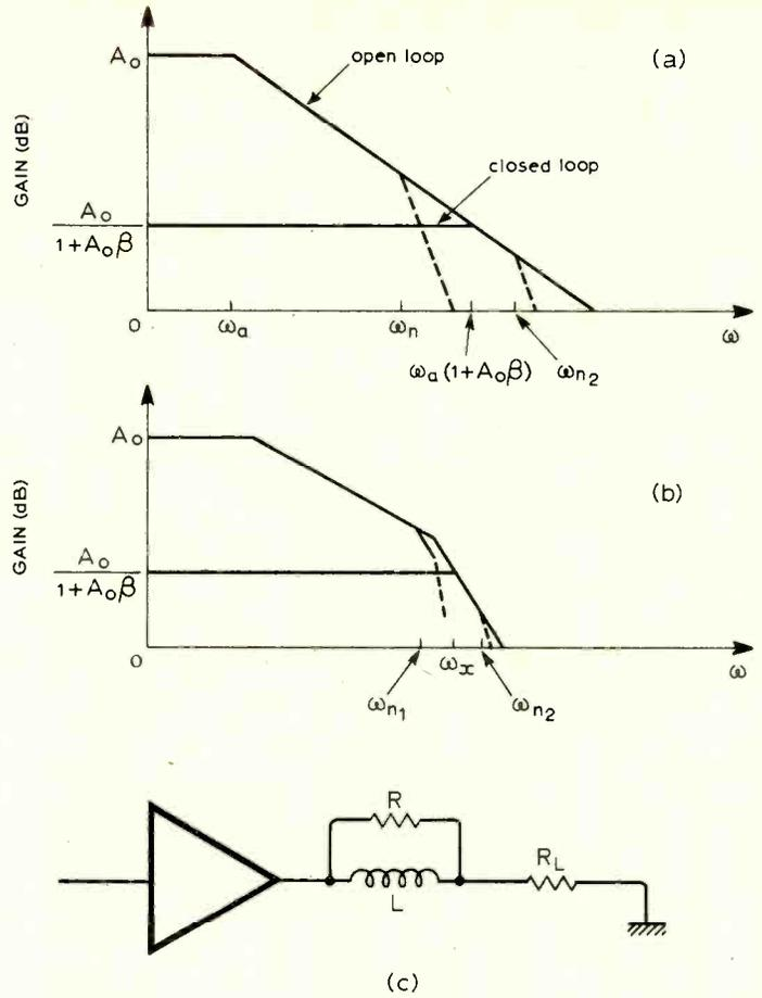
Fig. 21. Loop gain and phase characteristics of single pole amplifier.
