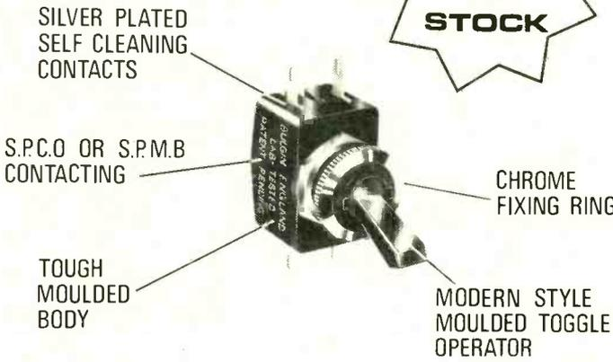
A new ingenious design of moulded Toggle switch employing a QMB wiping contact action, for AC/DC compatibility and heavy silver plated contacts/tags for long life. Illustrated is S.910. S.P.C.O. rated 2A at 250V. AC., is S.900 Make-Break contacting, rated 3A at 250V. is also available.
