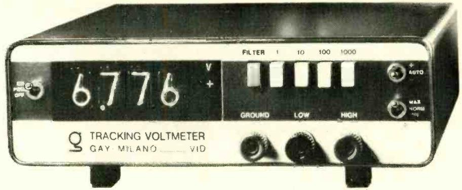
"maximum" and "minimum" peak holding memory modes. In the "maximum" mode the polarity switch can select either positive or negative peaks, whilst in the "auto" polarity position the absolute peak value (greater of positive or negative) is displayed, the polarity indicator acting as a polarity memory.
