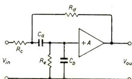
Fig. 2. Example of a band-pass active filter.
