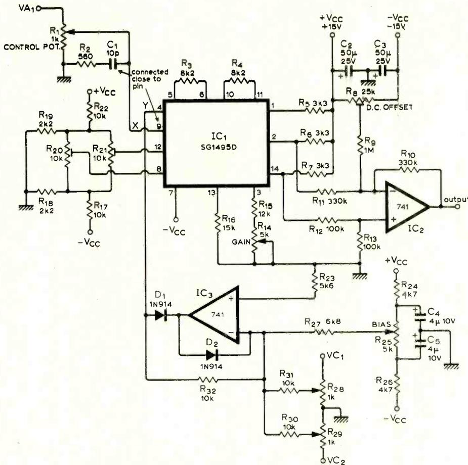
Fig. 18. Circuit diagram of voltage controlled amplifier  $VCA_{1,2}$ .
