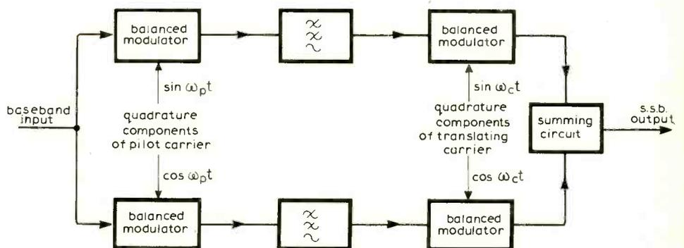
Fig. 3. Block diagram of the third method of s.s.b. signal generation, which involves both filtering and phasing techniques.
