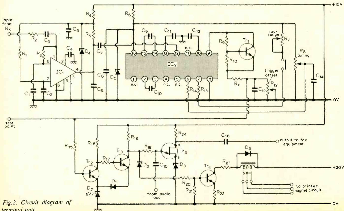
Fig.2. Circuit diagram of terminal unit.
