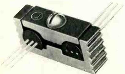
heat sinks for temperature balancing are the type 5DC/HA, providing a thermal rating of 50°C/W for use with TO5 transistors, and the 18DC/HA with the same thermal rating, but for use on TO18 transistors. Prices for these are 21.3p and 20p each respectively (for quantities again in excess of 100). Celdis Ltd, 37/39 Loverock Road, Reading, Berks, RG3 1ED.
