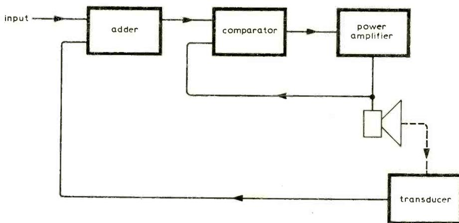
Fig. 1. Block diagram of the method used for deriving a corrective signal from a speaker's movement.
