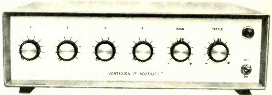
The mixer is arranged for 2-30/60 $\Omega$  balanced line microphones, 1-HiZ gram input and 1-auxiliary input followed by bass and treble controls. 100 volt balanced line output or 5/15 $\Omega$  and 100 volt line.
