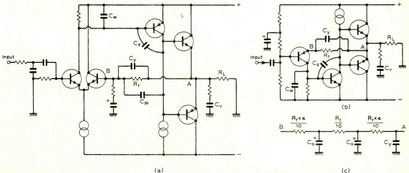
Fig. 11 (a), (b). Two typical amplifier configurations used to establish methods of measuring open and closed loop circuit performance. (c) Substitution of feedback resistor  $R_f$  by test jig circuit.
