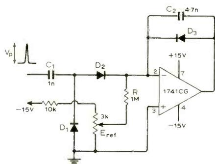
Fig. 13.1 Conversion of pulse height to time.
