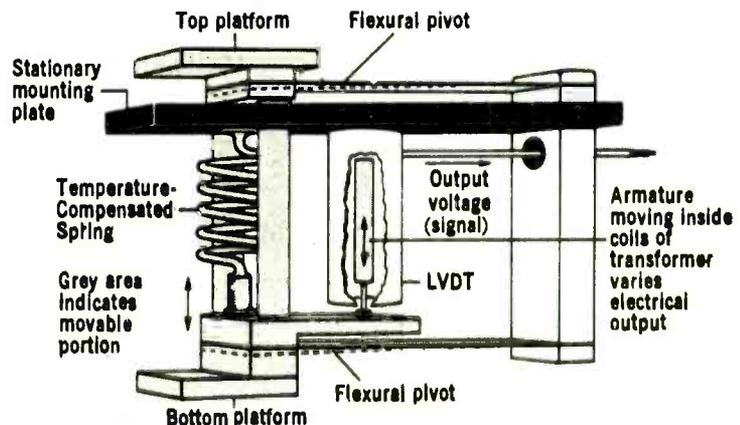
Fig. 1. The Hunting l.v.d.t. weighing cell.
