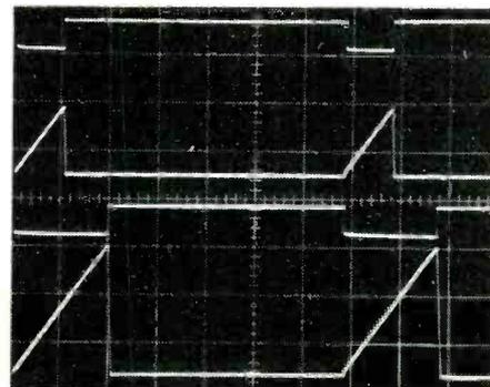
Fig. 14.2 Action of Fig. 14.1 circuit illustrated by negative-going rectangular-pulse gating signals of different widths. Rectangular waves, 5V/div.; ramp waveforms 2V/div.; horizontal scale 2ms/div.
