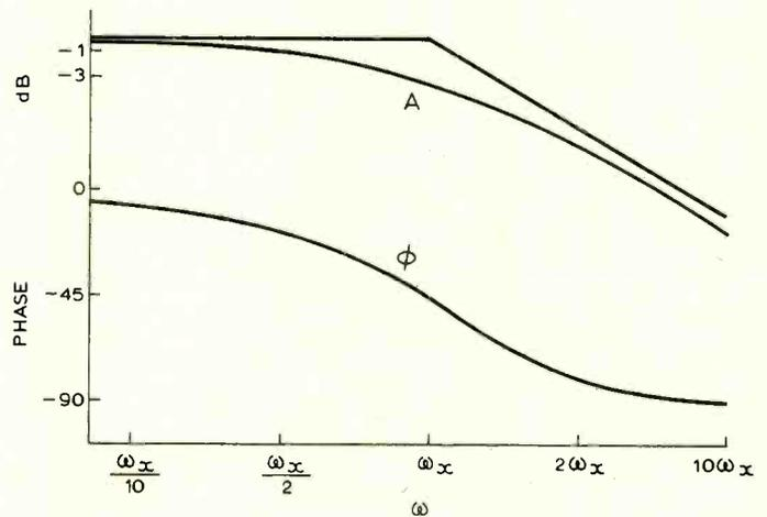
Fig. 22. The projected effect on distortion of the amplifier loop characteristic.
