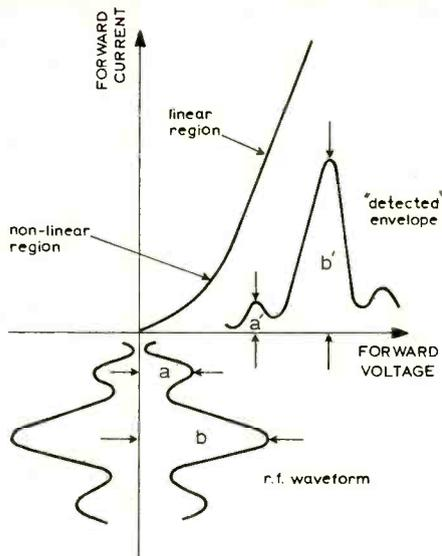
Fig. 2. Diode detector characteristics and operation.
