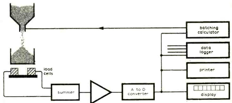
Fig. 2. A possible configuration of a complete weighing system with ancillary recording and batching equipment. The batching controller detects coincidence between the digital output of the display unit and a preset number, and controls the hopper output.
