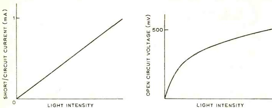
Figs. 5 & 6. In light-sensitive devices based on a p-n junction, current is a linear function of light intensity falling on the junction (Fig. 5, left). Open-circuit voltage can be as high as 0.5V with silicon photodiodes (Fig. 6, right).
