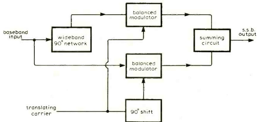
Fig. 2. Block diagram of the phasing method for s.s.b. signal generation.
