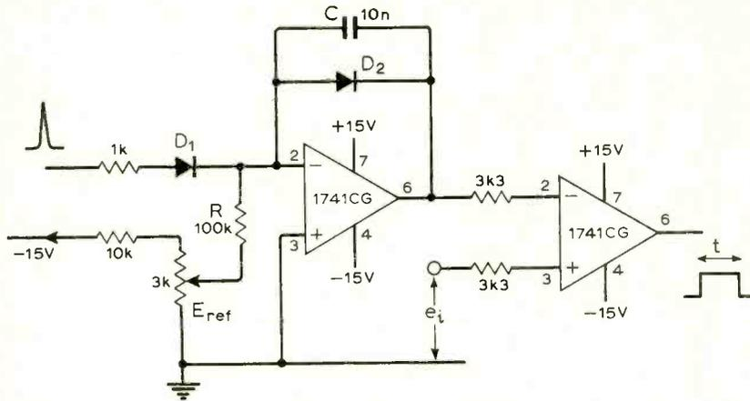
Fig. 15.1 D.C. voltage to time conversion, achieved by adding a comparator to Fig. 13.1 circuit.
