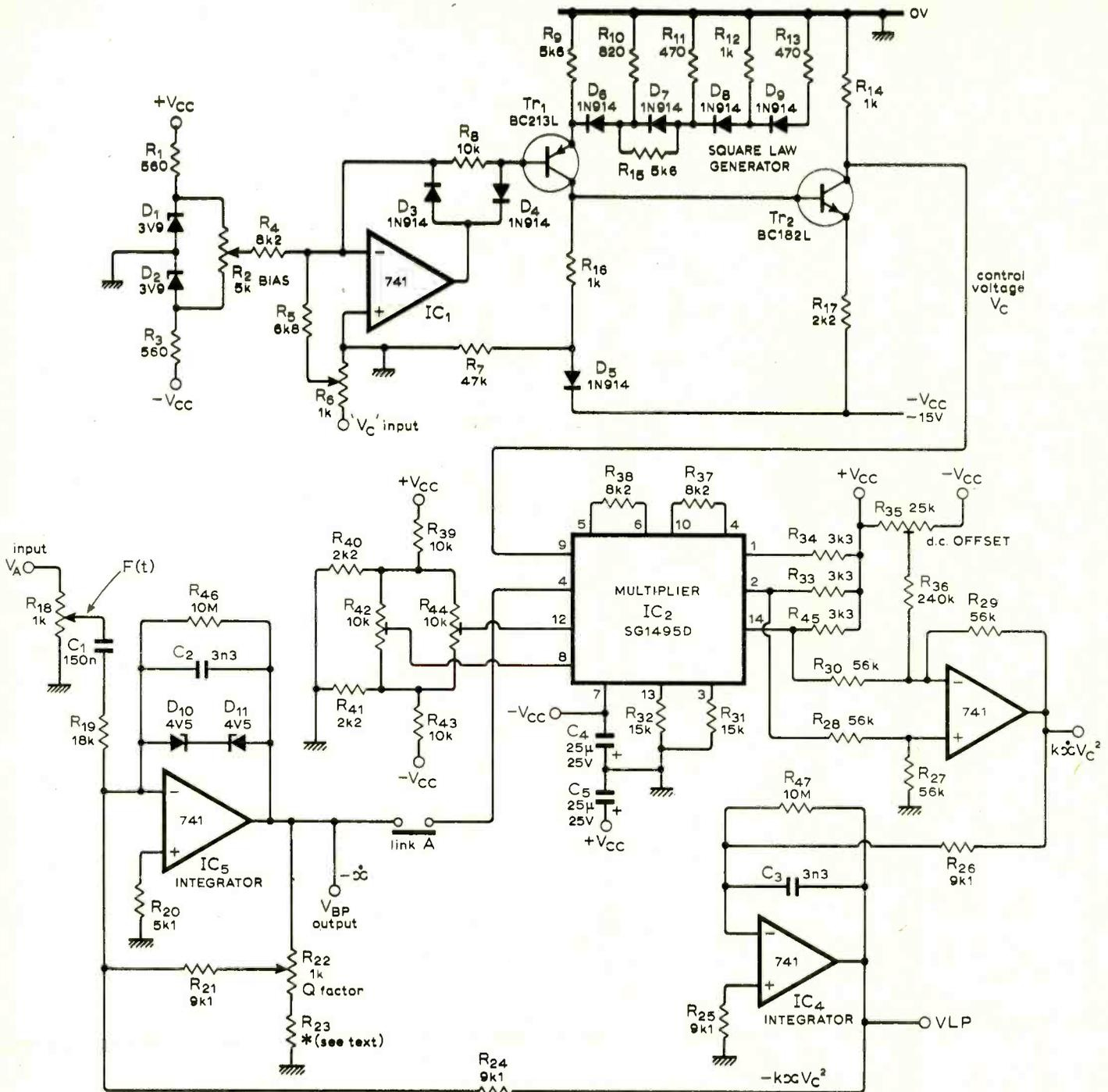
Fig. 20. Circuit of the voltage controlled filter.
