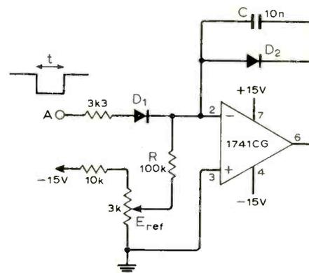
Fig. 14.1 Circuit for time to voltage conversion.
