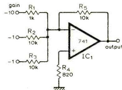
Fig. 24. Direct coupled virtual-earth mixer.
