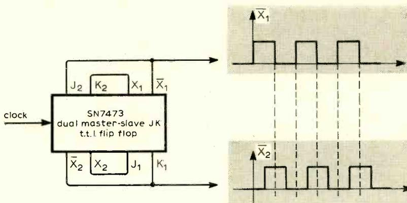
Fig. 5. Use of a t.t.l. i.c. to obtain quadrature square-waves.
