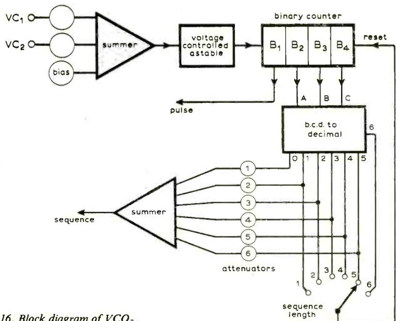
Fig. 16. Block diagram of  $VCO_3$ .
