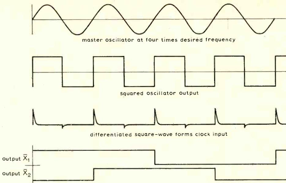
Fig. 4. Stages in the production of quadrature square-waves.
