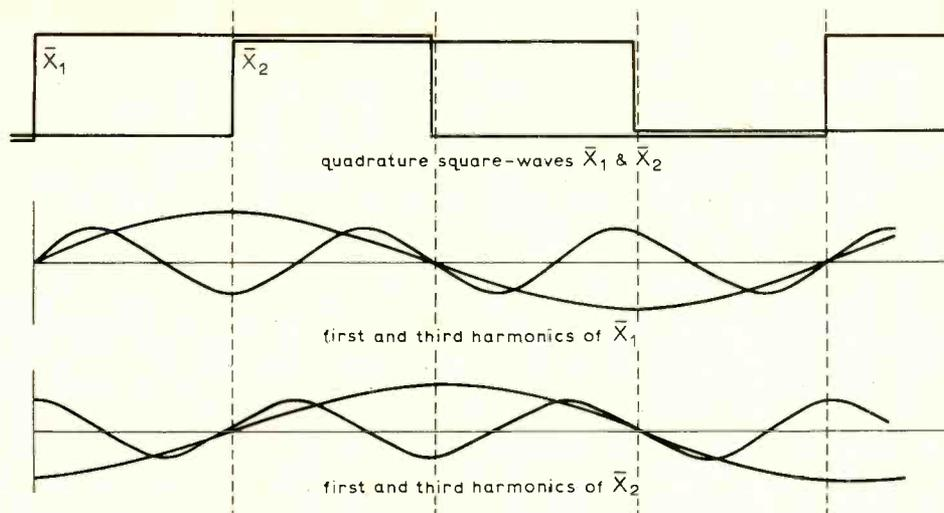
Fig. 7. Harmonic components of the quadrature square-waves, which also form quadrature pairs.
