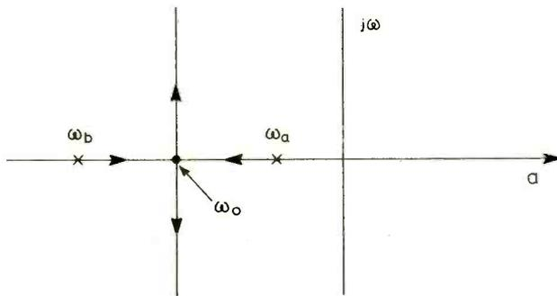
Fig. 18. An  $s$ -plane plot showing the effect of negative feedback on the natural frequencies of the two pole system shown in Fig. 17.
