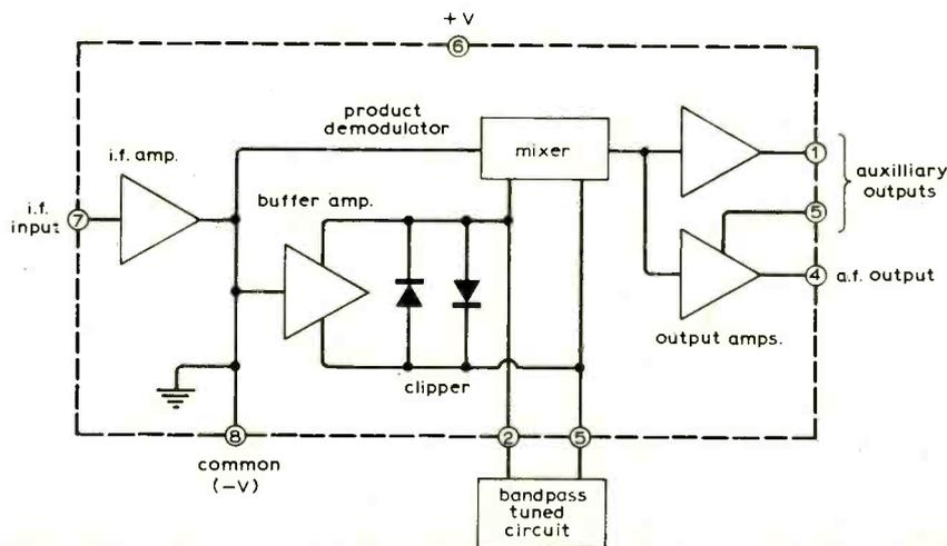
Fig. 3. Block diagram of MC1330P i.c. demodulator.
