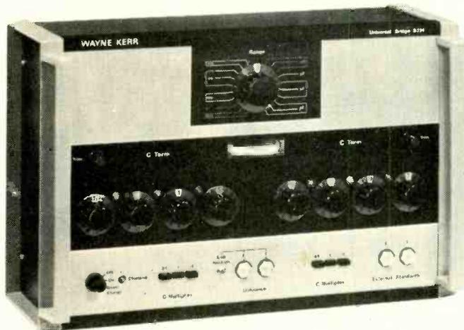
**The B224 is a manually operated bridge,** the resistive and reactive terms being independently set to a null indicated on the meter. A rechargeable battery is fitted in order to make the instrument portable.
