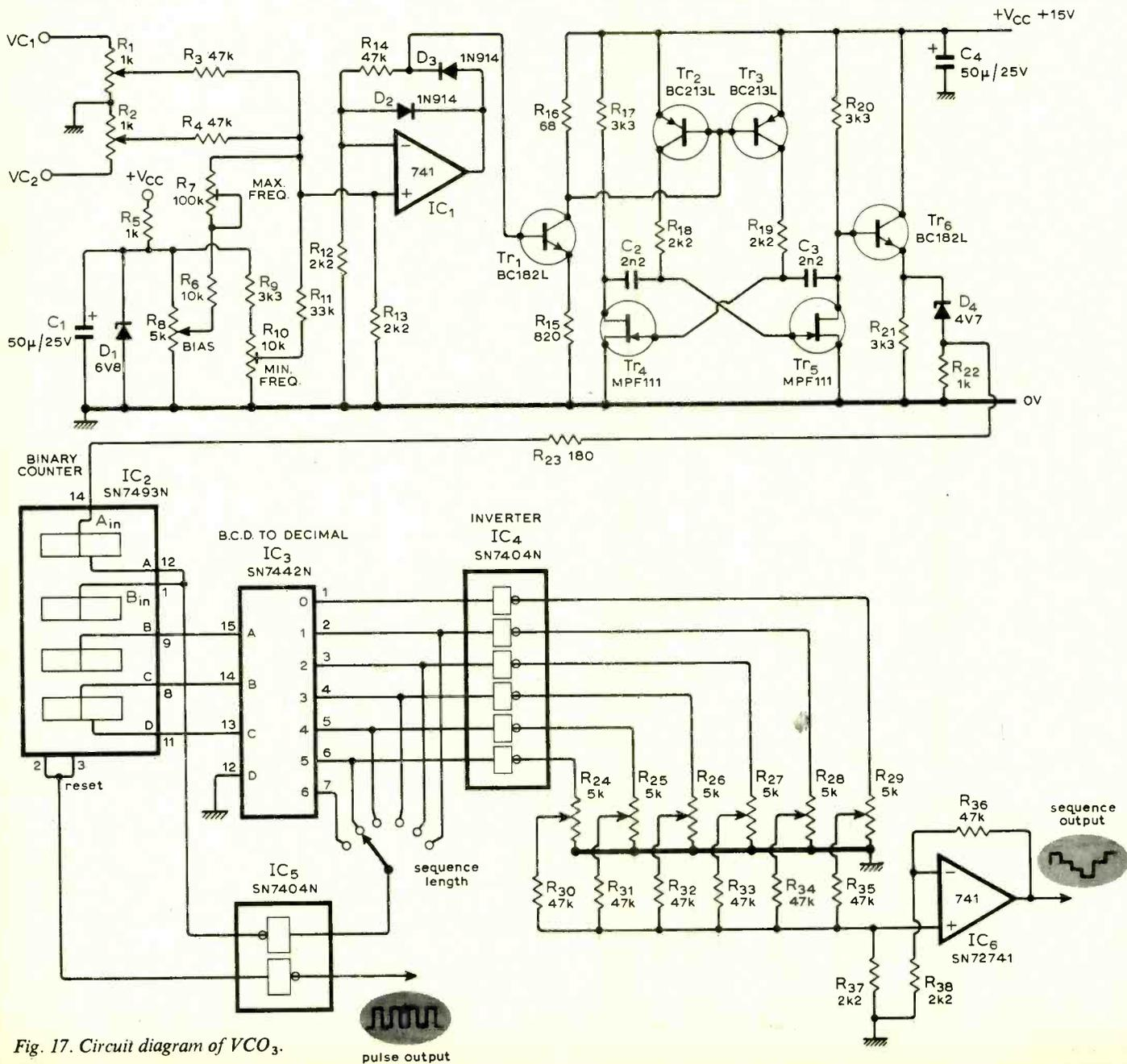
Fig. 17. Circuit diagram of  $VCO_3$ .
