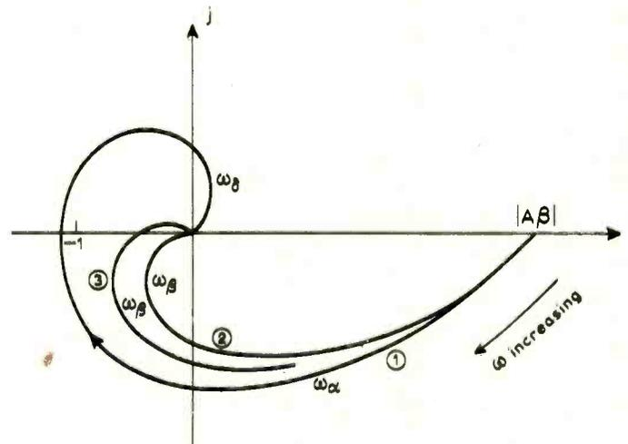
Fig. 15. Loop gain characteristic of a marginally stable amplifier.
