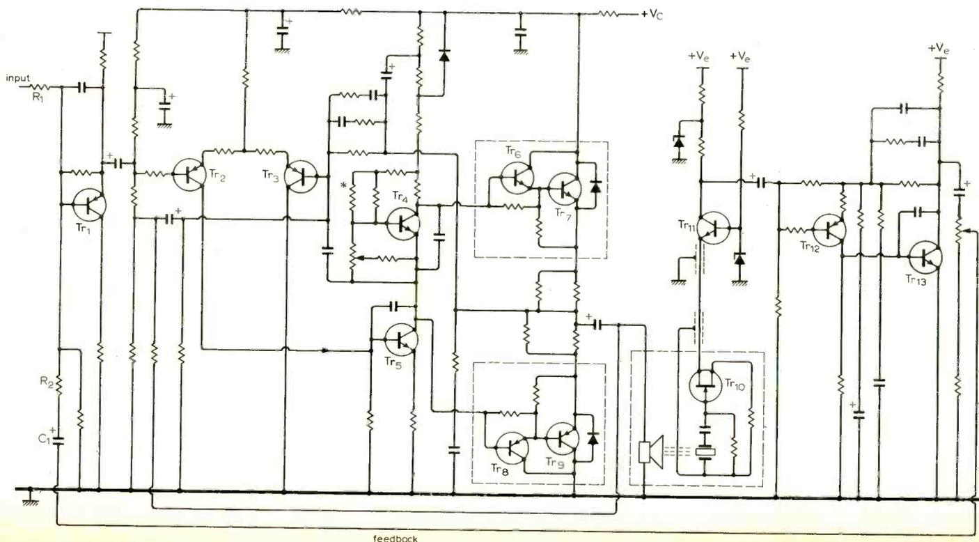
the inability of the system to cope with the condition cone velocity  $\propto$  frequency<sup>2</sup> for a constant sound pressure level. If the motion of the cone can be sensed in some way to generate a current proportional to the speaker's acceleration, then this can be compared with the input signal and a corrective signal generated to force the cone to move in the manner originally dictated to it.
