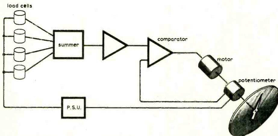
Fig. 3. A dial indicator in basic form. Batching can be carried out either by using the analogue signal or by causing the pointer to actuate photo-cell or inductive trips.
