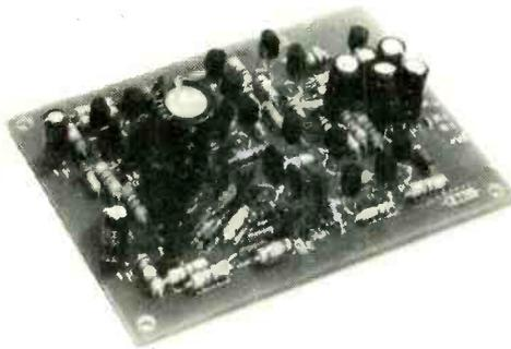
**High definition SQ\* quadrasonic decoder Fully built home constructor module**
