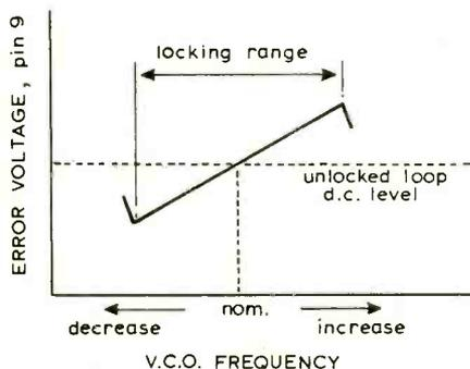
Fig. 1. Response of phase-lock-loop over locking range.
