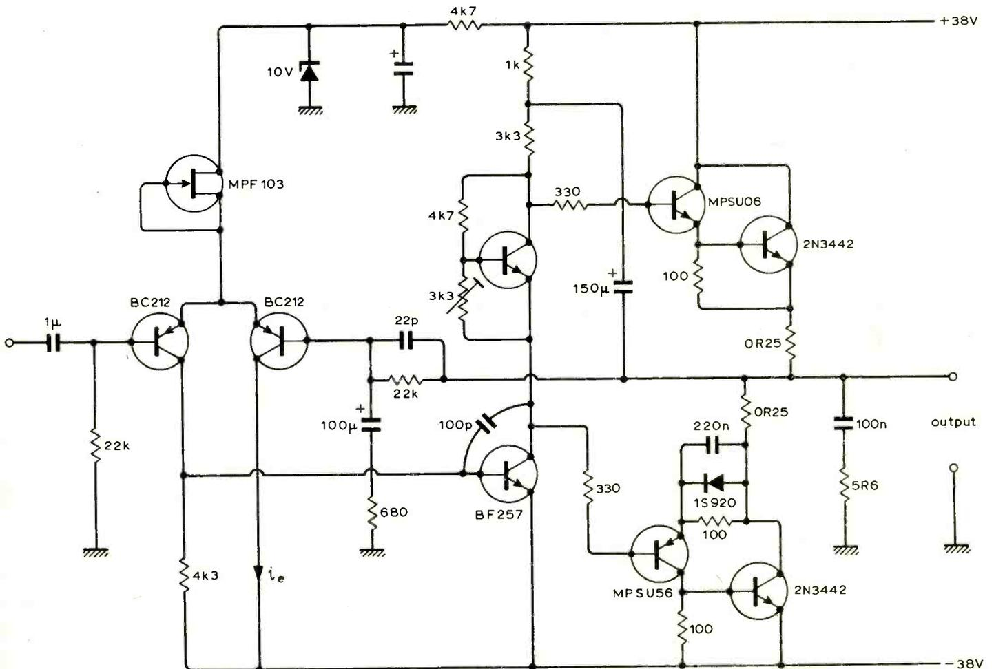
Fig. 26. Basic amplifier design produced to test transient distortion analysis.
