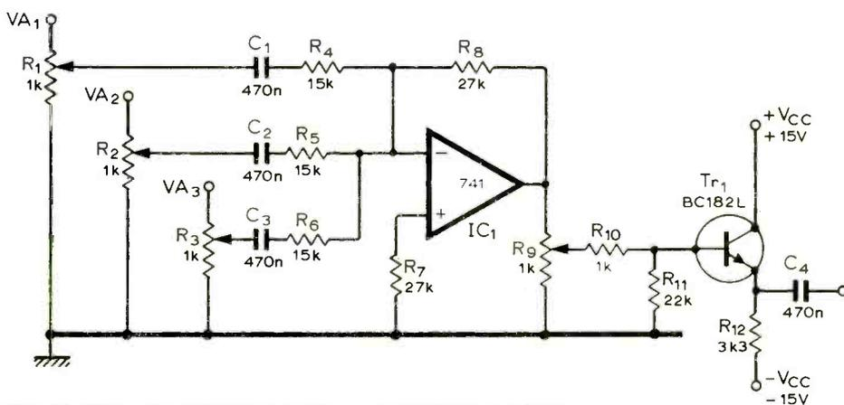
Fig. 23. Three-channel virtual-earth a.c. coupled mixer circuit.
