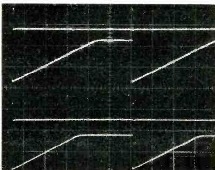
Fig. 13.2 Action of Fig. 13.1 circuit illustrated by input pulses of different heights. Pulse waveforms, 10V/div; integrator outputs, 1V/div; horizontal scale 1ms/div.
