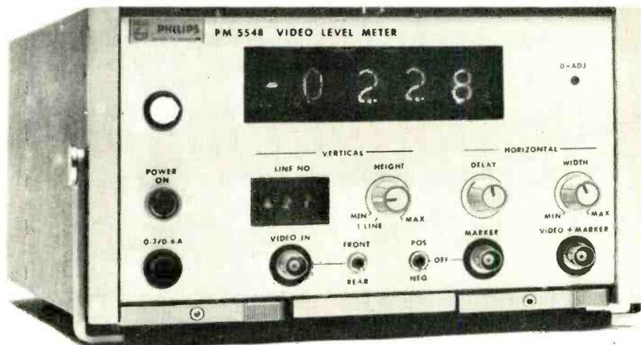
A new video-signal level meter was shown for the first time by Philips at this year's International Television Exhibition in Montreux and is available from Pye Unicam Ltd. Designed to perform signal-level measurements on composite TV signals, the PM 5548 is claimed to be the first instrument of its type available anywhere in the world.
