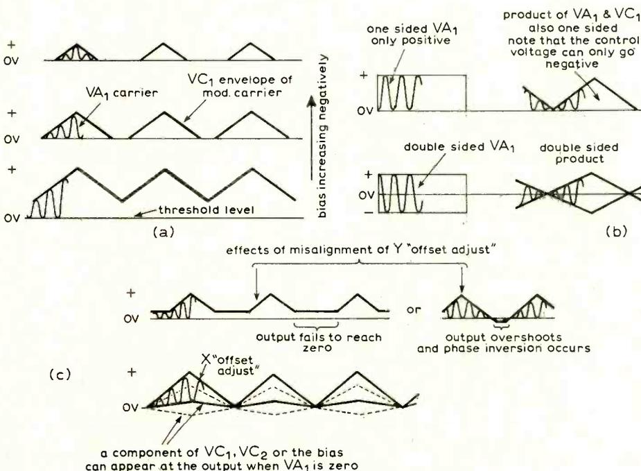
Fig. 19. (a) Variable threshold effect in aligning the v.c.as. (b) Waveform envelopes from  $VA_1$  and  $VC_1$  products. (c) Effects of misaligning the Y "offset adjust". See text for full explanation.
