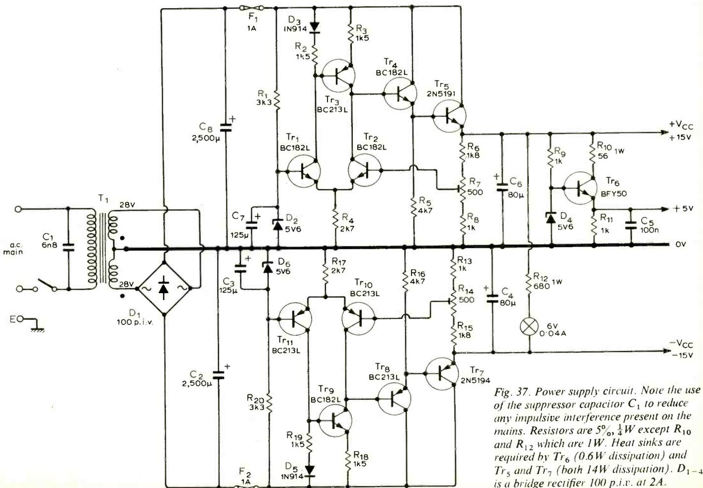
Fig. 37. Power supply circuit. Note the use of the suppressor capacitor  $C_1$  to reduce any impulsive interference present on the mains. Resistors are 5%, 1/4W except  $R_{10}$  and  $R_{12}$  which are 1W. Heat sinks are required by  $Tr_6$  (0.6W dissipation) and  $Tr_5$  and  $Tr_7$  (both 14W dissipation).  $D_{1-4}$  is a bridge rectifier 100 p.i.v. at 2A.
