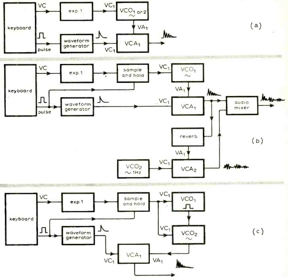
Fig. 36. Three examples of how the patch-board can be programmed for a particular sound synthesis. See text for explanation.
