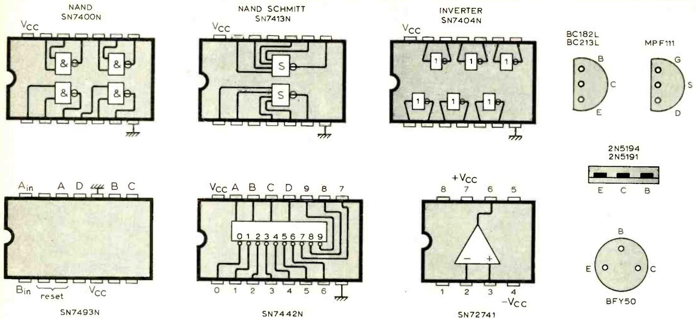
Pin connections for the transistors and integrated circuits used in the synthesizer's circuitry.
