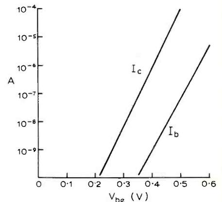
Fig. 1. Variation of  $I_c$  and  $I_b$  against  $V_{be}$  for a low leakage planar silicon transistor operated at constant  $V_{ce}$ .
