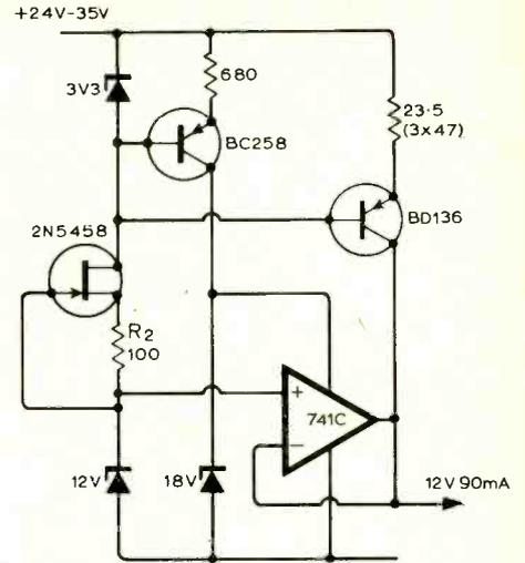
With the values shown the constant-current supplied is about 100mA of which 10 to 15mA are "sunk" by the 741. The circuit requires careful setting up as the current that can be sunk is severely limited. Coarse adjustment of the current source is achieved by altering  $R_1$ , the BD136 emitter resistor, fine adjustment by  $R_2$ .
