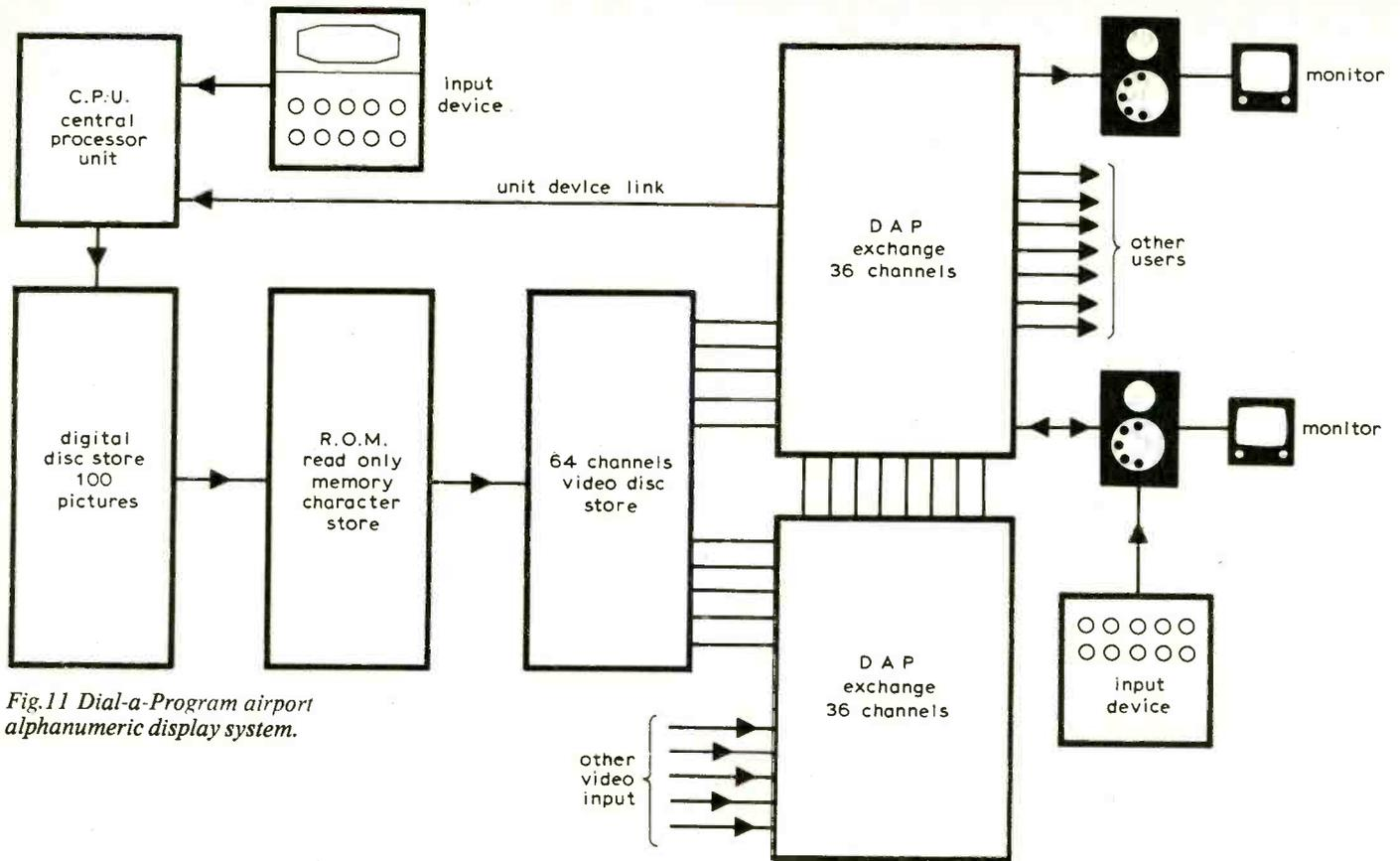
Fig.11 Dial-a-Program airport alphanumeric display system.
