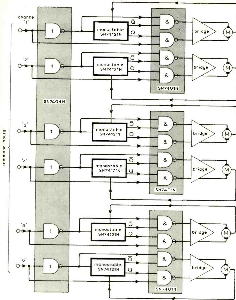
Fig. 6. Layout of components for least cost.
