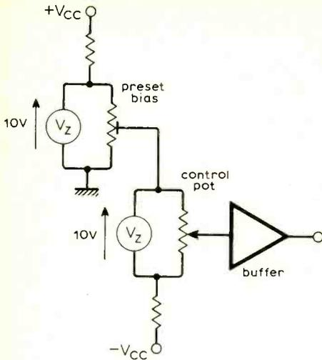
Fig. 34. Illustration of the joystick control circuit function.
