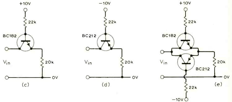
Fig. 5. (a) Conventional and (b) inverted transistor switches. Test circuits, using n-p-n and p-n-p devices are shown in (c) and (d) and (e) in the final form using both types.
