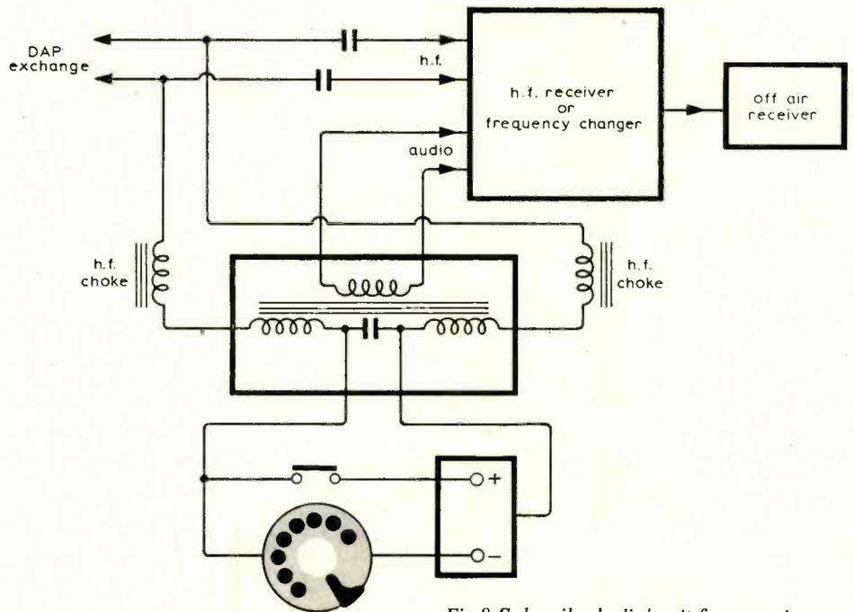
Fig. 8 Subscriber's dial unit for two-wire Dial-a-Program system.
