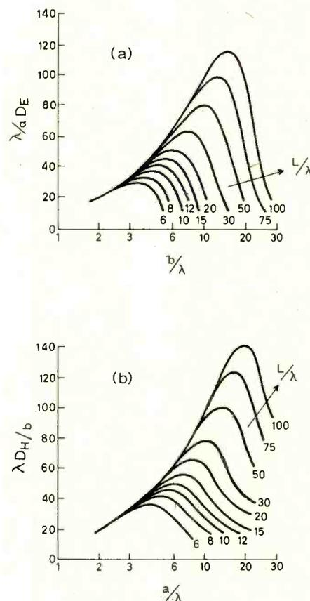
Fig. 3. For a fixed length of horn, directivity increases as the aperture widens and passes through a maximum value. Composite plots are shown here of the directivities of (a) E-plane and (b) H-plane sectoral horns having various lengths. Dimensions for an optimum horn can easily be seen.
