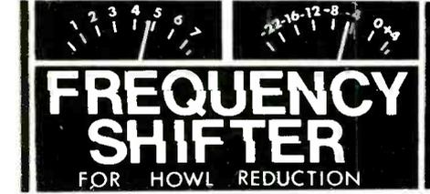
\* Public address \* Loudspeaker talkback \* Telephone broadcast programmes when caller leaves receiver on. Unity gain mains powered box 190 x 55mm, with bypass switch, shifts input 5Hz up in frequency and allows 6-8dB more gain before howl-round.
