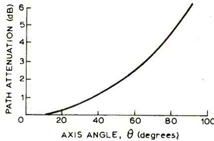
Fig. 7. Natural  $1/r^2$  variation in radiated energy contributes towards the aperture taper and must be taken into account when designing the feed.
