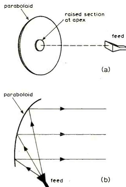
Fig. 9. Aperture blocking by the feed reduces the gain and degrades the side-lobe level of the paraboloid antenna and several methods exist for reducing the effect. Two are shown (a) raising the apex of the dish and (b) offsetting the feed.
