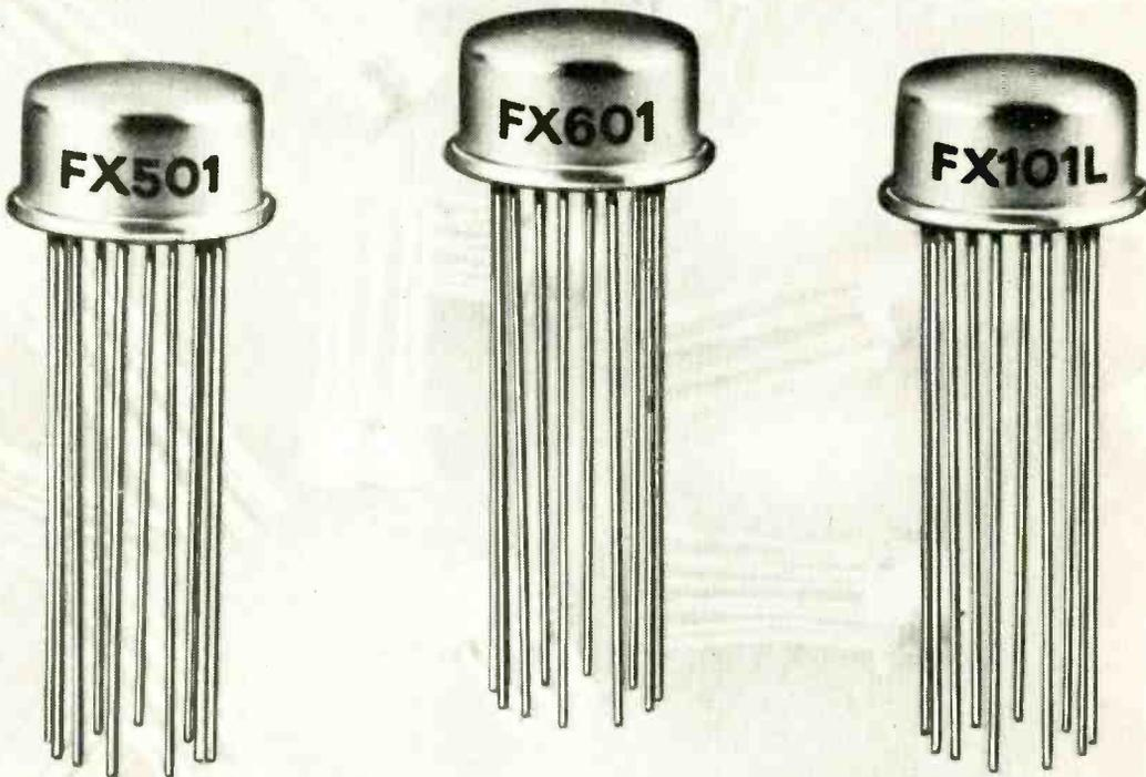
The FX-101L, FX-501 and FX-601 series of tone operated switches are designed for use as tone receivers in Remote Control, Alarm, Automation, Communications and Telemetry systems. Each device incorporates a semiconductor switch which operates when a specific input tone frequency is received. A choice of Direct Acting, Bistable or Monostable switching functions are available according to the device type. All frequency discrimination and timing
