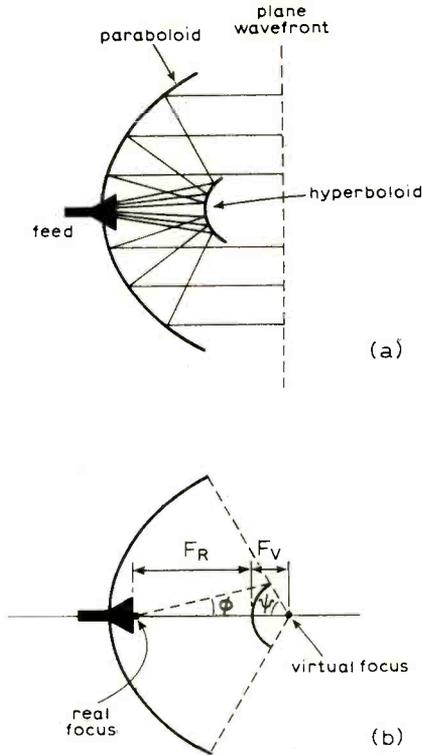
Fig. 10. Cassegrain antenna uses an additional element in the form of an hyperbolic sub-reflector and has an effective focal length which is longer than the focal length of the parabola. An image of the feed is formed at the virtual focus and illuminating radiation appears as coming from this point.
