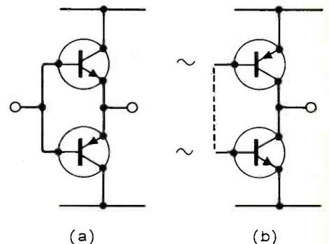
Fig. 3. Replacement of a complementary pair of emitter followers (a) by common emitter stages with emitters taken to opposite sides of the supply (b).
