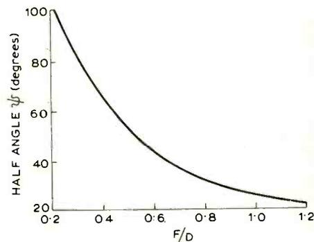
minating beam, thereby introducing more aperture blocking, while the large dish makes feed design difficult in obtaining a uniform phase. Generally, parabolas have an  $F/D$  ratio of between 0.3 and 0.5.
