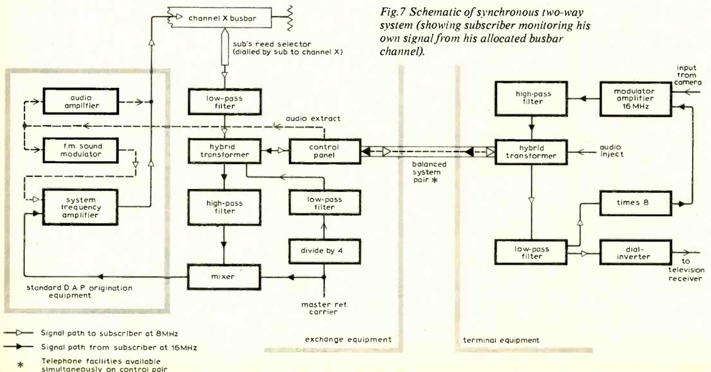
Fig. 7 Schematic of synchronous two-way system (showing subscriber monitoring his own signal from his allocated busbar channel).
