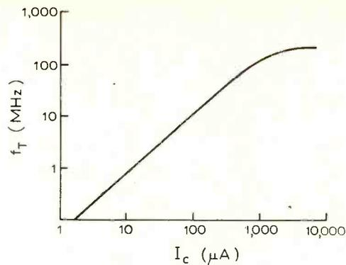
Fig. 4. At high frequencies the gain-bandwidth product of a transistor is an almost linear function of quiescent current.
