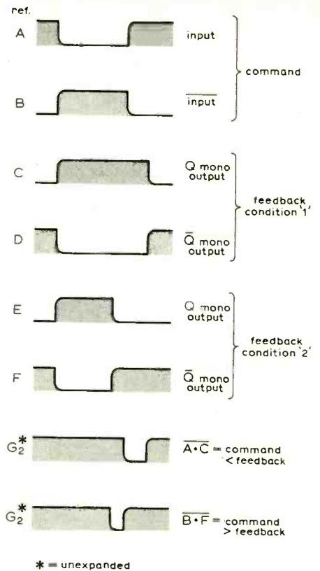
Fig. 7. Pulse-width comparator logic.
