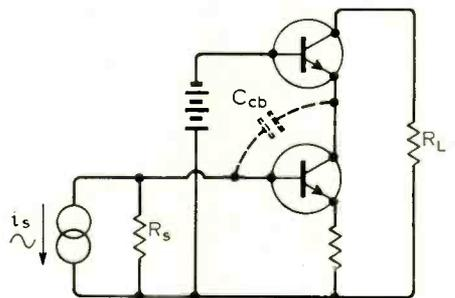
Fig. 33. The cascode circuit.
