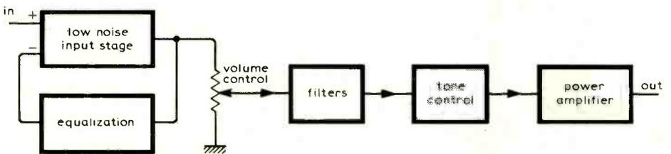
Fig. 34. Block diagram of a typical audio amplifier.
