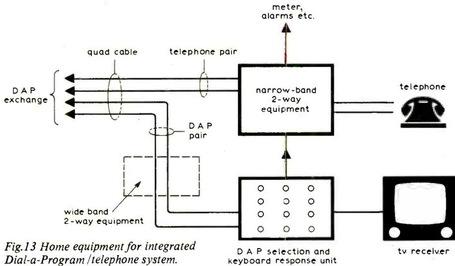
Fig.13 Home equipment for integrated Dial-a-Program/telephone system.
