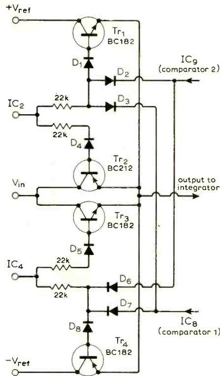
Fig. 6. The complete analogue switching circuit.
