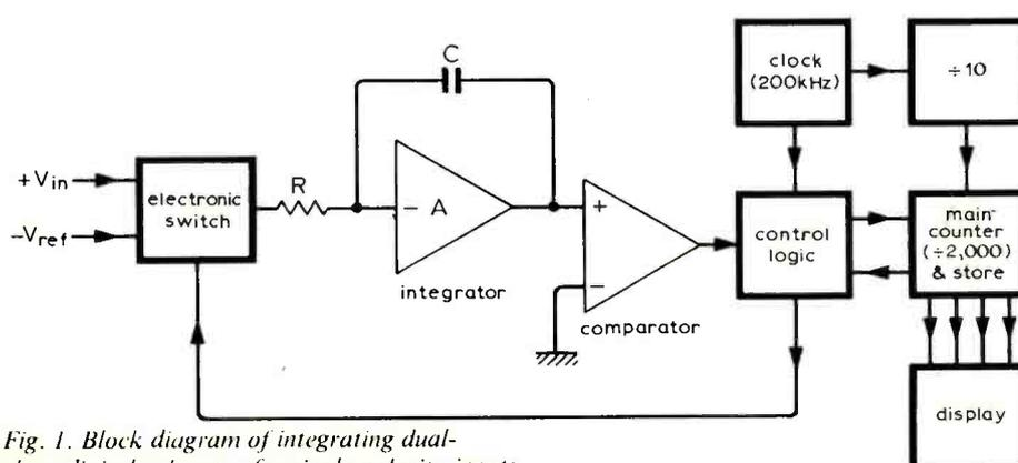
Fig. 1. Block diagram of integrating dual-slope digital voltmeter for single-polarity inputs.
