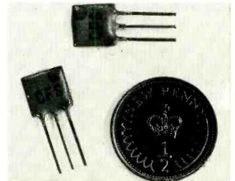
The performance parameters are closely specified, and include a centre frequency shift within ±150 p.p.m. per °C in the temperature range -10 to +60°C.
