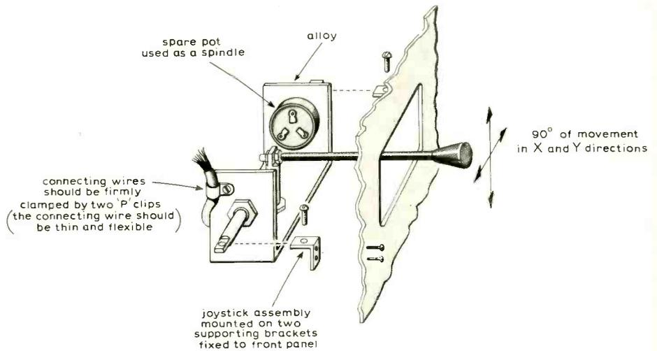
Fig. 32. Mechanical assembly of the joystick control.
