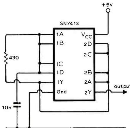
Fig. 7. Clock pulse generator, using a dual 4-input Schmitt NAND.
