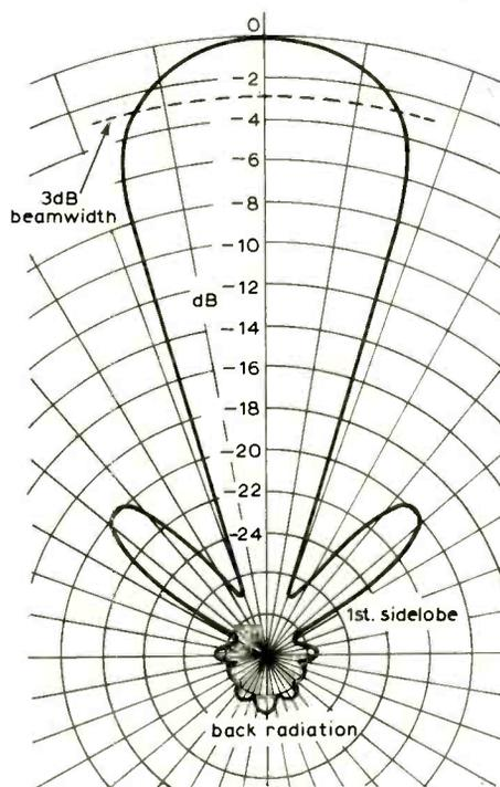
Fig. 1. General polar diagram showing the directive type of main beam that can be obtained in the microwave region. Parameters such as gain, beamwidth and side-lobe level are within the control of the designer.
