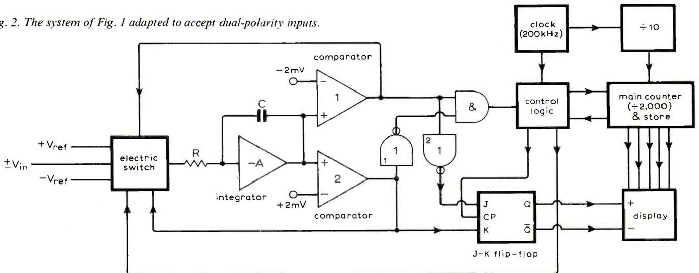
of an input voltage, and 2mV represents a resolution of less than the least significant digit displayed.
