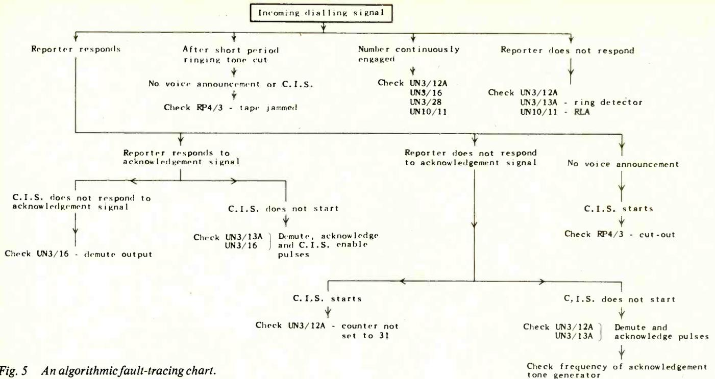
Fig. 5 An algorithmic fault-tracing chart.
