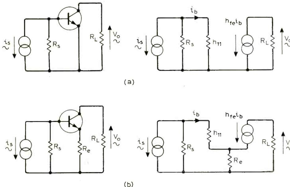
Fig. 32. Common emitter amplifier drawn (a) without feedback and (b) with feedback together with their small signal equivalents.
