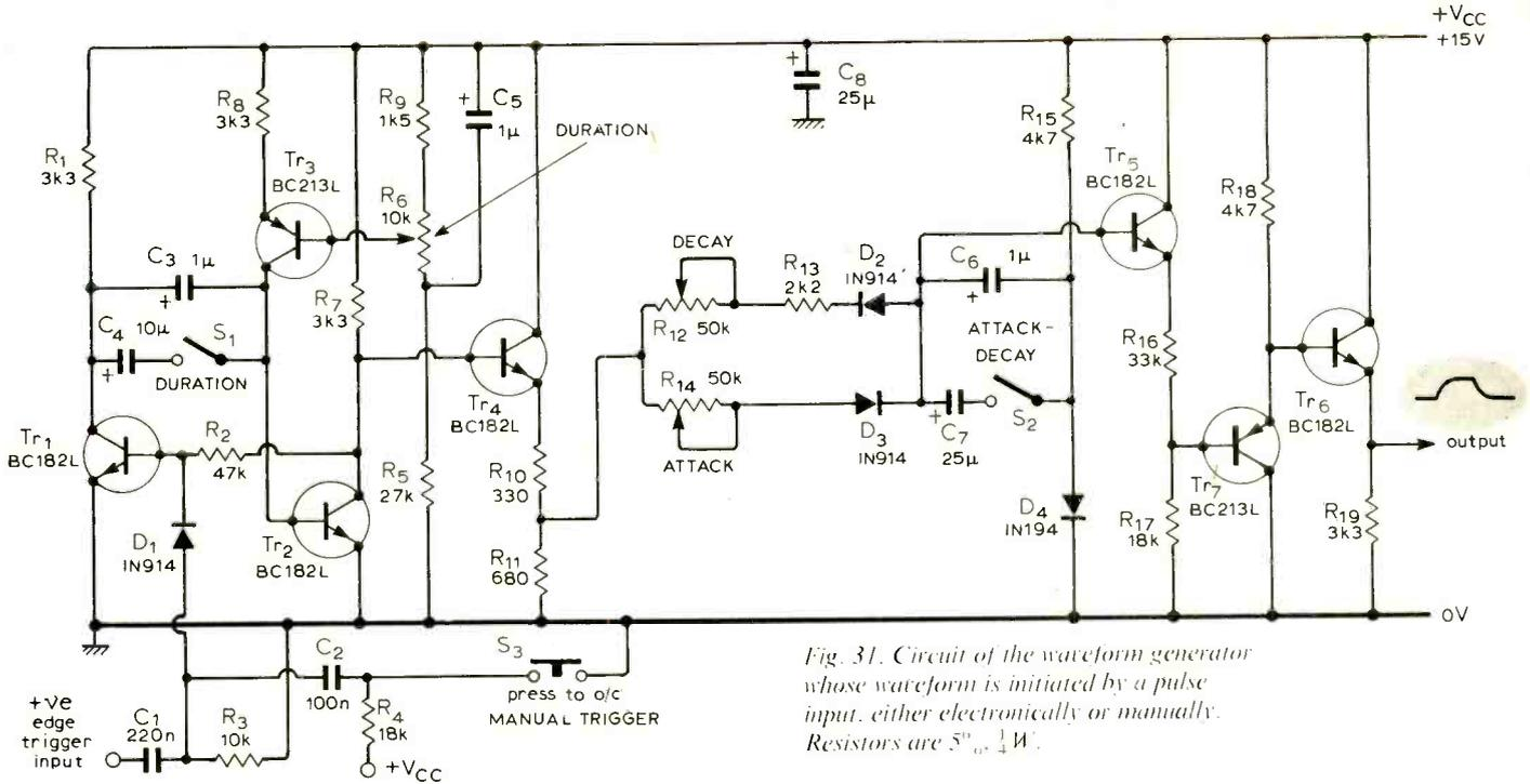
Fig. 31. Circuit of the waveform generator whose waveform is initiated by a pulse input, either electronically or manually. Resistors are 5%, 1/4 W.
