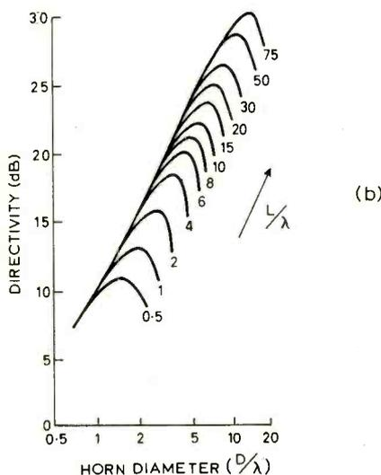
Fig. 4. In similar fashion to the sectoral horns, the pyramidal and conical versions also have optimum aperture dimensions for a fixed length. Directivities are plotted for (a) pyramidal horn and (b) conical horn.
