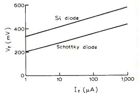
Fig. 2. The Schottky-barrier diode has a p.d. appreciably lower than that of a silicon diode.
