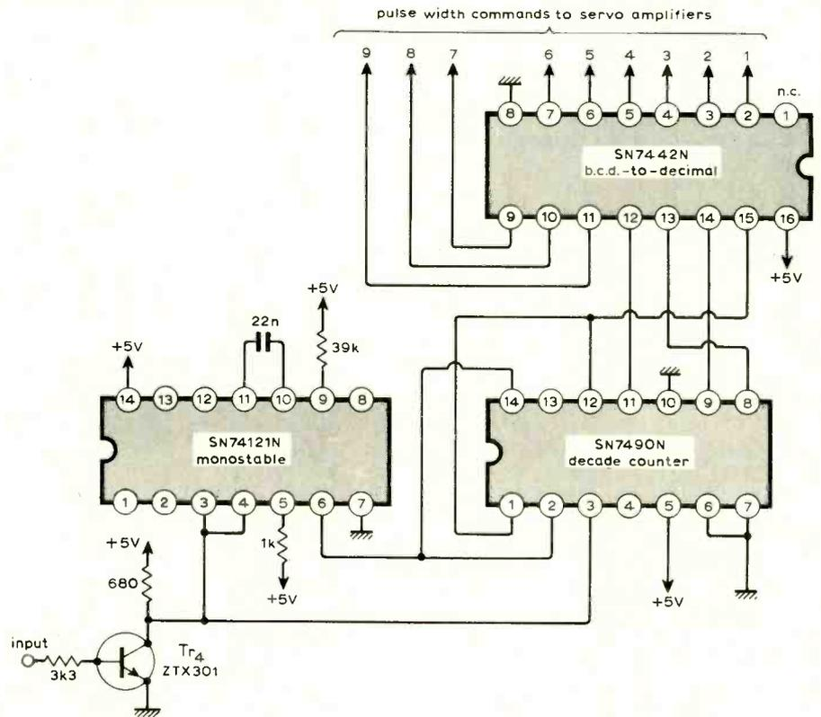
Fig. 4. Sync detector operation.
