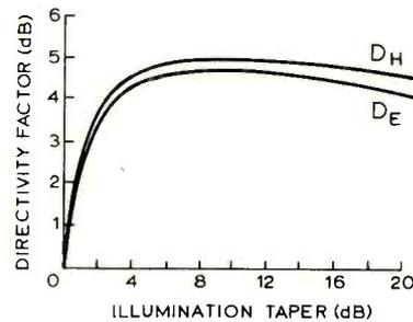
Fig. 8. Directivity of the complete parabolic aerial can be estimated with relation to the feed parameters. Plotted here are E- and H-plane directivity factors for a pyramidal horn.
