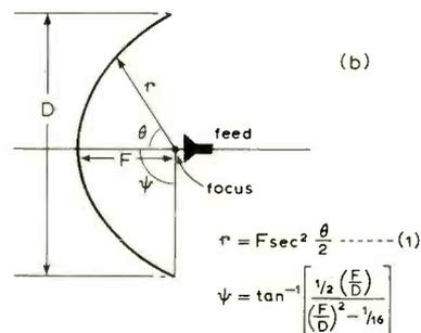
Fig. 5. Paraboloid reflector can produce high directivity and a narrow, pencil beam and allows side-lobe level control by proper design of the feed. Because all path-lengths from the feed to the far field are equal, the paraboloid converts the initially spherical wavefront into a plane-wavefront, collimated beam.
