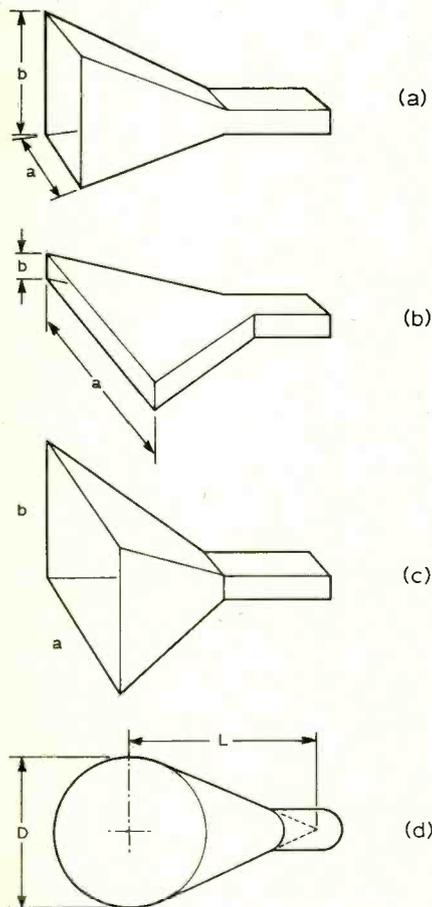
Fig. 2. Main types of waveguide horn formed by flaring the waveguide walls in a controlled fashion (a) E-plane sectoral horn, (b) H-plane sectoral horn, (c) pyramidal horn, (d) conical horn.
