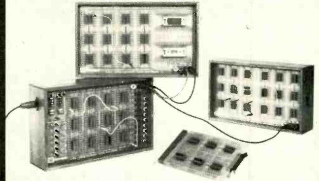
Limrose's new family of low-cost universal mounting boards, plug-in cards and breadboarding systems is useful for development work, device testing and circuit evaluation.
