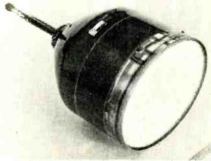
from single transients and recurrent waveforms to half-tone pictures. Designed primarily for use in air traffic control radars, it is equally useful for medical, tabular display or other applications involving viewing under high ambient light conditions.
