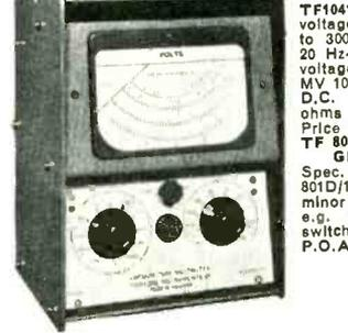
**TF1044 VTMV A.C. voltage range 300 MV to 300V in 7 ranges, 20 Hz-1500 MHz. D.C. voltage ranges 300 MV 1000V in 8 ranges. D.C. resistance 50 ohms to 500 ohms. Price £62.50.**
