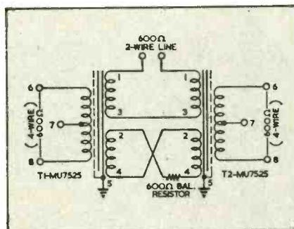
*So accurate is the balancing of the windings on some of these transformers that, when used as pairs in a hybrid circuit (as illustrated) we can guarantee a rejection of better than  $-55$ dB over the frequency range 50Hz to 10kHz and normal rejection of up to  $-75$ dB may be expected.*
