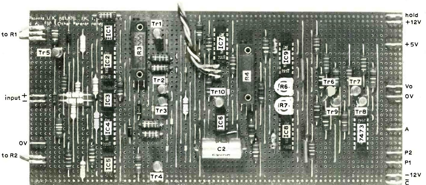
Fig. 13. Layout of analogue circuit.
