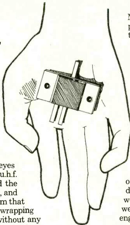
Mullard u.h.f. modules are completely encapsulated and the question of tuning or trimming simply does not arise.
