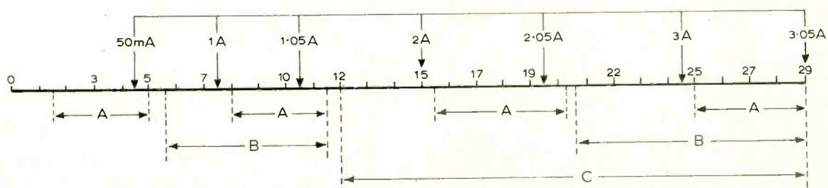
Fig. 2. Switching points recognized by the sensors of the whistle (A), the lights (B) and the locomotive motor (C).
