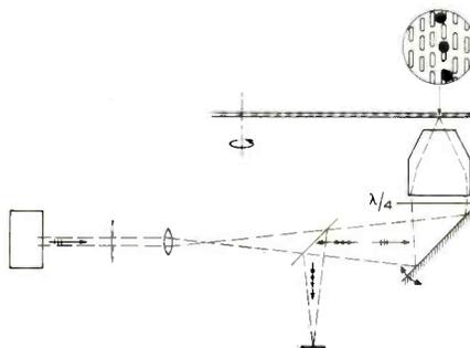
Fig.3. In the VLP optical system, electromagnetic transducers are attached to the objective lens for focusing and to the mirror for centring and tracking. Laser beam is split by a diffraction grating to provide the two auxiliary spots before and after the main spot. Detectors either side of the main beam sense the reflected auxiliary beams to provide control signals for mirror movement.
