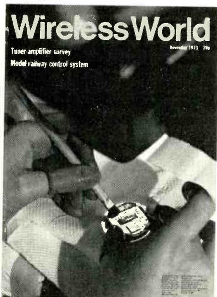
This month's cover picture shows the sealing in of the "works" of a digital wristwatch, including a Monsanto I.e.d. display seen as the dark rectangle in the middle.
