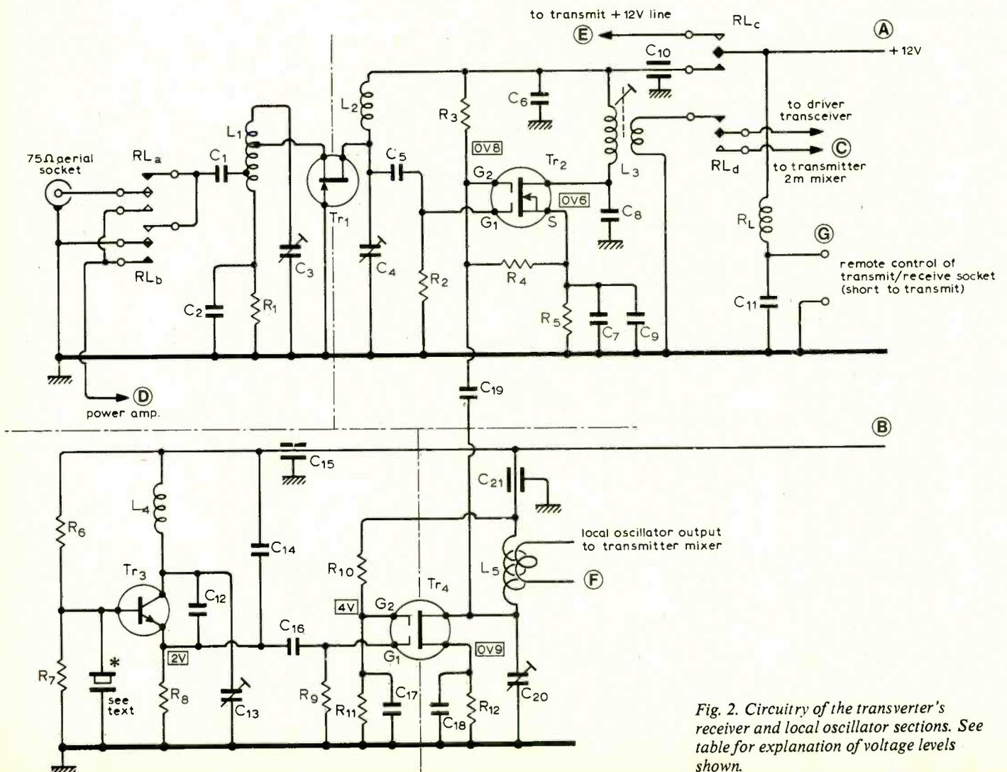
Fig. 2. Circuitry of the transverter's receiver and local oscillator sections. See table for explanation of voltage levels shown.
