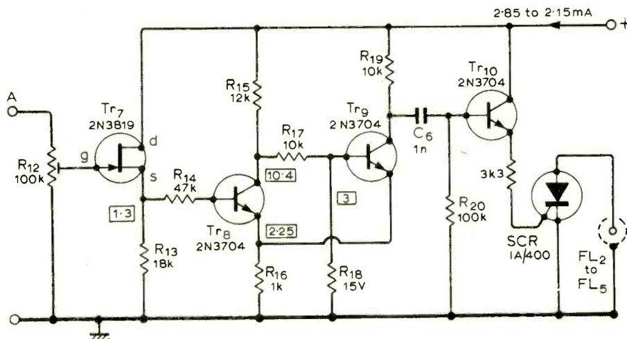
Fig. 3. Four voltage-operated switches, all identical to this circuit, are set to trip at different points of the ramp waveform.
