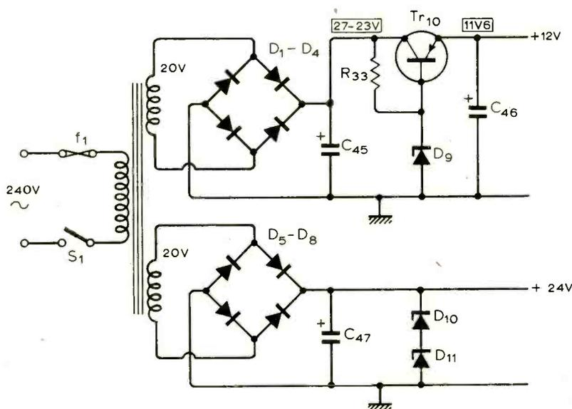
Fig. 4. Power supply circuit. See components list for transformer details.
