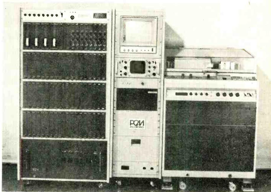
To achieve the necessary bandwidth for p.c.m. this recorder uses a conventional 525-line video tape recorder. Editing is made easier by the provision of a 30-Hz frame synchronizing signal on the control (audio) track.
