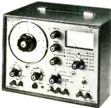
**DM344A Distortion Factor Meter.** Designed to make accurate and rapid measurements of total harmonic distortion generated within high quality audio amplifiers, recording and transmission equipment. Selling Price: Chassis - £132.50.c/w. Case - £140.00 + VAT.
