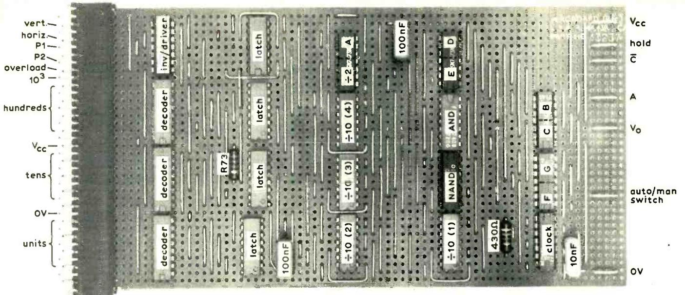
Fig. 14. Control circuitry and display logic
