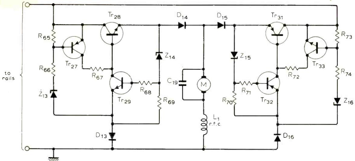
Fig. 6. Motor drive unit.
