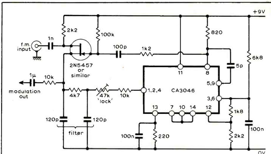
Fig. 10. Phase locked loop configuration built around the v.c.o., suitable for use as an f.m. demodulator. The f.e.t. is used as a synchronous chopper type phase sensitive detector.
