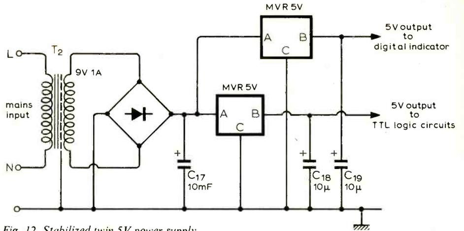
Fig. 12. Stabilized twin 5V power supply.
