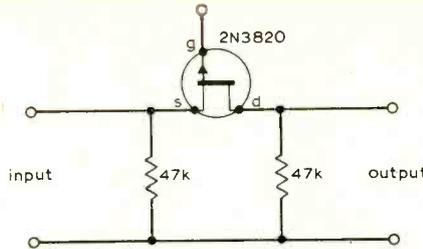
Fig.3. Elements of the f.e.t. switch used to control the receiver output.
