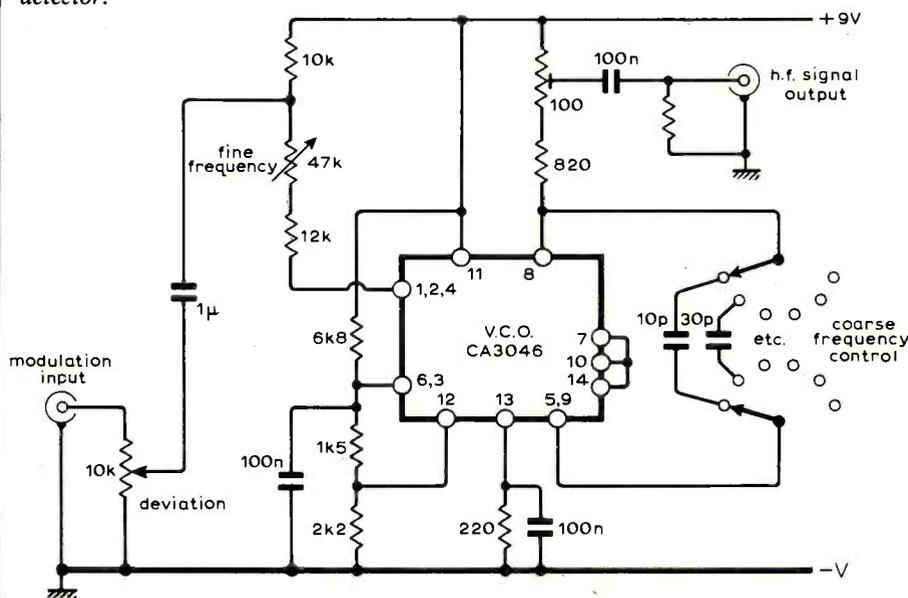
Fig. 11. Using the v.c.o. in an arrangement for a low distortion f.m. signal generator, or as a "wobbulator".
