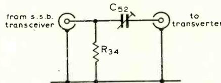
Fig. 7. Dummy load attenuator circuit. Internal layout of the transverter circuitry.
