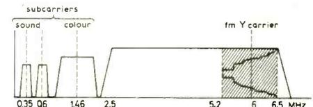
Fig. 1. If the normal PAL video signal modulated the VLP disc carrier directly, colour information encoded at 4.43MHz would be lost as video bandwidth is about 3MHz. Therefore the colour information is transposed down to 1.46MHz, while luminance information frequency modulates the 6-MHz carrier, only the first lower sideband being recorded.
