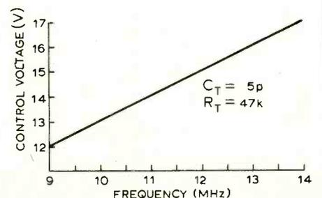
The performance of this circuit for a timing capacitor of 5pF, and with the other values as indicated, is shown in Fig. 9. The linearity of this arrangement is as good as that of the circuit in Fig. 4, but the long term stability of the Fig. 4 circuit is slightly better. Several CA3046 units were tried and gave identical free running operating frequencies.
