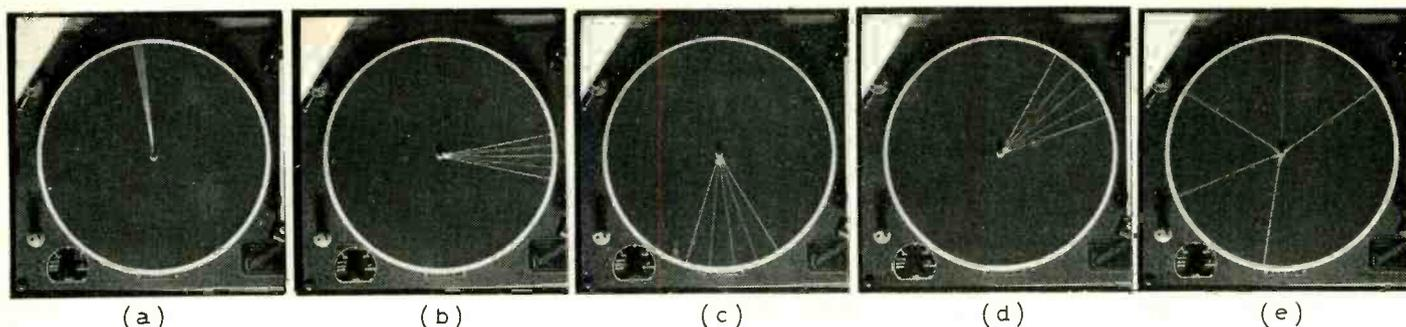
Fig. 6. To check linearity of 0.1- $\mu$ F and 1.0- $\mu$ F ranges the five flash units were used to photograph a string tied between spindle and rim of a 78 rev/min turntable. For the 0.1- $\mu$ F range,  $R_{10}$  was set at min., mid. and max. settings (a, b and c) and at min. and mid. settings for the 1.0- $\mu$ F range (d and e).
