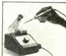
ETC/1 Electronically Temperature Controlled System
