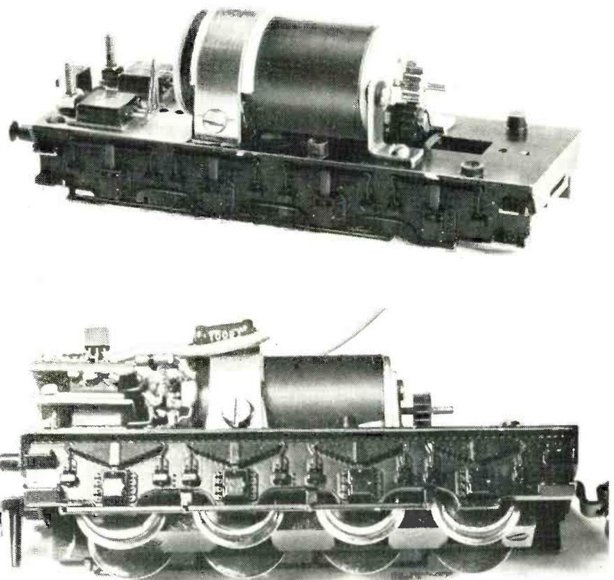
Fig. 7. Motor and control mounted in the tender.
