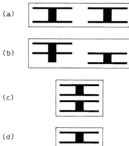
Fig.4 Four reel arrangements now standardized by the EIAJ for domestic video cassette/cartridge systems.
