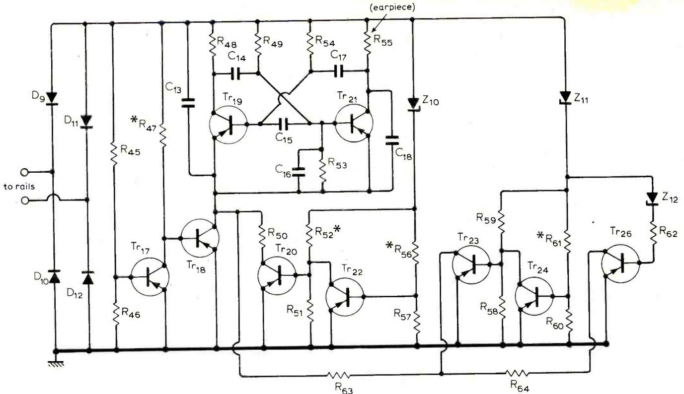
Fig. 5. Whistle level sensing and regulation circuit. Components marked with an asterisk may need adjustment to achieve the correct switching levels.
