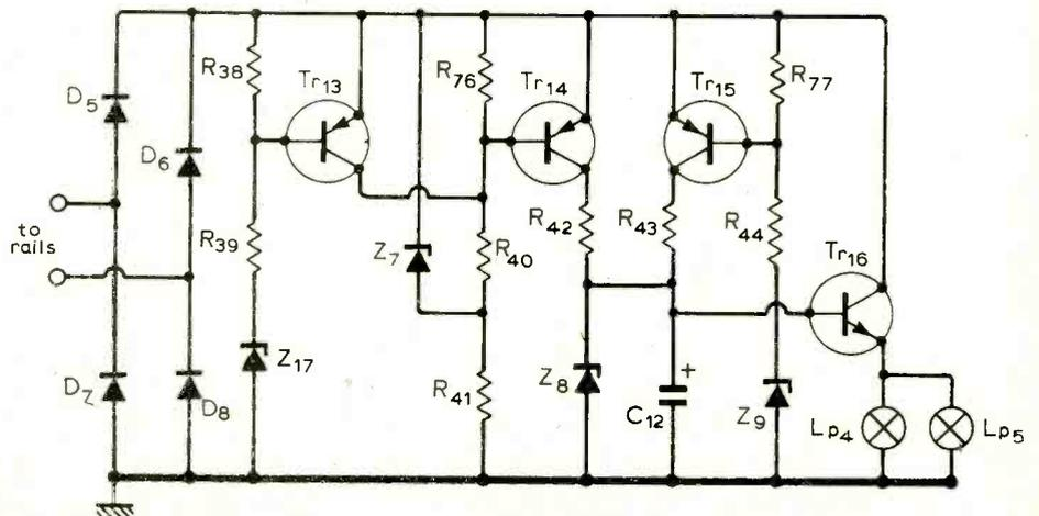
Fig. 4. Circuit diagram of the coach lights controller.
