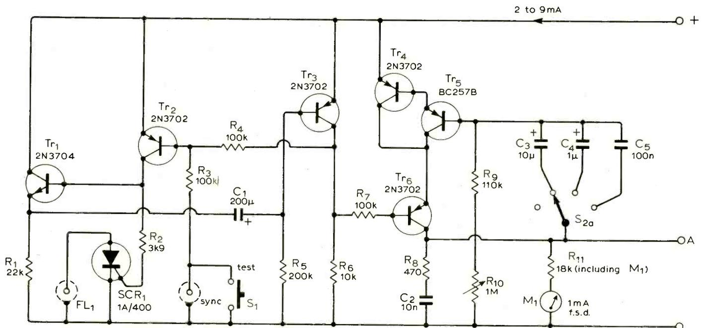
Fig. 1. Camera shutter contacts trigger the monostable circuit which turns on the thyristor to provide the first flash trigger. If  $C_1$  were directly connected to  $Tr_2$  collector, rise time would be too great. Timing circuit provides ramp output at A.
