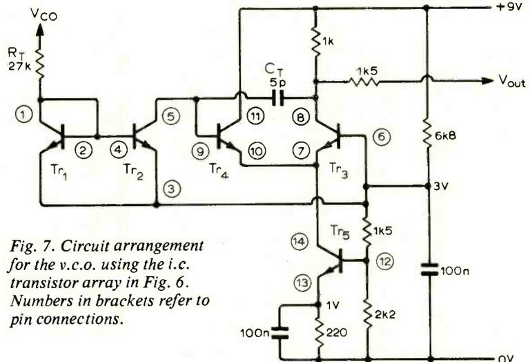
Fig. 7. Circuit arrangement for the v.c.o. using the i.c. transistor array in Fig. 6. Numbers in brackets refer to pin connections.
