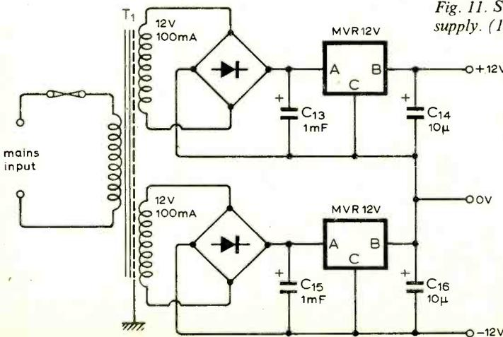
Fig. 11. Stabilized  $\pm 12V$  power supply. (1mF = 1000 $\mu$ F).
