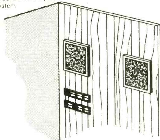
Two Sinclair Q.16 loudspeakers suitably positioned together with Project 80 could be mounted on to a false wall.
