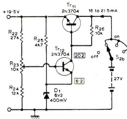
Fig. 4. Stable battery supply circuit.
