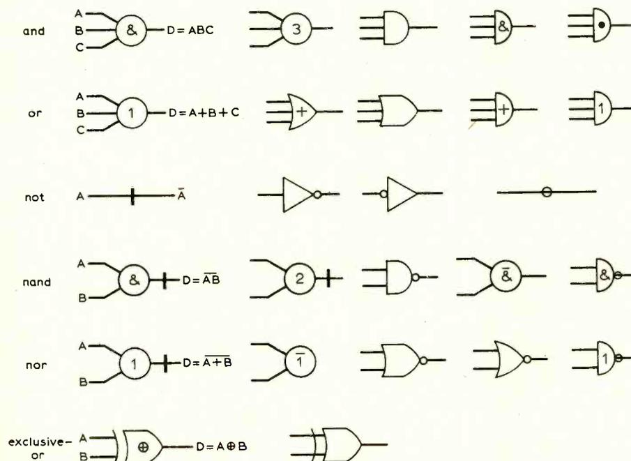
Fig. 3. Some of the symbols used for logic gates.
