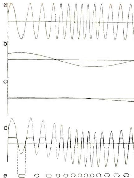
Fig.2. In coding the VLP, symmetrically limiting signals for luminance (a), colour (b) and sound (c), and combining in the ratios 20:4:1, produces a train of rectangular pulses whose frequency represents brightness and whose duty cycle carries colour and sound information.
