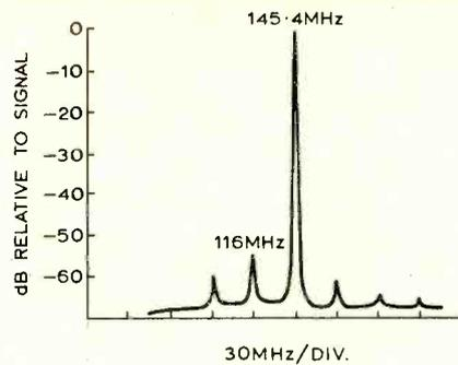
Fig. 5. Signal purity of the transverter.
