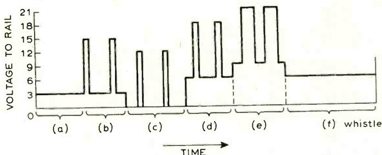
Fig. 1. A complete train movement, showing all functions operating.
