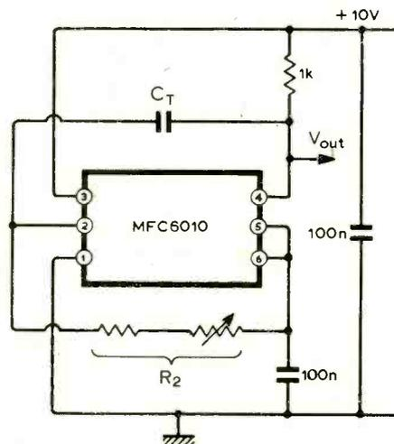
Fig. 2. Square-wave oscillator with a high long term stability. Operation is up to at least 20MHz.
