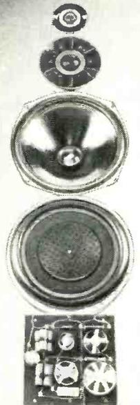
1.) Celestion's new super tweeter. 2.) New design 'pressure' mid-range unit. 3.) Ultra Linear 12" Bass drive unit. 4.) A.B.R. ensures controlled bass down to 16Hz. 5.) Precision crossover for perfect system integration.
