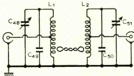
Fig. 6. High Q 28MHz filter whose use depends on the exciting transceiver used (see text).
