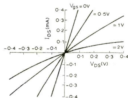
Fig.2. A sketch graph of the f.e.t.  $V_{DS} = I_{DS}$  characteristics.
