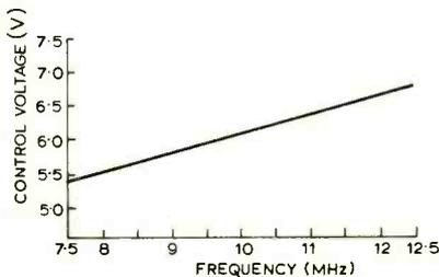
Fig. 5. Performance of the circuit shown in Fig. 4.
