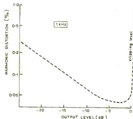
As well as featuring a flat amplitude response from d.c. to 20kHz, the p.c.m. technique shows excellent linearity of input-output level and a noise level that permits at least 75dB dynamic range.
