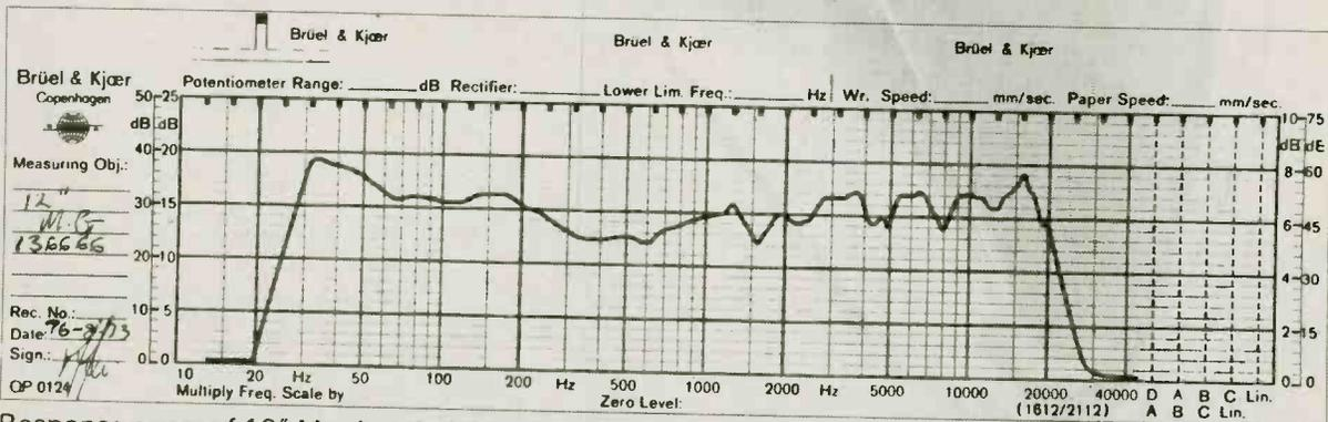
Response curve of 12" Monitor Gold mounted on Works test Enclosure
