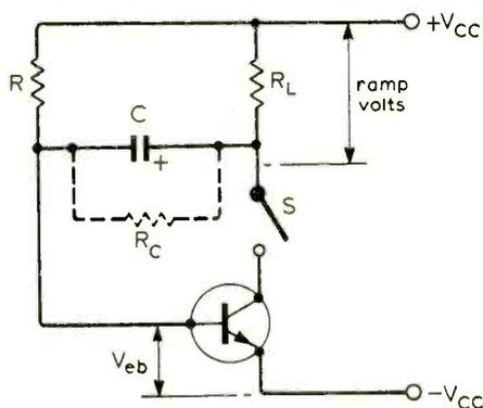
Fig. 2. Basis of the timing circuit is a Blumlein (Miller) integrator, the linear portion of the ramp being about CR seconds long.
