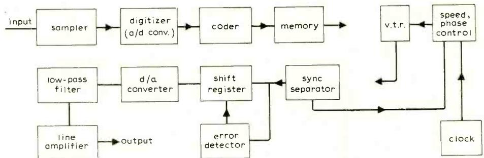
In this eight-channel p.c.m. system for making studio master recordings, fidelity — already improved over conventional tape recorders as illustrated in the graphs — can be further improved by duplicating channels where only two or four are required using digital error-correcting procedures.
