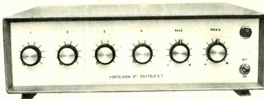
The mixer is arranged for 2-30/60 $\Omega$  balanced line microphones, 1-HiZ gram input and 1-auxiliary input followed by bass and treble controls. 100 volt balanced line output or 5/15 $\Omega$  and 100 volt line.
