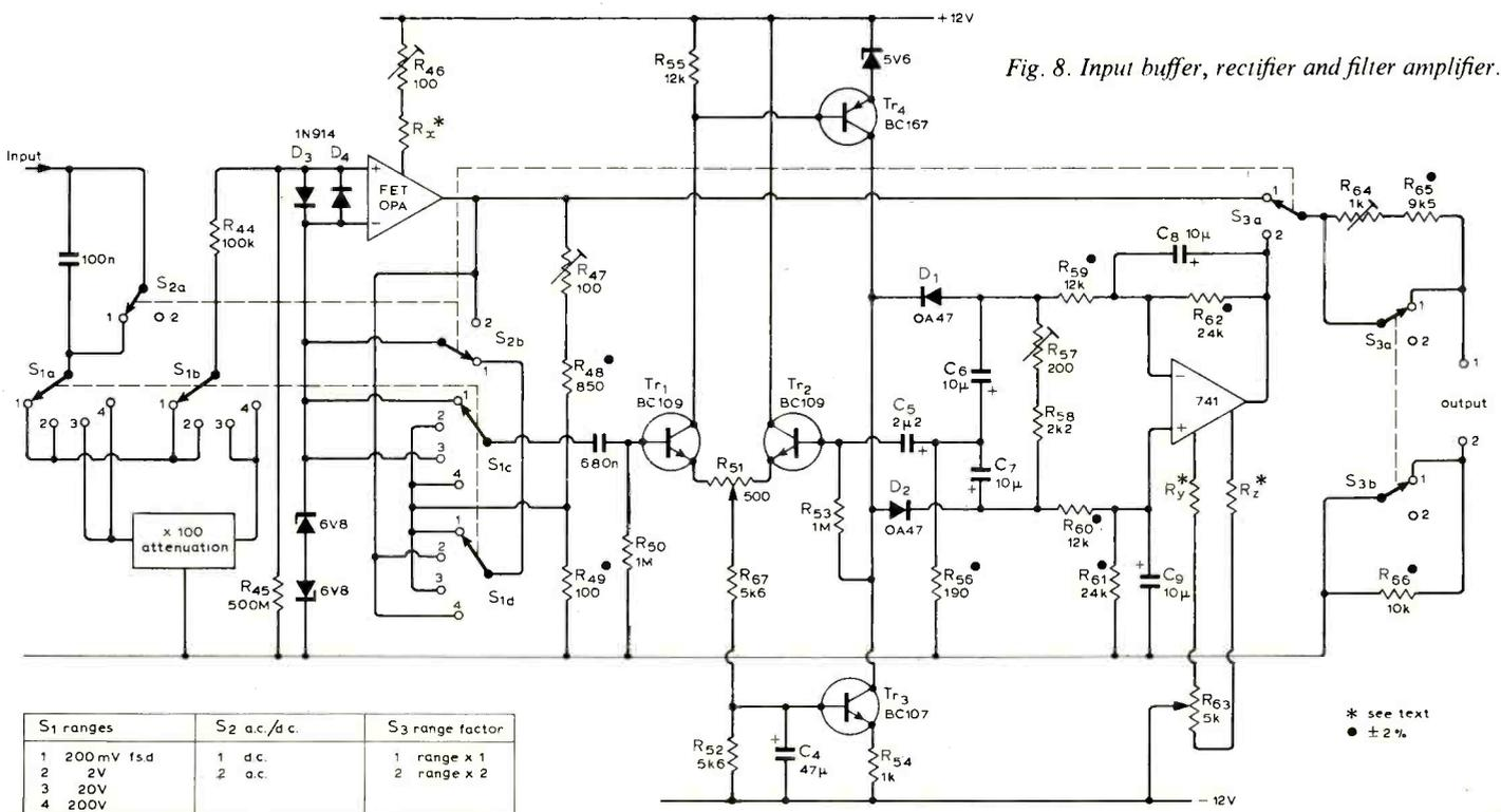
Fig. 8. Input buffer, rectifier and filter amplifier.
