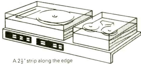
A 2 1/2" strip along the edge a shelf could be sufficient to contain a complete system
