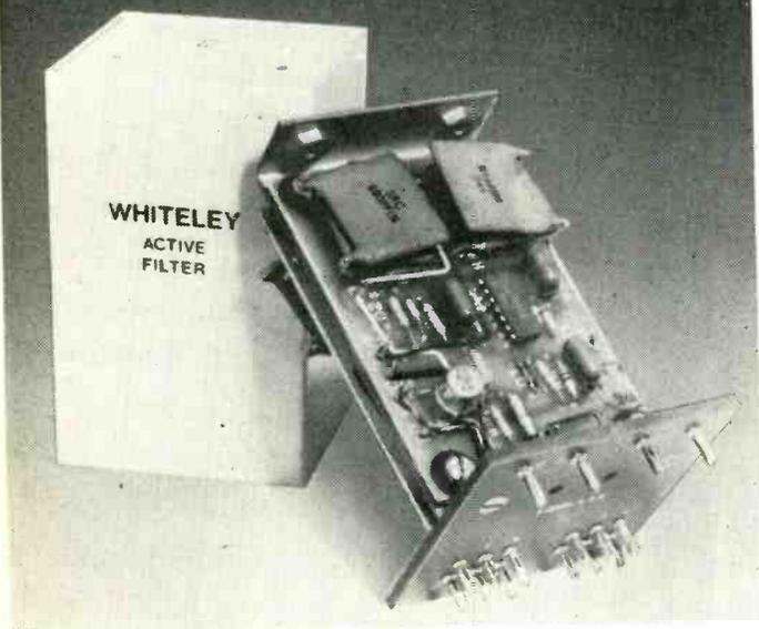
These active filters are designed to take over the functions of passive filter networks in audio telecommunications systems. They offer several advantages, in space-saving, economy and reliability.
