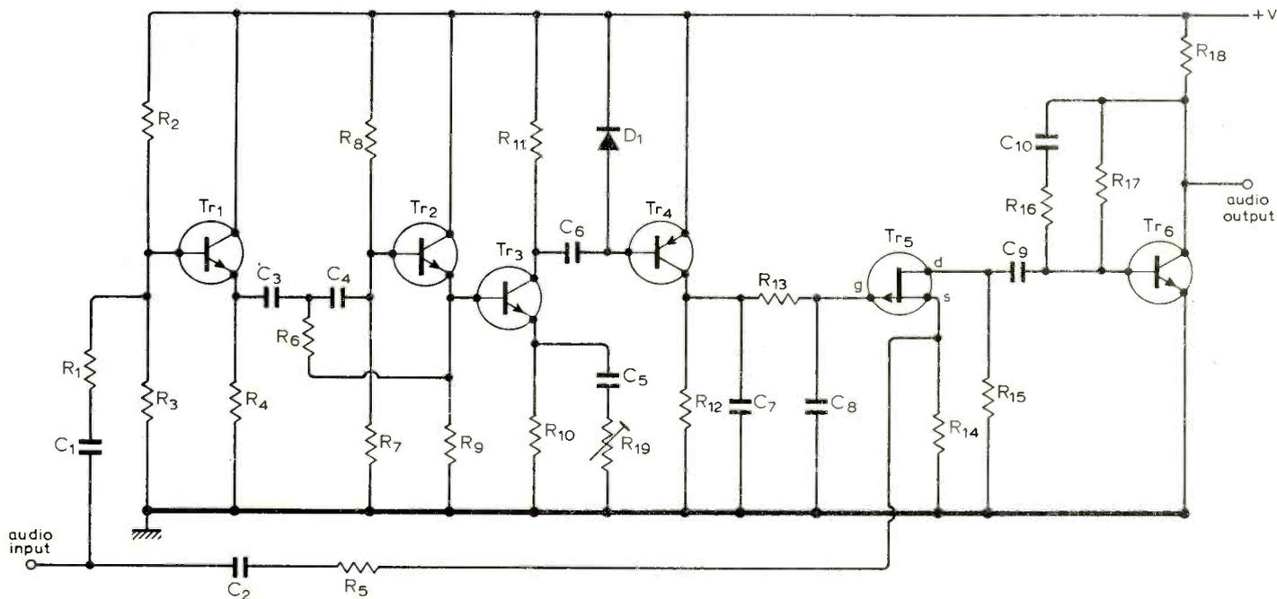
Fig. 1. Complete circuit of automatic noise limiter.
