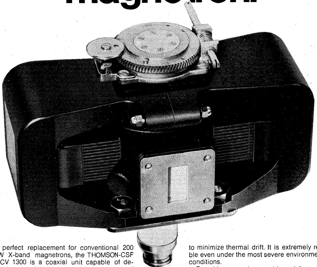
A perfect replacement for conventional 200 kW X-band magnetrons, the THOMSON-CSF MCV 1300 is a coaxial unit capable of delivering a minimum peak power output of 200 kW over the frequency range of 8.5 to 9.6 GHz.
