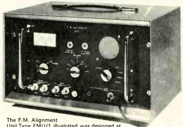
The F.M. Alignment Unit Type FMU/1 illustrated was designed at the Royal Radar Establishment, Malvern, to suit Ampex Recorders working on the IRIG intermediate band specification (using ES 100 Electronics) e.g. Model Numbers FR 1200, FR 1260, FR 1300, FR 1800L, FB 400, PR 500
