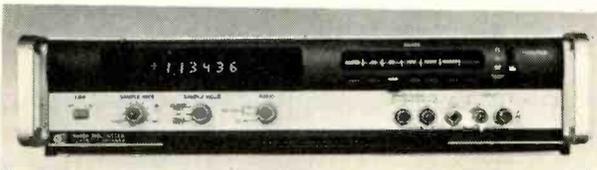
The DOM 100 ohms module provides for the measurement of resistance from 999mΩ to 1GΩ full-scale. The measuring circuit is a self-balancing bridge with a front-panel lamp to indicate when the bridge comes to balance. Remote sensing terminals are provided for lead resistance compensation. The resistance of inductive windings can be measured and the power applied to components being measured is less than 1mW.
