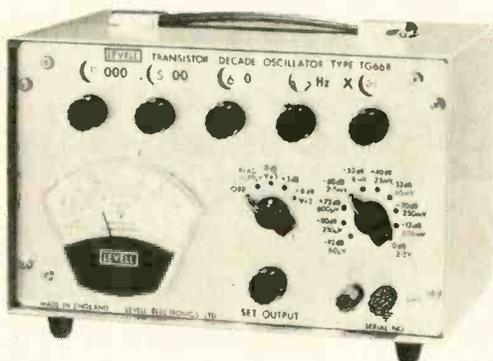
**FREQUENCY** 0.2Hz to 1.22MHz on four decade controls.
