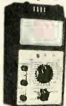
**U4341;** 27-range multimeter, with AC/DC voltage and current coverage plus transistor tester giving current gain measurements from 10 to 350. Sensitivity 16,700/3,300 o.p.v. Accuracy 2.5/4% £10.50
