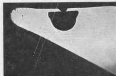
Sectioned iron-plated bit, after 40,000 simulated operations using 60/40 Solder.
