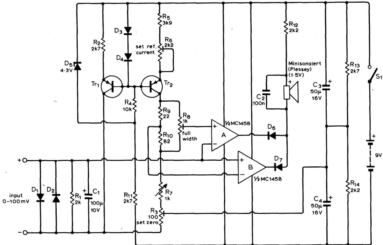
Circuit of multimeter for blind students (G. P. Roberts).  $Tr_1$  and  $Tr_2$  are silicon p-n-p types, e.g. BC177, BC187.  $D_5$  is a 400mW, 4.3V zener diode, e.g. BZX79/C4V3, and other diodes are small signal silicon types, e.g. BA100, IN914A.
