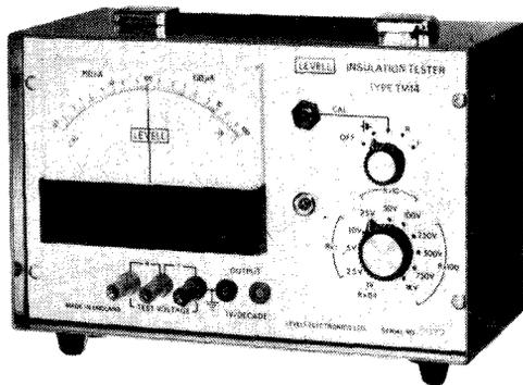
A logarithmic scale covering 6 decades is used to display either insulation resistance or leakage current at a fixed stabilised test voltage. The current available is limited to a maximum value of 3mA for safety and capacitors are automatically discharged when the instrument is switched off or to the CAL condition. The instrument operates from a 9V internal battery.
