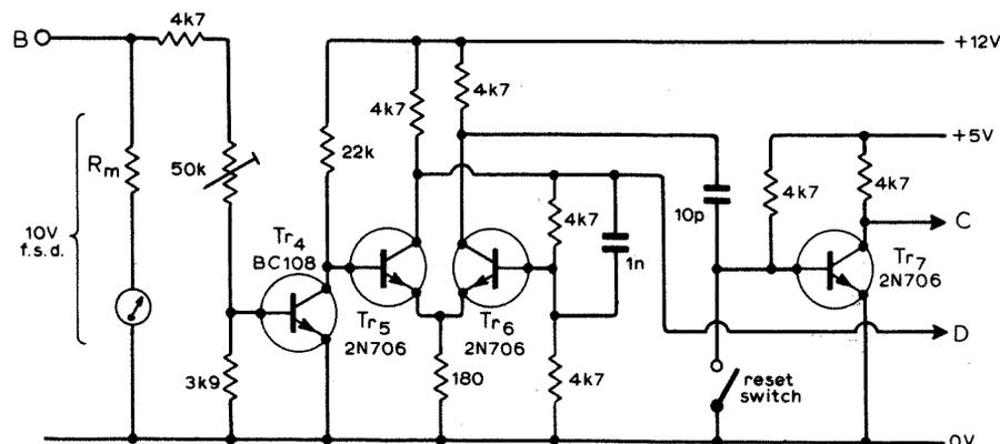
Fig. 3. Meter and trigger circuit. Meter can be 1mA or less.
