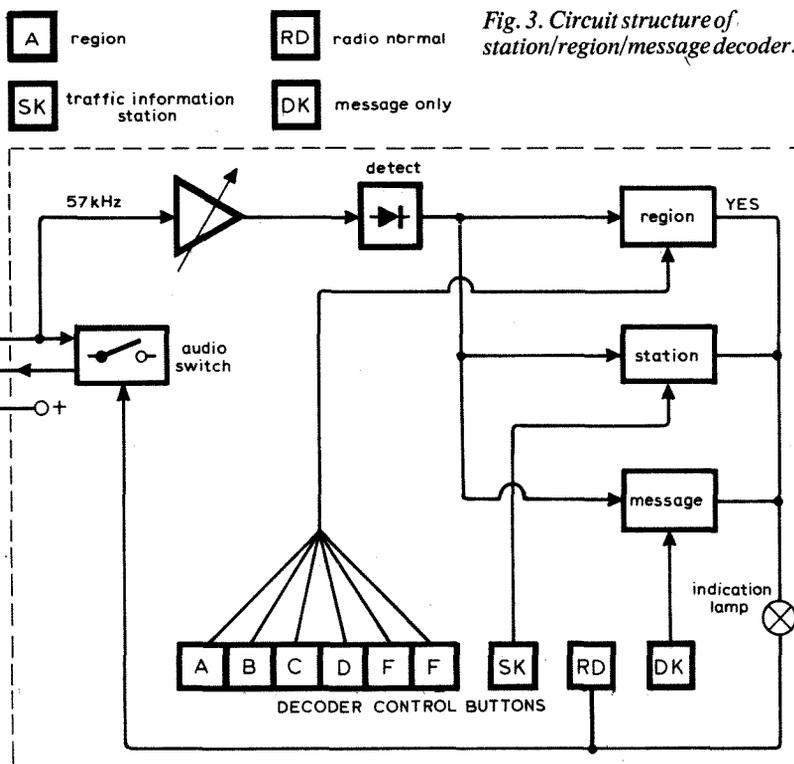
Fig. 3. Circuit structure of station/region/message decoder.
