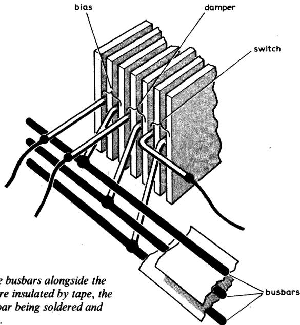
Fig. 19. Three busbars alongside the keyswitches are insulated by tape, the "switch" busbar being soldered and insulated first.
