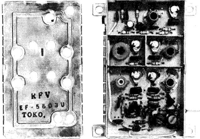
The model EF 5603U high performance FM Varicap Tuner, incorporates back-to-back diodes with a five gang triple interstage coupling.
