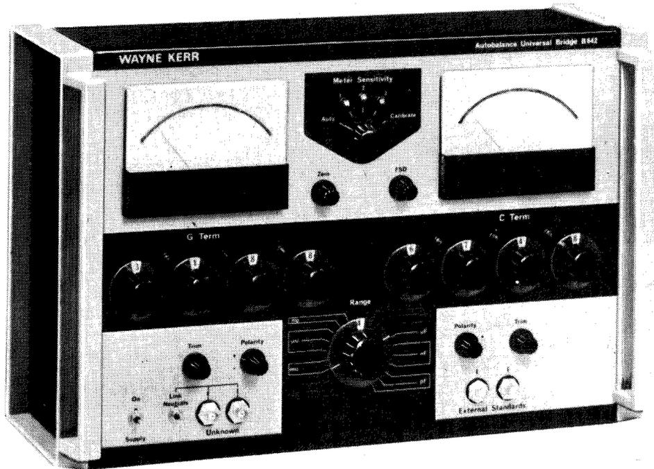
Meets modern requirements. Is accurate to 0.1%. Is self-balancing. Has 2, 3 and 4-terminal connections. Continuous readout of real and quadrature terms. Overall range 10 micro-ohms to 100 gigohms, 0.001pF to 10 farads, 1 nanohenry to 10 megahenrys and 10 picomhos to 100 kilomhos. Built-in source/detector (1592Hz). Connectors for 200Hz—20kHz manual operation. Comparator facilities. Analog outputs. Adjustable sensitivity. Ask for B642 Data Sheet.
