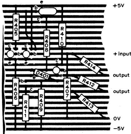
Fig. 18. Layout of one divider and key circuit. Outputs from divider feed four similar (except for  $D_1$  position) key circuits alongside that shown. (Thirteenth divider feeds only one key circuit). Two large boards bear 61 key circuits and 13 dividers. In the five key circuits related to any one divider, uppermost wire of  $D_1$  connects to different i.c. terminals or tracks (see text). A minor modification to this board is suggested in part 3.
