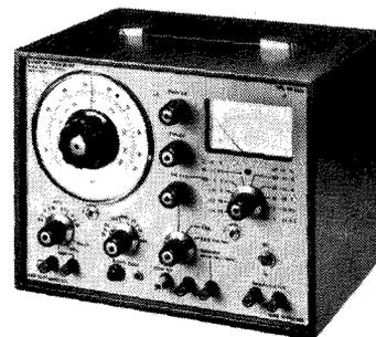
**DM344A Distortion Factor Meter.** Designed to make accurate and rapid measurements of total harmonic distortion generated within high quality audio amplifiers, recording and transmission equipment. **Selling Price: Chassis — £132.50.c/w. Case — £140.00 + VAT.**
