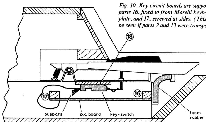
Fig. 10. Key circuit boards are supported by parts 16, fixed to front Morelli keyboard plate, and 17, screwed at sides. (This would be seen if parts 2 and 13 were transparent.)
