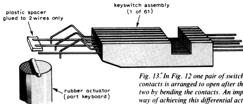
Fig. 13. In Fig. 12 one pair of switch contacts is arranged to open after the other two by bending the contacts. An improved way of achieving this differential action is to glue pads to contacts as shown.
