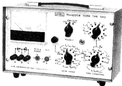
Tests bipolar transistors, diodes and zener diodes. Measures leakage down to 0.5 nA at 2V to 150V. Current gains are checked from 1 $\mu$ A to 100mA. Breakdown voltages up to 100V are measured at 10 $\mu$ A, 100 $\mu$ A and 1mA. Collector to emitter saturation voltage is measured at 1mA, 10mA, 30mA and 100mA for  $I_C/I_B$  ratios of 10, 20, 30. The instrument is powered by a 9V battery.
