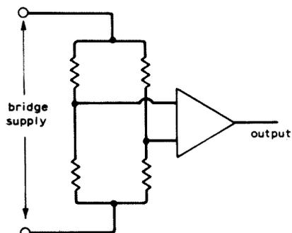
Fig. 2. Bridge circuit for including a sensing resistor.
