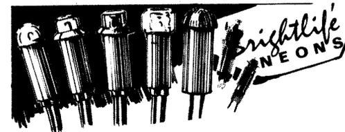
Brightlife neons, illustrated, are PC/A or C, PC/F, PC/G or I, PP/A or B. Q & S are brighter and give an average of 25,000 hrs life. The 0.5" dia. are red or white, the 0.375" are red, amber or white; these have three cap shapes, and all may be supplied for 115, 240V or the PP neons in 110, 240 and 440V, with 6" or 30" leads.
