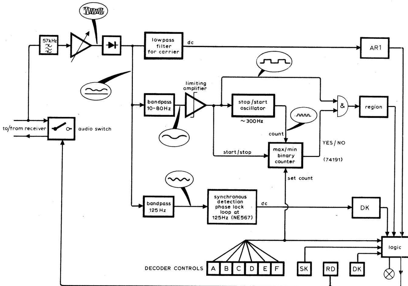
Fig. 4. Functional organization of the decoder circuits.
