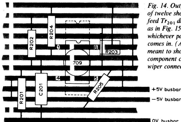
Fig. 14. Output from the oscillators (one of twelve shown) is taken from  $R_{205}$  to feed  $Tr_{201}$  drivers, which can be arranged as in Fig. 15. Board wiring is the same whichever package the 709 or 741 i.c. comes in. (Arrangement of  $R_{203}$  is meant to show the outer leads of the component connected together, with the wiper connected to track 5.)
