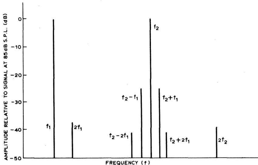
Fig. 1. Distortion spectrum of a 7in loudspeaker unit.
