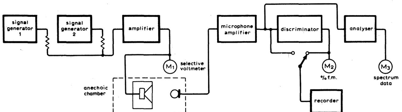
Fig. 2. Block diagram of the test equipment.
