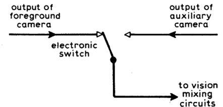
Fig. 1. Basic requirements for an overlay system.
