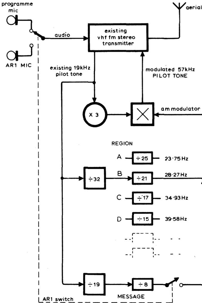
Fig. 2. Traffic information station transmitter showing additional circuits.
