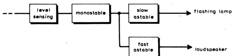
Fig. 3. Arrangement for operating a lamp and/or loudspeaker.
