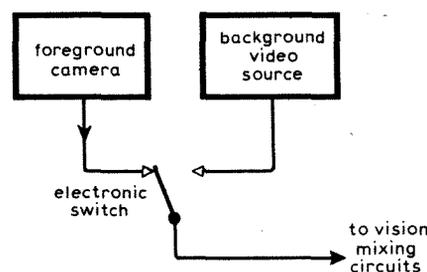
Fig. 6. Signal paths for overlaying full-size picture in part of frame.
