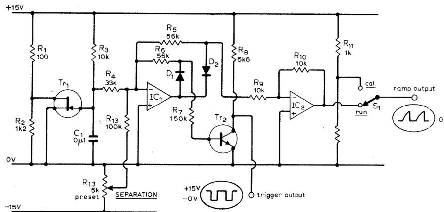
Fig. 7. Circuit diagram of the ramp generator.
