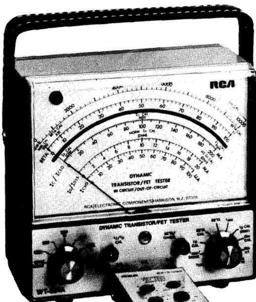
RCA introduces the WT-524A, a new "one for all" tester for solid-state devices. With it, you can measure AC beta—up to 5,000—of any bipolar transistor, and G<sub>m</sub>—up to 100,000 μmhos—of any field-effect transistor (FET). *And you'll do it with an accuracy of ±3%!* It also checks diodes, SCRs and triacs—and can do the job in-circuit or out.
