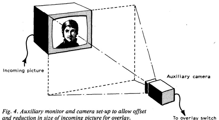
Fig. 4. Auxiliary monitor and camera set-up to allow offset and reduction in size of incoming picture for overlay.
