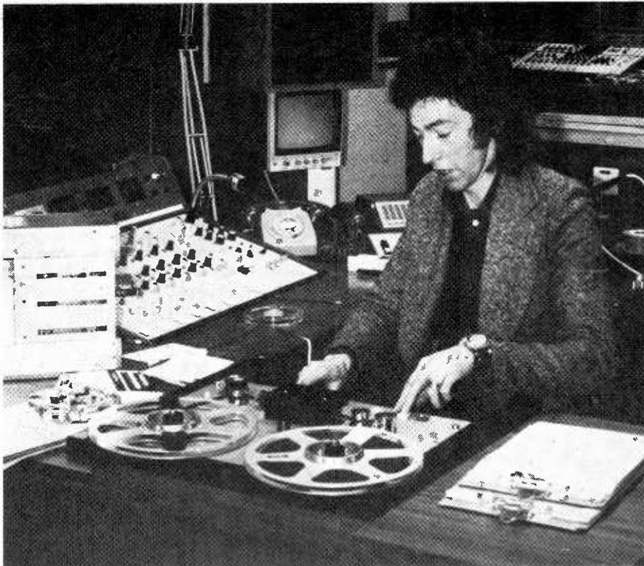
Some of the equipment installed in the Radio Clyde control room, Glasgow. The tape machine shown is supplied by Bias Electronics who can also provide a version which gives a delay of 8 seconds at  $7\frac{1}{2}$  i.p.s. This facility is useful for monitoring and editing live "phone-in" programmes as necessary.
