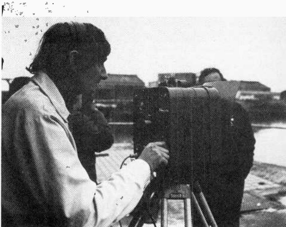
Engineer seen operating the remote unit of a Tellurometer microwave measuring system during winch-out of "Graythorp One", the world's largest oil rig, on the first stage of its 250-mile journey to BP's Forties Field.
