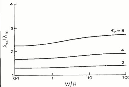
Fig. 6. Ratio of free space wavelength ( $\lambda_o$ ) to stripline wavelength ( $\lambda_m$ ).
