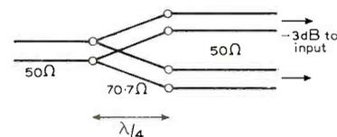
Fig. 3. Simple means of forming a power splitter.
