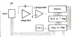
This state-of-the-art MOS LSI chip contains all the logic necessary for a 3 1/2 decade, dual slope integrating, automatic polarity detecting DVM. Supplied with free data and circuit booklet.
