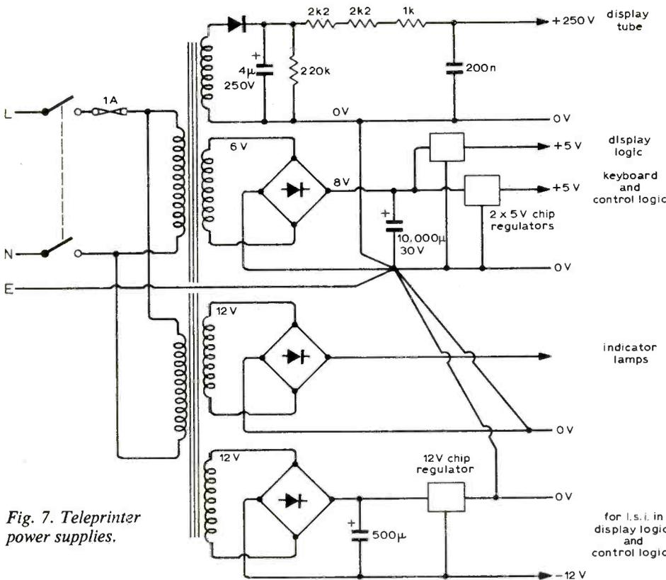
Fig. 7. Teleprinter power supplies.
