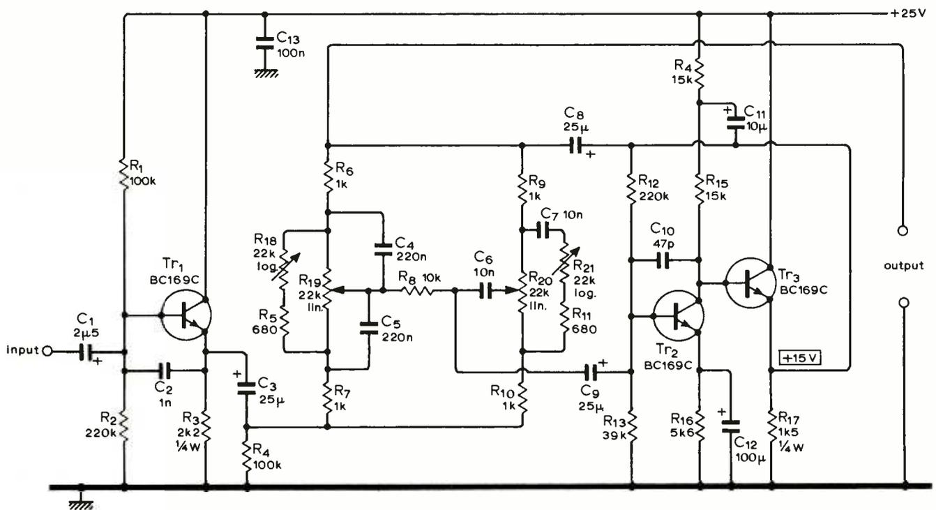
Fig. 5. Complete circuit. Resistors can be  $\frac{1}{8}$  watt unless shown otherwise.
