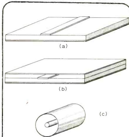
Fig. 1. Transmission line methods of construction (a) stripline, (b) triplate, (c) coaxial.
