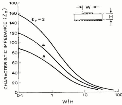
Fig. 5. Characteristic impedance curves of a stripline construction.
