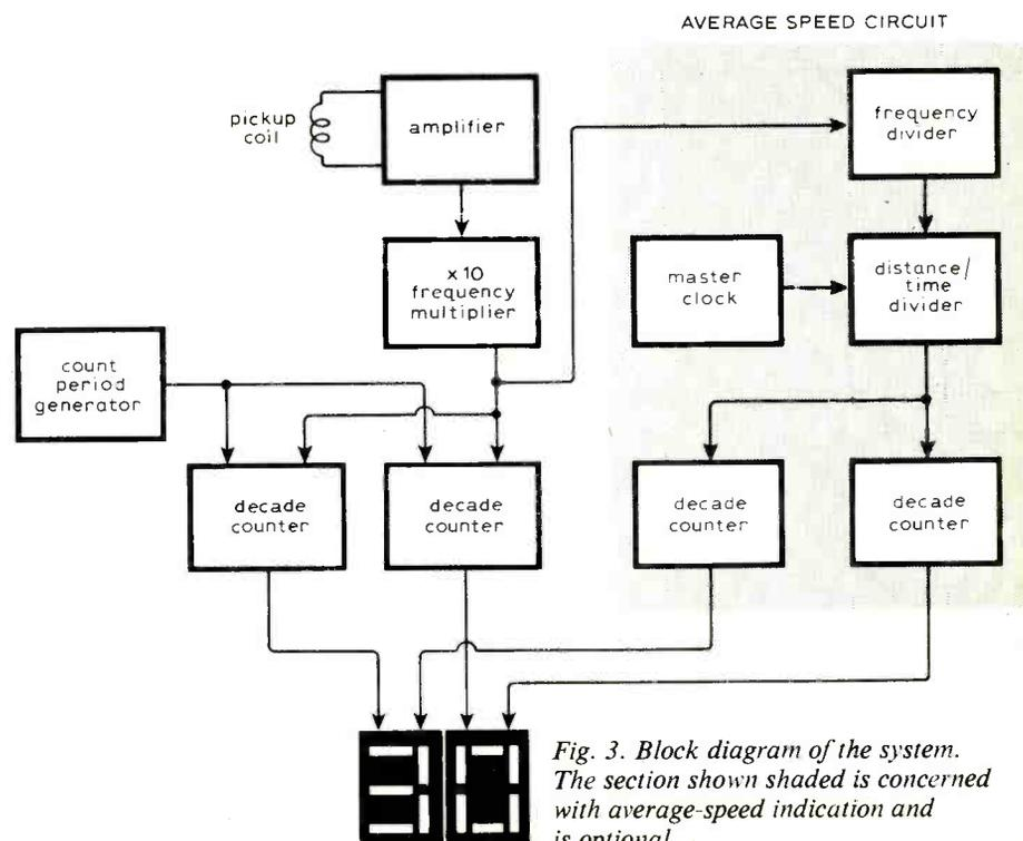
Fig. 3. Block diagram of the system. The section shown shaded is concerned with average-speed indication and is optional.
