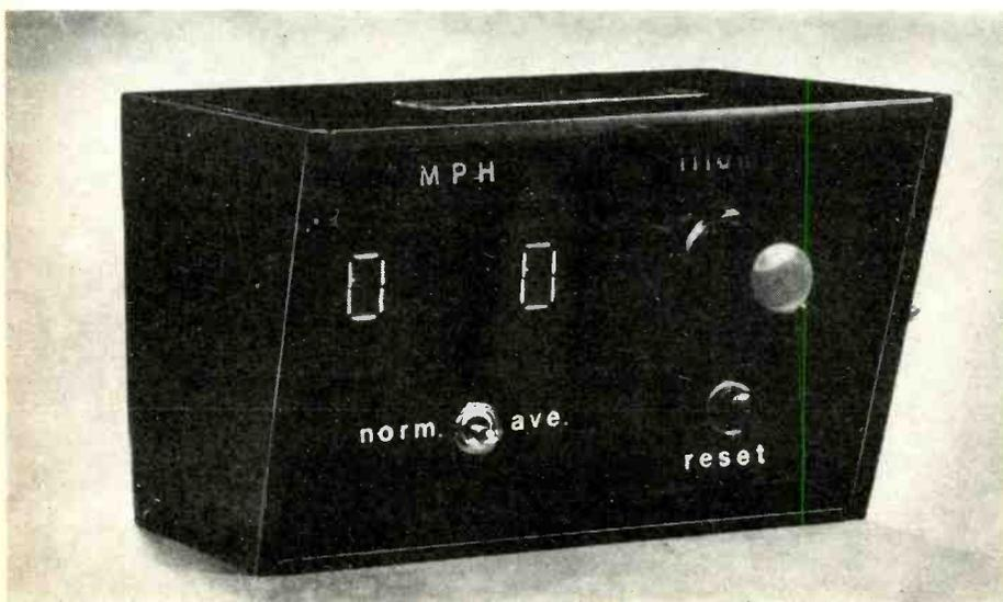
Fig. 1. The completed speedometer and average speed indicator.
