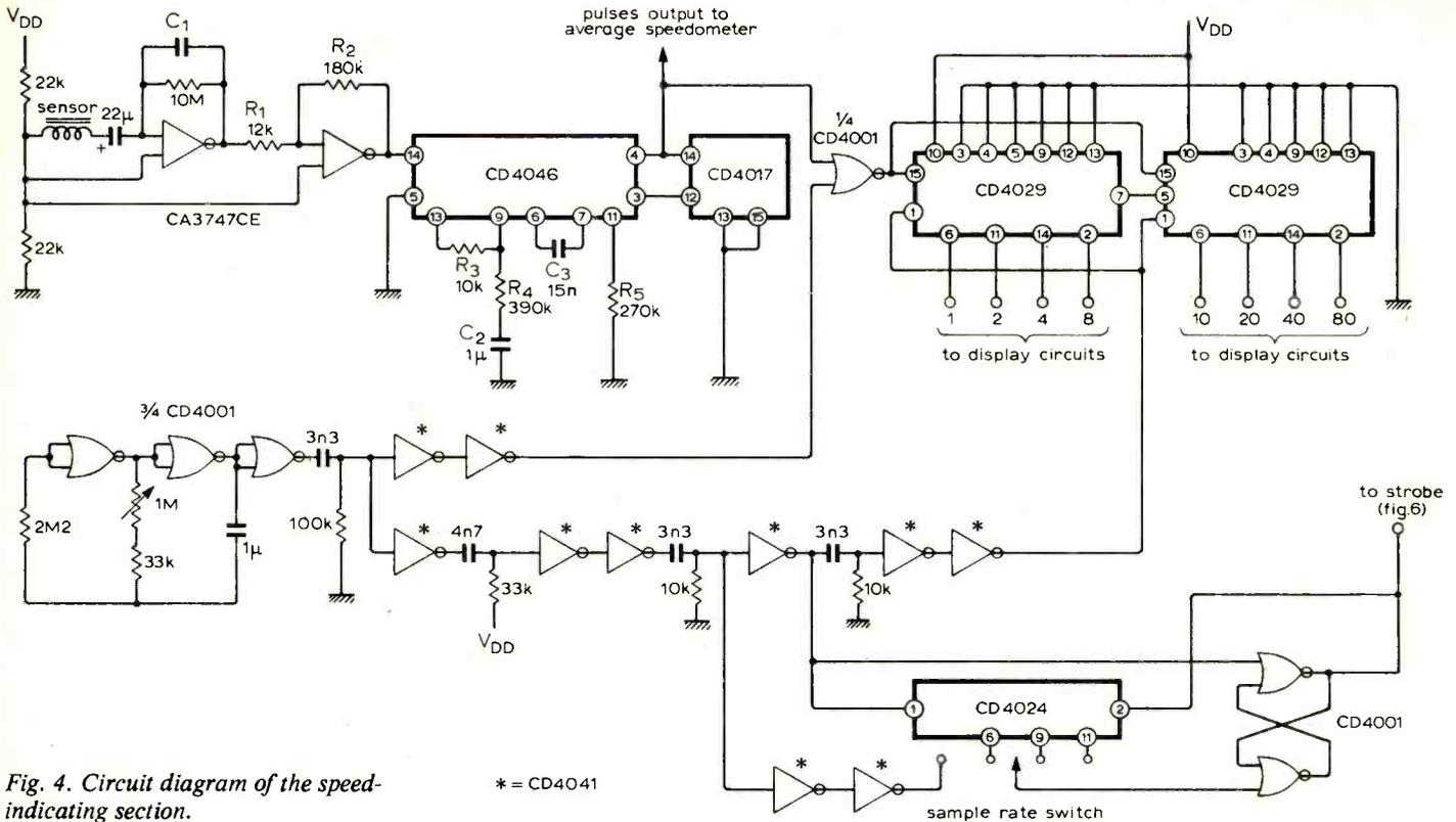
Fig. 4. Circuit diagram of the speed-indicating section.
