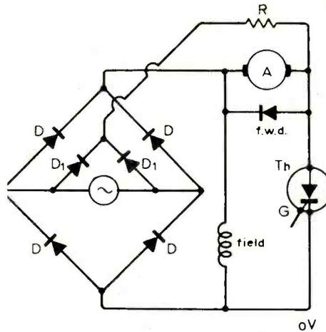
Fig. 3. Basic circuit of power unit showing auxiliary diodes *D<sub>1</sub>* and resistive load *R*.
