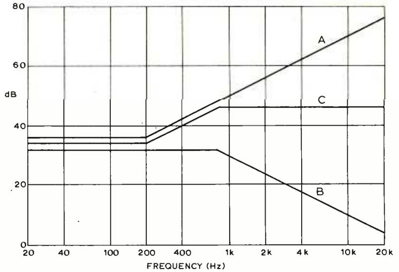
Fig. 3, but in order to obtain a flat response it is necessary to simultaneously boost and cut the signal, which can cause overload and noise problems as the two operations are performed in different parts of the circuit, in contrast to the Baxandall arrangement.
