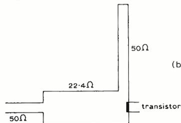
Fig. 7. Stripline methods of construction for (a) power splitter, and (b) transistor match.
