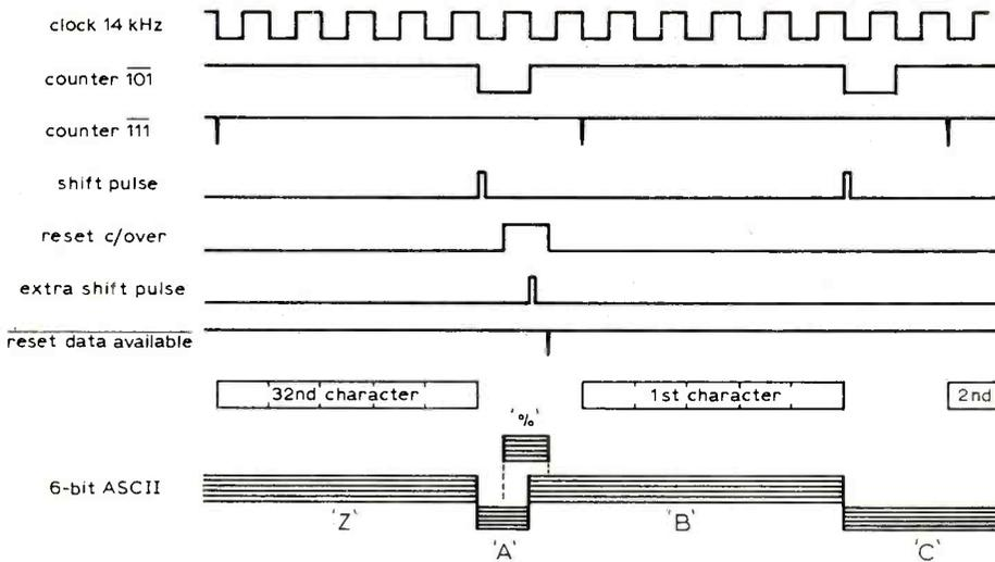
Fig. 2. Display control logic timing diagram. Regular shift pulses output new ASCII data from the shift register to the read-only memory character generator as soon as the last column of the current character has been displayed. New characters are added during the reset period. The foremost right-hand character "A" is then lost and the next character "B" takes its place at the right-hand end of the display.
