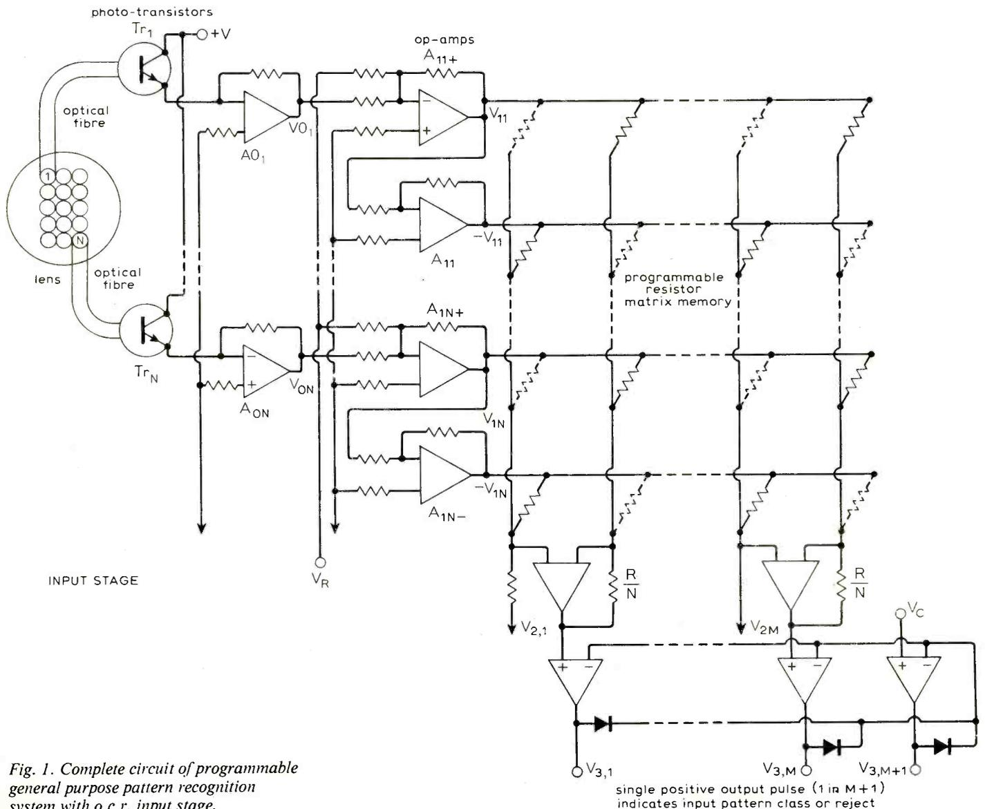
Fig. 1. Complete circuit of programmable general purpose pattern recognition system with o.c.r. input stage.
