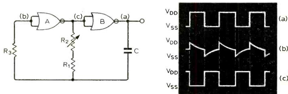
Fig. 7. c.m.o.s. timing oscillator circuit, with waveforms.  $R_2$  varies the frequency.
