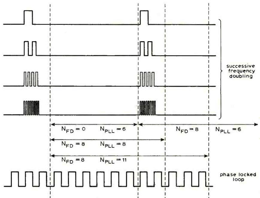
Fig. 5. Frequency-doubling techniques compared with a p.l.l. method of frequency multiplication.  $N_{FD}$  and  $N_{PLL}$  are the number of pulses obtained by each method.
