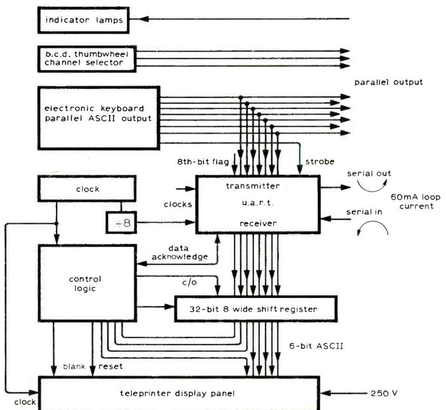
Fig. 1. Keyboard/display block diagram.
