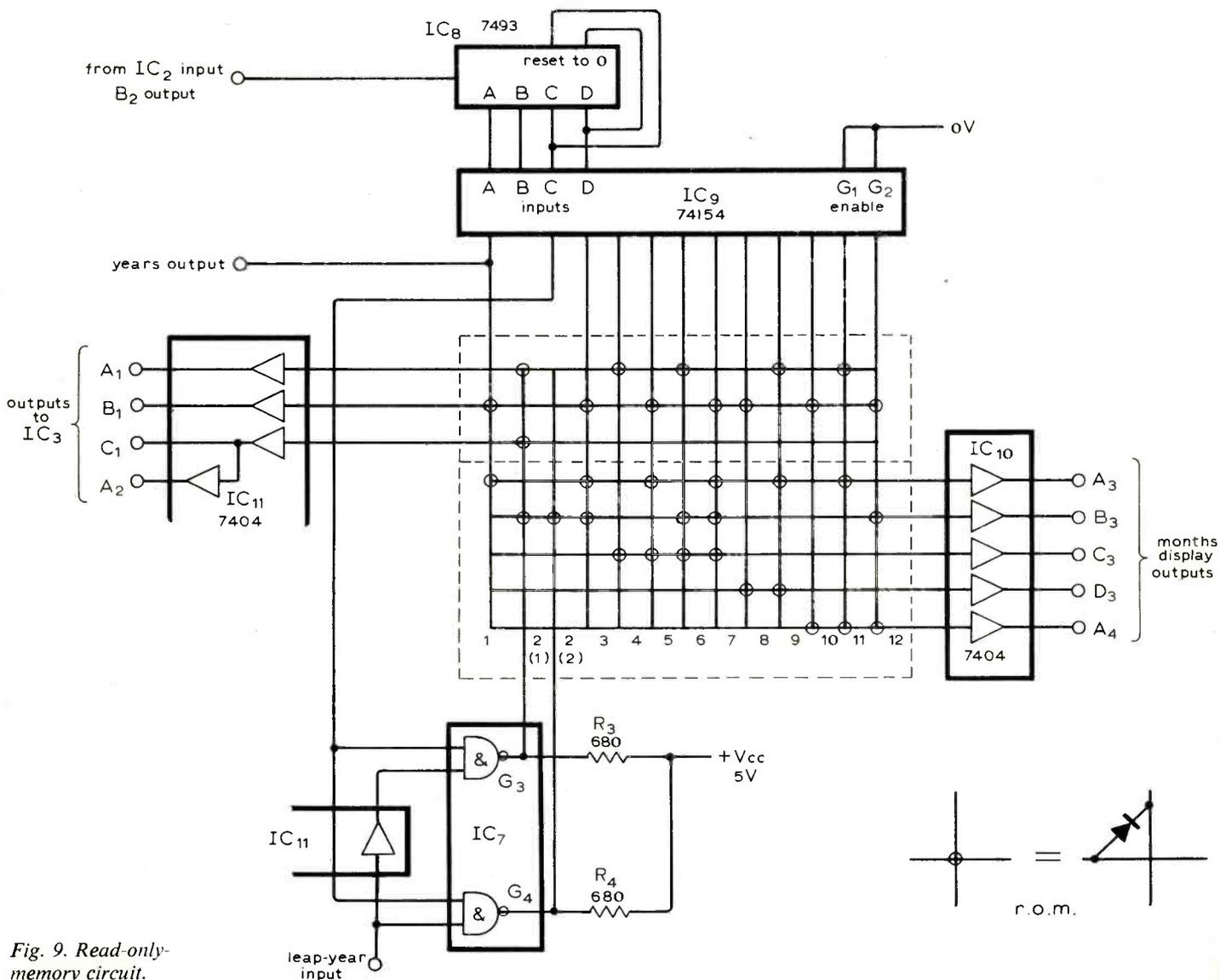
Fig. 9. Read-only-memory circuit.
