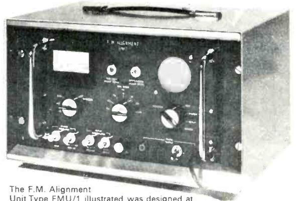
The F.M. Alignment Unit Type FMU/1 illustrated was designed at the Royal Radar Establishment, Malvern, to suit Ampex Recorders working on the IRIG intermediate band specification (using ES 100 Electronics) e.g. Model Numbers FR 1200, FR 1260, FR 1300, FR 1800L, FB 400, PR 500
