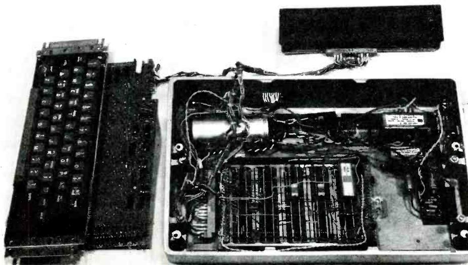
Fig. 9. Internal view of the "teleprinter" showing general layout.
