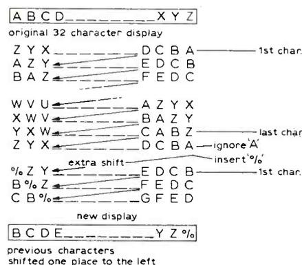
Fig. 3. New character insertion at right-hand end of display.
