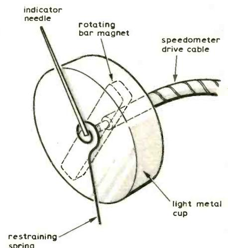
Fig. 2. A conventional mechanical speedometer.
