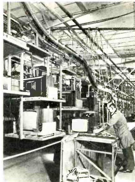
*End of the production line at the Telefusion Group's fully mechanized factory at Kearsley, Lancashire. Hytrac conveyers link the stages of assembly—printed circuit board construction, test and inspection, cable loom, plug and socket assembly, chassis sub-assembly, chassis assembly and a thorough eight-hour soak test of the completed sets.*
