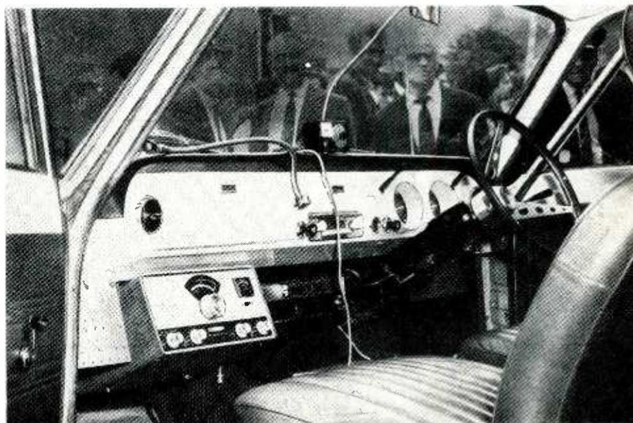
The mobile installation of G3WRV, Grahame Harding, comprising a Heathkit HW-32 200W, 14MHz transceiver and an Eagle RF-40 field strength meter.
