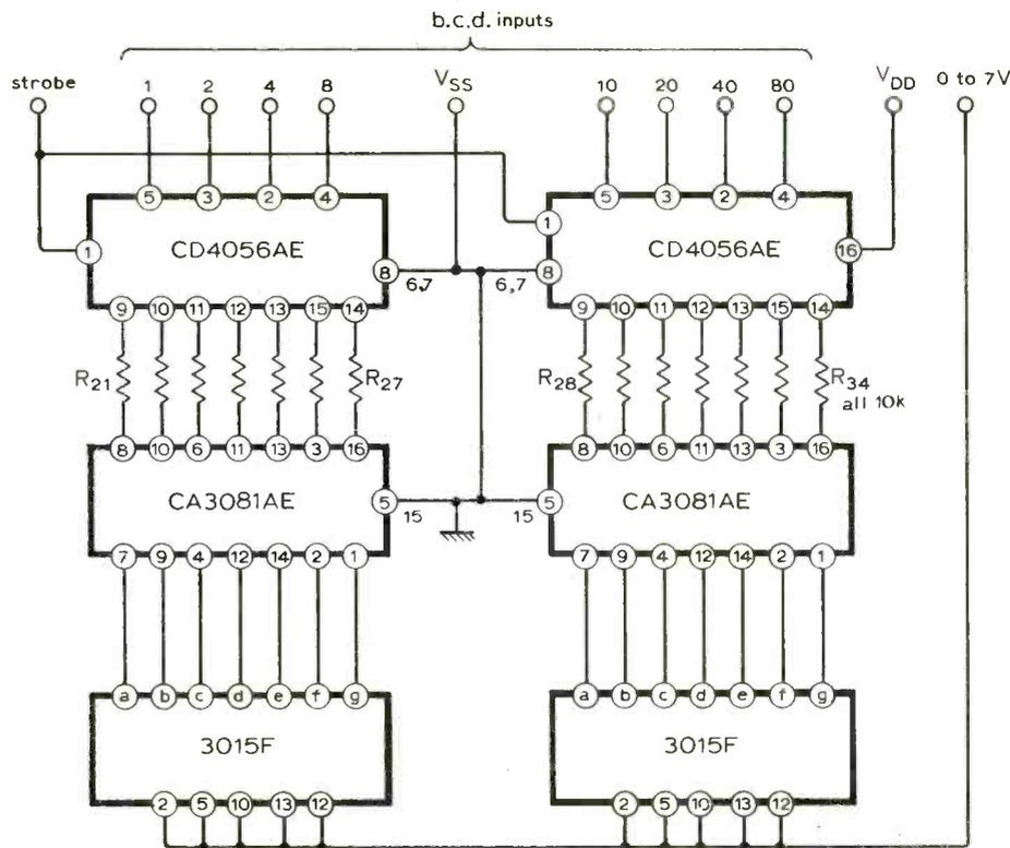
Fig. 6. Decoder, driver and display.
