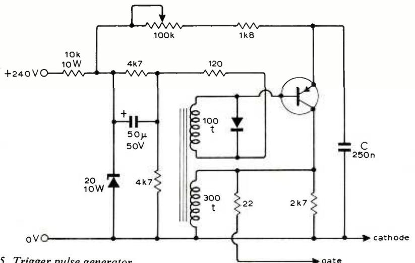
Fig. 5. Trigger pulse generator.
