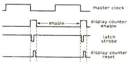
Fig. 9. Timing of the enable, latch and reset pulses.
