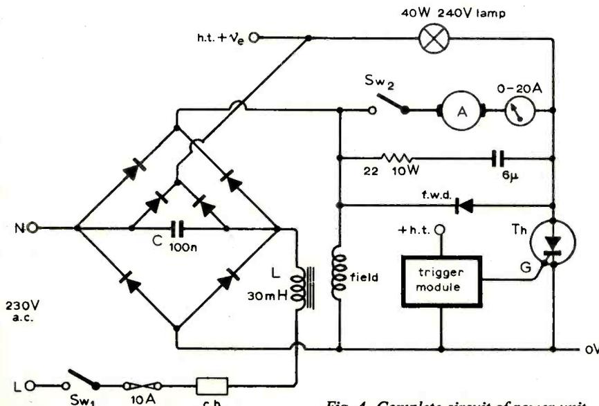
Fig. 4. Complete circuit of power unit.
