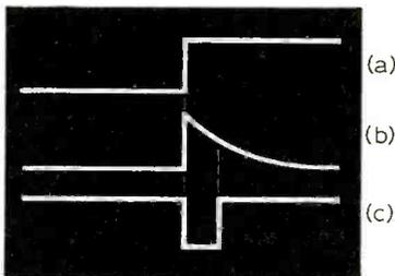
Fig. 8. Differentiating circuit and NOR gate used as a monostable delay element.
