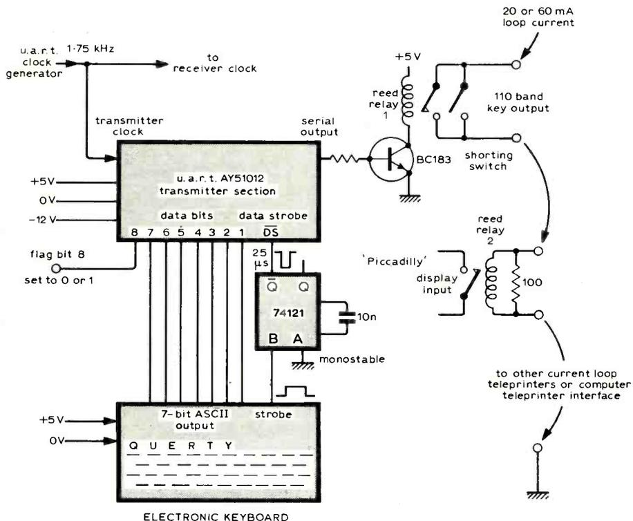
Fig. 5. Keyboard serializer. This circuit may be used independently to provide a serial current loop output from any parallel ASCII keyboard. Maximum line speed is limited by the reed relays which may be replaced with opto isolators.
