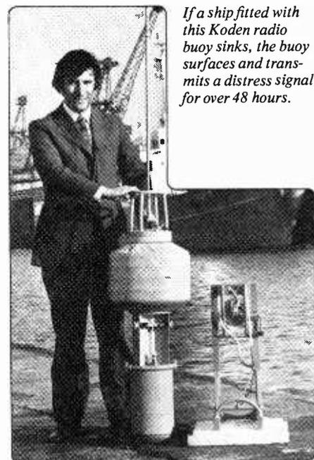
*If a ship fitted with this Kodan radio buoy sinks, the buoy surfaces and transmits a distress signal for over 48 hours.*
