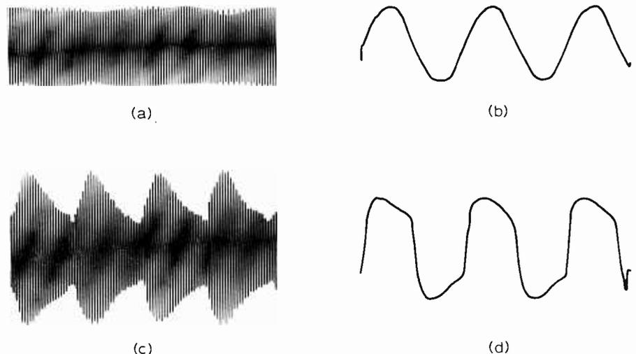
Fig. 4. S.s.b. signals produced from different input signals. A is given by B, and C by D. The peak amplitude ratio of the s.s.b. signals is greater than that of the inputs.
