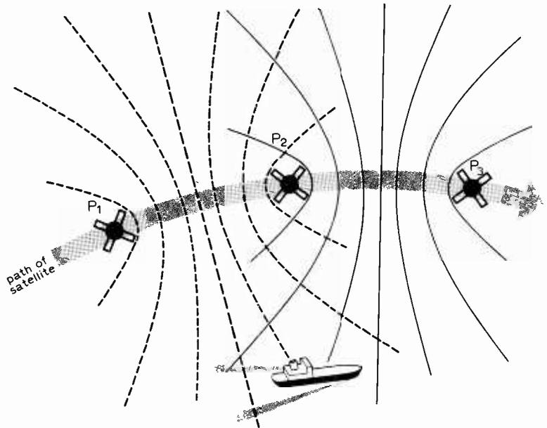
Fig. 1 Hyperbolae representing range differences measured in a ship between "transmitters" at P<sub>1</sub>, P<sub>2</sub> and P<sub>3</sub>, which are in fact successive positions of an orbiting satellite carrying a u.h.f. transmitter. Intersection of two (or more) hyperbolae locates the ship's receiver.
