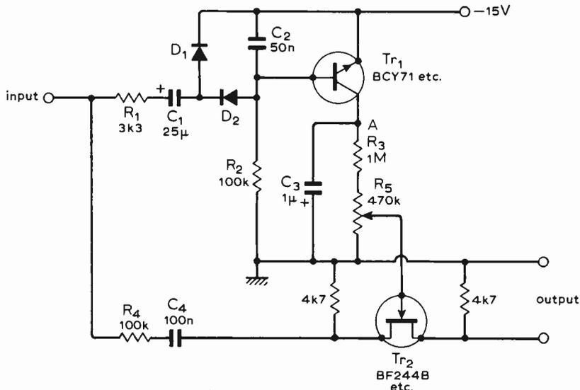
The f.e.t. gate is controlled by this discharging capacitor. Potentiometer  $R_5$  ensures the f.e.t. just switches off when  $C_3$  is fully discharged. When the signal is removed  $Tr_1$  conducts,  $C_3$  charges and so
