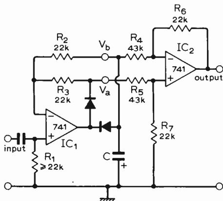
The required voltage waveform, with its minimum d.c. level restored to zero, appears as  $V_a - V_b$ . A low-impedance single-ended output is provided by  $IC_2$  and, in this case, unity gain overall.
