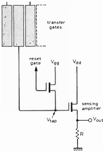
Fig. 6. Biased-gate tapping technique for the fabrication of transversal filters with electronically-variable weighting coefficients.
