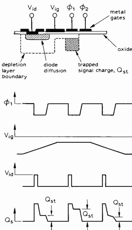
Fig. 3. Technique for the linear injection of charge into a c.c.d.
