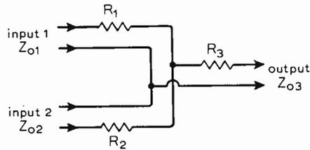
Fig. 2. Simple matched T pad for combining the outputs of two generators. When  $Z_{01} = Z_{02} = Z_{03}$ ,  $R = R_2 = R_3$ , such that  $R_1 = Z_{01}(n-1)/n+1$ , where  $n$  is the number of inputs (two in this case). Insertion loss is 6dB.
