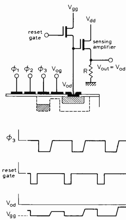
Fig. 4. Floating diffusion reset method of converting the charge present in a c.c.d. to an electrical signal.
