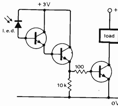
sistors lose gain at low currents, but the frequency response is poor as the stored charge can only be removed by internal recombination. There is no problem, though, in devising faster amplifier circuits, particularly if d.c. response is not required, and the inherent speed of the l.e.d. can be expected to be high.
