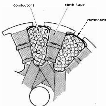
Fig. 2. Armature insulation.
