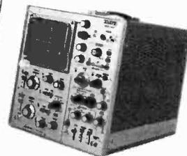
5mV/cm Sensitivity, full delay sweep 1us to 100us/DIV. Timebase A sweep range 0.1us/DIV to 2S/DIV in 23 steps. X 10 magnified. Timebase 3%. Full triggering facilities. Use as XY Mode. Fully solid state. Limited quantity of ex-demonstration. Fully tested and guaranteed special offer. **£349.50** Manual **£7.50**. X 10 probes available **£8.50**.
