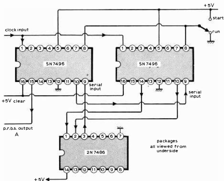
Fig. 7. 1023-bit l.r.s. generator using two five-bit t.t.l. shift registers and an exclusive-OR gate.
