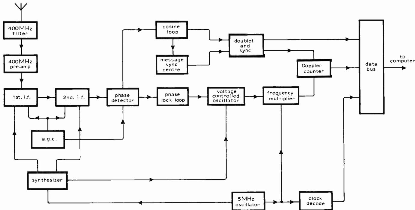
Fig. 9 Simplified receiver block diagram.
