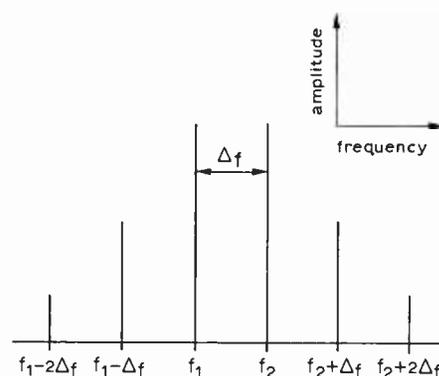
Fig. 3. Intermodulation products produced by clipping a two-equal-tone signal, omitting the products centred on harmonics of the two basic frequencies.
