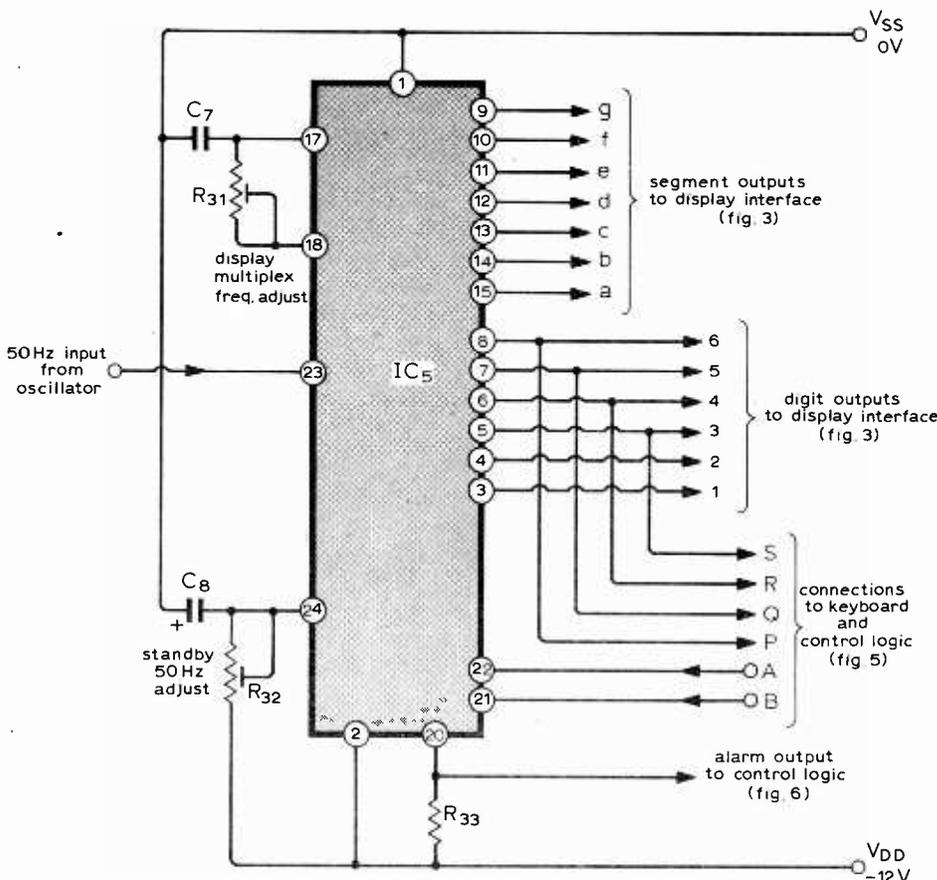
Fig. 4. The clock chip with its associated presets and outputs.
