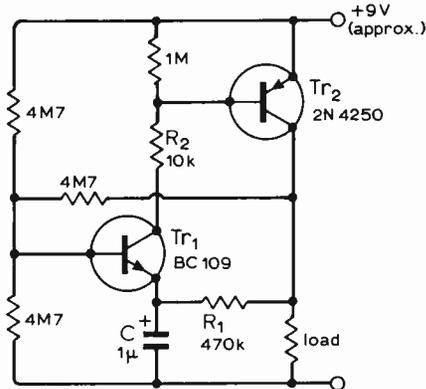
about 10% over the  $-20^\circ\text{C}$  to  $+100^\circ\text{C}$  temperature range. This variation may be reduced to about 1% by the addition of an emitter follower on the base of  $Tr_1$ , of complementary polarity to  $Tr_1$ , to cancel the  $V_{BE}$  temperature drift of this transistor.
