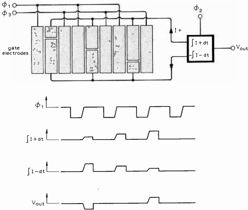
Fig. 5. Split-gate tapping technique for the fabrication of fixed weighting coefficient transversal filters.
