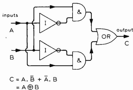
Fig. 2. Logic function and circuit realization of exclusive-OR (modulo-2) gate.
