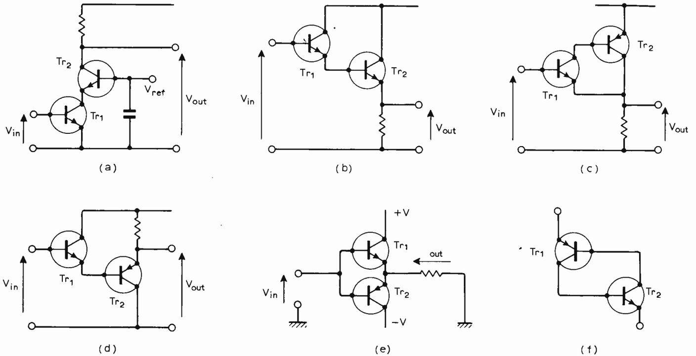
Fig. 2. Other ways of connecting two transistors are common-emitter, common-base i.e. cascode (a), common-collector pair i.e. Darlington (b), complementary pair with only one  $V_{be}$  drop (c), complementary pair with no  $V_{be}$  drop (d), symmetrical complementary pair i.e. class B amplifier (e), and the regenerative pair (f).
