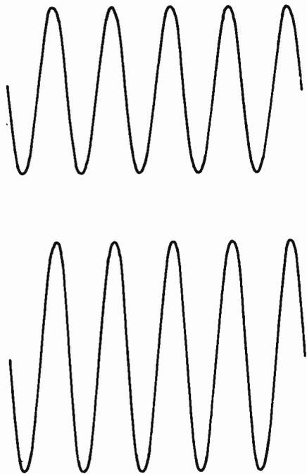
Fig. 8. Top: output of Datong r.f. clipper with input sinusoid just below clipping threshold. Bottom: same but input level 20dB above clipping threshold.
