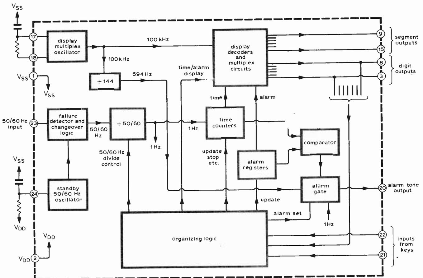
Fig. 1. Block diagram of the digital clock logic.
