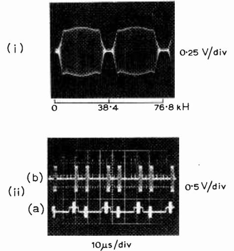
Fig. 8. Swept frequency response (i) and simulated clutter cancellation (ii) of a moving target indicator using c.c.ds. (Lower trace: filter input; upper trace: filter output.)
