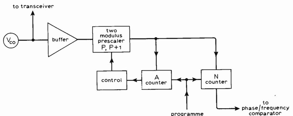
The only restriction is that  $A$  is less than  $N$ . If for any reason  $A$  must be greater than  $N$ , then a three-modulus counter, i.e.  $\div 40/41/42$ , can be used, thus halving the  $A$  count.
