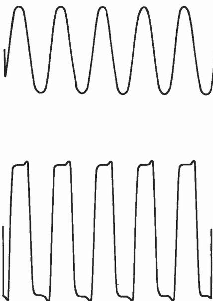
Fig. 2. Top: the output of an a.f. clipper when fed with a sine wave at a level just below the clipping threshold. Bottom: the same but with the input level increased by 20dB.
