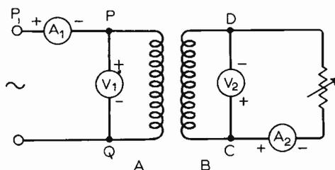
Fig. 2. Connection of meters to the transformer.
