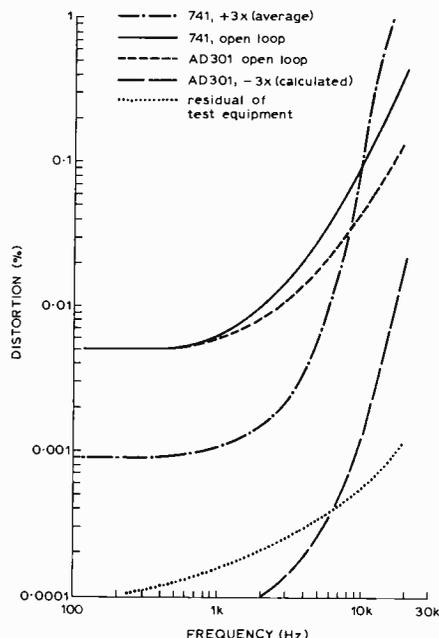
with common-mode signals of equal amplitude, proving Mr Linsley Hood's point about common-mode failure. It turned out that results varied widely between specimens, the best of the 20 op-amps tested producing about 0.001% at 2V output and the worst about 0.1%, when measured with series feedback at 8kHz ( $A_v=3$ ). From this one can conclude that it is wise to avoid series feedback at gains of less than, say,  $10\times$  when using these operational amplifiers in low-distortion circuits.
