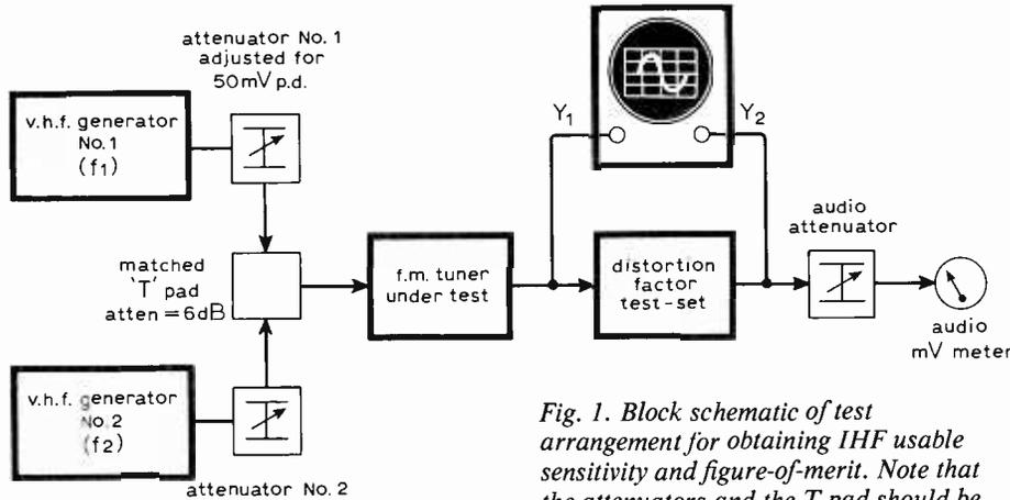
Fig. 1. Block schematic of test arrangement for obtaining IHF usable sensitivity and figure-of-merit. Note that the attenuators and the T-pad should be matched to each other and to the aerial input of the tuner.
