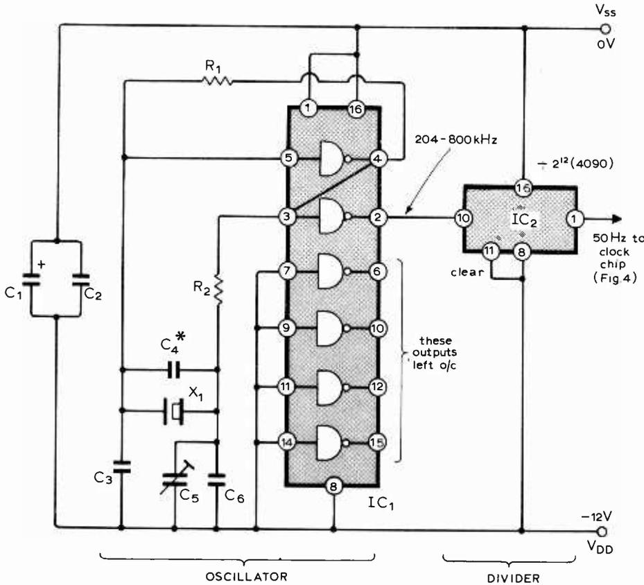
Fig. 2. Crystal oscillator and frequency divider. (For note on asterisked  $C_4$  see next month.)
