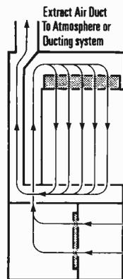
Provides vertical flow of filtered air. Free standing unit utilising minimum floor space. Uses standard single phase electrics. Clean design.
