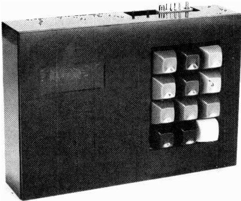
Fig. 7. The prototype clock. The unit is primarily intended as a timer, the display being of secondary importance. Connexions at top right are for an external power supply and switched output.
