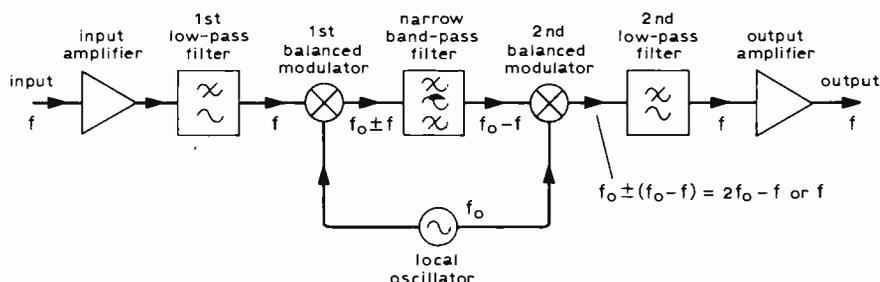
Fig. 5. Wave analyzer used in restored-frequency mode as a narrow-band tunable filter.
