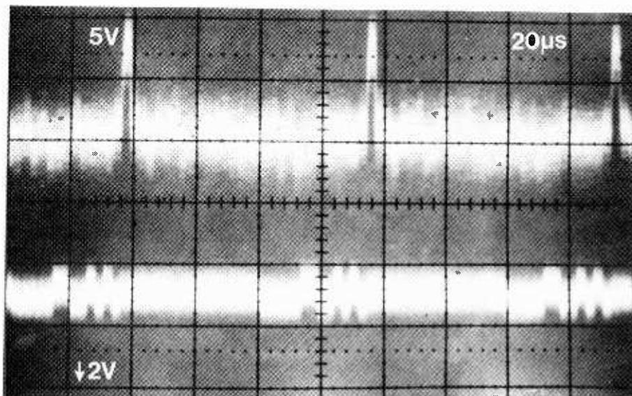
Fig. 11. Correlation of a 13-bit Barker sequence immersed in white additive noise. (Lower trace: input to c.c.d. matched filter; upper trace: filter output.)
