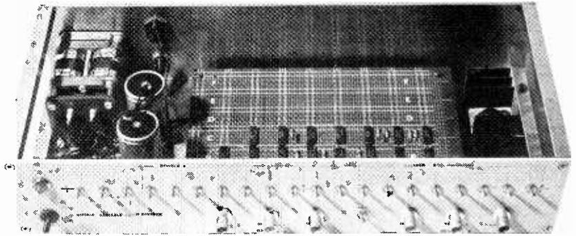
Fig. 8. Internal layout of the dual ten-stage 1023-bit p.r.b.s. generator/programmable frequency divider.
