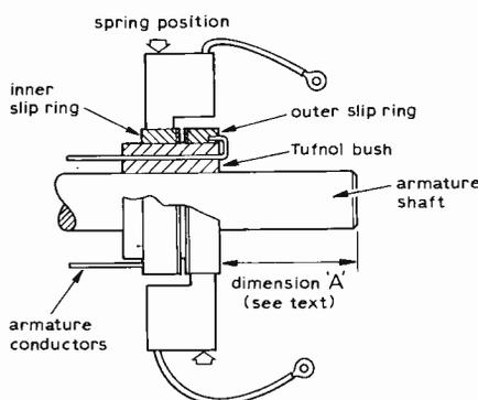
Fig. 1. Sectional view of slip-ring assembly and brushes.
