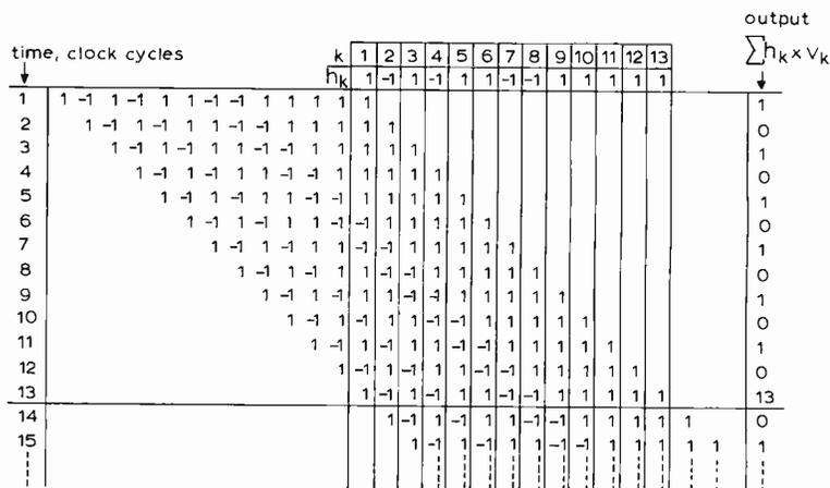
Fig. 10. Schematic of the operation of a matched filter when coded with a 13-bit Barker sequence. At clock cycle 1, the received sequence has just entered the matched filter. As the sequence progresses through the receiver filter, the auto-correlation function is output.
