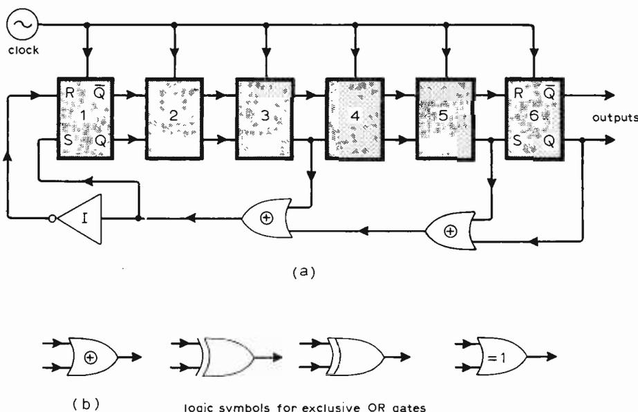
Fig. 1(a). P.r.b.s. generator using a shift register with exclusive-OR (modulo-2) feedback.
