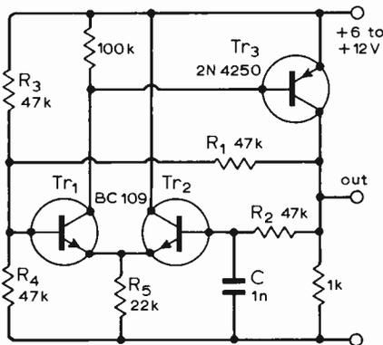
Timing may be varied with resistors  $R_1$  and  $R_2$ , and with capacitor  $C$ . Duty cycle is determined by the ratio of resistors  $R_3$  and  $R_4$ . The values shown give 50% duty cycle. Resistor  $R_5$  may be decreased in value to allow higher output currents and/or high frequency operation; however, temperature stability is then slightly degraded.
