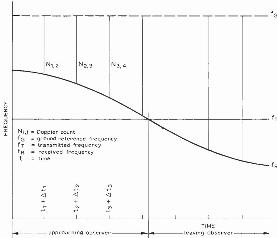
Fig. 4 Integrated Doppler count:  $f_T$  is the satellite's transmitted frequency;  $f_R$  the received frequency,  $f_G$  the ship's reference frequency; and  $N_{1,2}$  etc. the Doppler count ( $t$  = time).
