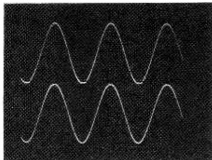
Lower trace is the input signal; upper trace is the output from the restorer. Oscilloscope was obtained with the circuit operating on a 150Hz signal with an amplitude of 40mV peak-to-peak.
