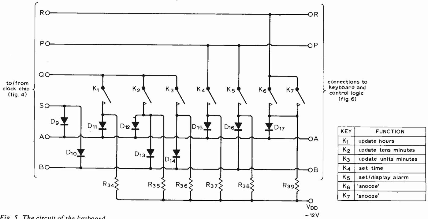
Fig. 5. The circuit of the keyboard.
