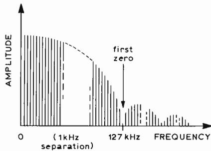
Fig. 4. Line spectrum of a 127-bit l.r.s. clocked at 127kHz.
