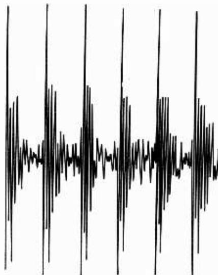
Fig. 1. A section of the first vowel sound in the word "hello" as seen on an oscilloscope
