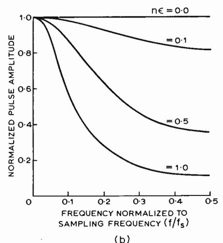
Fig. 2. Impulse response of a c.c.d. analogue delay line with varying  $n\epsilon$  product (a). Frequency response modification for a c.c.d. analogue delay line with varying  $n\epsilon$  product (b).
