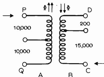
Fig. 1. Arrangement of Unilab transformer windings.
