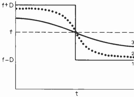
Fig. 3 Doppler shifts for observers at three different distances from the satellite's orbital path.
