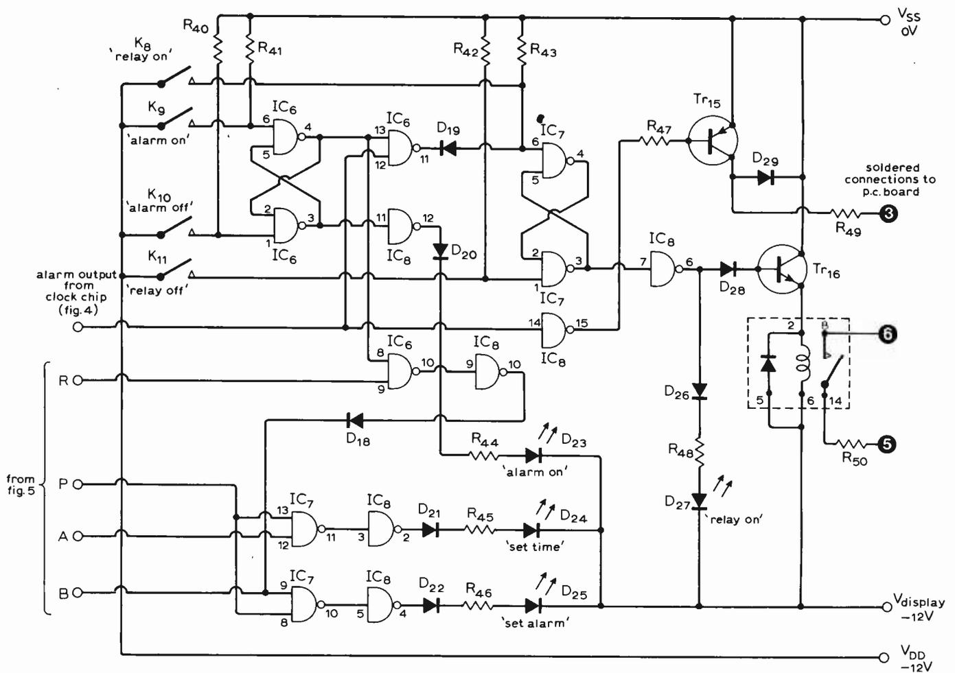
Fig. 6. Control logic circuit.
