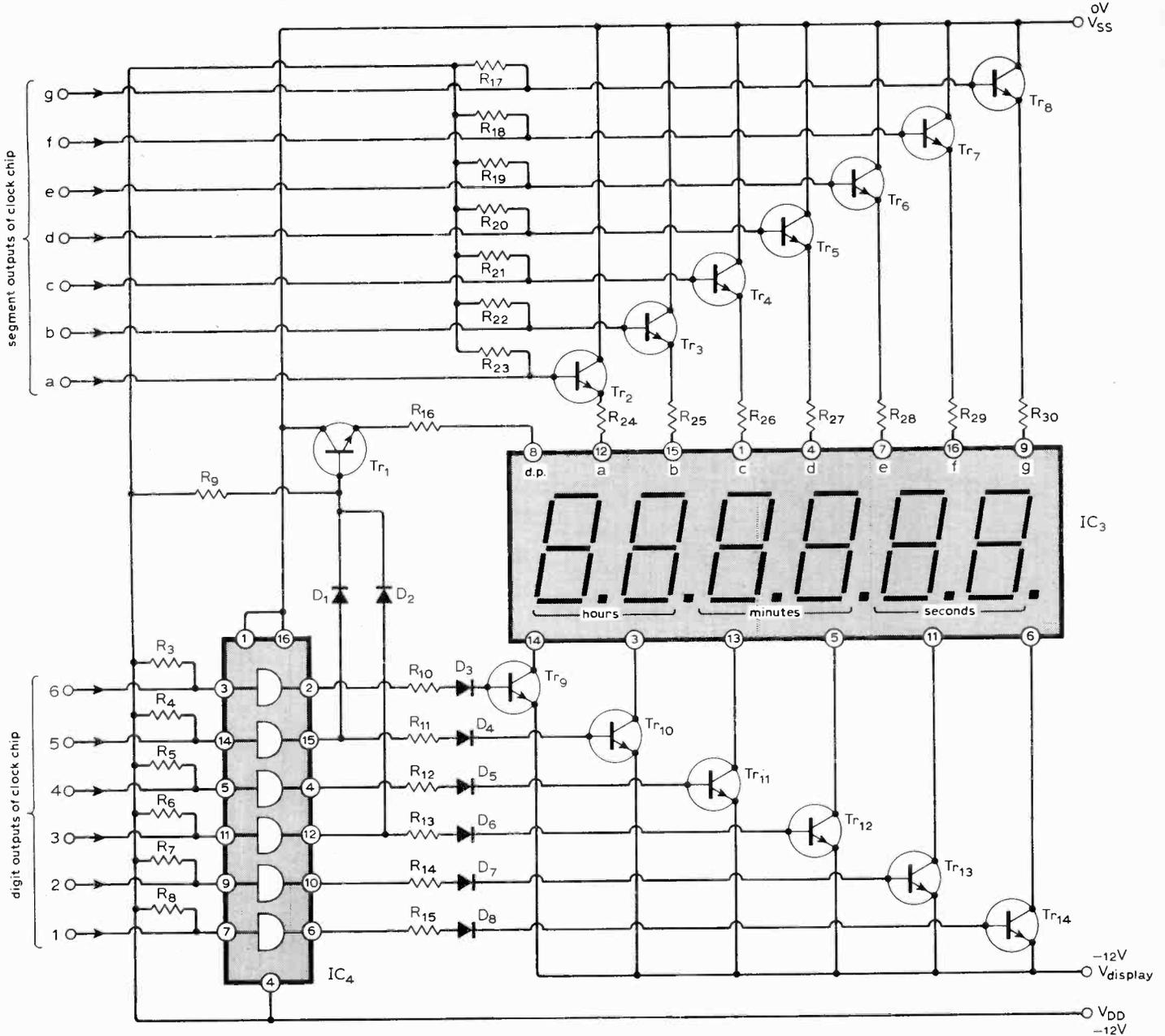
Fig. 3. Interface to enable the p.m.o.s. chip to drive the l.e.d. display.
