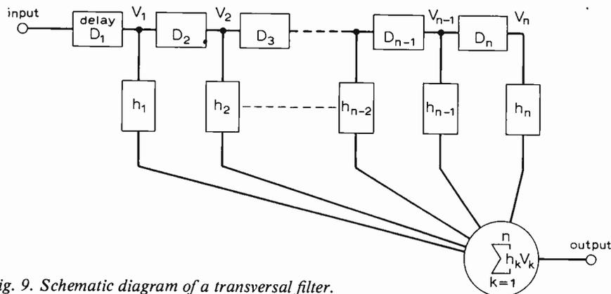
Fig. 9. Schematic diagram of a transversal filter.
