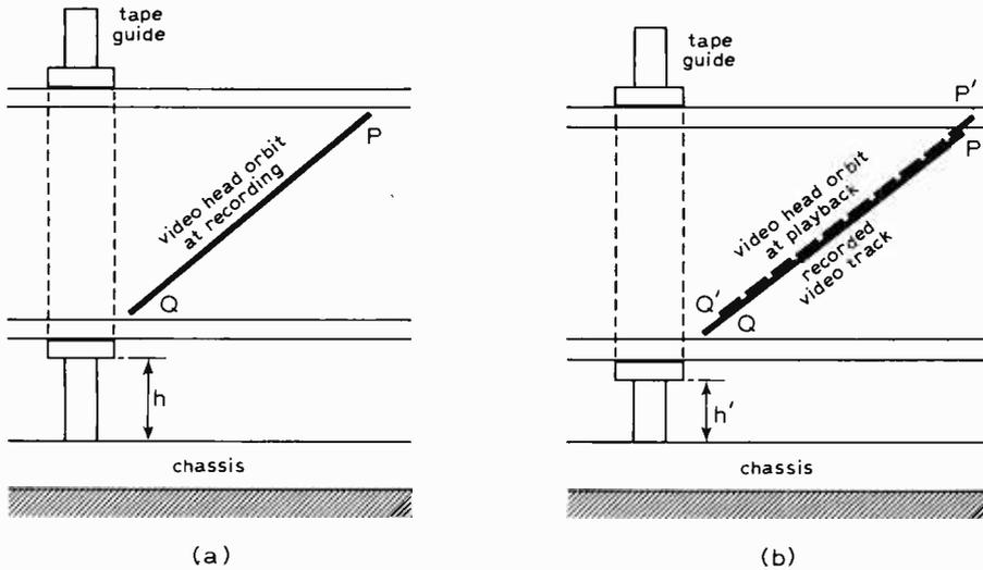
Fig. 5. Effects of tape guiding errors.
