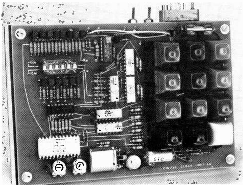
Fig. 10. The complete unit, assembled in a "tray" with the alarm speaker and batteries underneath the board.
