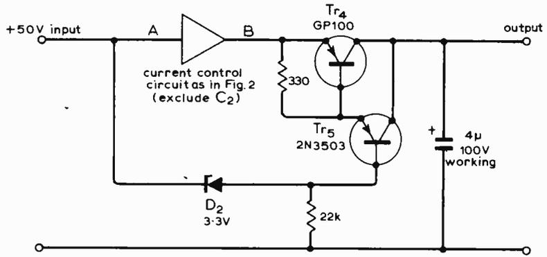
Fig. 3. Practical tandem current control circuit for several parallel loads.
