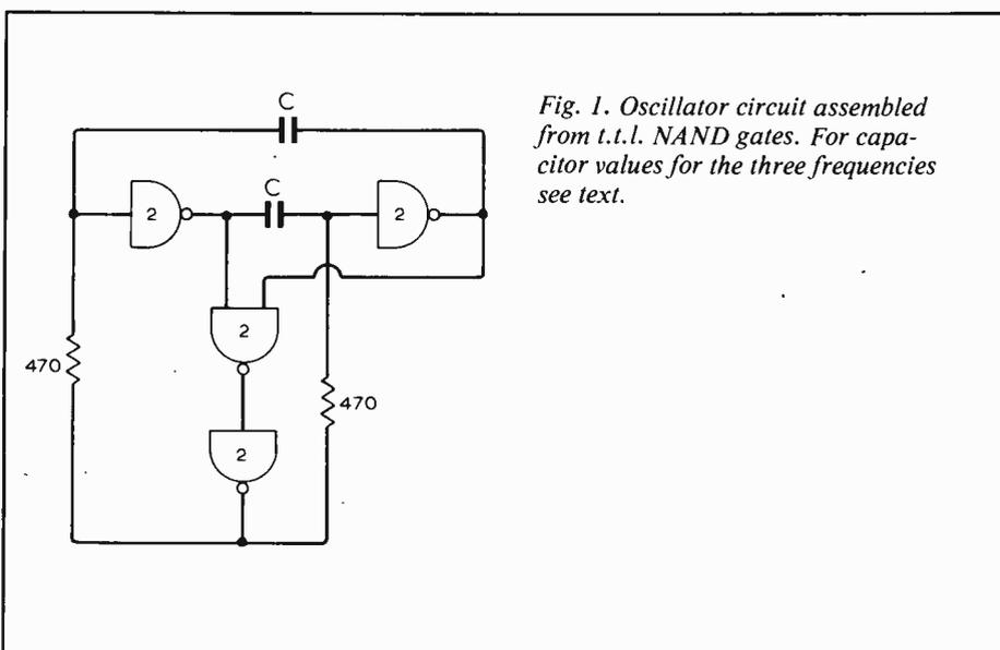
Fig. 1. Oscillator circuit assembled from t.t.l. NAND gates. For capacitor values for the three frequencies see text.
