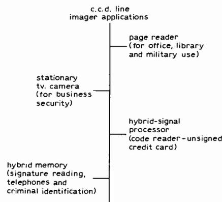
Fig. 1. Possible applications for a c.c.d. line imager.
