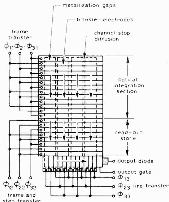
of the array is called the optical integration section; the area of the device upon which the image of the scene falls.
