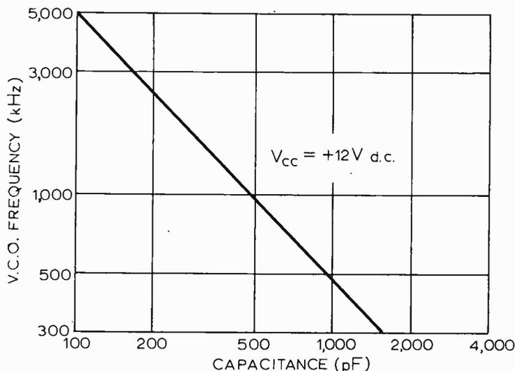
Fig. 5. Free running frequency of the v.c.o. plotted against the capacitance connected between pins 11 and 12.
