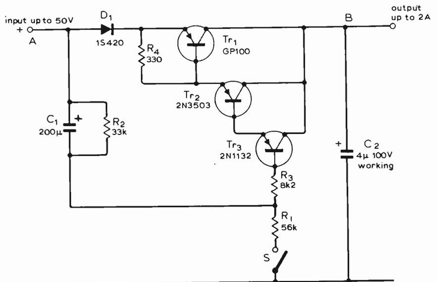
Fig. 2. Current control alone will be adequate in most cases.
