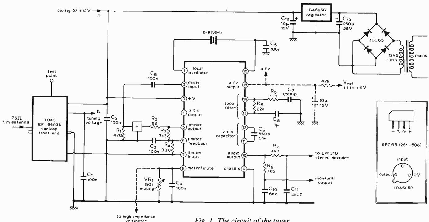
Fig. 1. The circuit of the tuner.
