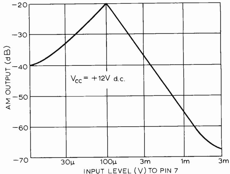
Fig. 3. A.m. rejection plotted against the signal input level to the NE563.
