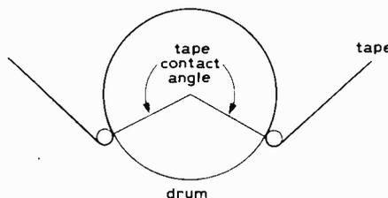
Fig. 4. Representation of the contact angle.
