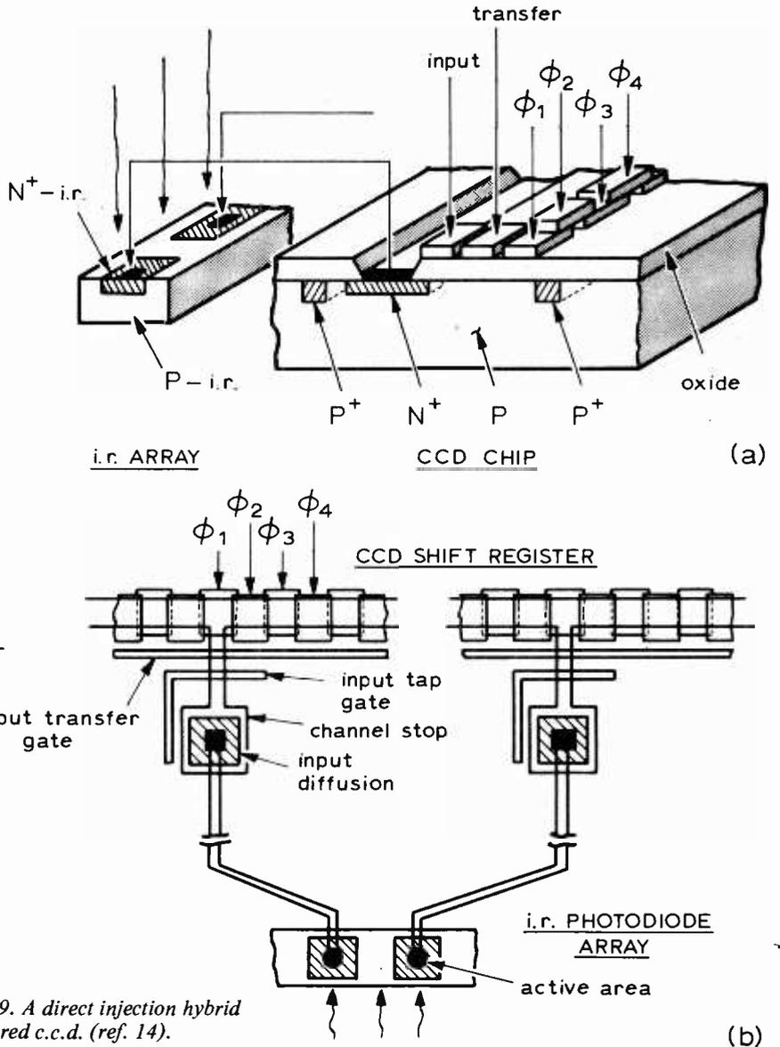
Fig. 9. A direct injection hybrid infrared c.c.d. (ref. 14).
