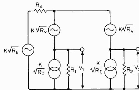
$$\text{NF} = \frac{\text{total noise output power}}{\text{noise output power produced by } R_S}$$
