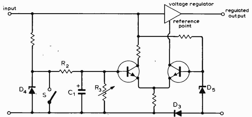
Fig. 4. Theoretical current control of regulated supply.
