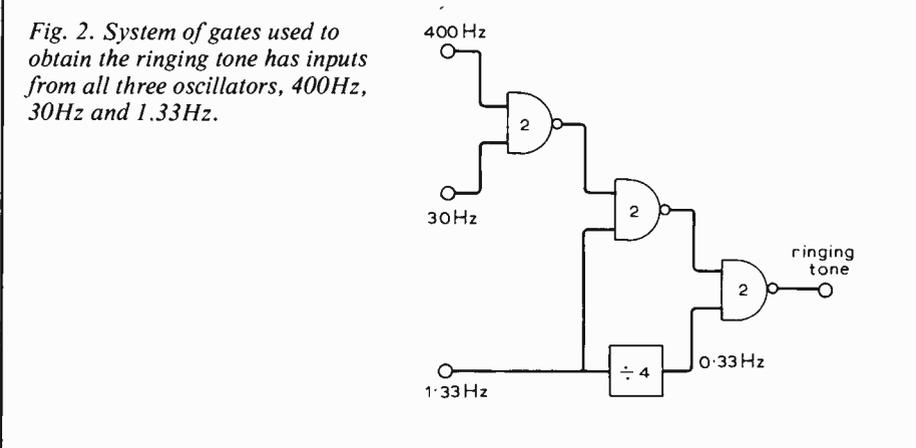
Fig. 2. System of gates used to obtain the ringing tone has inputs from all three oscillators, 400Hz, 30Hz and 1.33Hz.
