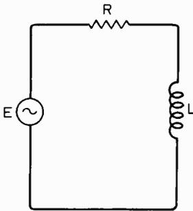
Fig. 2 Simple circuit for illustrating Kirchhoff's voltage law as extended to a.c.
