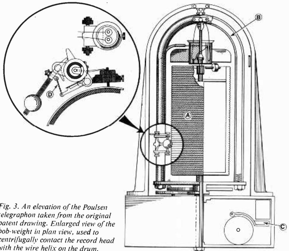
Fig. 3. An elevation of the Poulsen telegraphone taken from the original patent drawing. Enlarged view of the bob-weight in plan view, used to centrifugally contact the record head with the wire helix on the drum.
