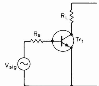
Fig. 2. Single transistor circuit.
