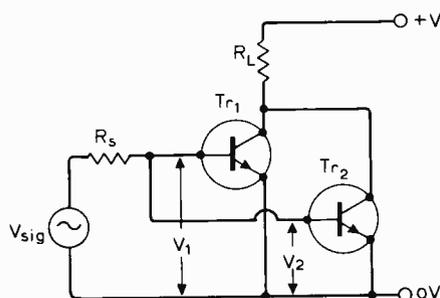
$Tr_1$  and  $Tr_2$  are identical transistors with the same input resistance, current gain and noise generators.
