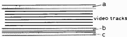
Fig. 2. Pattern of the tracks produced by a "longitudinal" mode v.t.r. Tracks a, b and c are also used for sound, synchronization pulses and cue.
