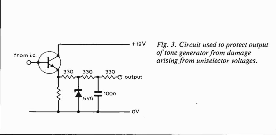
Fig. 3. Circuit used to protect output of tone generator from damage arising from uniselector voltages.
