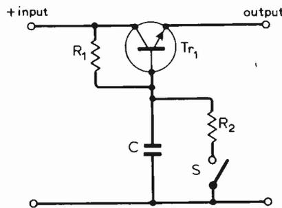
Fig. 1. Basic voltage control circuit.
