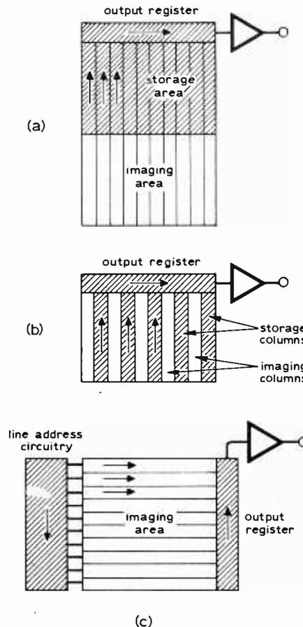
Fig. 8. Design choices—(a) frame transfer, (b) interline transfer, (c) line transfer (ref. 7).
