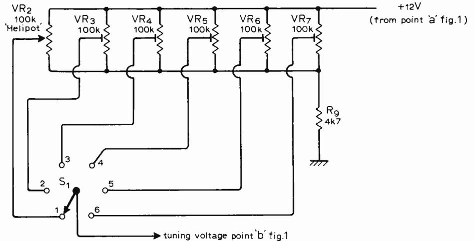
Fig. 2. The preset and continuous tuning unit.
