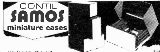
in easy-to-work blue and white PVC/steel. Assemble in the lower half; complete before springing cover into place—four Pozidrivs, two to hinge it, two to fasten it. Carries four P.C. boards horizontally, or two vertically; four required for each case (for one vertical board, two each case) Prices correct January 1975.
