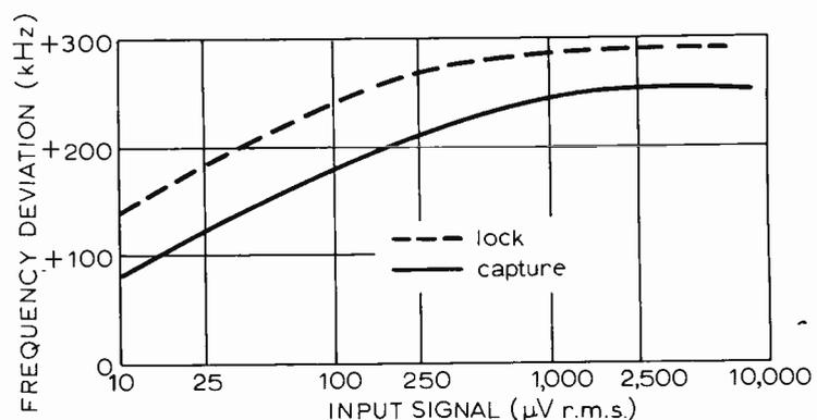
Fig. 4. Variation of the capture and lock ranges with the signal input level.
