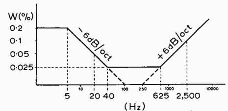
Fig. 6. Limits imposed on the frequency components of line frequency "wobbling" in the Philips model VCR N1500. The wobble figure *W* is defined by  $W = \Delta f_L / f_{Ln}$  where  $f_{Ln}$  is the nominal line frequency and  $\Delta f_L$  is the total frequency swing about  $f_{Ln}$ .
