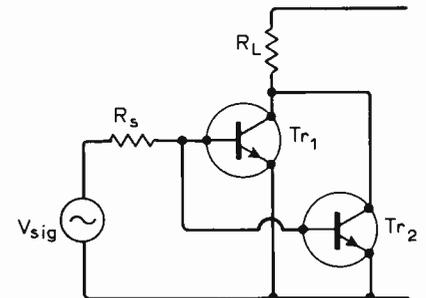
Fig. 1. Two transistors in parallel.
