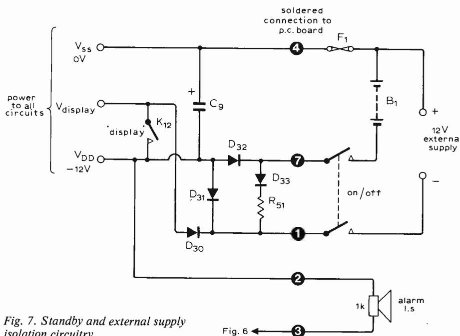
Fig. 7. Standby and external supply isolation circuitry.
