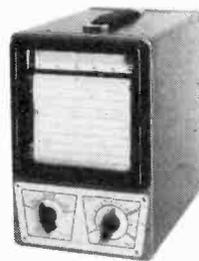
*Measurements ranges AC/DC:* 5-15-150-250-500mA, 1.5-5 Amps
