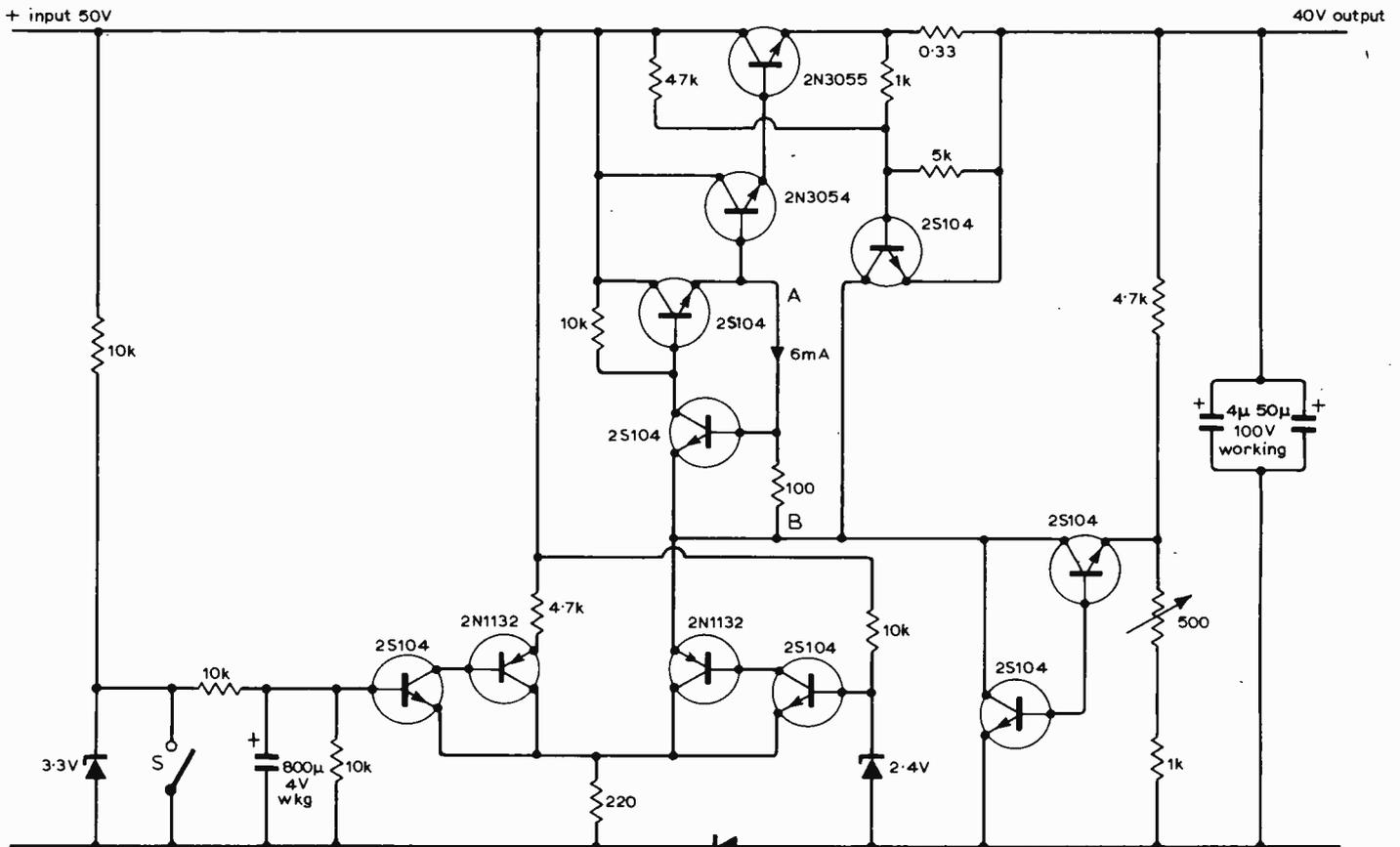
Fig. 5. Complete regulated power pack with current switching control.
