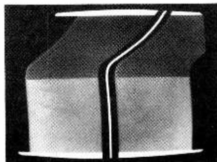
Fig. 9. Test pattern of Fig. 8 applied to the same receiver. In this case the video signal is affected by a  $+16\mu s$  phase jump.
