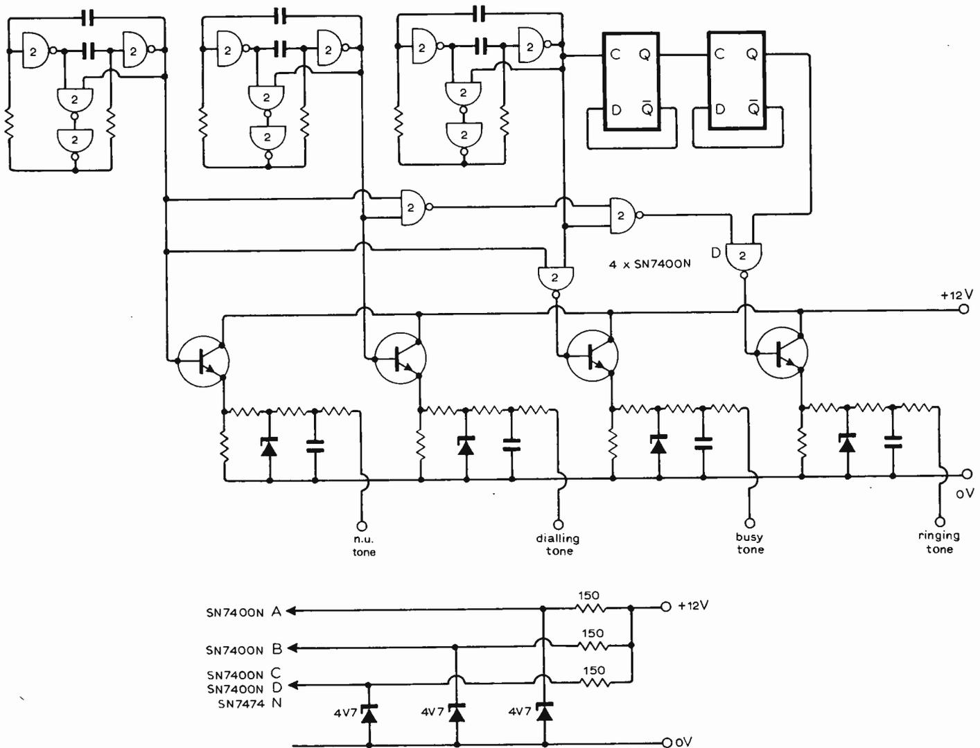
Fig. 4. Complete circuit diagram of the tone generator with voltage supply arrangements below.
