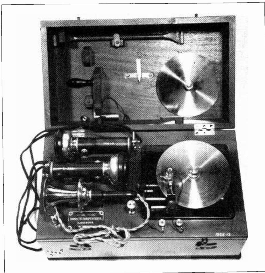
Fig. 4. A commercial version of the telegraphon, circa 1900. The electrical drive motor is not shown. (Photo courtesy Philips Gloeilampenfabrik.)
