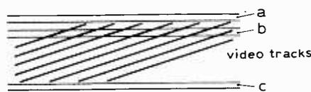
Fig. 3. Pattern of the track employed in helical recording. Again, a, b and c are sound, synchronization and cue tracks.
