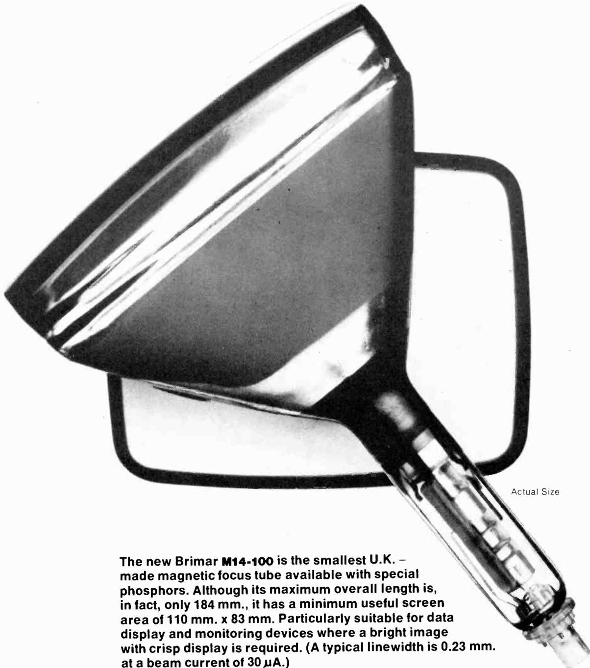
The new Brimar **M14-100** is the smallest U.K. – made magnetic focus tube available with special phosphors. Although its maximum overall length is, in fact, only 184 mm., it has a minimum useful screen area of 110 mm. x 83 mm. Particularly suitable for data display and monitoring devices where a bright image with crisp display is required. (A typical linewidth is 0.23 mm. at a beam current of 30  $\mu$ A.)
