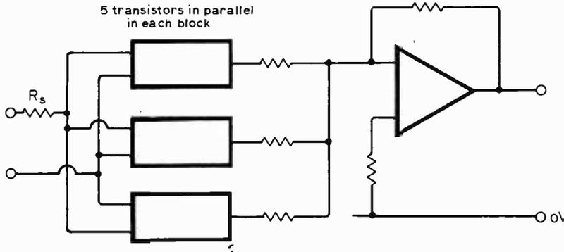
Fig. 4. Arrangement for using several of the Fig. 3 amplifiers and summing their outputs.
