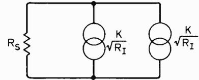
The noise voltage across  $R_S$  is the input voltage to both transistors.
