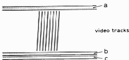
Fig. 1. Pattern of the tracks recorded onto a video tape produced by a "transverse" mode v.t.r. The edge tracks a, b and c are available for sound, synchronization pulses, and cue.
