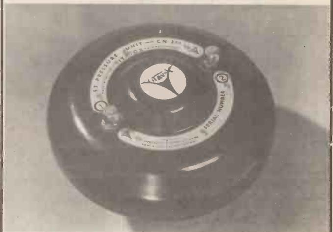
THE S3 PRESSURE UNIT has been designed to meet the growing demand for considerably increased power handling capacity without the sacrifice of either efficiency or frequency response. It features a powerful ceramic magnet and a strong but light diaphragm and voice coil assembly with many new features. It is a robust, reliable unit of exceptional quality. The S3 is one of the units of the Vitavox Power Range.
