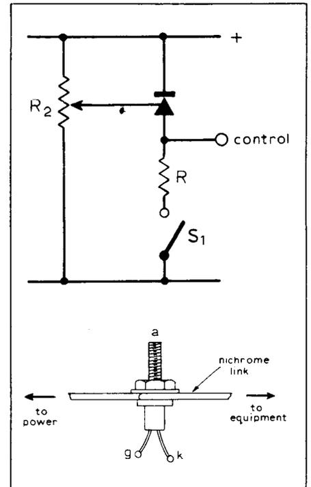
The heating element can be isolated from the thyristor case, or it can be a short resistive link, in the positive line or bolted to a heat sink, and connected to the thyristor anode as shown. In d.c. circuits a 1/25Ω will monitor a 25A circuit with ease. Thyristor packaging and mounting govern the thermal inertia of the system.
