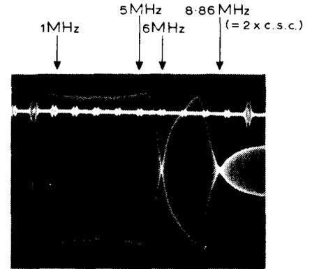
Fig. 10. Sweep response showing effect of 6MHz and 8.86MHz trap circuits.
