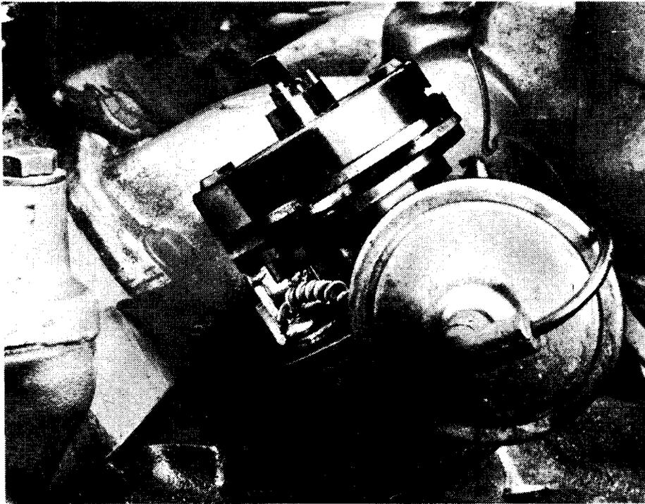
Fig. 8. Horizontal-axis sensor head mounted in a Delco Remy distributor on a Saab motor car.
