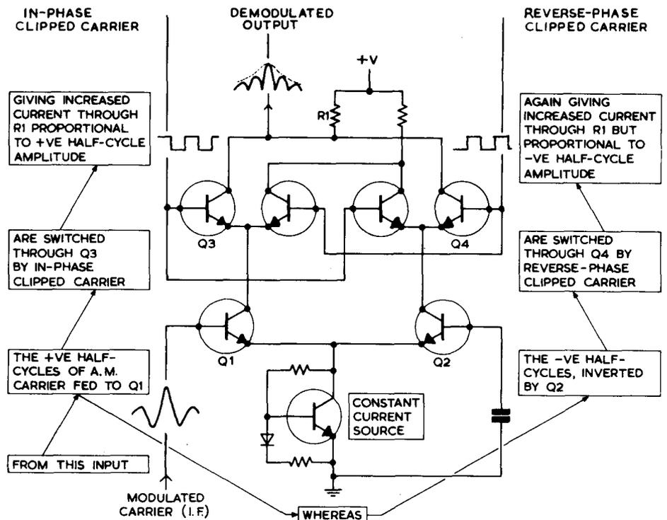
Fig. 9. Circuit action and waveforms of synchronous demodulator.
