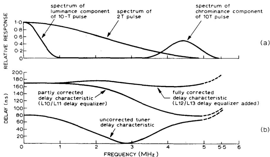
Fig. 11. (a) Spectral response of Insertion Test Signal pulses. (b) Curves showing result of two-stage delay correction.
