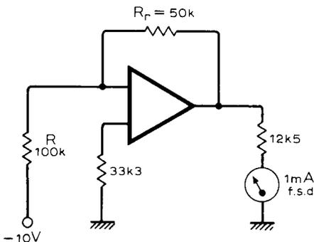
It uses a current instead of voltage meter, but as these are the only moving-coil types made it's of no practical concern.
