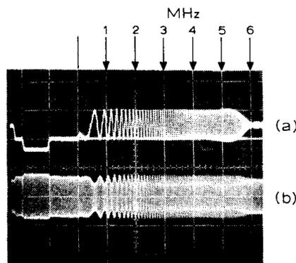
Fig. 12. (a) Tuner overall response (video terminated output) with line-repetitive sweep d.c. to 6MHz. (b) i.f. vision carrier envelope at input to MC1330 for the same signal as in (a).
