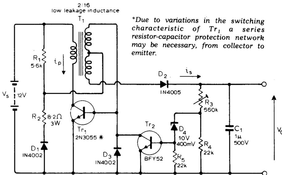
*\*Due to variations in the switching characteristic of  $Tr_1$  a series resistor-capacitor protection network may be necessary, from collector to emitter.*
