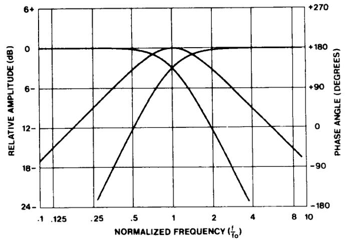
Fig. 7. Three-unit filler driver 2nd order system.
