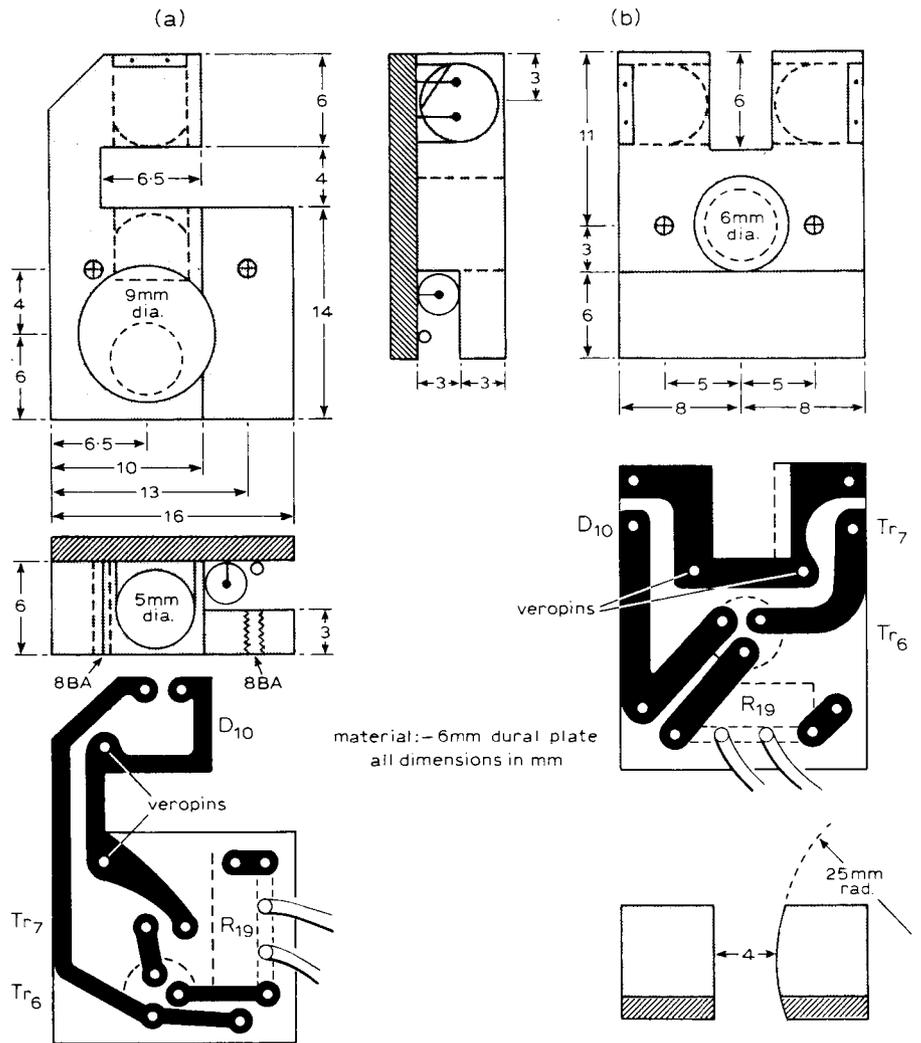
Fig. 5. Vertical and horizontal sensing-head details. The two Veropins in both types earth the circuit and act as locating dowels.
