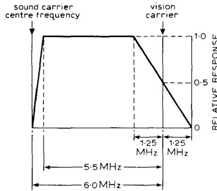
Fig. 8. Ideal receiver vision-channel response (taken from BBC/ITA publication: "Specification of television standards for 625-line system I transmissions". — 1971).
