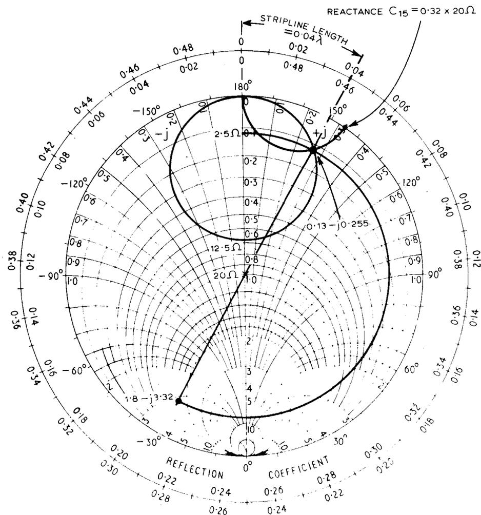
Fig. 1. Output matching network design using a Smith chart.
