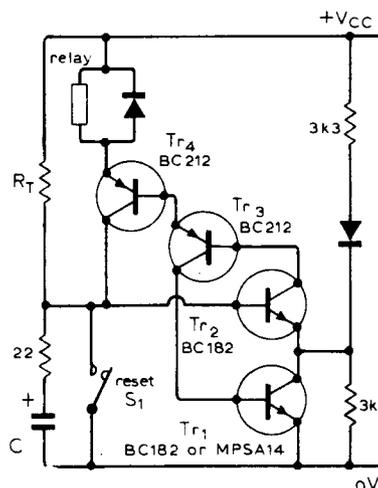
cycle is initiated either by the application of  $V_{cc}$  or by the opening of  $S_1$ . As in the 555, the timing period is  $V_{cc}$  independent as long as it is stable during the timing cycle.
