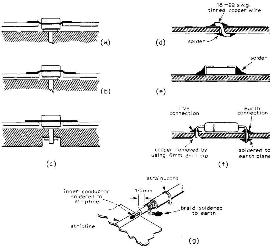
Fig. 4. Component mounting. In (a) and (b) spacers used in mounting a power transistor are not of the correct length, straining stripline leads and possibly causing fracture of package wall. In (c) the spacer is of the correct length. (d) through connection (e) chip capacitor mounting (f) typical resistor mounting (g) how low v.s.w.r. coaxial to stripline transition is made.
