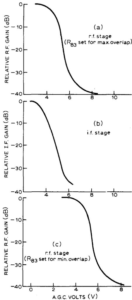
Fig. 13. Tuner a.g.c. characteristics (arranged to show the effect of crossover adjustment).
