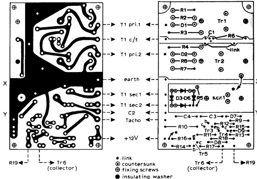
Fig. 2. Double sided p.c.b. layout measuring 2½ × 4 in. This board can be cut across XX and the two halves mounted back to back. Alternatively, if the trigger circuit is to be used with an existing Marston c.d. unit the board below YY may be used.
