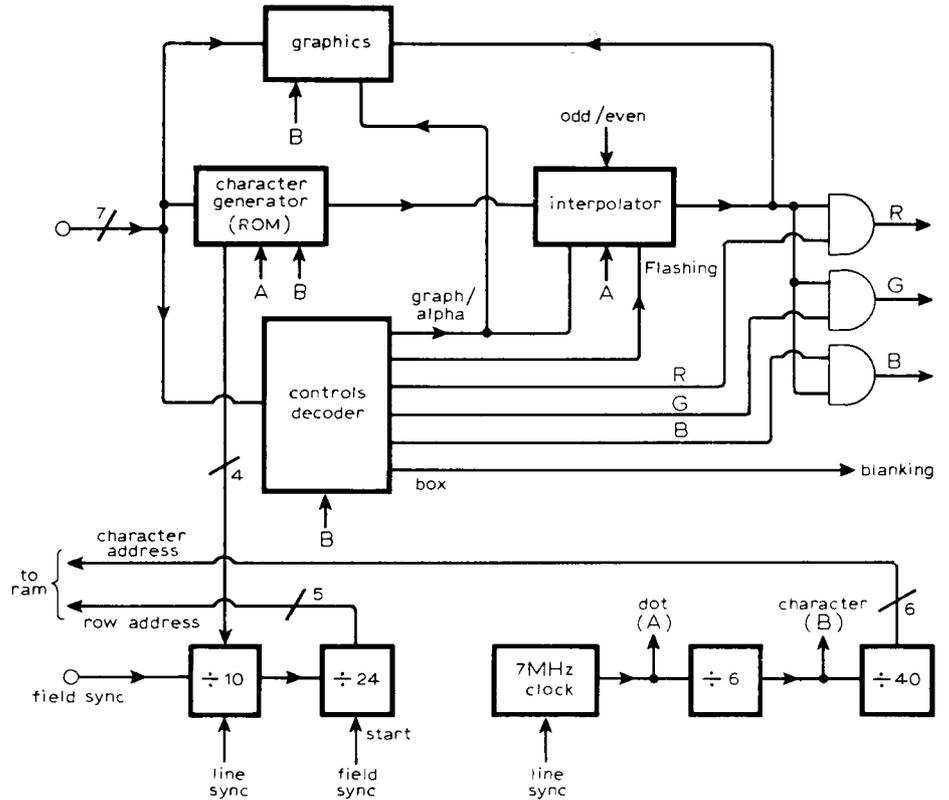
Fig. 8. A typical output processor.
