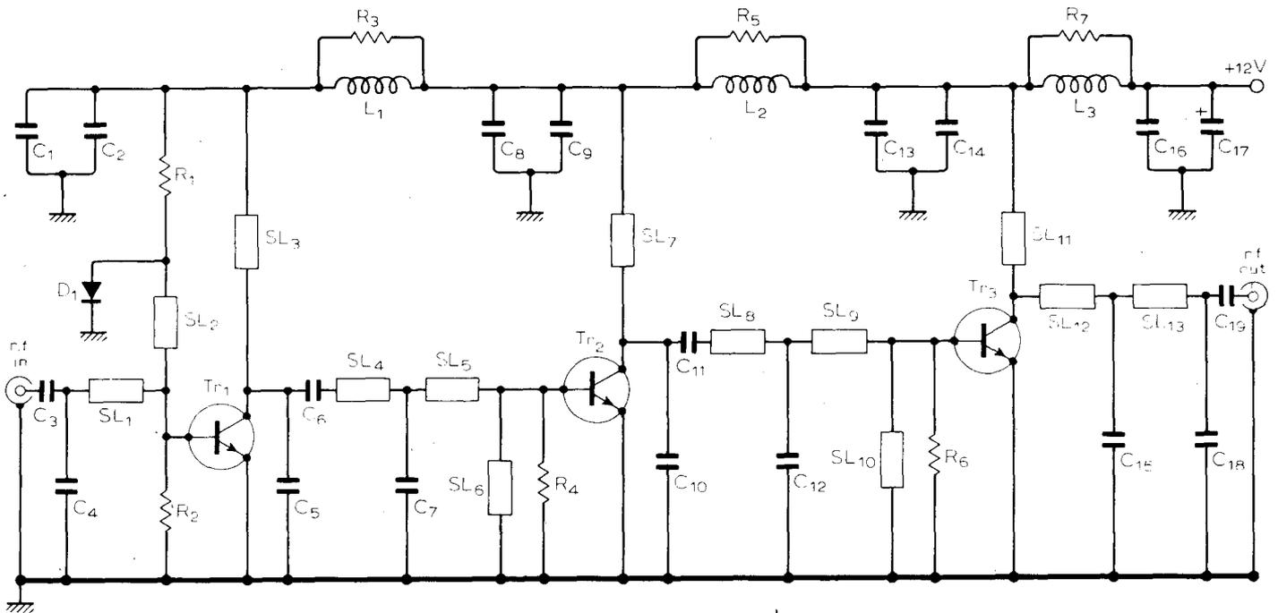
Fig. 2. Circuit diagram of the 20W v.h.f. power amplifier.
