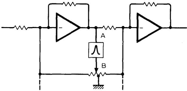
Fig.2. Two-integrator loop used in Technics equalizer permits independent control of Q and centre frequency (using three-gauged control).
