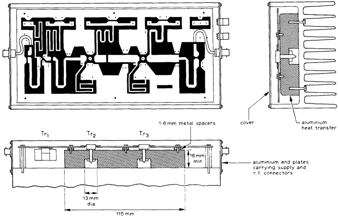
Fig. 3. Assembly of the power amplifier.
