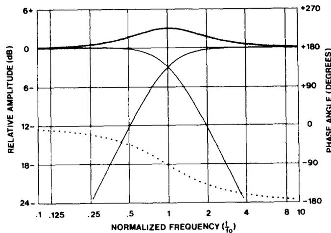
Fig. 3. As Fig. 2, but with tweeter phase reversed.
