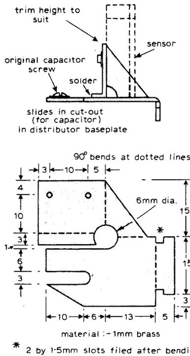
Fig. 6. Mounting bracket for use with a vertical sensing head in a Lucas distributor.
