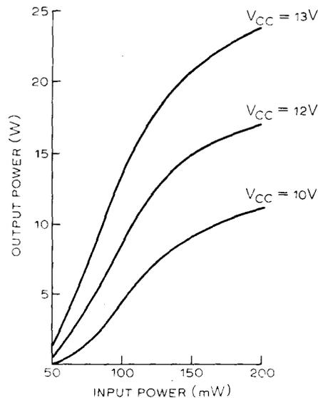
Fig. 5. Input/output characteristic of the amplifier over the 144-146MHz band.
