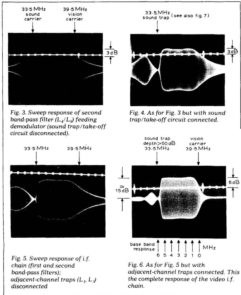
Fig. 3. Sweep response of second band-pass filter ( $L_4/L_6$ ) feeding demodulator (sound trap/take-off circuit disconnected).
