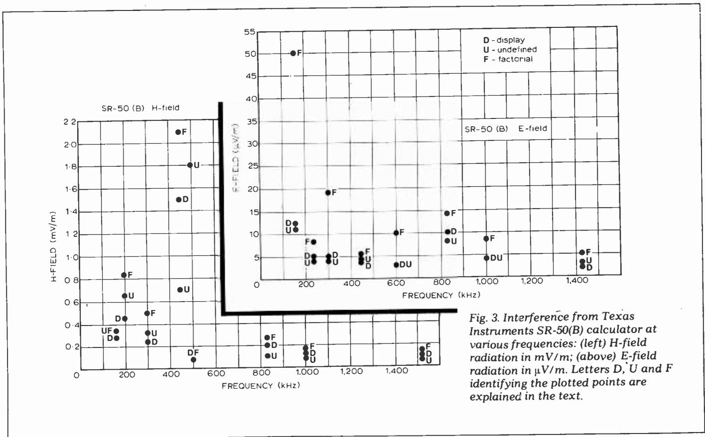
**Fig. 3. Interference from Texas Instruments SR-50(B) calculator at various frequencies: (left) H-field radiation in mV/m; (above) E-field radiation in  $\mu\text{V}/\text{m}$ . Letters D, U and F identifying the plotted points are explained in the text.**
