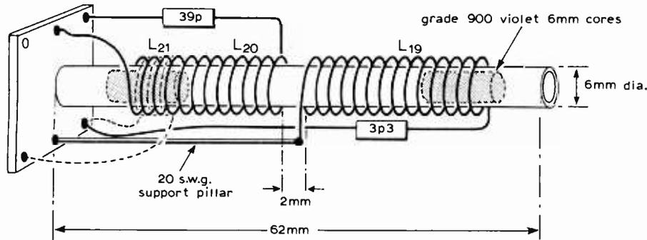
Fig. 15. Dimensions and form of L<sub>19</sub>/L<sub>20</sub>/L<sub>21</sub> coil construction.
