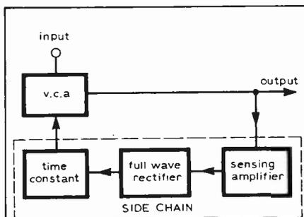
Fig. 1. Voltage-controlled attenuator with d.c. control loop.
