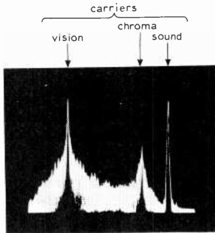
Fig. 18. Spectrum of r.f. television transmission showing distribution and relative energy content of side bands about the vision carrier (left), the colour subcarrier (centre), and the sound carrier (right).
