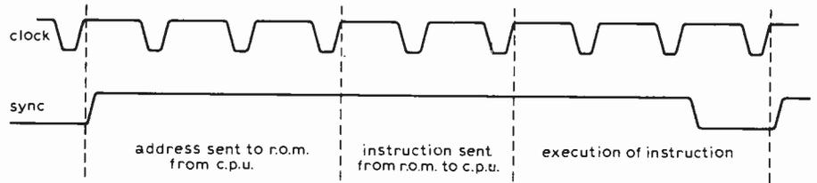
Fig. 5. One machine cycle using a 4-bit bus, illustrating the limitation when compared to higher-capacity buses.
