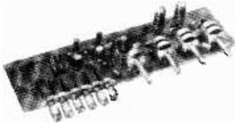
Built to a specification and NOT a price, and yet still the greatest value on the market, the PA100 stereo pre-amplifier has been conceived from the latest circuit techniques. Designed for use with the AL50 power amplifier system, this quality made unit incorporates no less than eight silicon planar transistors, two of these are specially selected low noise NPN devices for use in the input stages.
