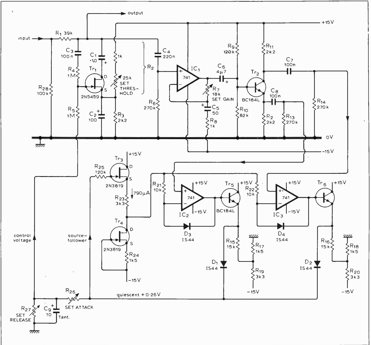
about two Volts. The prevention of saturation is necessary because the recovery time of the 741s causes the frequency response of the precision rectifier circuit to drop off at about 1kHz. The addition of the anti-saturation networks provides a frequency response that starts to fall off significantly above about 12kHz which is ample for our purposes as program signals have very little energy content above this frequency.
