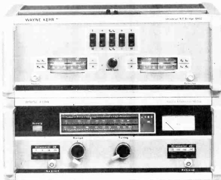
The B602 transformer ratio arm bridge measures impedance in all four quadrants of the complex plane over the frequency range 100kHz to 10MHz. Because of novel features incorporated in the design, values from virtually a short circuit to an open circuit can be measured. This bridge has established a standard of performance and flexibility which is unobtainable from any other radio frequency bridge.
