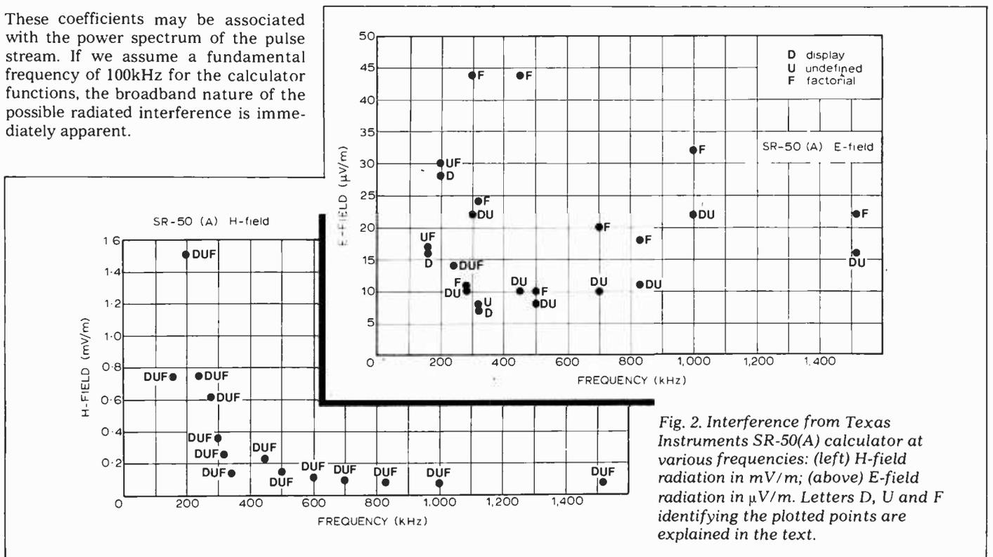
Fig. 2. Interference from Texas Instruments SR-50(A) calculator at various frequencies: (left) H-field radiation in mV/m; (above) E-field radiation in µV/m. Letters D, U and F identifying the plotted points are explained in the text.
