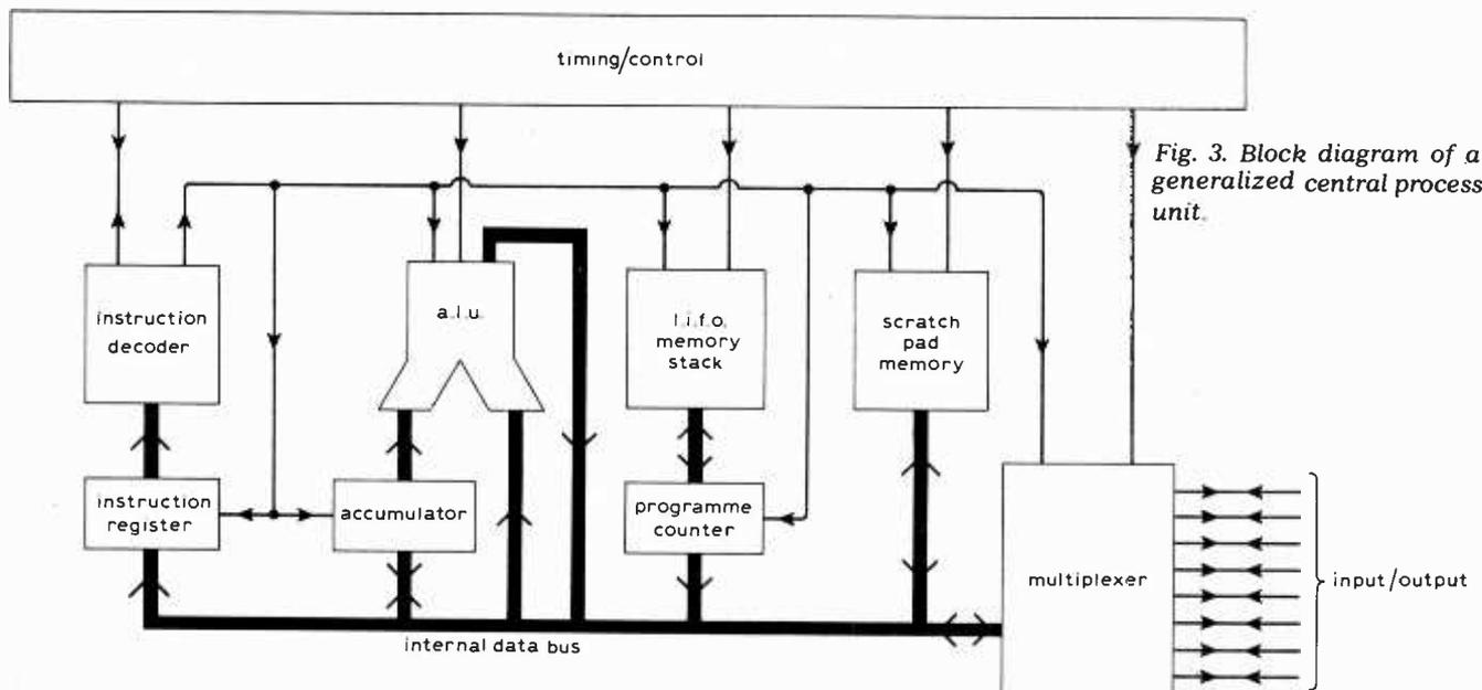
Fig. 3. Block diagram of a generalized central processor unit.
