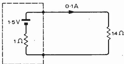
Fig. 1 Electrical circuit analogy for a permanent magnet with negative reluctance: the box can be said to contain a resistance of -14 ohms.
