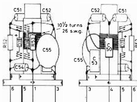
the coil turns are held tightly in position. Completely coat the coil in cement (Denfix) and leave overnight to dry thoroughly.
