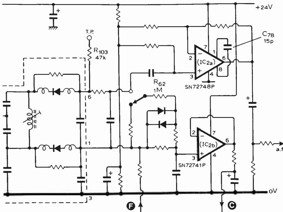
Fig. 14. Changes and corrections to the sound/a.f.c. circuit given in Fig. 2 (Part 1). Separate components in the  $IC_{2a}$  and  $IC_{2b}$  positions take advantage of better noise performance available from the SN72748P acting as the audio output amplifier.
