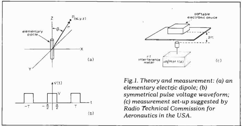
Fig. 1. Theory and measurement: (a) an elementary electric dipole; (b) symmetrical pulse voltage waveform; (c) measurement set-up suggested by Radio Technical Commission for Aeronautics in the USA.
