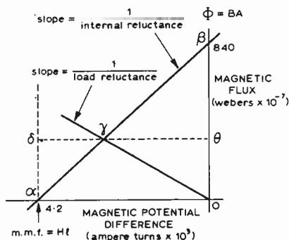
Fig. 2 Plot of magnetic flux against magnetic potential difference for a ceramic magnetic material.
