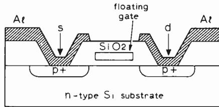
Fig. 7. Cross section through an idealised f.a.m.o.s. transistor.
