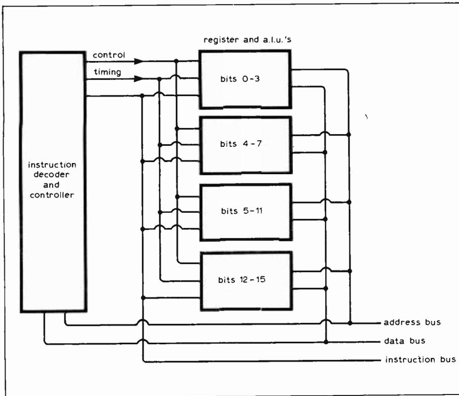
Fig. 4. "Bit slice" c.p.u. configuration.
