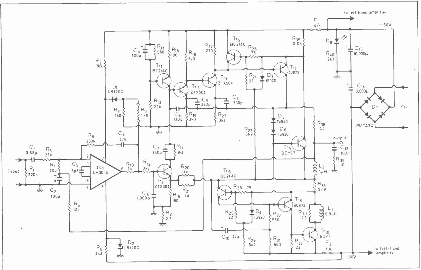
Fig. 4. Full circuit diagram. Resistor  $R_2$  is a protective connection provided to ensure earth continuity in the event that  $Tr_2$  and its associated component panel are disconnected from the common earth chassis.
