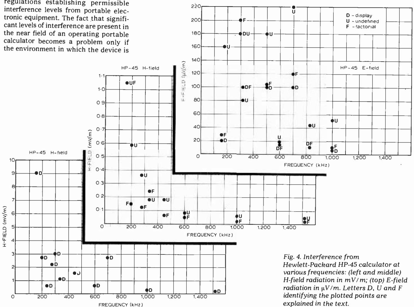
Fig. 4. Interference from Hewlett-Packard HP-45 calculator at various frequencies: (left and middle) H-field radiation in  $mV/m$ ; (top) E-field radiation in  $\mu V/m$ . Letters D, U and F identifying the plotted points are explained in the text.
