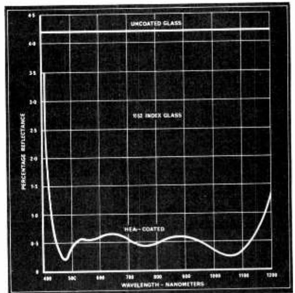
Comparison between OCLI Wide Band 'HEA'-coated and uncoated 1.52 index glass (measured performance).
