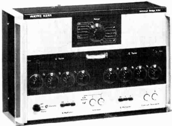
One part in one thousand is the accuracy of Universal Bridge B224 from 10 ohms to 1 gigohm, 0.1pF to 10 microfarads and 1 nanomho to 100 millimhos. Monitor its 1592Hz source frequency and also get 0.1% from 1mH to 10kH. With reducing accuracy, coverage extends above and below the ranges quoted, on R, C, G and L. Resistive and reactive terms read simultaneously. Sockets for 200Hz — 50kHz operation. Internal rechargeable battery. Many other valuable features detailed in Data Sheet B224.
