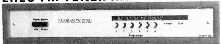
**Brief Spec.** Tuning range 88—104MHz. 20dB mono quieting @ 0.75µV. Image rejection — 70dB. IF rejection—85dB. THD typically 0.4%. IC stabilized PSU and LED tuning indicators. Push-button tuning and AFC unit. Choice of either mono or stereo with a choice of stereo decoders.
