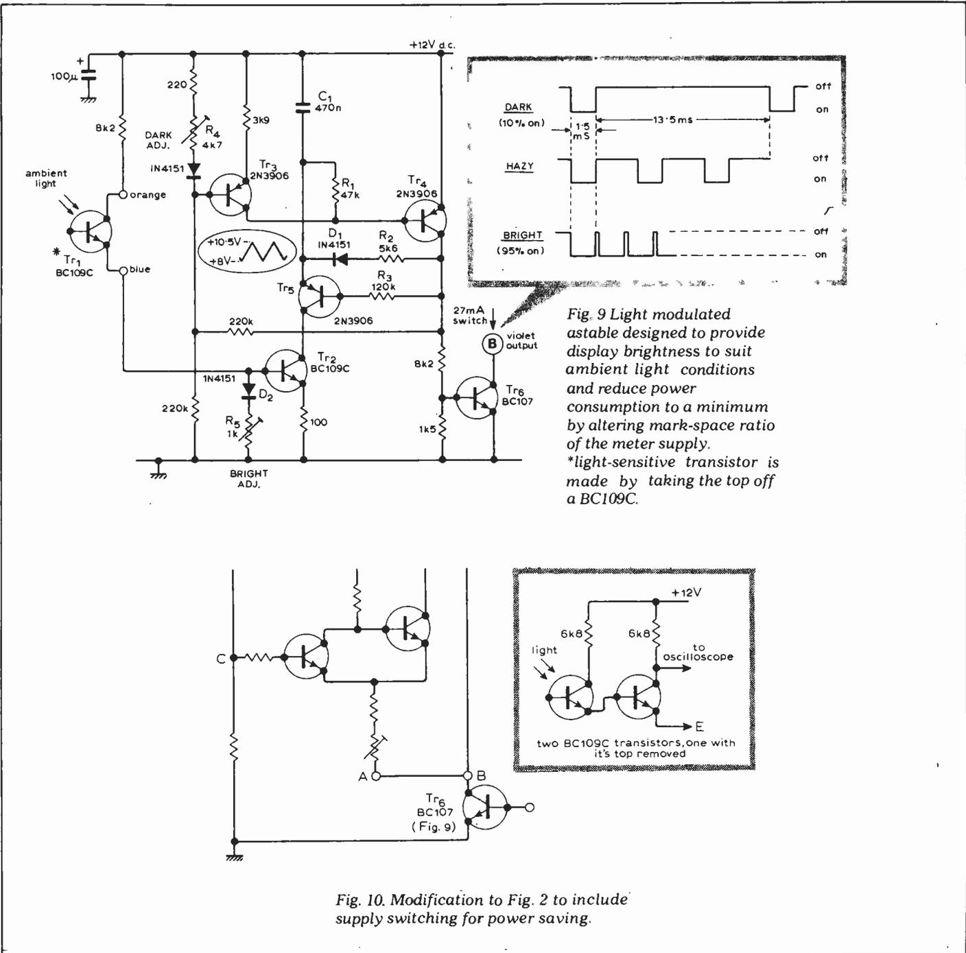
Fig. 10. Modification to Fig. 2 to include supply switching for power saving.
