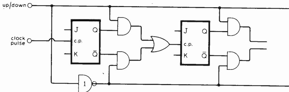
Fig. 10. Reversible count logic—single clock.
