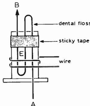
Then pulling end A will tighten the finish of the coil and pulling end B will tighten the start. It may help to attach the dental floss to the end with double sided sticky tape to start the coil. This makes a very firm coil.
