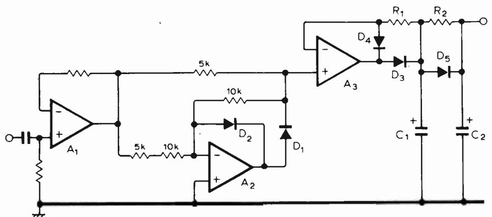
**Fig. 5 Complete schematic of the compander.** Op-amps are assumed to have  $\pm 15V$  power supplies. For best performance amplifier  $A_1$  should have separately decoupled supplies. The  $10k\Omega$  resistor in the compensation should be referred to the negative supply.
