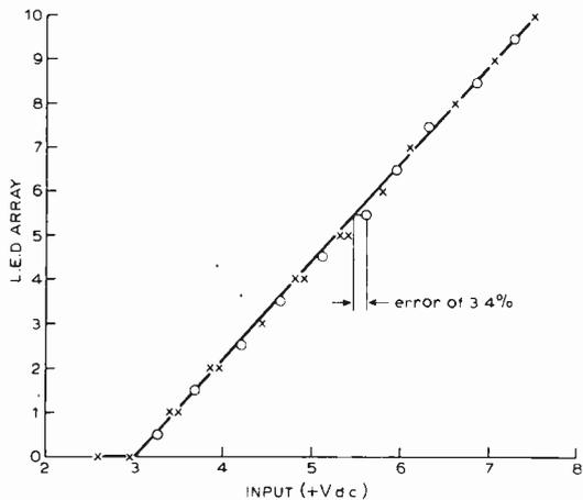
Fig. 3. Calibration curve for the display in Fig. 2 showing the input voltages required to light l.e.ds numbers 0 to 10. Points X represent a single l.e.d. when lit, points O represent two adjacent l.e.ds when equally bright; e.g. at an input of 5.6V both l.e.ds 5 and 6 are equally on and the error is about 0.12V. Full scale is 3.5V d.c. therefore error at full scale is  $0.12 \times 100/3.5 = 3.4\%$
