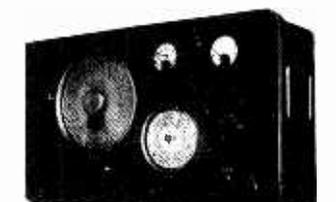
**EMF 1066 SIGNAL GENERATOR.** Freq. 10 470MHz with attenuator EMF from 50Ω square -6dB Price on application
