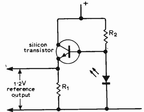
Fig. 3. A reference voltage using a gallium phosphide l.e.d.
