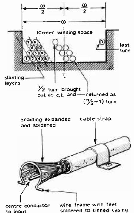
bending a small piece of wire (about 20 s.w.g.) into an omega-shape and soldering this to the tinned cover. The braid end is then pulled over and round the frame as shown and then soldered, allowing small amounts of solder to run over the braid to strengthen the hood.
