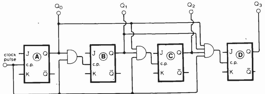
Fig. 6. Four stage synchronous clocking.
