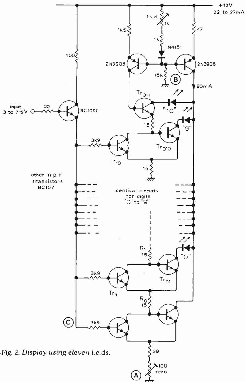
Fig. 2. Display using eleven l.e.ds.
