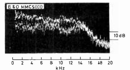
Fig. 12. Separation of 10dB or more extends to 13kHz in the case of the B&O mmc5000 cartridge.
