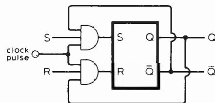
Fig. 2. Simple back-priming of RS flip-flop.
