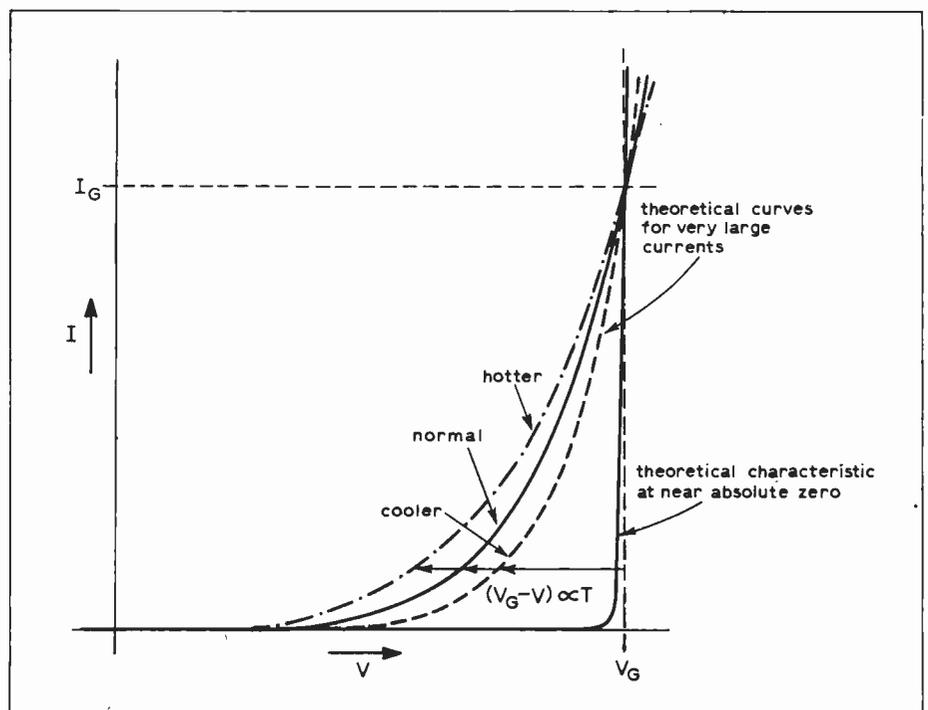
voltages below  $V_G$  and then turn on unlimited forward current, with an almost superconducting slope resistance, at that voltage. As the temperature is increased, the familiar exponential characteristic appears and expands linearly away from the  $V_G$  ordinate.
