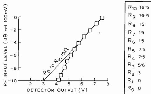
Fig. 4. Graph showing how the selection of the resistors  $R_0$  to  $R_{10}$  allows the circuit in Fig. 2 to be used for a non-linear application; in this case an r.f. calibrated receiver.
