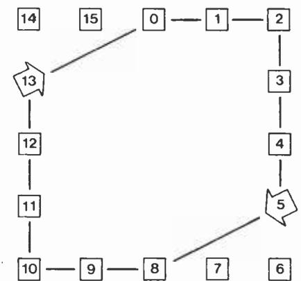
Fig. 5. Divide-by-twelve sequence diagram.
