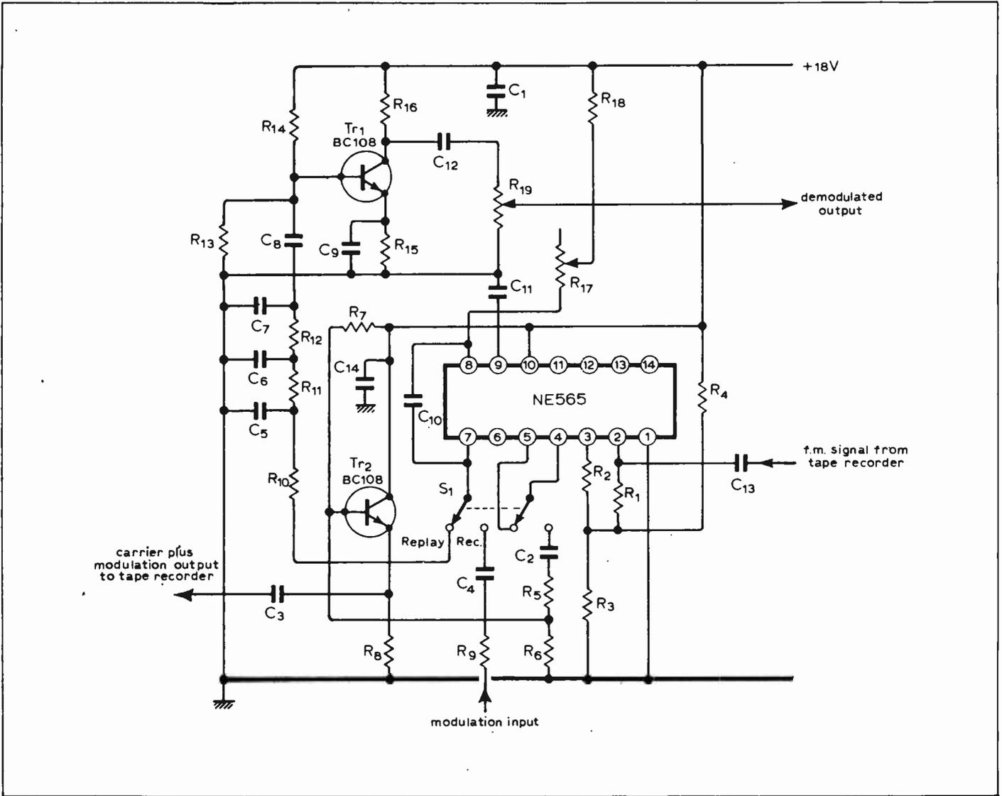
Fig. 2. Practical circuit for modulator / demodulator using one p.l.l. and a d.p.d.t. switch. Tr<sub>1</sub> provides an overall gain of 0dB in the replay mode, and Tr<sub>2</sub> isolates the v.c.o. output in the record mode.
