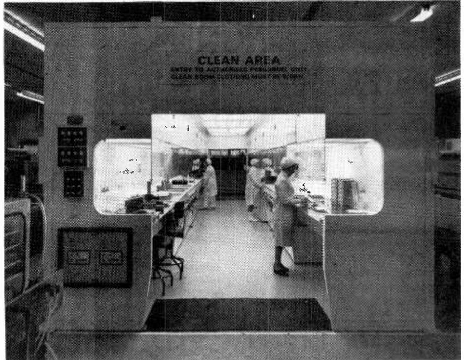
Clean room at Mullard Hazel Grove, a Philips Industries semiconductor components factory. Instead of having large open areas serviced with cleaned and filtered air, the working stations are fitted into modules that can be put together to form an open-ended tunnel.
