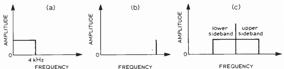
Fig. 2. Spectrum of an a.m. system which is to transmit baseband signals up to 4kHz.
