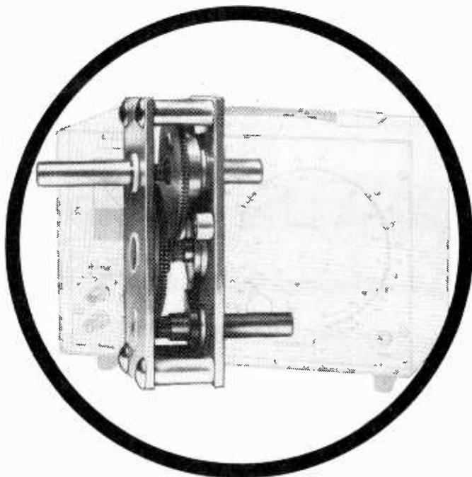
With the precision of the Jackson G10 Gearbox, you get ten turns of input equalling one effective turn of output. This makes the G10 ideal for decimal presentation for analog control. The Gear Box itself is packaged within 70mm by 35mm by 19mm. The output shaft drive torque is greater than 700 gm cms. Input shaft diameters are 6mm. All the gears are fully anti-backlash loaded. The Jackson G10, the compact, versatile gearbox.
