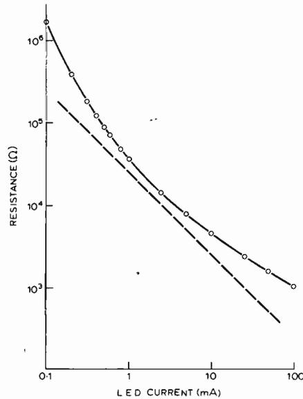
Fig. 2 Curve of photocell resistance versus i.e.d. current for a Clairex CL904N photocell when illuminated by a red i.e.d. The unbroken line is drawn through the experimental points. The dashed line represents ideal behaviour.
