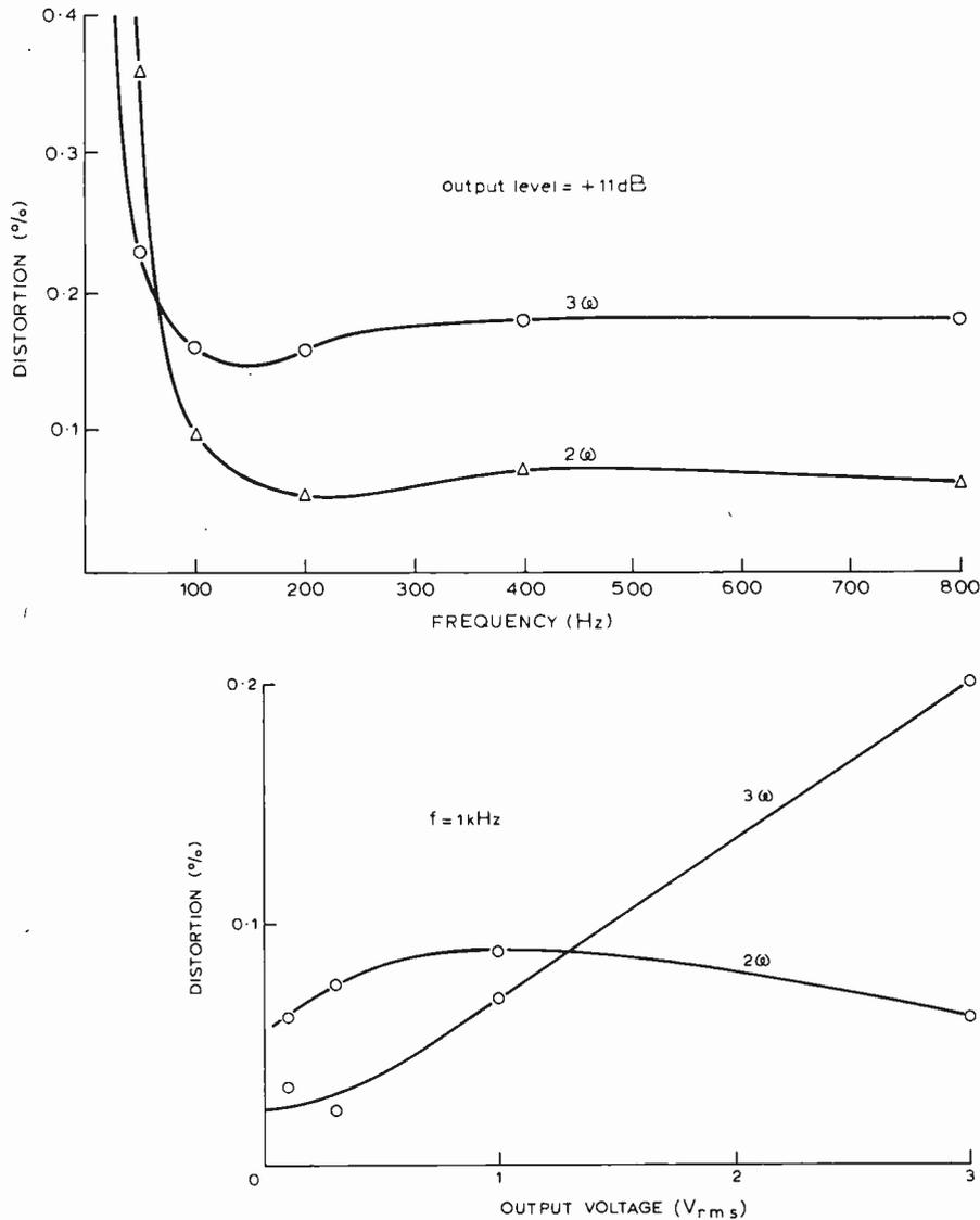
Fig. 9 Distortion of the compressor versus frequency for an input level of +10dB. Curves are substantially constant beyond 800Hz with a small increase beginning beyond 10kHz.
