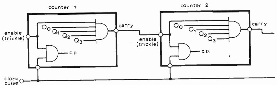
Fig. 8. Trickle group carry scheme —skeleton logic.
