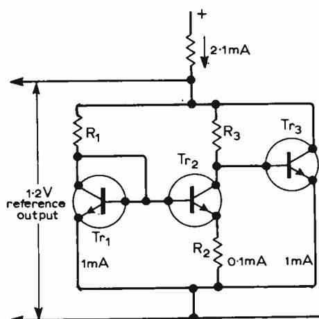
Fig. 2. The Widlar diode circuit.
