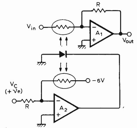
Fig. 3 Photocells and a controlling i.e.d. are used here as a multiplier using a concept similar to that shown in Fig. 1 (b). For this circuit  $V_{out} = V_c V_{in}/6$ .
