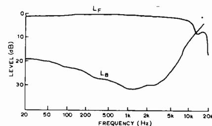
Fig. 13. Front-back separation measured using test bench generator. Sum signal delayed by 45μs with reference to the carrier signal.
