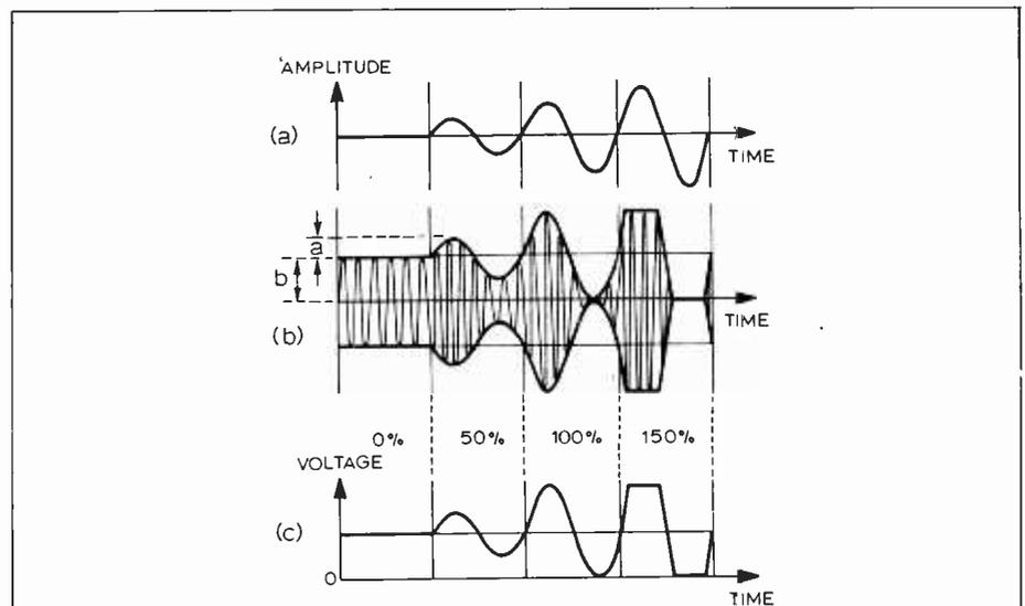
Fig. 1. Illustrating the meaning of modulation depth in an amplitude modulated system with examples of the waveforms expected for 0%, 50%, 100% and more than 100% modulation.
