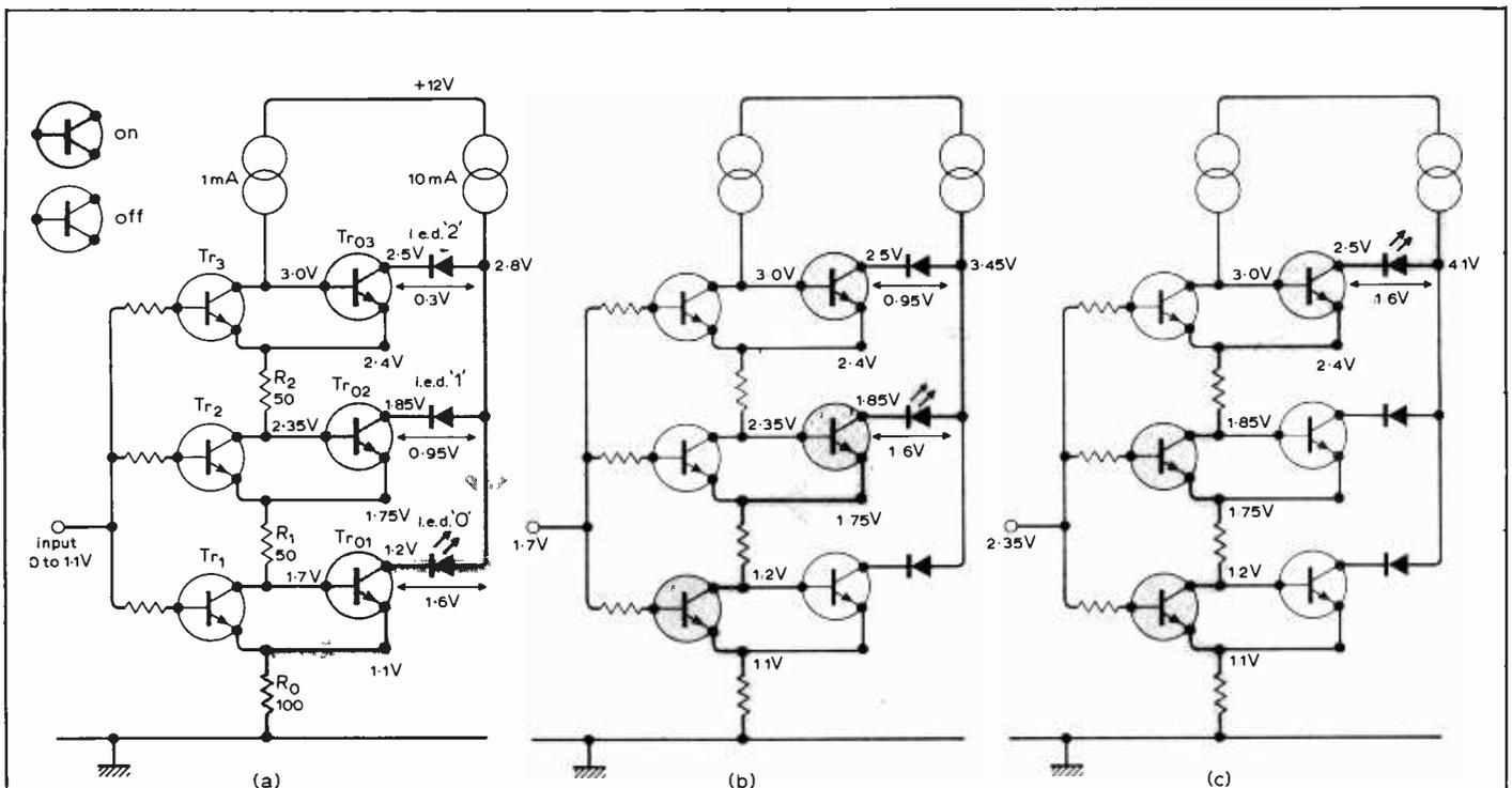
Fig. 1 Circuit for an I.e.d. array display for use as an output level meter, e.g. signal strength meter, showing how the I.e.ds switch on in sequence as the input voltage is increased. Voltage conditions assume  $V_{be}$  of 0.6V and  $V_{ce}$  of 0.1V.
