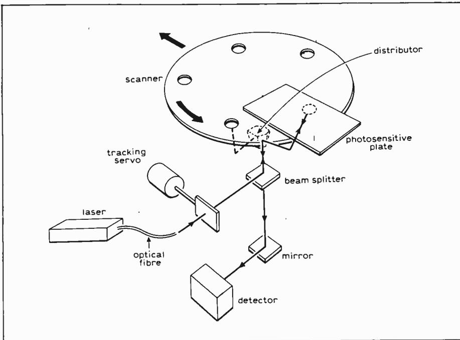
In the digital video record system, the 5×7in record is stationary and the scanner moves. A distributing prism acts to switch the beam from the end of one track to the start of the next.
