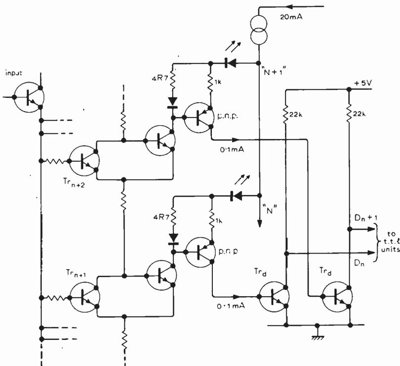
Fig. 8. Typical modification to Fig. 2 providing digital outputs arranged to drive a digital display of 1½ digits.
