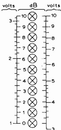
Fig. 6. Typical display array for l.e.ds showing 0 to 10dB and equivalent voltage levels.
