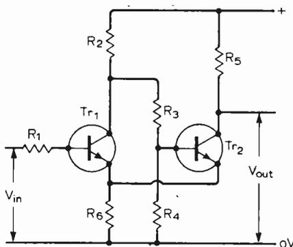
Fig. 1. Common form of non-inverting Schmitt trigger.
