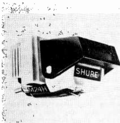
The capability of playing CD-4 records is claimed for this Shure M24H four-channel cartridge. The stylus tip is hyperbolic and the low stylus mass of 0.39mg enables the tracking force to be as little as 1 to 1.5g.
