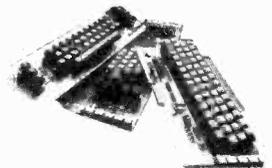
ASCII Coded TTL compatible 4-bank alphanumeric reed-switch keyboards with ROM encoder chip, strobed output, two-key rollover and debounce. Standard 7-bit ASCII code (no parity). Supplied complete with circuit diagrams and code chart
