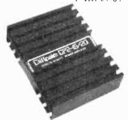
**Description:** This module is designed to give either a 20W + 20W stereo amplifier or alternatively a 40W single channel. It has built-in protection against accidental reversed supply connection and it incorporates a thermal shut-down facility to prevent over-dissipation. No external components are required.
