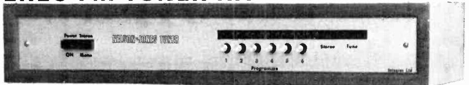
**Brief Spec.** Tuning range 88—104MHz. 20dB mono quieting @ 0.75 $\mu$ V. Image rejection — 70dB. IF rejection—85dB. THD typically 0.4% IC stabilized PSU and LED tuning indicators. Push-button tuning and AFC unit. Choice of either mono or stereo with a choice of stereo decoders.
