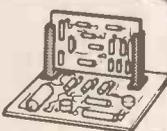
**P.C. BOARD SPACERS** are simple to fit, one-piece mouldings for use with p.c. boards. They have a self retaining shank for fastening into panels and a T-shaped anchor for securing p.c. boards of 0.062" thickness. They have good resistance to vibration and are suitable for board-to-board or board-to-chassis use.
