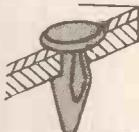
**PLASTIC HOLE PLUGS** are quick, inexpensive means of plugging unwanted holes. Hole Plugs keep out dust, dirt and moisture. Attractively shaped heads give a neat finish. The snap action grip of the Hole Plug makes a vibration resistant seal. Hole Plugs are made from nylon and are non-corrosive.
