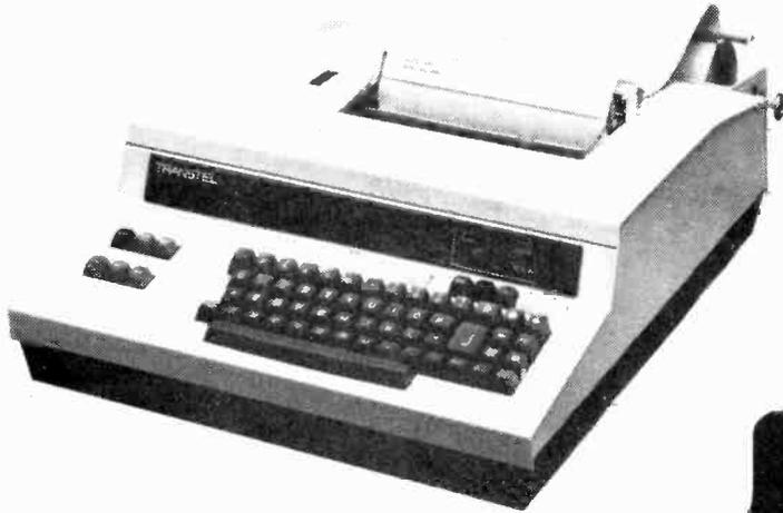
The Transtel 315 word processing communications terminal includes all the best developments and refinements that have been introduced in a decade of teleprinter technology.
