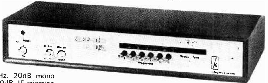
**Brief Spec.** Tuning range 88–104MHz. 20dB mono quieting @ 0.75 $\mu$ V. Image rejection – 70dB. IF rejection – 85dB. THD typically 0.4%. IC stabilized PSU and LED tuning indicators. Push-button tuning and AFC unit. Choice of either mono or stereo with a choice of stereo decoders.
