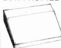
1mm Grey Aluminium panel sits recessed into front of console base, which is moulded in Orange, Blue, Black or Grey ABS and sits on 4 self adhesive rubber feet. Incorporating guides for holding 1.5mm thick pcb, the base also has stand-off bosses for supporting small sub-assemblies etc. and ventilation slots. Front panel is held by 4 screws which run into integral brass bushes.
