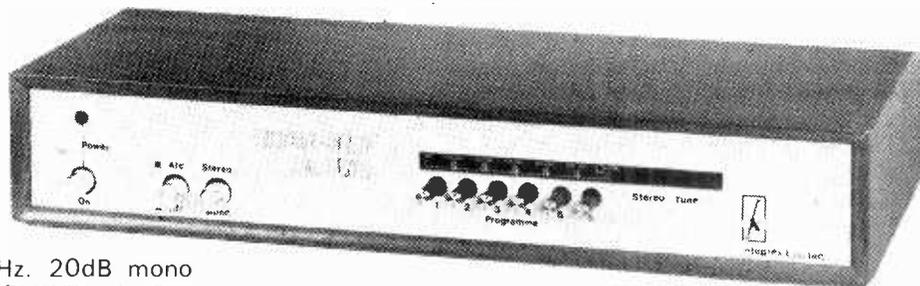
**Brief Spec.** Tuning range 88–104MHz. 20dB mono quieting @ 0.75µV. Image rejection – 70dB. IF rejection – 85dB. THD typically 0.4%. IC stabilized PSU and LED tuning indicators. Push-button tuning and AFC unit. Choice of either mono or stereo with a choice of stereo decoders.
