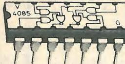
STICKIES are printed self-adhesive labels that stick to the top of ICs. They turn a board-full of ICs into a working circuit diagram! See at a glance where to place your soldering iron or test probe. Use STICKIES for building and de-bugging prototypes, fault-finding, experimenting, teaching — even designing PCB layouts.
