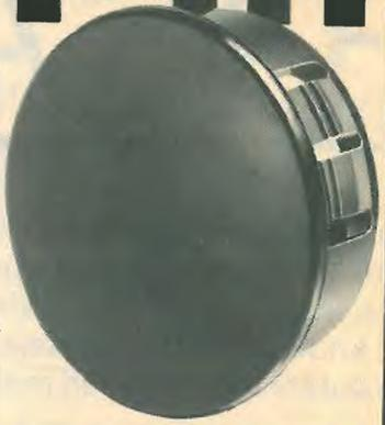
seal unwanted holes neatly, quickly and easily. Snap-lock into panels with fingertip pressure. Low cost. 20 sizes for holes from 3/16" to 2".
