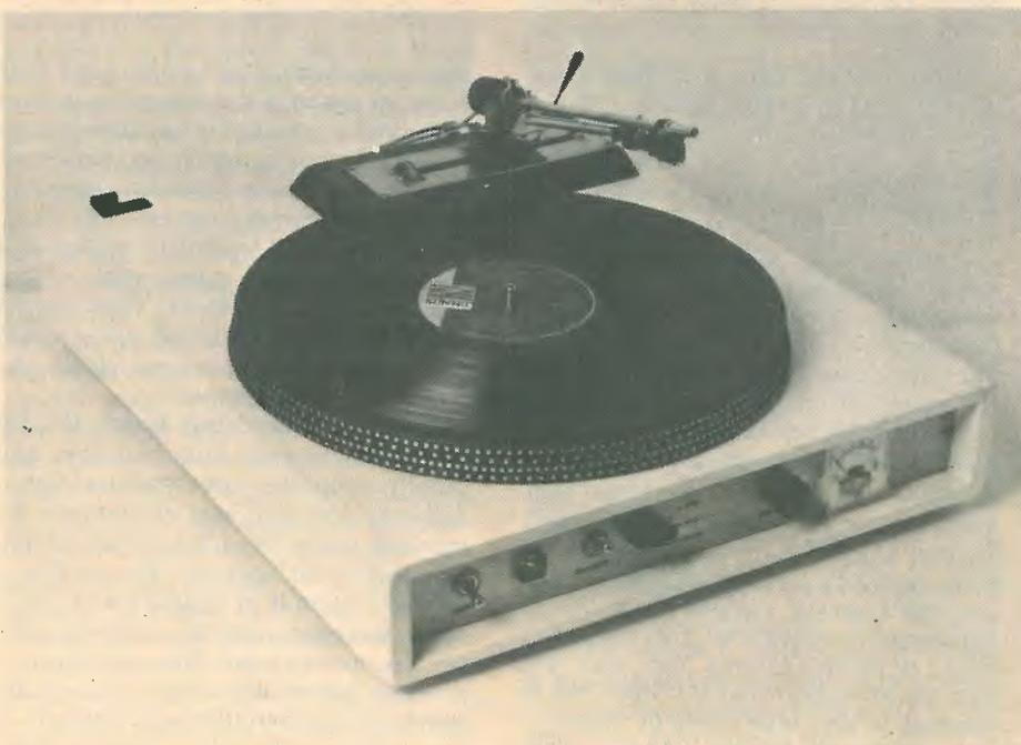
*Arm is cued by lowering hinged mounting platform; see part 2 for details. Meter is an essential part of design and indicates correct operation of the servo.*
