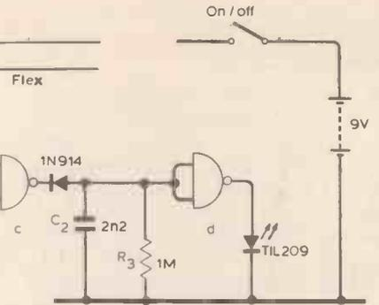
The oscillator formed by gates a and b feeds pulses into the neutral wire which induce a signal into the line. If the fuse is intact the induced signal is amplified by gate c, rectified and used to charge  $C_2$ . The voltage on  $C_2$  is amplified and used to drive the l.e.d. The fuse tester can be checked by touching the contacts with a finger.
