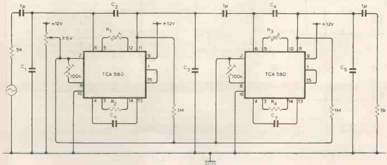
tions. On the left-hand page the pole/zero realisation is accomplished by using a triple op-amp arrangement based on a synthesis technique given by Huelsman<sup>5</sup>. On the right-hand page an LC tabulated design<sup>4</sup> is realised using gyrators<sup>6</sup>.
