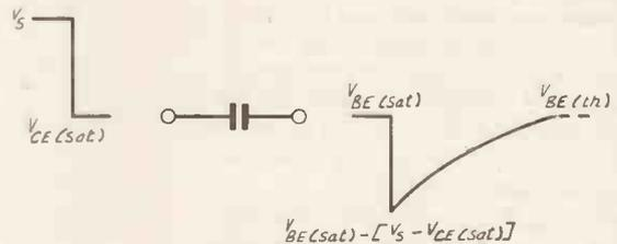
The waveform sketch is of a collector waveform falling from  $V_s$  to  $V_{CE(sat)}$ . Just prior to that instant the other base is at  $V_{BE(sat)}$  and is driven down by the same amount. When the base recovers to  $V_{BE(th)}$  the other transistor takes over the second half-cycle.
