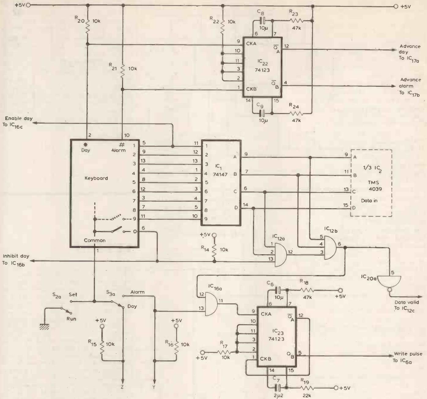
Fig. 5. Keyboard encoder and memory input circuit.
