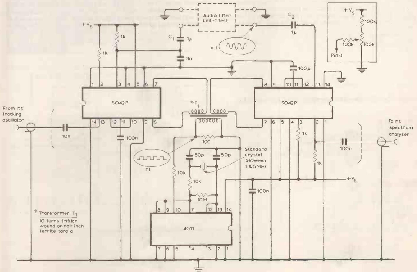
The unit shown in Fig. 1 provides a simple means of shifting an r.f. signal down to audio frequencies, and then up again to the same radio frequency. Operation is centred about a frequency determined by a c.m.o.s. crystal oscillator. This has good stability and its frequency is easily changed. The centre frequency can be between 1 and 5 MHz and is determined either by a crystal one has to hand or by the frequency required to match a receiver system being measured.
