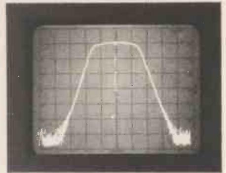
Fig. 7. Radio receiver selectivity response measurement, a car radio with  $100\mu\text{V}$  input at 1MHz. (vertical scale 10dB/div. relative to 1W; horizontal scale 1kHz/div. relative to 1MHz centre frequency).
