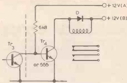
Fig. 8. Normal practice is to have a relay energized so that power failure can be indicated. For a high security area a 555 timer (fed by  $Tr_4$  or with  $Tr_3$  collector connected to pin 2) could be arranged to short a relay hold-off after a short interval.
