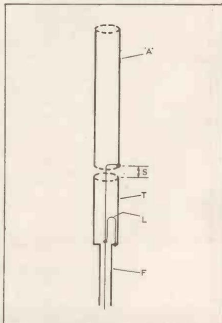
Fig. 1. Basic aerial, a half-wave element A and coaxial impedance transformer T. Loop inductor to augment impedance ratio obtainable.
