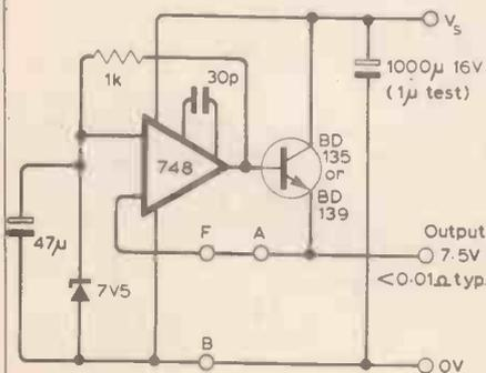
**Table 3. Use of op-amp as shown in Fig. 3 improves ripple rejection.**
