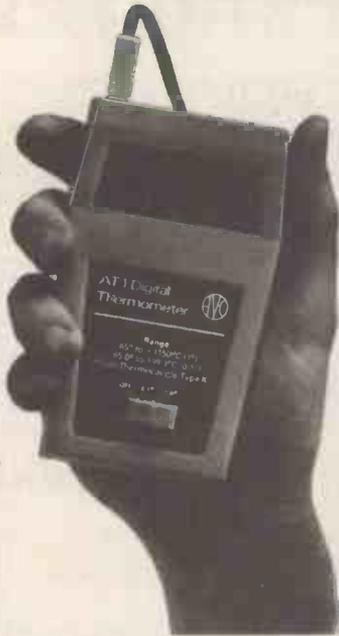
Now you can get Avo quality in digital thermometers. There are two units to choose from. The AT1, a battery operated, portable unit which is fast, accurate and easy to use; and the AT2, a battery/mains bench top model. Both feature large, easy to read displays, and together cover a wide temperature range from  $-65^{\circ}$  to  $+1200^{\circ}\text{C}$ .
