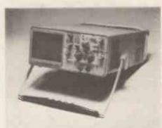
**TEKTRONIX** Storage Scope 434 Dual Trace. 25MHz
