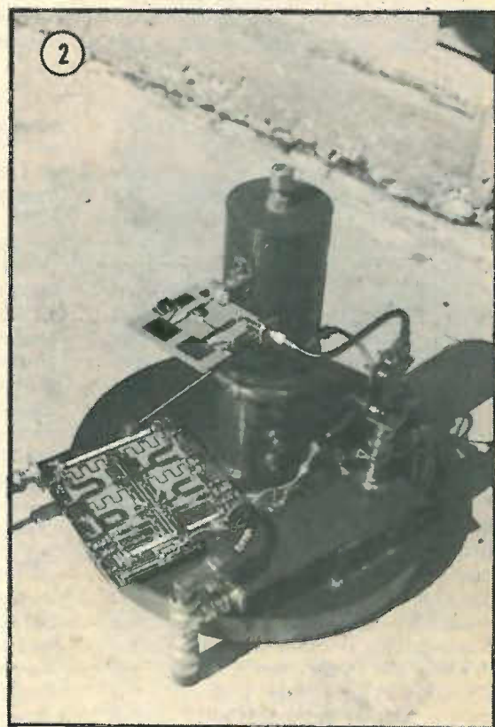
Fig. 1. Sheffield terminal's 8ft dish antenna with 4GHz feed in position. Fig. 2. 4GHz head unit. The GaAs f.e.t. stage is mounted near the top. Fig. 3. 11-12GHz feed system mounted at the prime focus point.
