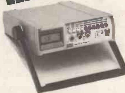
**8050A** 4 ½ Digit LCD DMM with true RMS on AC volts and current DC volts 200mV-1KV, 10µV resolution AC volts. 200mV-750V, 10µV resolution. DC/AC current 200µA-2A, 0.01µA resolution resistance 200Ω-20MΩ, 0.01Ω resolution. Also reads dB direct referenced to 16 stored impedances. Conductance ranges 2mS and 200nS. **£199** mains model **£239** mains battery.
