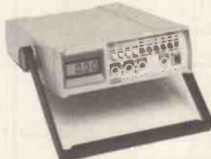
**8010A 3 1/2 Digit LCD DMM** Same spec as 8012A plus a 10Amp AC/DC current range, but no low resistance range. **£159.00 mains model £179.00 mains battery.**
