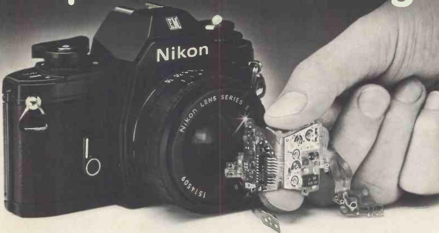
When a solder medium for the microprocessor-based circuitry of the new Nikon EM camera was needed, a Multicore Oxide-Free Solder Cream was chosen.
