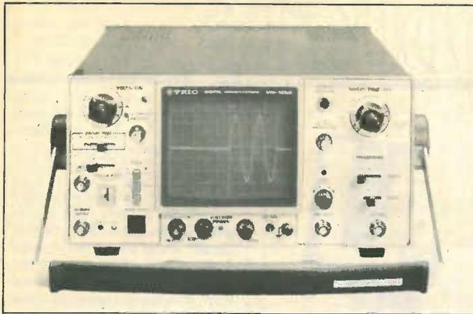
the cabinet. The MS-1650 incorporates a 118×98mm c.r.t., weighs only 9kg, measures 284×138×400mm, and costs £1440 with a two year guarantee. House of Instruments, 34/36 High St, Saffron Walden, Essex CB10 1EP.
