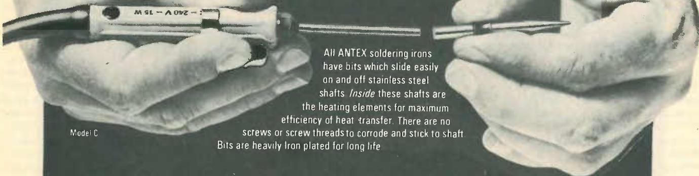
All ANTEX soldering irons have bits which slide easily on and off stainless steel shafts. Inside these shafts are the heating elements for maximum efficiency of heat transfer. There are no screws or screw threads to corrode and stick to shaft. Bits are heavily Iron plated for long life.
