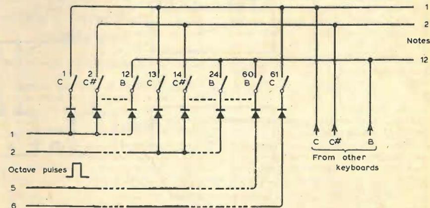
Fig. 2. Identical notes are wired together on one side of matrix, with all 12 notes in each octave wired together via diodes on the other side.
