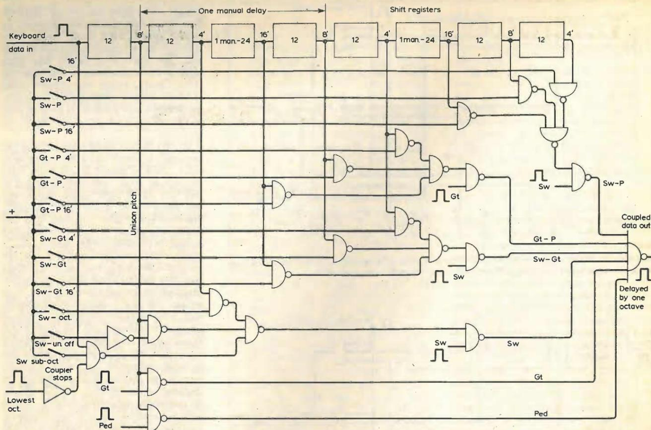
Fig. 5. Extra manual delays are required during scanning to avoid intrusion of pulses into next pedal scan period. Diagram shows coupling system for two-manual church organ.
