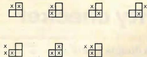
Fig. 3. Two, three and four errors, distributed as at (a) are detected, since the parity check gives an odd result at some point as the data stream passes the checking area. The pattern at (b) is not detected, because the parity remains even at any position.
