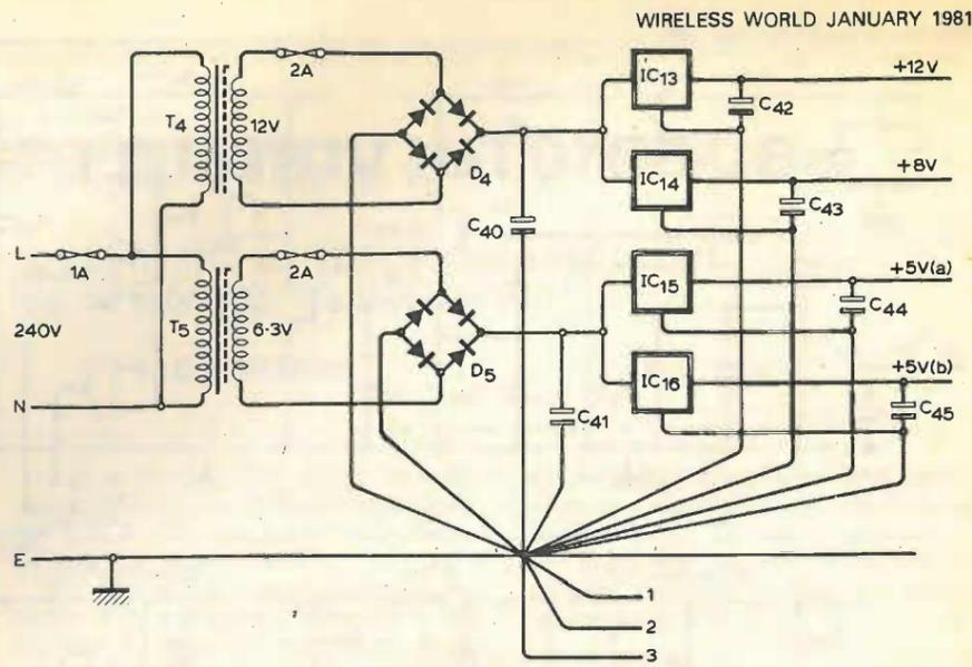
Fig. 6. Four rail power supply.
