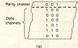
Fig. 1. Parity bits in serial (a) and parallel (b) data channels.
