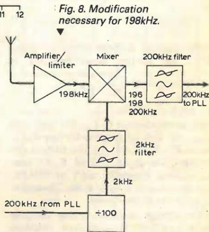
Fig. 8. Modification necessary for 198kHz.
