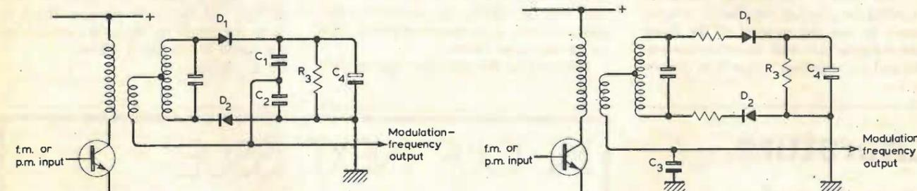
Fig. 10. The circuit of Fig. 9 (b) modified so as to give a measure of a.m. rejection. Fig. 11. An unbalanced ratio-detector circuit with a single reservoir capacitor  $C_3$ .
