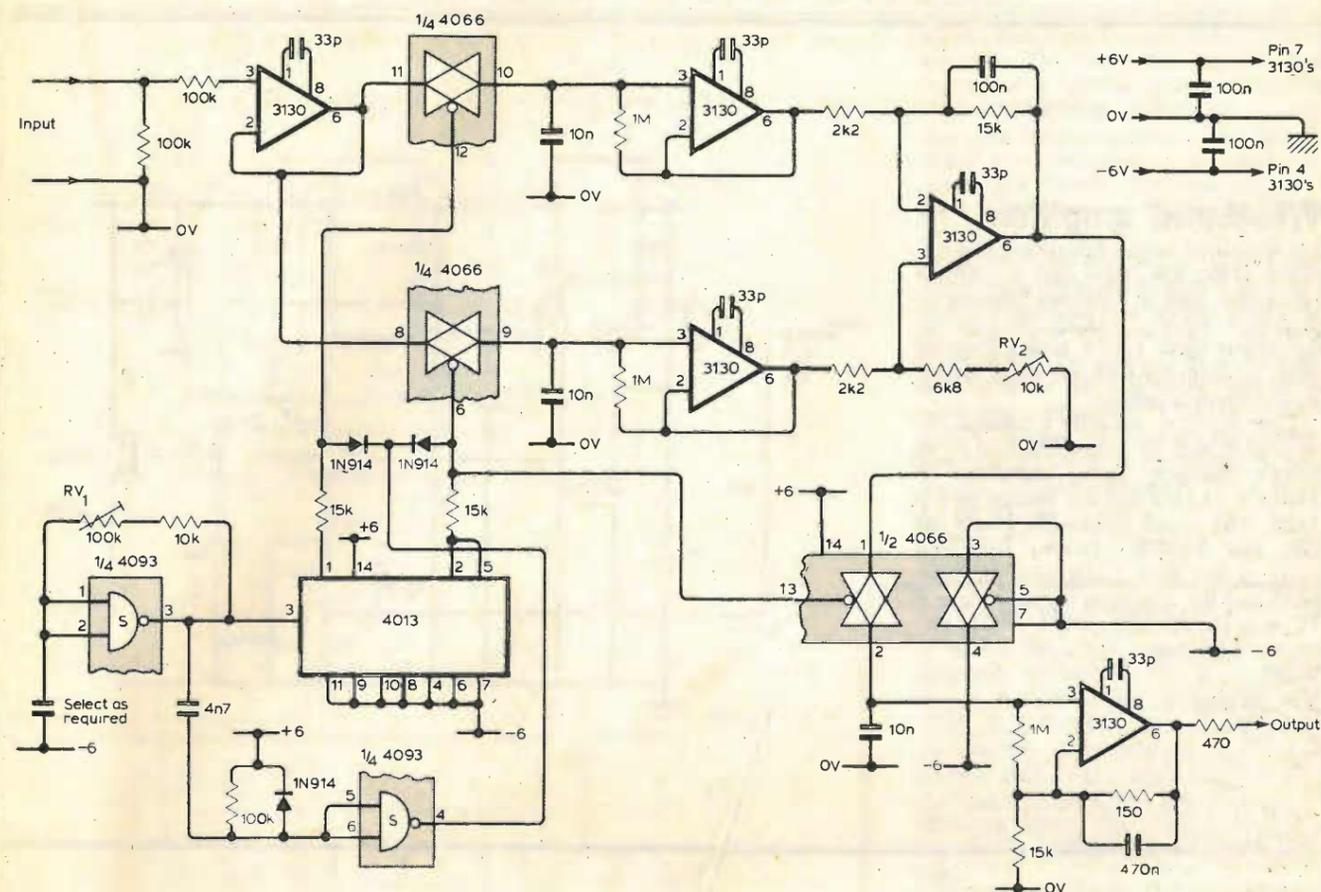
Fig. 4. Complete circuit diagram. 4013 is a dual, D-type flip-flop.
