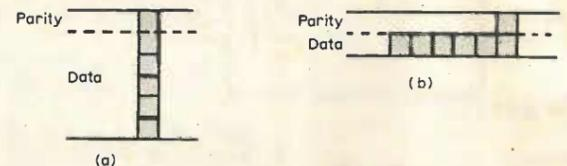
Fig. 2. Checking area of a parallel channel can be 'bent' to enable one parity bit to check serial data as in (b).
