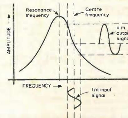
Fig. 2. Simple f.m. slope detector.
