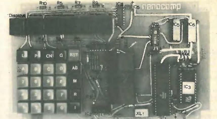
Fig. 4. Assembled printed circuit board and layout details. The board measures 200 x 120mm.
