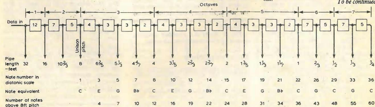
Fig. 6. Shift register can be tapped at necessary increments and simple gating controls appropriate frequencies from generators or pipes. (See part 2, Fig. 7, for simplified control system.)
