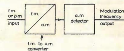
Fig. 1. Block diagram illustrating the form of a number of types of f.m. detector.
