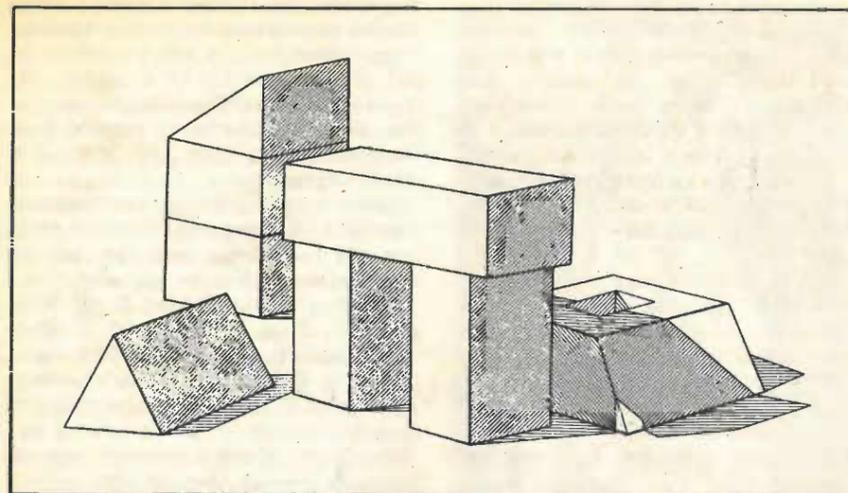
Fig. 2. A line drawing correctly interpreted by David Waltz's program for computer vision.
