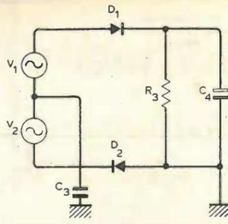
Fig. 12. Equivalent circuit of Fig. 11.
