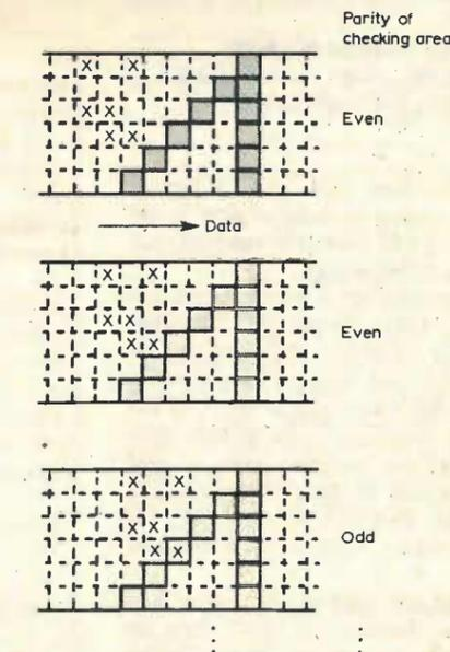
Fig. 6. Operation of the parity check of Fig. 5.
