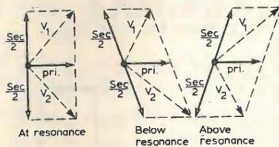
Fig. 6. Vector diagram for the circuit of Fig. 5 showing how the voltages  $V_1$  and  $V_2$  applied to the diodes vary with frequency.
