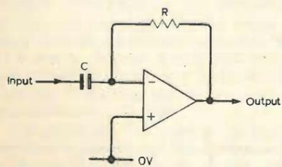
Fig. 1. Ordinary type of RC differentiator - useless for very long time intervals.
