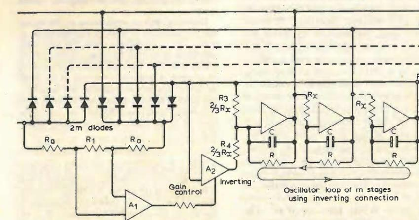
Fig. 1. Oscillator of  $m$  phases.
