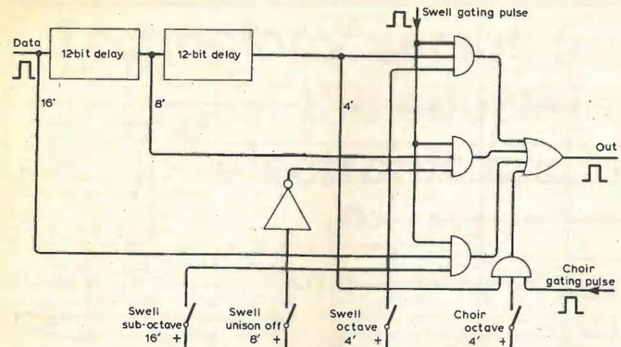
Fig. 3. As scanning is sequential note-by-note and octave-by-octave, 12 pulses separate keys an octave apart, and octave coupling is achieved using 12 pulse data delays.
