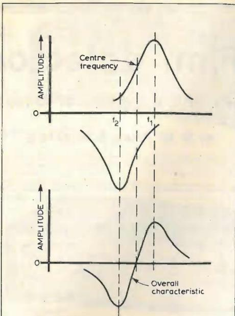
Fig. 4. Derivation of overall characteristic of Round-Travis f.m. detector.
