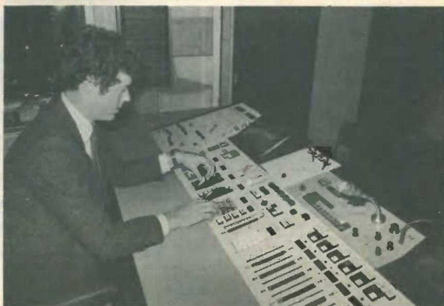
Studios 7 and 8 at BBC Television Centre are now being lit by a microprocessor-controlled system developed by Thornlite in collaboration with the BBC's Capital Projects Department. The unit can control up to 500 studio lights and use nine Motorola 68000 microprocessors.
