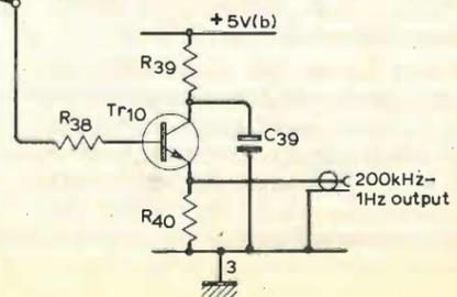
from the receiver. To minimize signal frequency and counter noise, buffers are included before and after the divider chain in Fig. 5, and separate earth and power supplies are provided. Double-sided printed circuit board is also important with one side used as an earth plane. The power supply in Fig. 6 uses 1A voltage regulators and smoothing capacitors to provide the low noise level necessary for a clean output signal.
