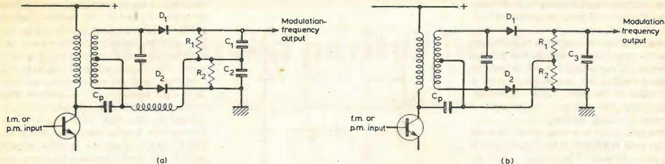
Fig. 8. Two forms of Seeley-Foster circuit using a capacitive link between primary and secondary windings.
