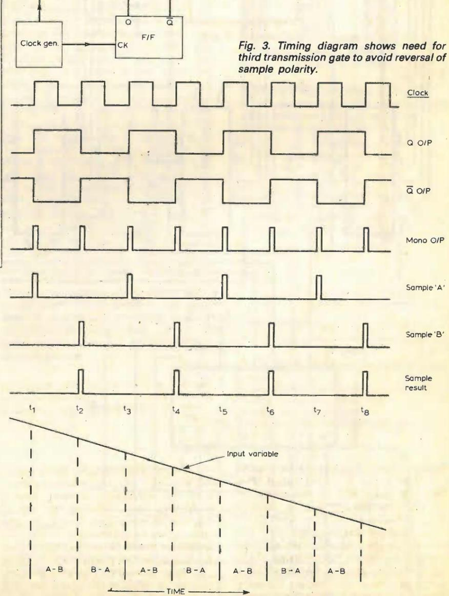
Fig. 3. Timing diagram shows need for third transmission gate to avoid reversal of sample polarity.
