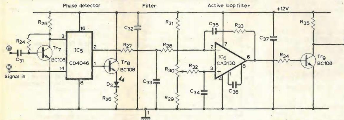
Fig. 3. Phase locked 10MHz oscillator.
