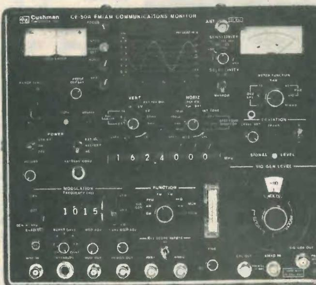
**Compact, versatile field service monitors for two-way radio maintenance**
