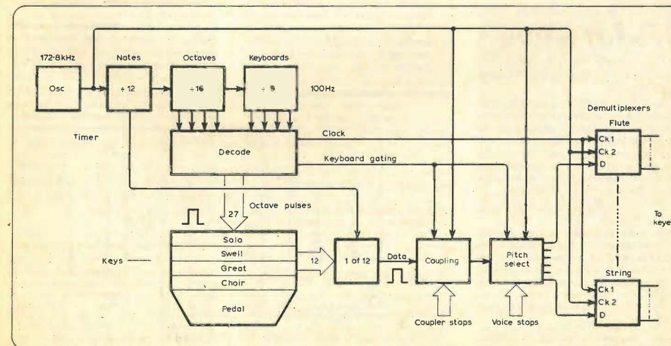
Fig 1. Sequential scanning of keyboard matrix in electronic or pipe organs reduces wiring by sending data over single wire.
