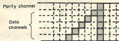
Fig. 5. Suggested checking area for parallel data channel.
