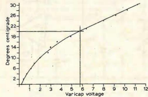
Fig. 7. Varicap voltage versus ambient temperature (loop locked).
