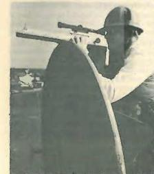
Monitoring of trans-horizon interference provides information needed to improve predictions for transmission/reception quality between earth stations and to study the effects of weather on microwave radio paths. Ron Fitzgerald is seen here lining up an aerial to measure over-the-horizon interference at British Telecom's Martlesham laboratories.
