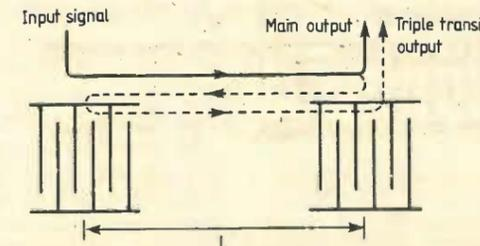
Fig. 8. Triple transit mechanism in s.a.w. devices. The triple transit signal results from successive electrical reflections from the output and input transducers before detection.
