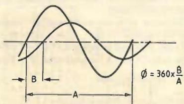
Fig. 2. The zero-crossing method, which can be tricky to set up symmetrically on the screen.
