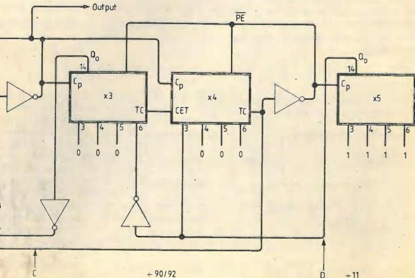
divide by 90 and 92 and, since both are even numbers, the Q<sub>0</sub> output of X3 will, regardless of which division is performed, always alternate between 0 and 1.
