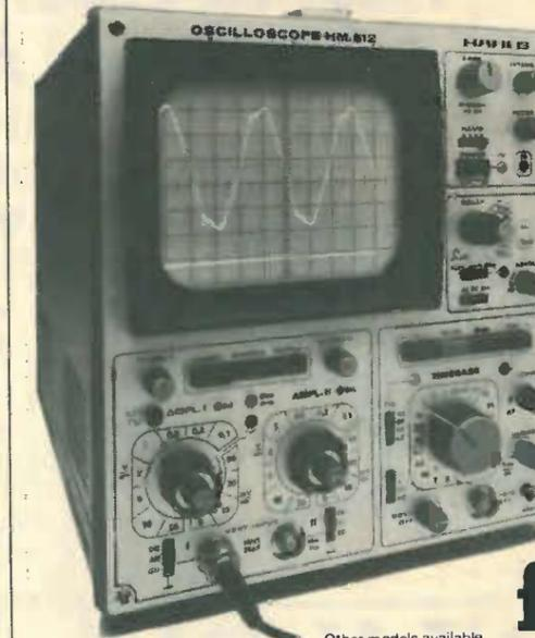
**HM512 Dual Trace Oscilloscope with delayed sweep.**
