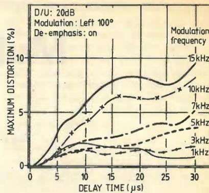
Fig. 3. An example of the relationship between the delay time of an echo and maximum distortion with an aerial direct/unwanted (D/U) ratio of 20 dB for different audio frequencies.
