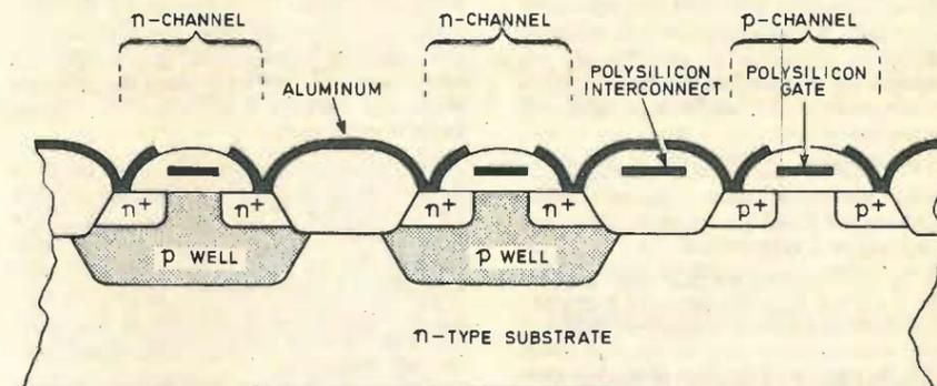
This cross section illustrates the basic principle of ISO-CMOS
