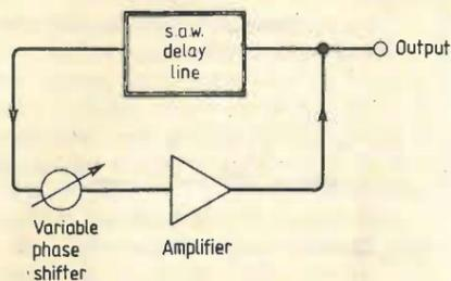
Fig. 17. Delay line oscillator. The circuit will oscillate at a frequency where the total phase shift around the loop is an integral multiple of  $2\pi$ .
