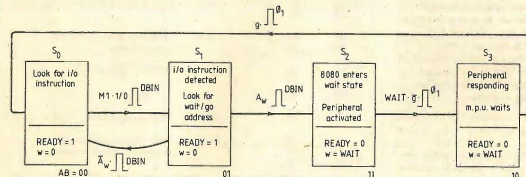
Fig. 8. State diagram of the wait/go logic for the Intel 8080.
