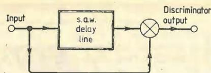
Fig. 16. Delay line discriminator using the good linear phase characteristics of the delay line.
