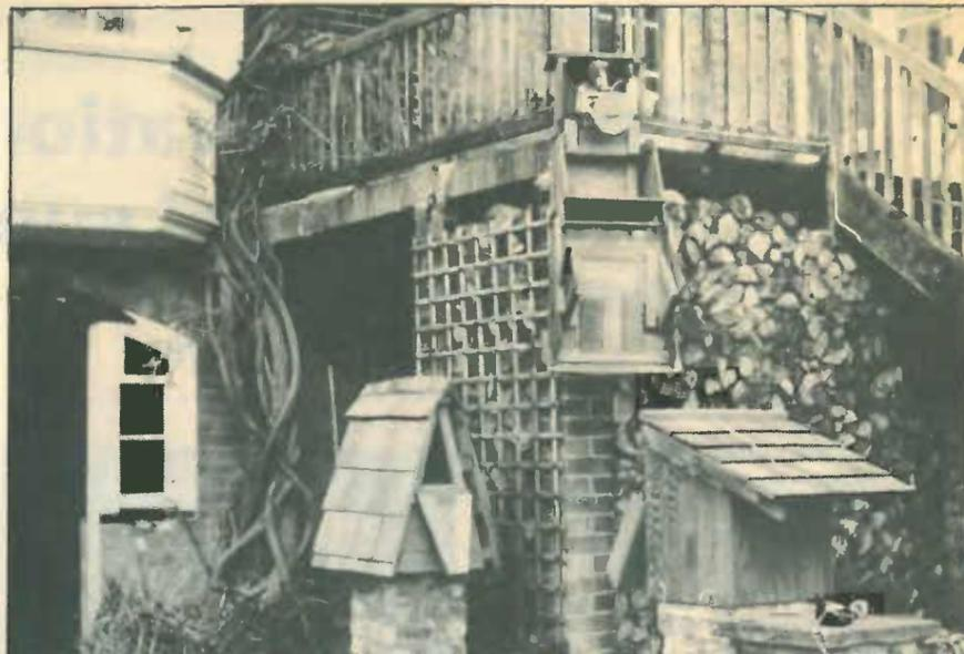
Fig. 7. The spectroheliograph. A mirror (top centre) follows the sun and reflects light towards the second unit (bottom right) which in turn passes through the garden room door off to the left via the lens housing (bottom left).
