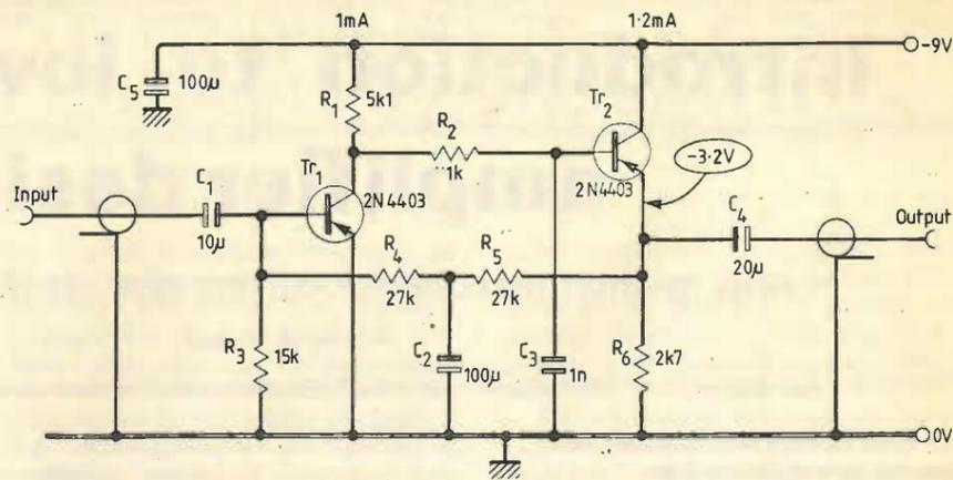
Fig. 2. Instrumentation preamplifier is suitable for microphone use.
