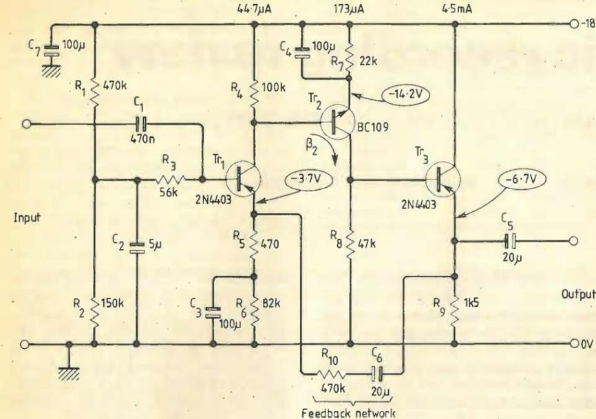
apart from the 2N930. The 2N4403 transistor has been chosen for the practical circuit, and the examples.
