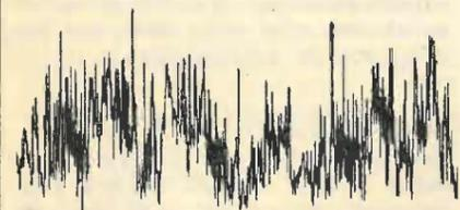
Fig. 4. A ten minute recording of a solar noise storm which occurred on 30 October 1973 at 136MHz.
