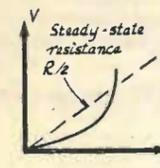
● Networks are used as amplitude-controlled negative feedback. At low amplitudes the steady-state resistance is  $>2R$  for the thermistor or  $<R/2$  for the lamp. Hence feedback  $<1/3$  and for standard Wien type oscillators the amplitude increases. Conversely at high amplitudes the feedback  $>1/3$  and amplitude decays, stabilizing at the steady state level where the negative feedback just balances the positive feedback.
