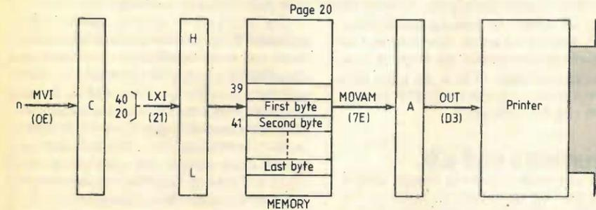
Fig. 14. Programming model for the PRINT problem using the Intel 8080.
