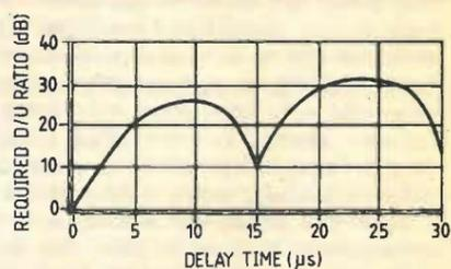
Fig. 5. Relationship between the delay time of an echo and the required D/U ratio if "monkey chatter" crosstalk from an SCA transmission into the main programme is to remain below -55dB (just perceptible). Note that crosstalk into the SCA-programme from the main programme, due to multipath effects, is greater than crosstalk into the main channel.
