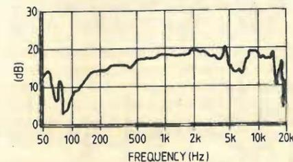
Fig. 1. Basis of modified design is this on-axis speaker response curve.
