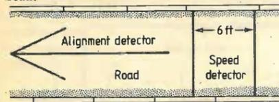
Vehicle speed is computed from the interval in time between the wheels passing over each of the two parallel tubes. Alignment is computed by the driver first of all driving along a straight
