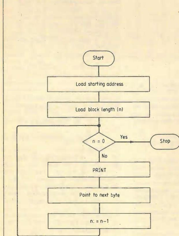
Fig. 11. Step-by-step operation of a wait/go system used to PRINT.
