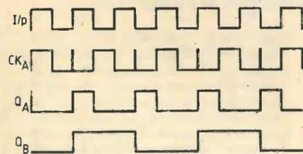
Fig 2(b) Waveforms of divide-by-3 circuit
