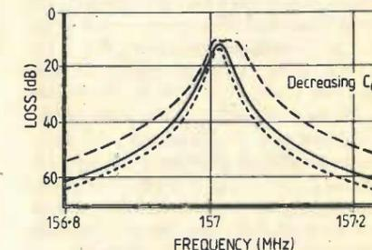
Fig. 14. The effect of varying coupling on s.a.w. resonator response. Note that decreasing the value of the capacitance  $C_c$  increases the coupling and results in a broader bandwidth and lower loss as with conventional filters.
