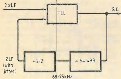
Fig. 3. Sub-carrier frequency (SC) derived from twice line frequency.
