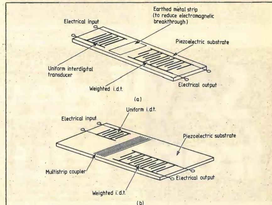
Fig. 7. (a) S.a.w. transversal filter geometry; (b) s.a.w. transversal filter incorporating multistrip coupler to suppress unwanted bulk waves.
