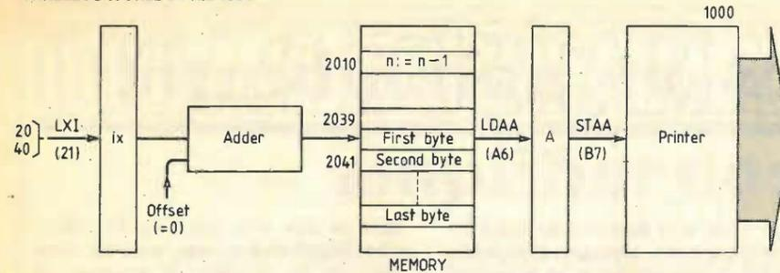
Fig. 12. Programming model for the PRINT problem using the M6800.
