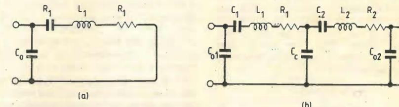
Fig. 13(a) Equivalent circuit of one-port s.a.w. resonator; (b) equivalent circuit of two-port s.a.w. resonator.
