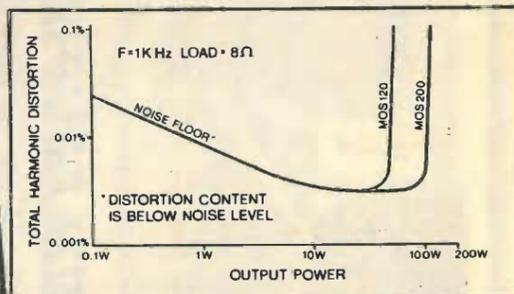
Load impedance both models 4Ω - ∞ Input impedance both models 100KΩ
