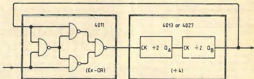
Fig 2(a) divide-by-3 circuit
