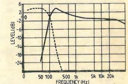
Fig. 2. New crossover frequency of 100Hz is chosen for dual electrostatic + common bass combination.
