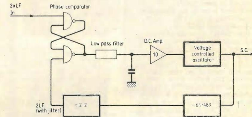
Fig. 7. Phase-locked loop used for synthesis of sub-carrier from twice line frequency.
