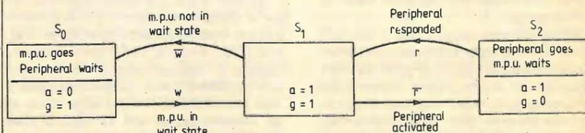
Fig. 4. Internal state diagram of a wait/go interface.
