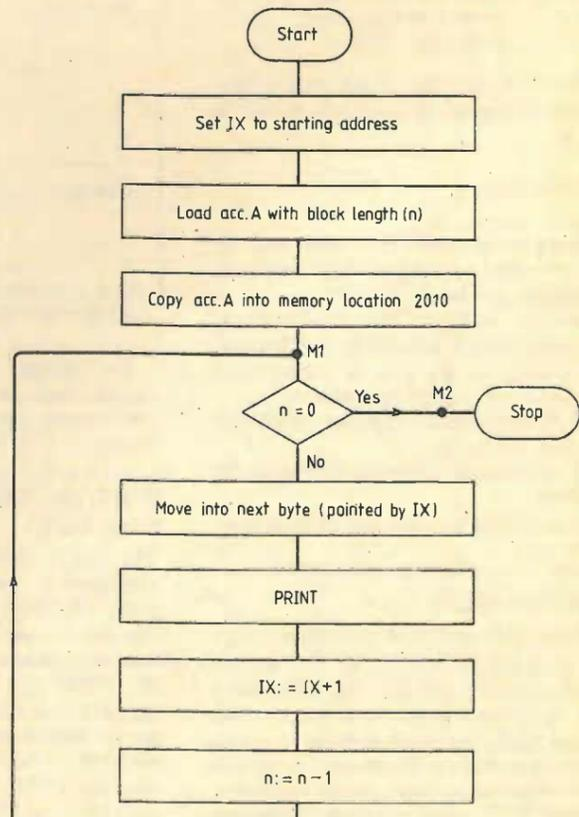
Fig. 13. Programming chart of the PRINT problem using wait/go and the M6800.
