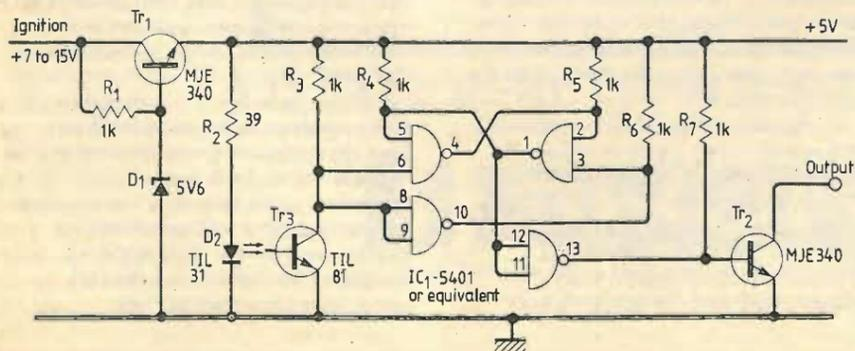
Fig. 1. Switching circuit and regulator. Tr<sub>1</sub> and Tr<sub>2</sub> do not require heatsinks, but should be secured with the screws that hold the p.c.b. in place. Note that IC<sub>1</sub> must be a ceramic type to ensure reliable operation during large temperature changes.
