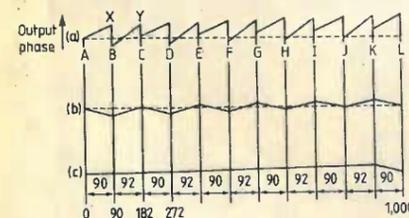
Fig. 6. 756.25 Hz, 378 Hz, and 68.75 Hz jitter components.
