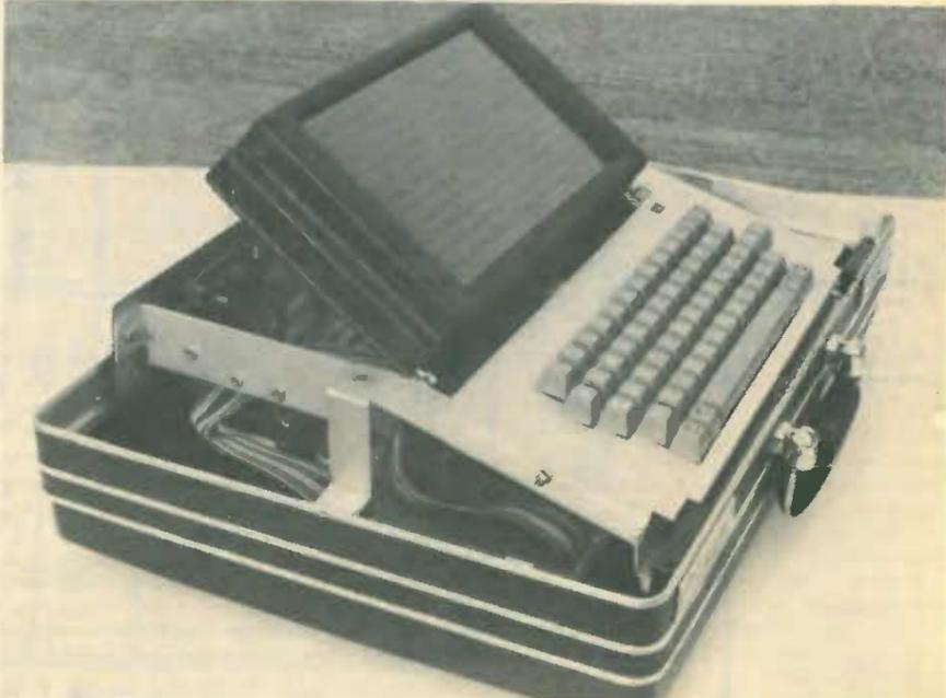
An early prototype of the Microdata model 8400 briefcase computer, now going into production.
