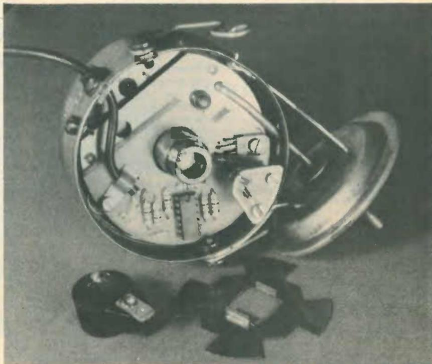
Fig. 2. Printed circuit board mounted on the action plate of a distributor. In the prototype Tr<sub>1</sub> was mounted underneath the board.
