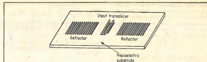
Fig. 12. One-port s.a.w. resonator geometry showing the transducer located between two reflectors.
