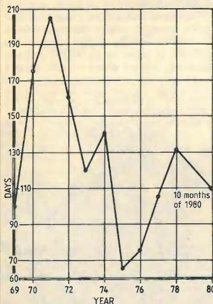
Fig. 5. Solar activity as recorded by the author originally at 136MHz and later at 143MHz (see text). Note that the peak in '71, the low in '75/'76 and the rise thereafter correspond with the recognized cycles.
