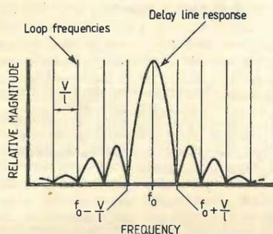
Fig. 18. Loop frequencies and transducer response of s.a.w. delay line oscillator, showing the comb of loop modes, one of which ( $f_0$ ) is selected by the transducer response.
