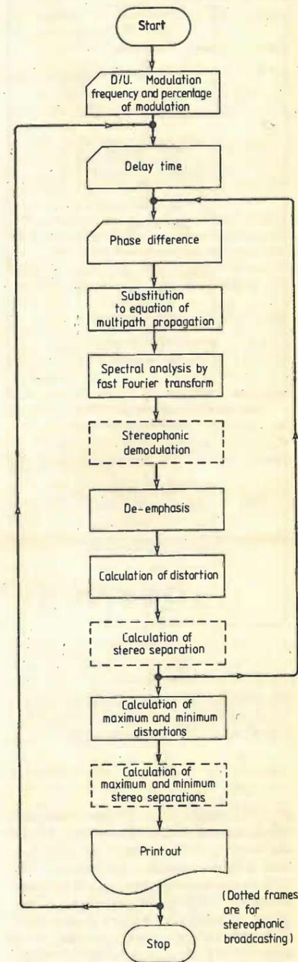
Fig. 1. The procedure used by Mitsuo Ohara (NHK) for computing multipath distortion of monophonic or stereophonic broadcasting.
