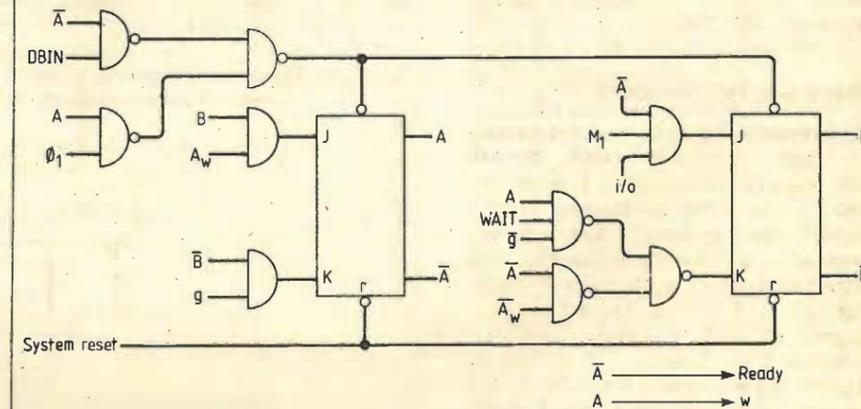
Fig. 9. Circuit implementation of the wait/go logic for the Intel 8080.
