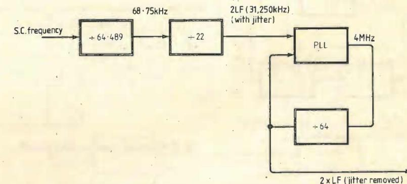
Fig. 2. Twice-line frequency (2LF) derived from sub-carrier frequency.
