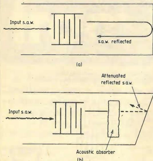
Fig. 10. (a) Spurious s.a.w. reflections from substrate end; (b) suppression of reflections from substrate end. These reflections cause distortion of the filter amplitude and phase responses.
