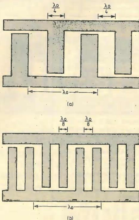
Fig. 11. (a) Conventional 'single electrode' interdigital transducer; (b) equivalent 'double finger' interdigital transducer used to suppress mechanical reflections.
