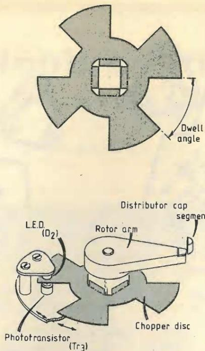
Fig. 5. Typical shape and mounting for the chopper disc. It is imperative that, when the disc just interrupts the light beam, the rotor arm is directly opposite a distributor segment with the vacuum pushrod at mid travel.
