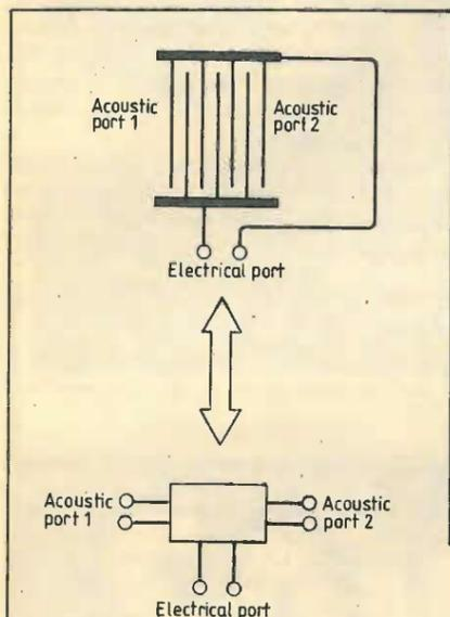
Fig. 9. Three-port nature of the interdigital transducer.
