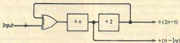
Fig 1(b) Divide-by-(2n-1) with (n-1/2) output
