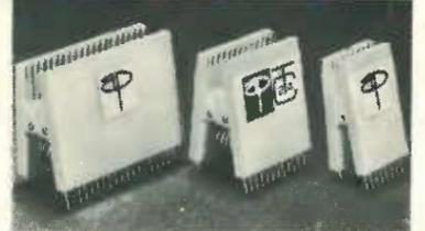
Clip an AP TEST-CLIP over an IC and you immediately bring up all the leads from the crowded board into an easy working level. 22 NEW AP TEST-CLIPS TO PICK FROM
