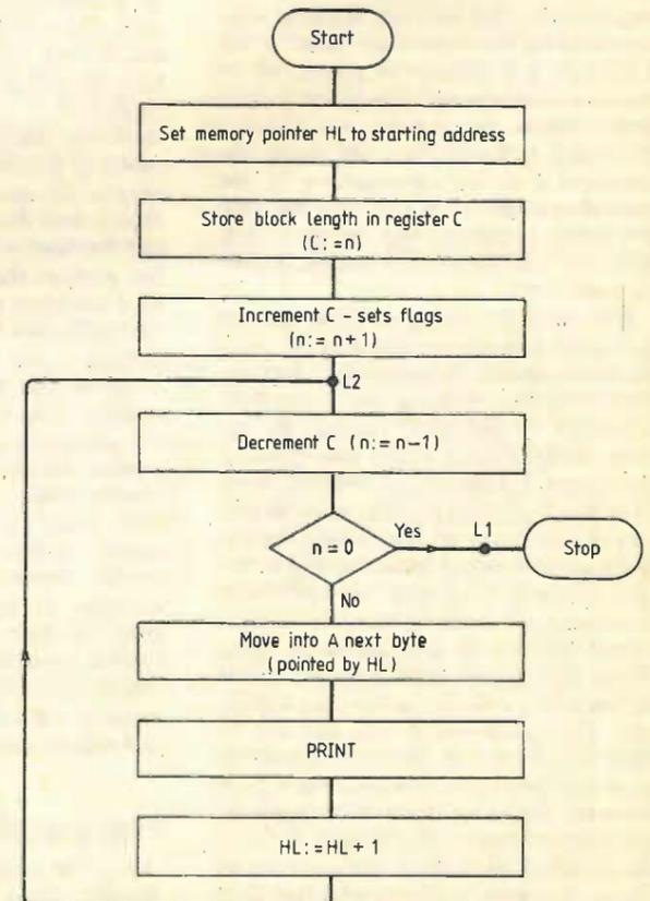
Fig. 15. Programming chart of the PRINT problem using wait/go and the Intel 8080.
