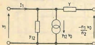
**Question 24.** See diagram. For neutralization  $I_1 = 0$  when  $v_1 = 0$ .
