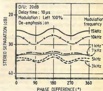
Fig. 4. An example of the relationship between phase difference of an unwanted signal and stereo separation for a D/U ratio of 20dB.
