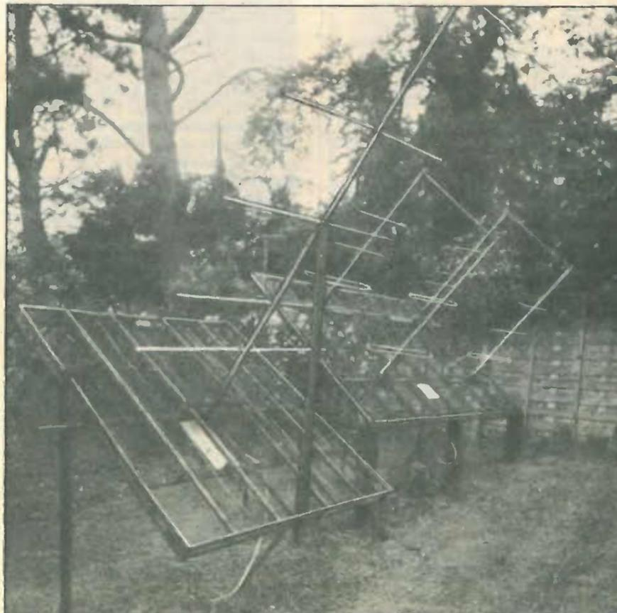
Fig. 2. Four 4-element yagis used to collect radio waves from the sun.
