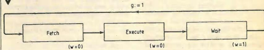
Fig. 3. Block diagram of a wait/go system.
