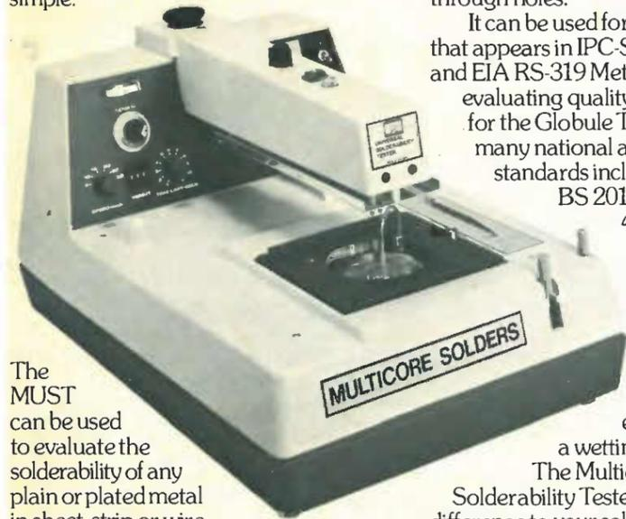
The MUST can be used to evaluate the solderability of any plain or plated metal in sheet, strip or wire form. It is, however, ideal for use with electronic component terminations, metal clad laminate,
