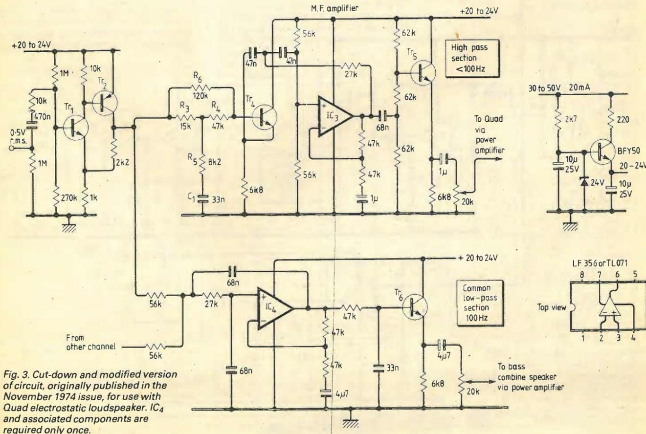
Fig. 3. Cut-down and modified version of circuit, originally published in the November 1974 issue, for use with Quad electrostatic loudspeaker. IC4 and associated components are required only once.
