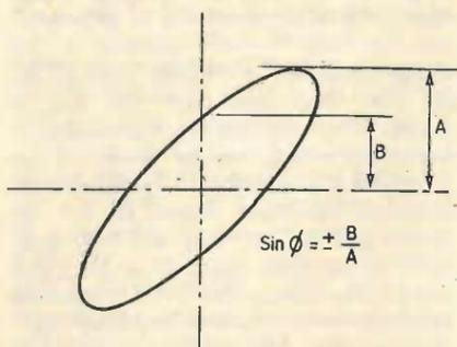
Fig. 1. Phase measurement by the Lissajou figure method. This is difficult, since the graduations on the cursor are usually on the centre line.
