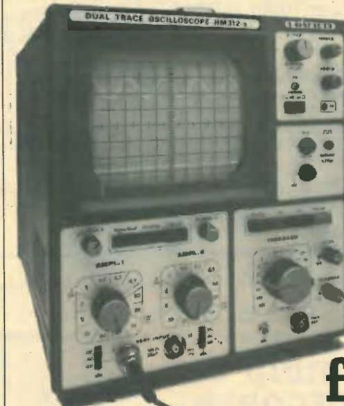
HM312 Dual Trace Oscilloscope. DC-20MHz. Sensitivity 5mV-20V/cm. Time base range 0.5uS-0.2S/cm with x5 horiz mag to 100nS/cm, with variable control uncalibrated to 40nS/cm. CRT screen 8 x 10cm. Full XY using ch II as X input. Bandwidth 2.3MHz. TV trigger.
