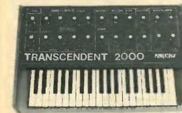
Designed by consultant Tim Orr (formerly synthesizer designer for EMS Ltd.) and featured as a constructional article in ETI, this live performance synthesizer is a 3-octave instrument transposable 2 octaves up or down giving sweep control, a noise generator and an ADSR envelope shaper. There is also a slow oscillator, a new pitch detector, ADSR repeat, sample and hold, and special circuitry with precision components to ensure tuning stability amongst its many features.
