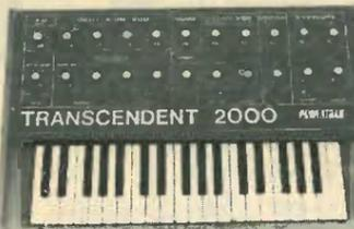
Designed by consultant Tim Orr (formerly synthesizer designer for EMS Ltd.) and featured as a constructional article in ETI, this live performance synthesizer is a 3-octave instrument transposable 2 octaves up or down giving sweep control, a noise generator and an ADSR envelope shaper. There is also a slow oscillator, a new pitch detector, ADSR repeat, sample and hold, and special circuitry with precision components to ensure tuning stability amongst its many features.
