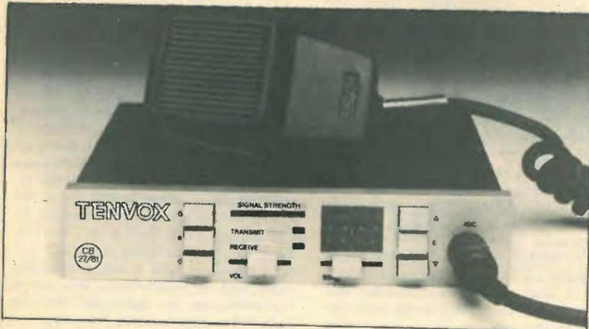
(June issue, p.65) and, as well as being designed and produced in the UK, it uses British made semiconductors, from Plessey, for the r.f. and frequency synthesizer circuitry. In fact the synthesizer circuitry is similar to that published by Peter Chadwick of Plessey Semiconductors in our September issue, p.59-61. Mr Chadwick collaborated with Mr Bryant in the design of the set.
