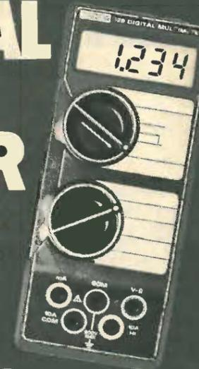
Keithley quality: professional performance. At a price no enthusiast can afford to miss! That's the new 129 from Keithley Instruments - one of the leading names in DMM's. Specification includes ● full 10 amp range ● only one calibration adjustment required per year ● 25 ranges; 5 functions; ac/dc VI and Ohms ● 20,000 hour M.T.B.F. ● Resolution 100µV, 1µA, 0.1% ● 0.8% dc accuracy. The 129 is now available on mail order bringing it to the widest possible market. At the lowest possible price.
