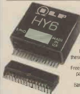
For easy mounting we recommend: B 6 mounting board for modules HY6-HY13 £0.90 inc. VAT. (0.78 ex. VAT.) B 66 mounting board for modules HY66-HY77 £1.12 inc. VAT. (0.99 ex. VAT.) All modules are encapsulated and include clip-on edge connectors. All operate from +15V minimum to +30V maximum, needing dropper resistors for higher voltages. Modules HY6 to HY13 measure 45 x 20 x 40mm. HY66 to HY77 measure 90 x 20 x 40mm.
