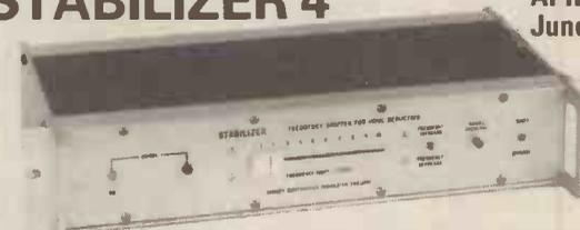
The Stabilizer is a high quality frequency shifter for howl reduction on speech and music. It offers variable shifts either up or down between 1 and 10 Hertz so allowing choice of the optimum shift for the particular acoustics and sound sources involved in each installation. Rack and box versions.
