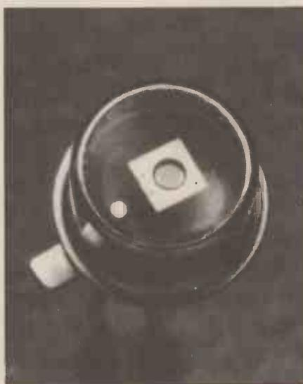
Fig. 6. Silicon reach-through avalanche photodiode is made by diffusion and implantation of dopants into a low-doped silicon substrate. Guard ring lowers electric field at the perimeter of the junction, preventing premature breakdown. Commercial silicon reach-through avalanche photodiode in a TO-18 can is the RCA 3090ZE.
