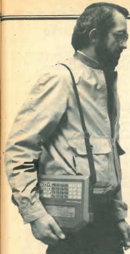
The Husky 144 by DVW Microelectronics is a sturdy, waterproof microcomputer for data entry in the field
