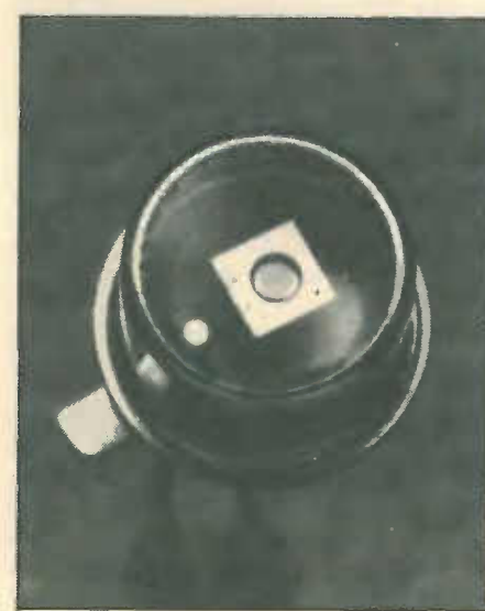
Fig. 6. Silicon reach-through avalanche photodiode is made by diffusion and implantation of dopants into a low-doped silicon substrate. Guard ring lowers electric field at the perimeter of the junction, preventing premature breakdown. Commercial silicon reach-through avalanche photodiode in a T0-18 can is the RCA 3090ZE.
