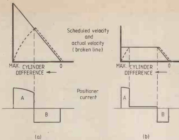
**Fig. 11.** In example (a), dissipation in the positioner is continuous, causing a heating problem. The effect of limiting the scheduled velocity above a certain cylinder difference is shown in (b), where heavy current only flows during acceleration and deceleration. In between, only enough current to overcome friction is required. Back to e.m.f. causes the curver acceleration slope.
