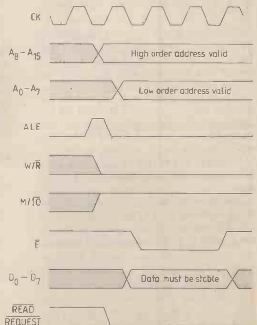
Fig. 15. READ REQUEST enables the appropriate address buffer and sets memory to read mode.
