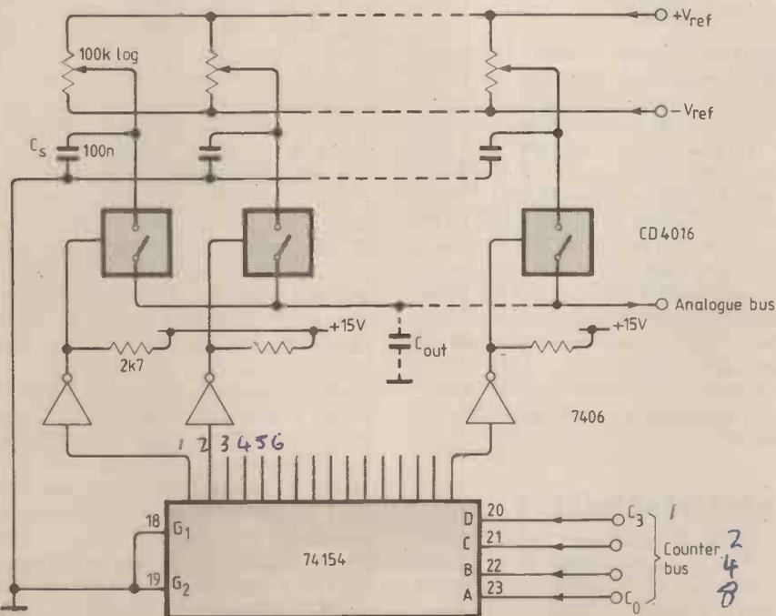
Fig. 11. Address decoding is performed by a 4-bit code.
