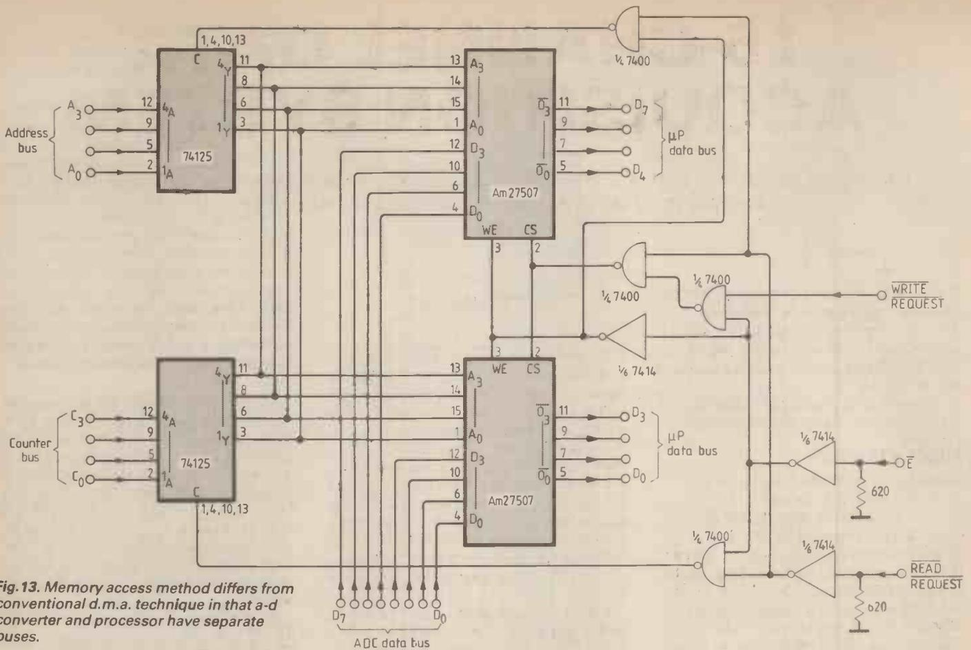
Fig. 13. Memory access method differs from conventional d.m.a. technique in that a-d converter and processor have separate buses.
