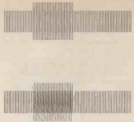
Fig. 8. Parallel bar and Moiré type gratings used to modulate a light beam produce triangle and sine-wave outputs respectively. These gratings are used to detect position and velocity.
