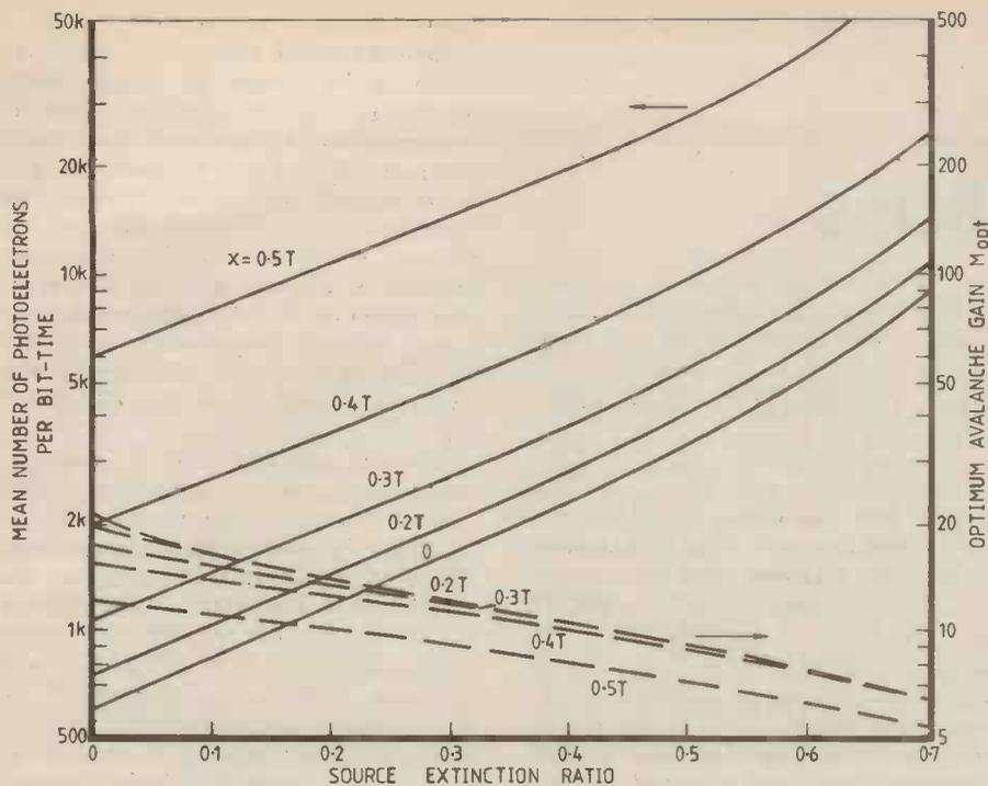
Fig. 13. Receiver sensitivity and optimum avalanche gain as functions of the source extinction ratio, assuming a value of unity for the excess noise factor exponent  $x$ . Parameter  $\alpha$  is the r.m.s. width of the impulse response of the fibre normalized to the bit-time  $T$ , and assumed to be Gaussian for convenience in calculation, ie it is a measure of the bandwidth of the fibre.
