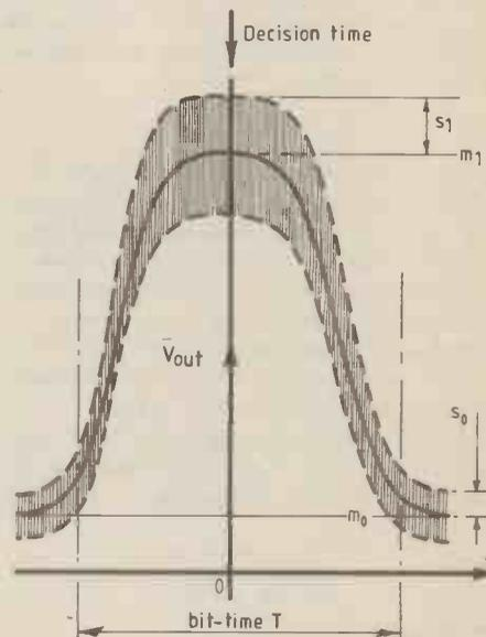
Fig. 9. In the unfiltered output pulse from an optical receiver, the shaded region indicates the variance (mean-square noise voltage), shown to depend on signal level. Mean levels  $m_1$  and  $m_0$  correspond to zero and one bits (spaces and marks). Pulse is slightly dispersed so that some energy is outside the bit-time  $T$ .
