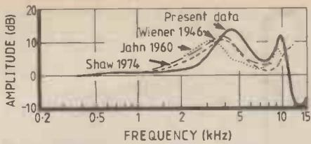
Fig. 1. Filtering effect of the ear canal, showing peaks near 5 and 10kHz, common to all that we hear. All frequencies above 11kHz are much weaker.
