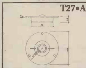
Melnex dome high frequency unit with extended frequency response and wide dispersion.
