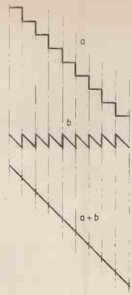
**Fig. 13.** Staircase from a d.-to-a. smoothed by adding a sawtooth waveform.
