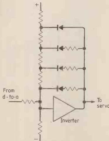
**Fig. 12.** Voltage-dependent feedback around the operational amplifier permits a piecewise linear approximation to a curved velocity profile. This speeds up short seeks without causing dissipation problems on long seeks.
