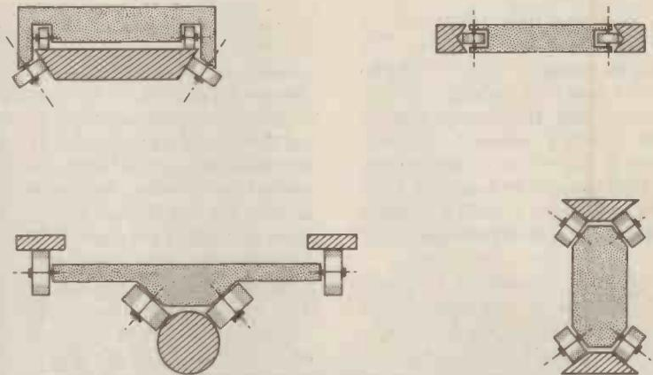
Fig. 1. Four methods used for mounting disc-drive positioner carriages. Common purpose of these is to allow only one degree of freedom, ideally along radius of the disc.
