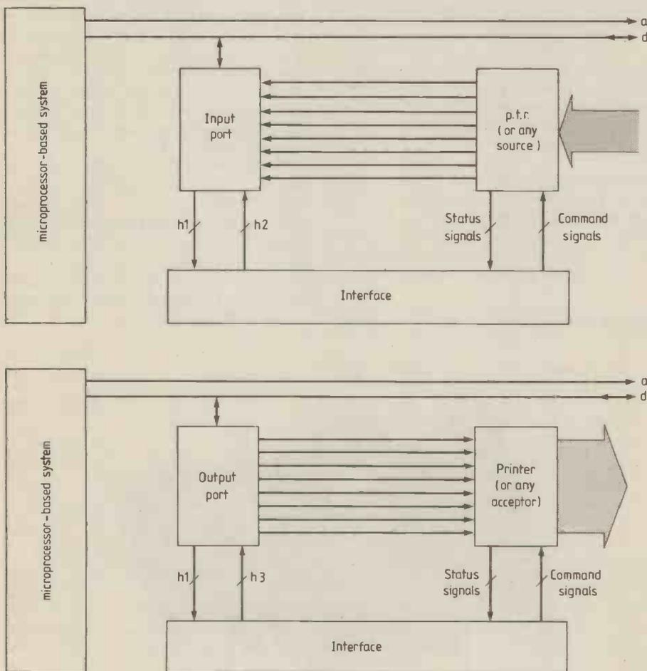
Fig. 5. Microprocessor-based system with input port and source (paper tape reader), top, output port and acceptor (printer), bottom.
