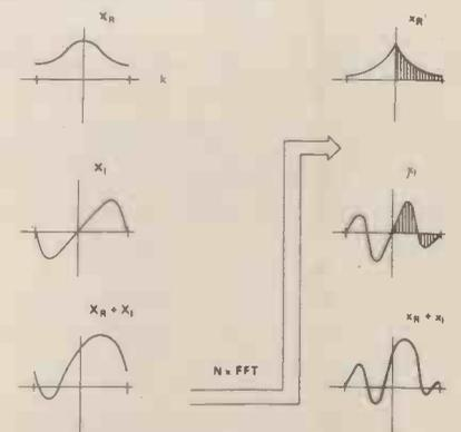
Forward transform. Add the real and imaginary parts for positive and negative time. The negative time section will be located in the second half of the record and can be removed to its correct position before the first half. Zero time will then be in the centre of the record.
