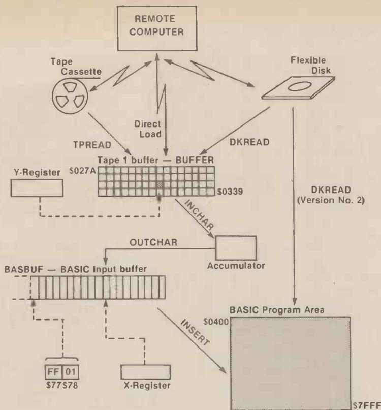
Fig. 4. Data flow diagram for the source code loading program shown in Fig. 3.
