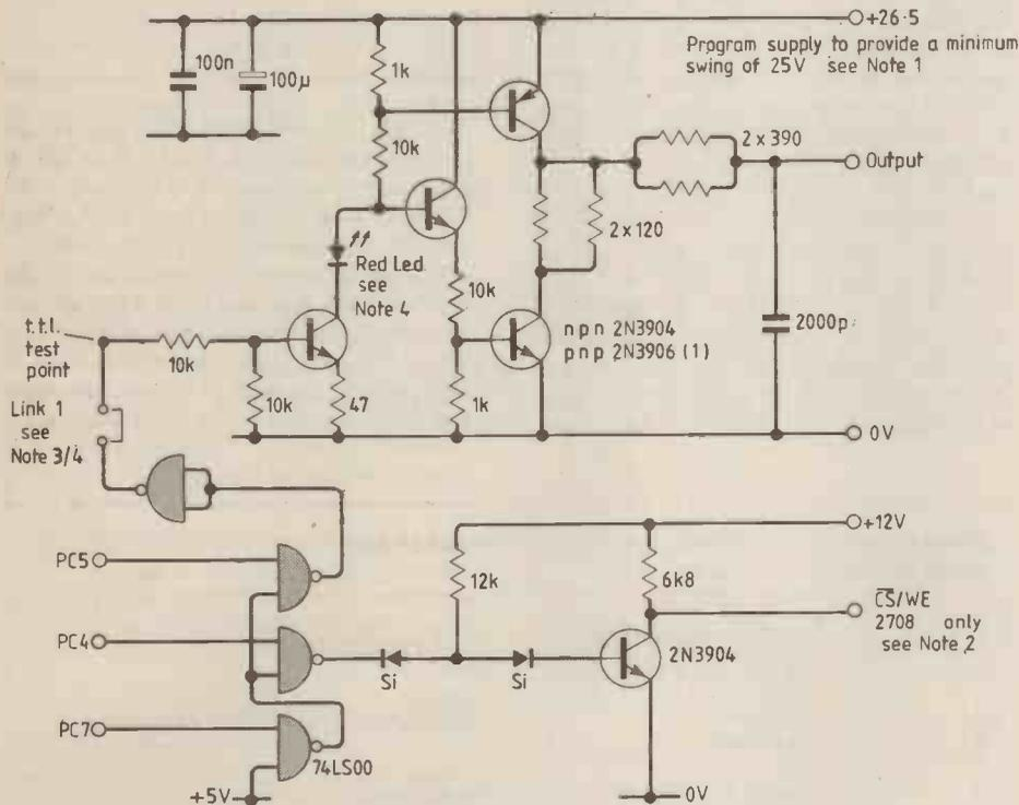
**Fig. 6.** In this transistor interface and reset logic PC7 is used to detect the high impedance state after reset occurs. This prevents unwelcome voltage appearing on the e.p.r.o.m. socket. Normal operation with PC7 = output, logic 0 is  $V_p = 26V$  with PC5 = logic 1. Notes:
