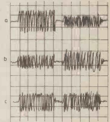
Fig. 16. Alignment disc has flux patterns displaced alternately about the centre line of the reference track. In the resulting oscillograph at (a), the head is too close to the spindle, at (b) too far from the spindle, and at (c), in the correct position.
