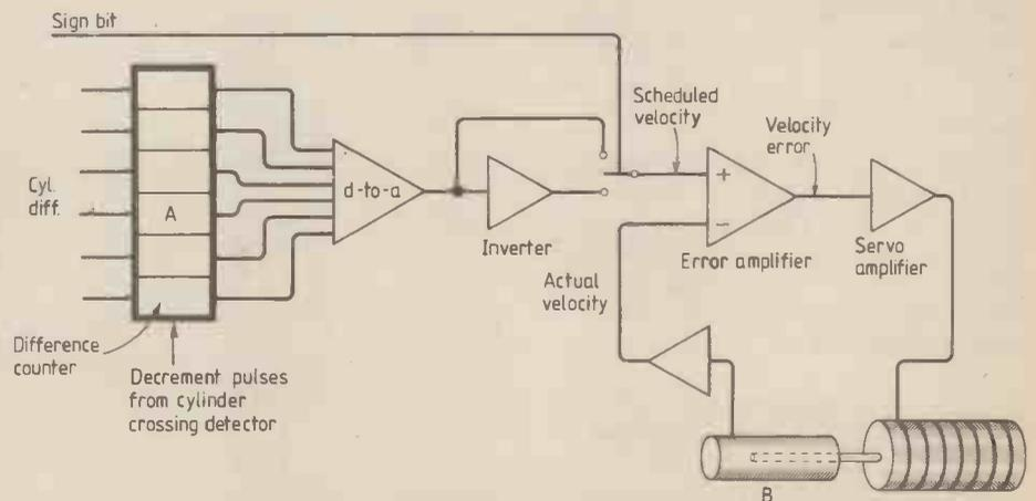
Fig. 10. Carriage velocity control by cylinder difference. Cylinder-difference value is loaded into the difference counter, A. A d-to-a converter generates an analogue voltage, called the scheduled velocity, from the cylinder difference. This is compared with the actual velocity from transducer B to generate a velocity error signal which drives the servo amplifier.
