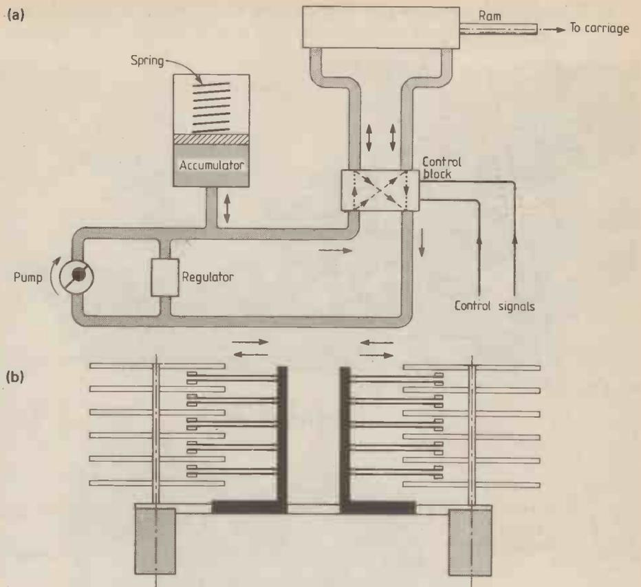
**Fig. 3.** Essential elements of a hydraulic positioner are shown at (a), in which the pressure from the fluid pump is regulated by a bypass valve and control signals from the drive logic operate solenoid valves in the control block. Accumulator permits high peak-flow rates without large pressure fluctuations. In (b), two opposed positioners are used to cancel out reactions caused by fast carriage acceleration.
