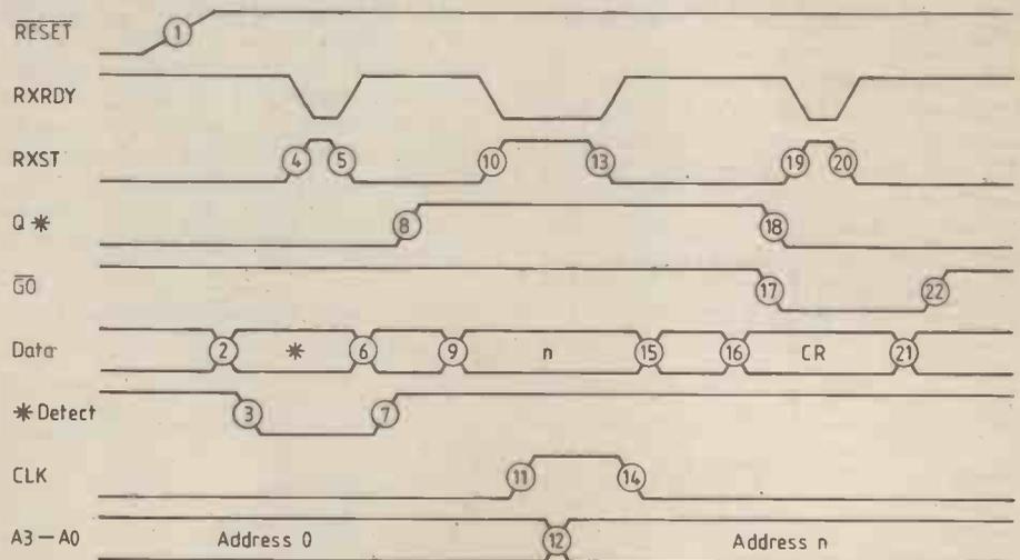
Fig. 9. Conversion cycle timing sequence.
