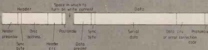
*Representative disc-data block. Header cyclic-redundancy check (c.r.c.) and data-error correction words will be discussed later. The postamble is included to prevent data corruption when the write current is switched off.*
