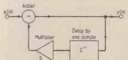
**Fig. 1.** First-order digital filter applies numerical operations to the sampled input signal  $x(n)$  to produce an output  $y(n)$ .
