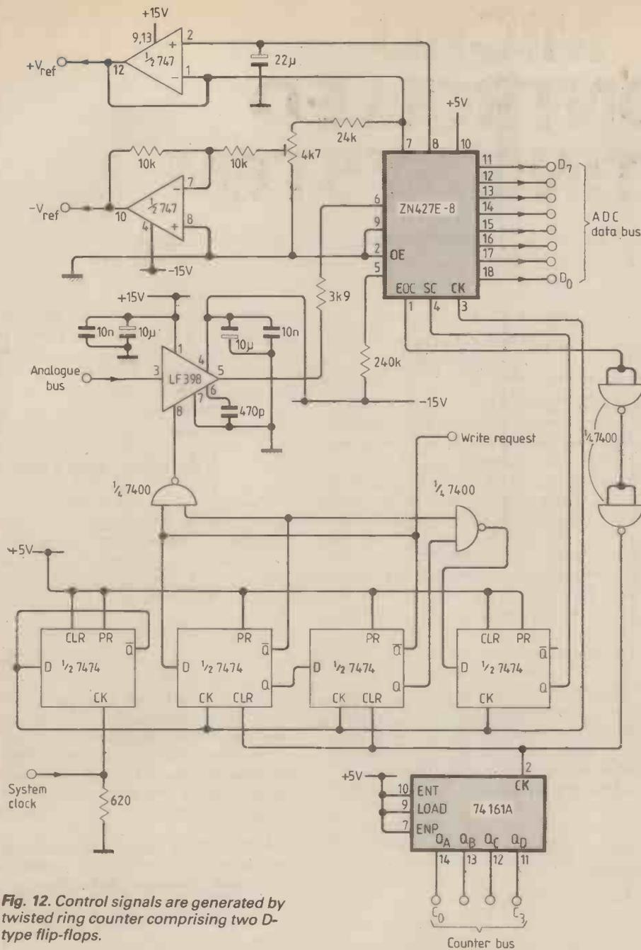
Fig. 12. Control signals are generated by twisted ring counter comprising two D-type flip-flops.
