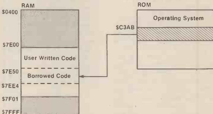
Fig. 2. The function of a source-language loading program. These diagrams, although specifically relating to the PET, are typical of most microcomputers. Underlined sections in (b) indicate the positions in memory of the Basic statement numbers.
