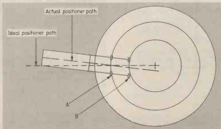
Fig. 2. Mounting read/write heads side-by-side in multi-platter drives reduces height of the disc pack and hence weight moved by the positioner, but alignment between carriage centre line and disc radius becomes more critical. Here, the heads are aligned at track A and the error caused by carriage/track-radius misalignment becomes apparent at B.
