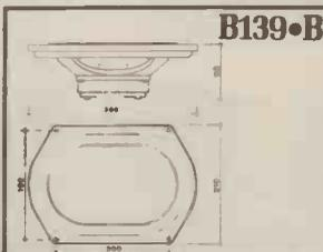
Low frequency unit with full-stressed expanded polystyrene diaphragm and highly compliant surround, suitable for totally enclosed box, reflex, transmission line, horn and other specialised low frequency applications.
