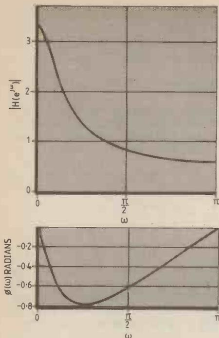
Fig. 4. Frequency response of a digital filter (in this case Fig. 1 with  $b=0.7$ ) characterizes its response to sampled sinusoidal inputs of the form  $A\cos\omega n$ . Amplitude response at top, phase response bottom.
