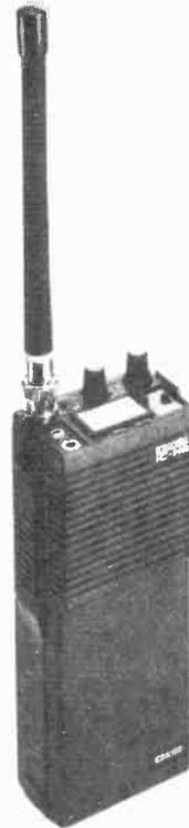
The ICH2 is the first of a new breed of synthesized hand-held radio transceivers. Being synthesized, it requires no crystals to be set on to frequency. All that is required is to lift a recessed panel on the top of the set and cut the correct diodes to program the set to one or two channels. Duplex or simplex is obtained in the same way. This really is a boon to the busy dealer and convenient for the customer who wants those extra few sets "yesterday".
