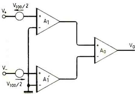
**Fig. 6.** Unequal magnifications of  $V_+$  and  $V_-$  together with offset voltage are taken into account in this class 3 equivalent circuit.
