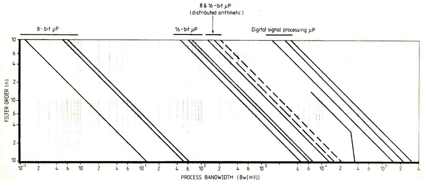
The microcomputer services can be evaluated when implementing a second-order filter; on the other hand, the microcomputer maximum processing speed for an nth-order filter will result from extrapolation as follows:
