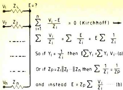
**Fig. 6.** Millman's theorem allows ready calculation of the voltage  $E$  at which a junction will settle. Strictly speaking it is result (a), stated in terms of admittances, and it is useful to abolish denominators in difficult algebra. Form (b) is more useful in easier cases.
