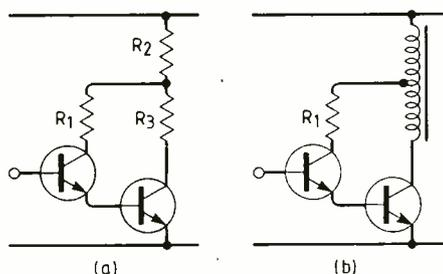
tolerance of current, the drop in  $R_3$  need only be ( $V_{CE\text{ Sat } 1} + V_{BE2} - V_{CE\text{ Sat } 2}$ ), about half a volt, and the load current is then, for the typical case, increased by some 10-15%. The introduction of  $R_1$  gives better control at the price of lower efficiency.
