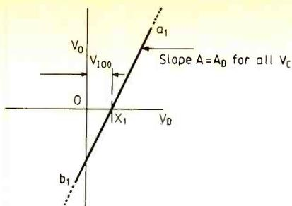
**Fig. 4.** Class 2 op-amps have straight-line transfer characteristic with intercept on the  $V_D$  axis, equal to the input offset voltage,  $V_{I00}$ , arising simply from small differences in the active devices.
