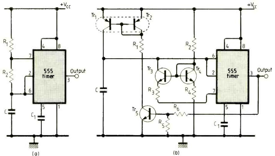
$Tr_1, Tr_2$ . In this case we have to introduce resistors<sup>2</sup> in the emitter circuits of  $Tr_1$  and  $Tr_2$  as in  $Tr_3$  and  $Tr_4$  (the emitter resistor of  $Tr_1$  in this case can be used for frequency control as well). For the current source  $Tr_3, Tr_4$  the resistor  $R_3$  and  $R_4$  are necessary to compensate for the saturation voltage of the 555 inner switch (this voltage can be as large as 0.1V).
