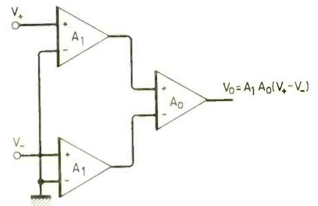
Fig. 3. Common-mode signal is rejected due to identical magnifications, though the signal paths are different, as indicated.
