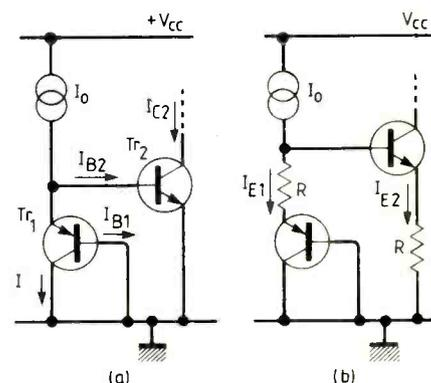
Complementary transistor current mirror with matched transistor (a) and matched emitter resistances (b).
