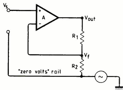
Fig. 4. Amplifier of infinite gain must produce  $V_f$  equal to  $V_s$  even when a voltage source drives the floating "zero volts" rail with respect to which these quantities are measured. Think what would happen if  $V_f$  fell short.
