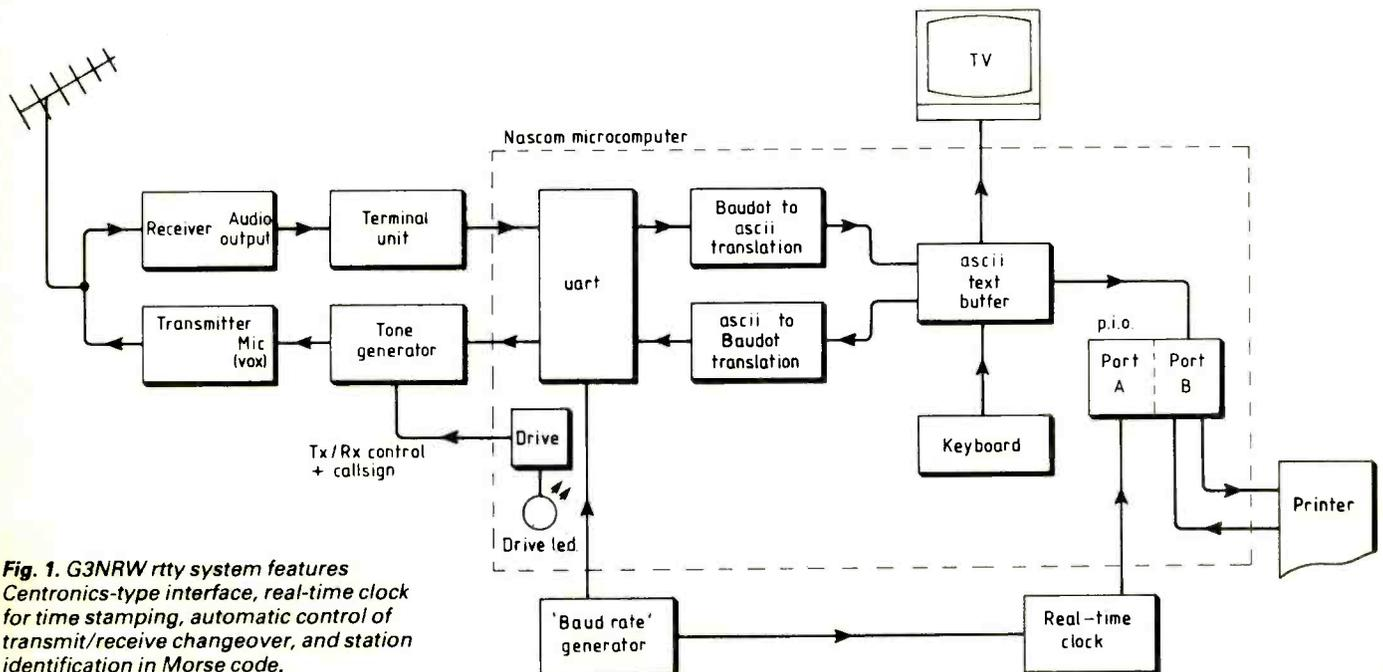
Fig. 1. G3NRW rtty system features Centronics-type interface, real-time clock for time stamping, automatic control of transmit/receive changeover, and station identification in Morse code.
