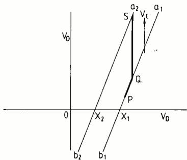
**Fig. 11.** Transfer characteristic of class 3 op-amp comprises a series of parallel lines, two of which are shown, corresponding to the projection of lines such as  $a_2'b_2'$  on the plane
