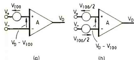
**Fig. 5.** Class 2 op-amp is represented by a class 1 with an offset voltage generator in either of its inputs (a). Alternatively, for analysis, offset voltage can be split into equal components one in series with each input (b).
