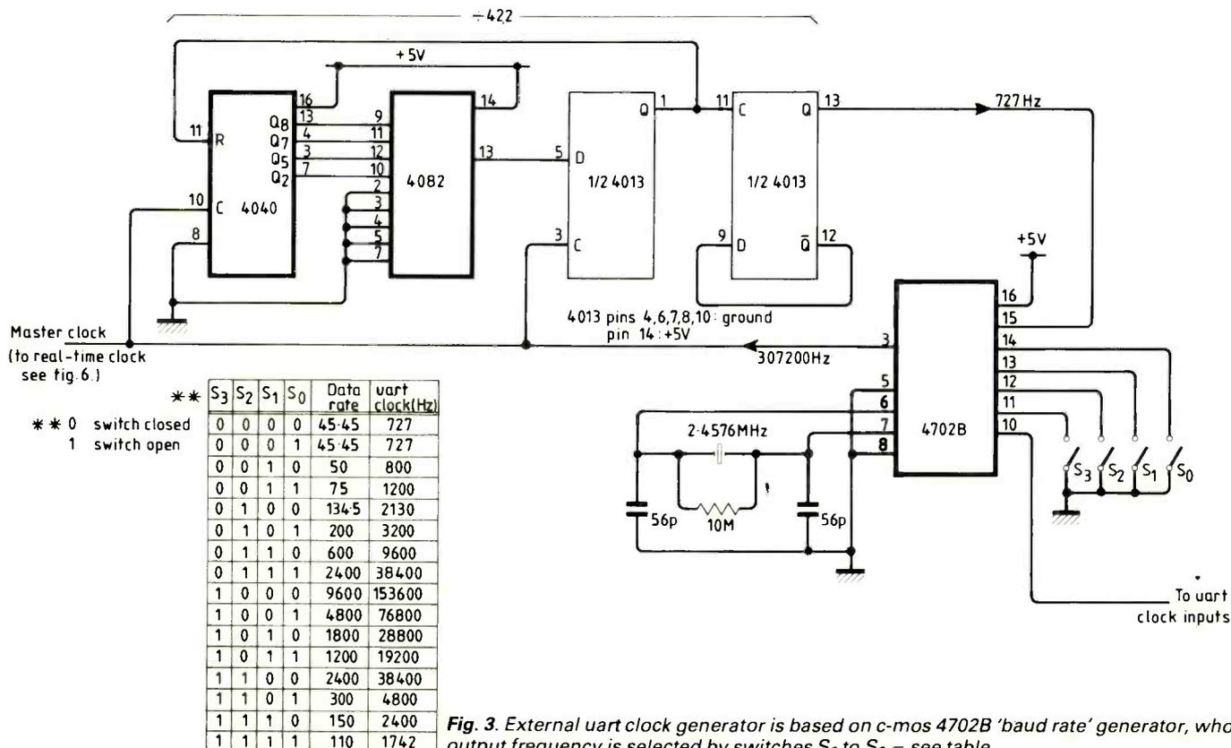
Fig. 3. External uart clock generator is based on c-mos 4702B 'baud rate' generator, whose output frequency is selected by switches S<sub>0</sub> to S<sub>3</sub> - see table.
