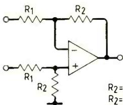
$R_2=3R_1$  for the input stage
