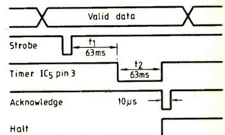
In a Centronics parallel interface a strobe pulse from the computer signals that valid data is available. The computer must receive an acknowledge pulse from the peripheral device before any further data transfer can take place.
