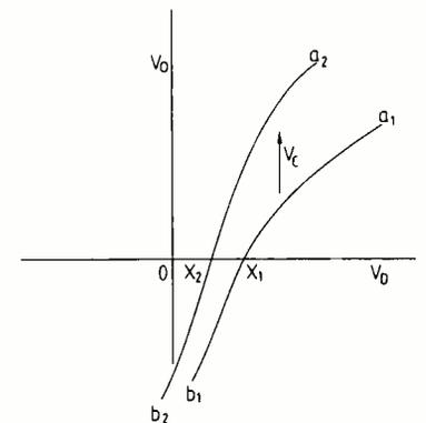
**Fig. 14.** Family of Class 4 transfer characteristics associated with Fig. 13 obtained by projection onto the plane  $V_C=0$  are now neither straight nor parallel.
