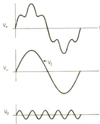
Fig. 2. Common-mode gain for class 1 op-amp is zero so if  $V_+$  and  $V_-$  have the form indicated,  $V_0$  is an amplified version of  $V_D$  only.
