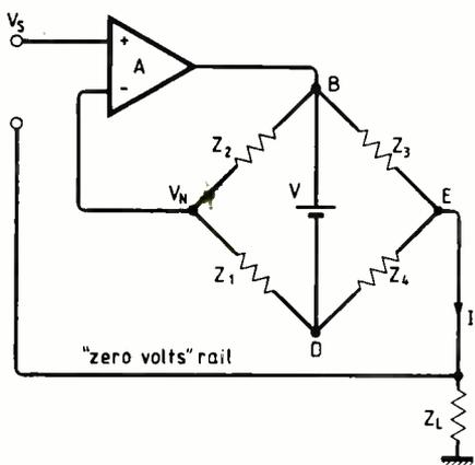
Fig. 5. Modelling the dumpers of Fig. 1 as a voltage source  $V_f$ , Vanderkooy & Lipshitz redraw the circuit as a bridge.
