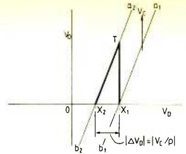
**Fig. 12.** Construction not only gives information about line spacing but also leads to an alternative definition of common-mode rejection that is useful for measurement.
