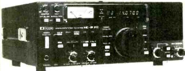
The professional communications receiver for point to point, ship to shore, and general coverage radio work. RANGE 100KHz-30MHz ★ MODES AM, SSB, CW, RTTY and optional FM ★ CPU based 10Hz step digital PLL synthesizer with DUAL VFO's ★ Frequency display 6 digit to 100Hz ★ STABILITY less than 50Hz after one hour ★ POWER SUPPLY 117 or 235V AC and optional 12V DC ★ IF - 1st 70.4515MHz, 2nd 9.0115MHz, 3rd 455KHz, 4th 9.0115MHz ★ Optional transceive units and filters available.
