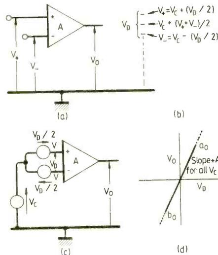
Fig. 1. Symbol for 'quasi-perfect' op-amp uses thickened line to denote non-ideal behaviour (a). Signals  $V_+$  and  $V_-$  can be split into common-mode component  $V_C$  and differential component  $V_D$  (b). Redrawn version (c) emphasizes significance of  $V_C$  and  $V_D$ . This class 1 op-amp is completely specified by transfer characteristic (d).
