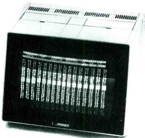
The new microprocessor controlled EP8000 Emulator Programmer will program and emulate all EPROMs up to 8k x 8 sizes, and can be extended to program other devices such as 16k x 8 EPROMs, Bipolar PROMs, single chip microprocessors with external modules.
