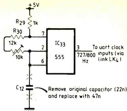
Fig. 2. Modification to 555 clock generator to run the uart at 44.45/50baud. Component numbers refer to those in the Nascom 1 manual.
