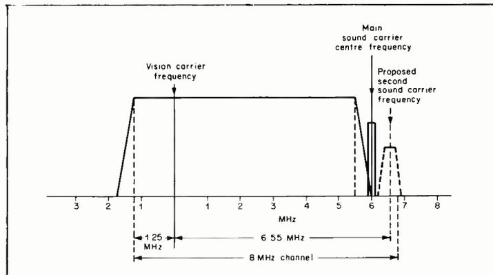
Fig.2. Frequency bands occupied by the colour picture components and sound signal of one television channel with the proposed digital sound signal added.
