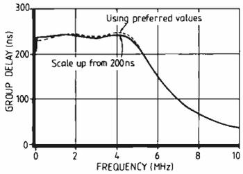
Errors caused by rounding components of Fig.87 (bottom circuit) to preferred values are shown by the group delay response above (Fig.88).
