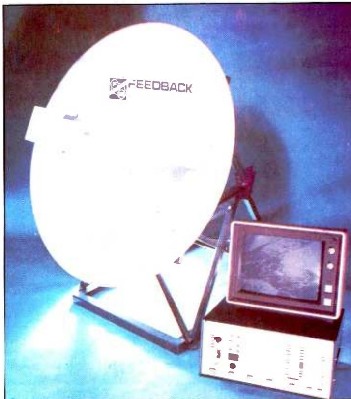
in the dish antenna. The signal from this goes through an r.f. switch which is used to select S-band or APT transmissions. Controls include channel selection, automatic scan synchronization, semi-automatic picture acquisition and the selection of a specific part of the image for storage in the memory. Apart from its obvious uses in weather prediction, the system
