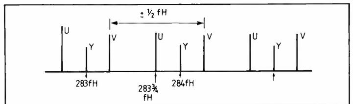
Fig. 10. In PAL, subcarrier must be at odd multiple of one quarter line rate for U and V spectral peaks to interleave with luminance (Y). Unlike NTSC, there is no dominant component at 1/2f<sub>H</sub> points.
