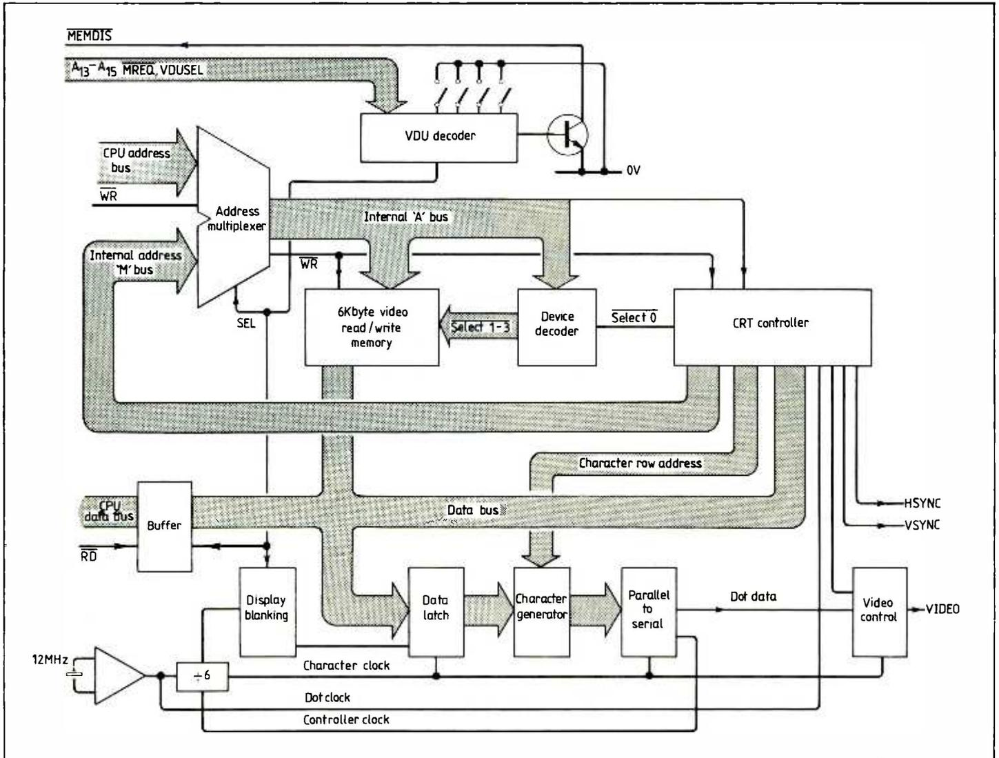
Designed chiefly for fast clear high-density text display, the monochrome v.d.u. section of SC84 is memory mapped and uses the pipelining technique. Output is separate video and sync. signals in either polarity.
