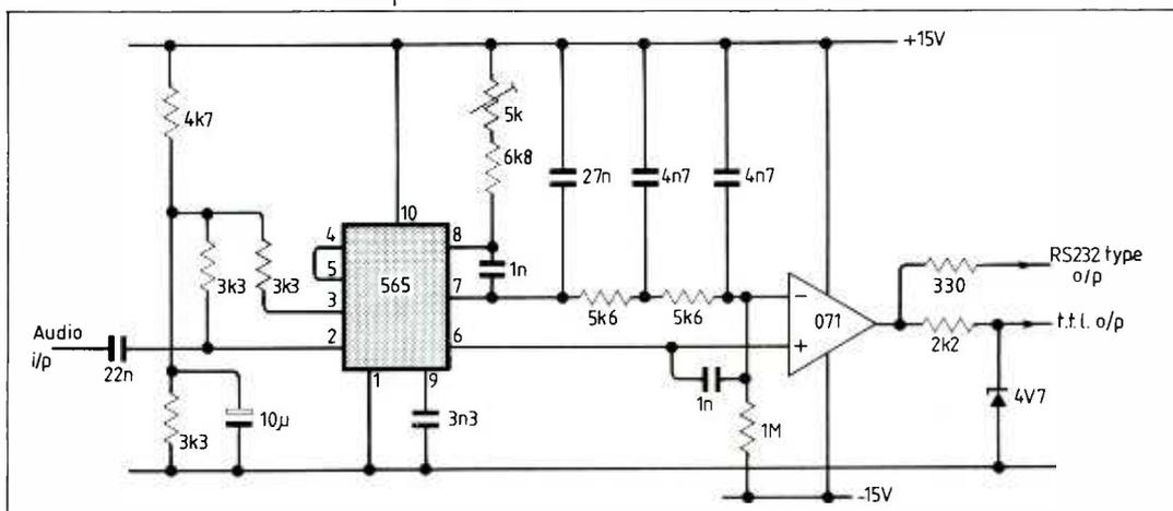
Fig. 7. F.s.k. demodulator, using Signetics 565 phase-locked loop.
