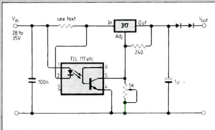
1.5V above control voltage to limit output current under a dead short. Power and resistance ratings of the series resistor are chosen to suit the required current limit and the diodes must
