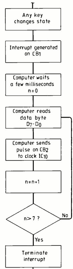
At switch on, the counter is set to zero and its synchronism is checked each time the keyboard is read. The delay allows for key bounce and for the fact that is impossible to play all the notes of a chord simultaneously.
