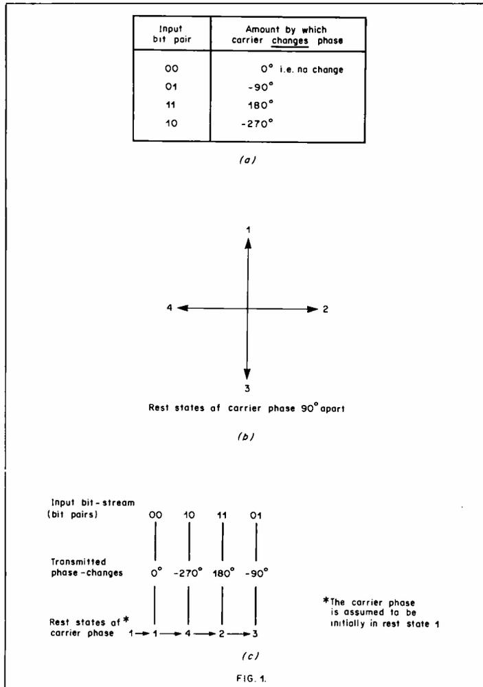
Fig.1. In the differential coding process four bit-pair combinations which modulate the carrier cause it to change phase by the amount shown in the table (a). Carrier has four possible rest states 90° apart (b). An example of carrier rest states adopted for the input bit-pair sequence 00, 10, 11 and 01 is shown in (c).
