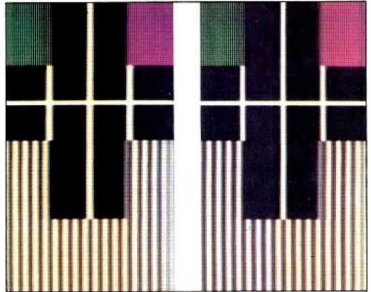
**Fig. 100. Resulting picture improvement with scan-velocity off and on (screen photographs taken from a Mullard report).**
