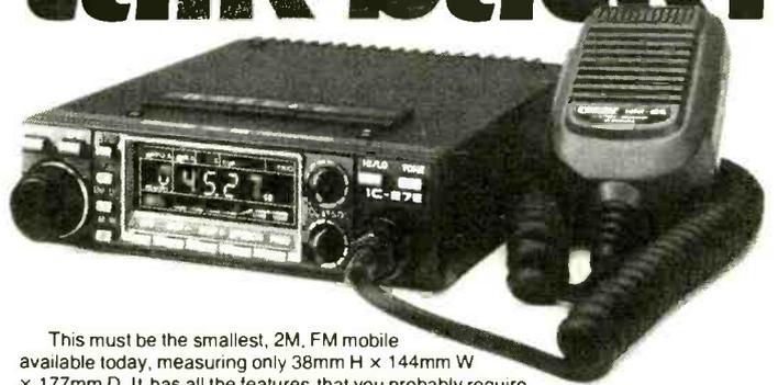
This must be the smallest, 2M, FM mobile available today, measuring only 38mm H x 144mm W x 177mm D. It has all the features that you probably require included in this microprocessor controlled unit. In addition, if you feel lonely and can't find anybody on the band, just press "speech" and the optional built in speech synthesizer will tell you the frequency you are tuned to. This is a boon to the blind operator or to those that tuck their rigs out of sight.
