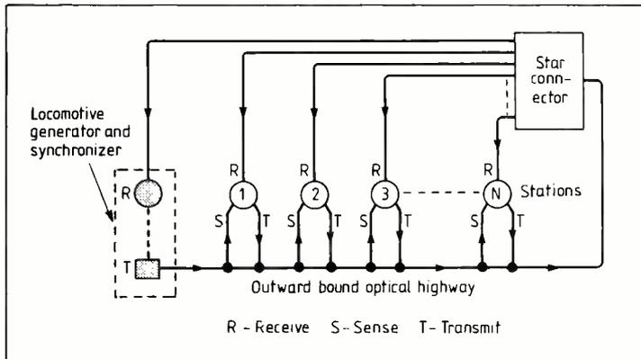
**Fig. 6. D-Net optical lan combines a data highway and a star return, making it more like an open ring.**
