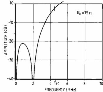
**Fig. 94. Amplitude performance of the chroma path filter.**
