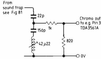
**Fig. 93. Circuit of modified chroma-path filter when using the better i.f. s.a.w. filter. Subcarrier (equivalent frequency 35.067MHz) is only 0.5 to 2dB down.**
