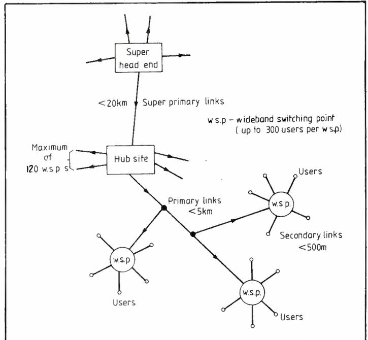
Fig.4. British Telecom's proposed multi-star wideband network will use fibre optics in all but the short final link to the customer.
