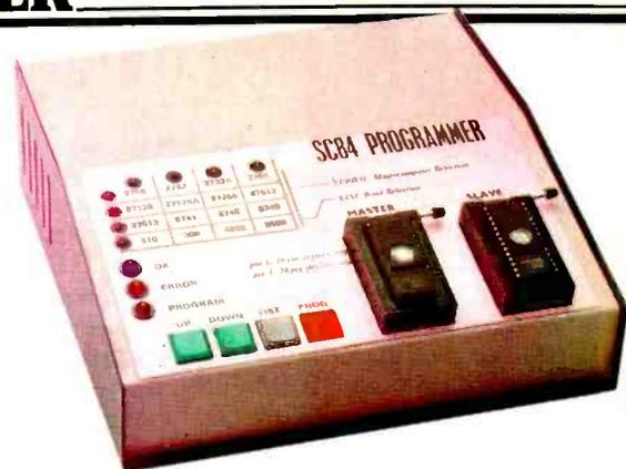
Having its own processor, this intelligent programmer can quickly copy eproms up to the 27512 and list eprom data on a serial printer — under computer control it programs one-chip microcomputers. Part two discusses computer control software and construction.
