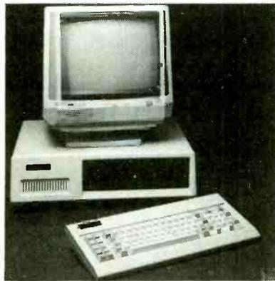
The PC-16 16-bit computer provides PERFECT COMPATIBILITY with the IBM PC/XT range. The motherboard can be supplied in two versions for stereoscopic convenience. The 'N' version has no memory on board and the 'B' version with space for 64 to 256K RAM. Addition of the Memory Expansion Card provides a further 64 to 512KB of RAM. BASIC FEATURES INCLUDE:
