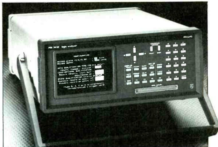
reference data and compare with incoming data on the instrument. Each of the 32 channels may be examined to a depth of 1000 samples or four channel to a depth of 8000. A further option is an RS232C interface card.
