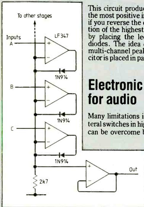
This circuit produces an output equal to the most positive input (or most negative if you reverse the diodes). Visual indication of the highest input can be obtained by placing the leds in series with the diodes. The idea can also be used as a multi-channel peak-hold circuit if a capacitor is placed in parallel with the resistor.
