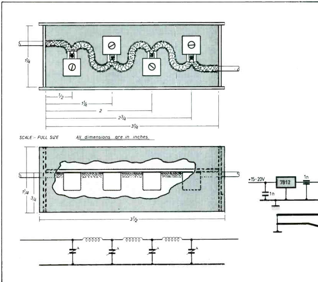
Fig. 2. Circuit diagram of the u.h.f. oscillator and filter. Pin numbering of the mixer module may vary with different makes.
