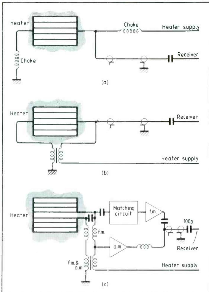
Fig. 3. A demister may be used as an aerial, with the demister isolated from the heater supply circuit by simple chokes (a). In (b), a single bifilar-wound choke ensures that the d.c. magnetization is eliminated. (c) Shows the complete demister aerial system incorporating a vhf matching circuit and pre amplifiers for both a.m. and f.m. bands.
