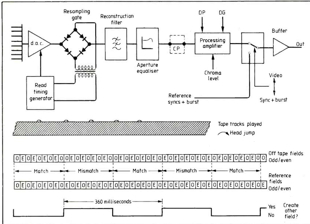
Fig. 3. Simplified d-to-a and output subsystem converts memory samples to analogue video and adds reference sync pulses and bursts. For varispeed a colour processor is necessary and this is connected at 'CP' if colour processing follows timebase correction.
