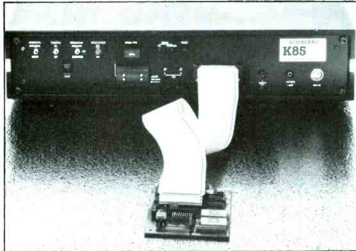
port provided, or downloaded to another computer through the RS232 link. Text files produced by the K85 are Wordstar compatible and editing may be carried out on the second computer if the K85 is in use for emulation.
