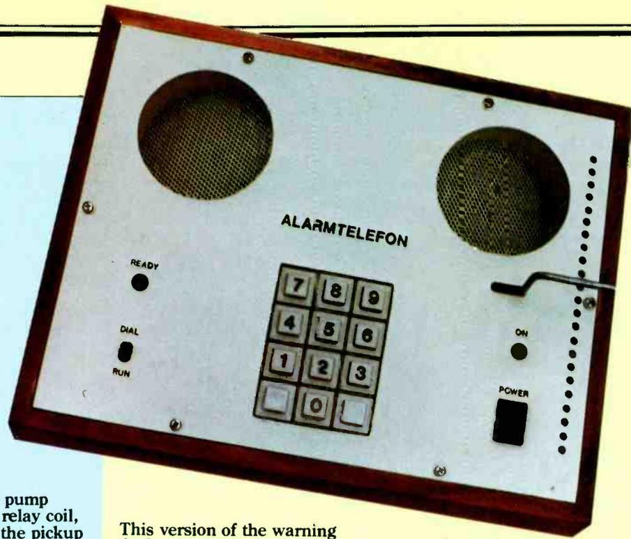
small loudspeakers one as the transmitter and one as the receiver. The machine is placed beside the telephone in such a way that permits the solenoid arm to hold the hook switch deactivated.
