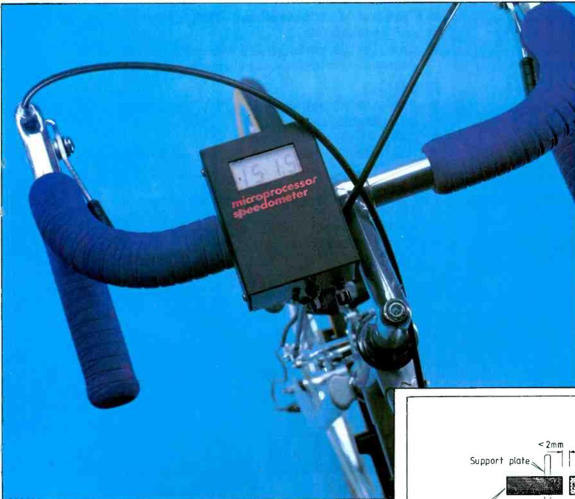
To keep all the components within a reasonably sized box, the display and its driver reside on a separate board, and electrical contact between them is through a series of soldered 5cm long wires. For compactness, the display is mounted directly above its driver; the height gained as a result allows the display to be placed close to the transparent cover above the slot cut in the lid.
