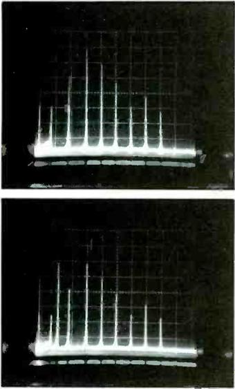
Fig. 4. (top) 50MHz comb generator pattern. This tuner had an unusual problem, a spread caused by changing voltage-frequency ratios at the low as well as the high frequency end.
