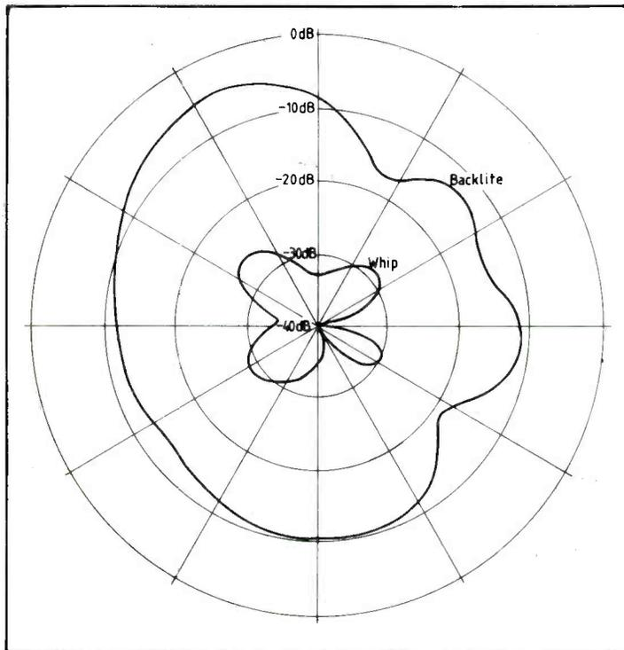
Fig. 7. Horizontal polar diagram of Ford Orion demister aerial with horizontally-polarized signals — compared with a quarter-wave whip in the centre of the roof. The demister aerial gives substantially greater signal voltages and less variation with direction.
