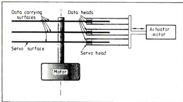
Fig. 3. Low-density magnetic-disc store in which one disc surface carries only servo information.
