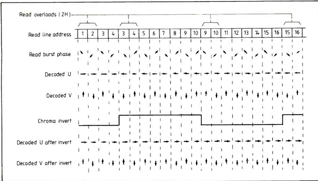
**Fig.7. Example of chroma inversion.** In reverse shuttle, read overloads occur periodically, causing two memory lines to be re-read (3,4;9,10;15,16). Owing to the PAL four-line sequence, this causes chroma inversion, decodes of U and V being in error. Chroma invert signal, effectively Overload/2, compensates for overload by inverting chroma before decoder. In forward shuttle, write overloads have similar effect except that overload is stored in chroma invert memory until line is read.
