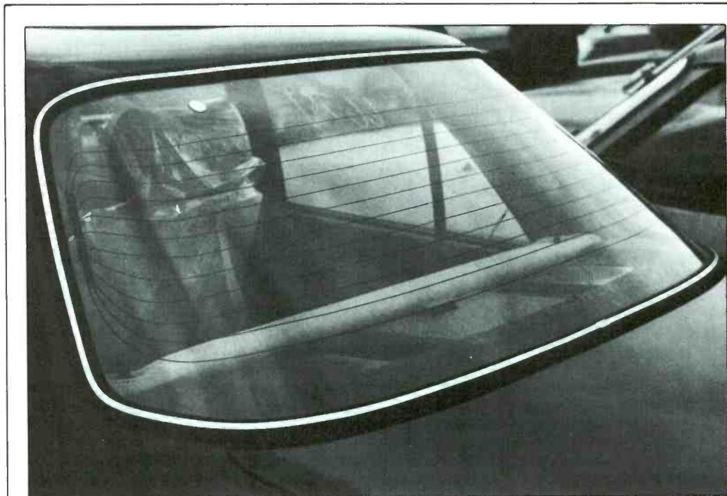
Fig. 5. Ford Orion demister aerial. The folded heater pattern allows both heater connections to be made via a single isolator unit.
