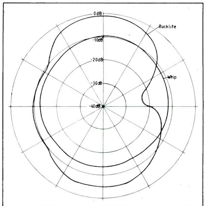
Fig. 8. Horizontal polar diagram of Ford Orion demister aerial with vertically-polarized signals. The demister aerial provides a performance comparable to the roof-mounted quarter-wave whip which, in this case, is greatly superior to the standard wing-mounted car radio aerial.
