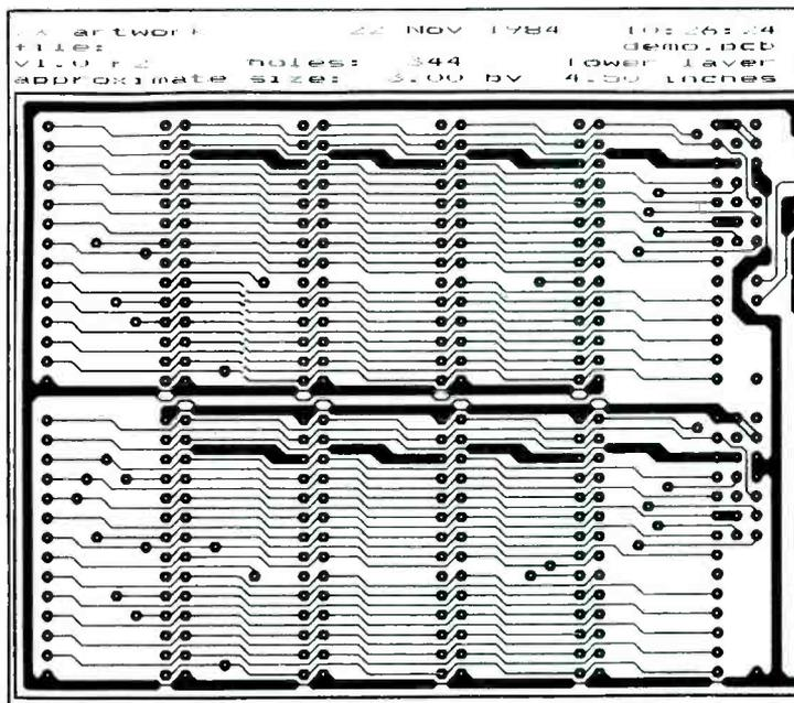
Artwork produced on an Epson dot-matrix printer. The X2 printout is here reduced to approximate board size.
