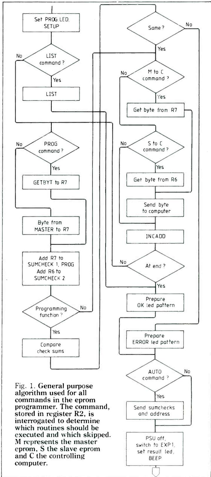
Fig. 1. General purpose algorithm used for all commands in the eprom programmer. The command, stored in register R2, is interrogated to determine which routines should be executed and which skipped. M represents the master eprom, S the slave eprom and C the controlling computer.
