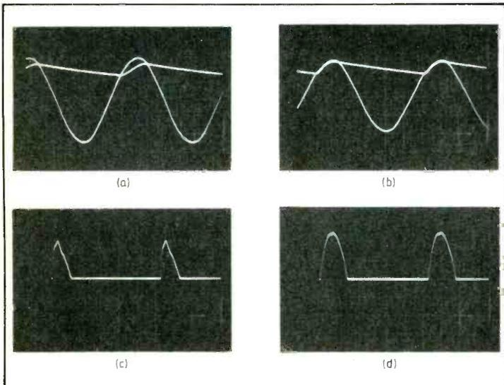
Fig. 5. These oscillograms were taken with the circuit conditions described in the text and in Table 1. The current waveforms especially show the degree of approximation assumed when taking the pulses in (c) and (d) as sine wave 'caps'.
