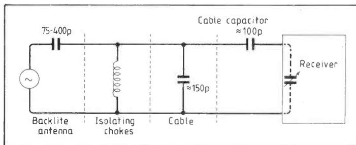
Fig. 4. Equivalent circuit, for medium and long waves, of the demister aerial with isolating chokes and standard car-radio extension cable incorporating series capacitor. Aerial and cable capacitances form a potential divider which reduces the signal voltage at the receiver aerial terminals.
