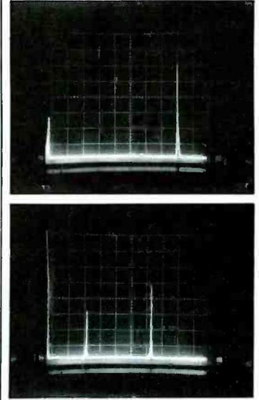
Fig 6. (top left) A signal at 100MHz into the completed mixer-oscillator unit (see text).
